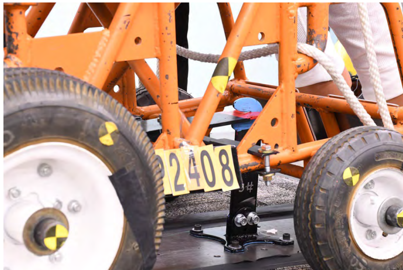
Figure 5. Q'Straint QLK™ Stabilizer Bracket, as used on the test wheelchair
