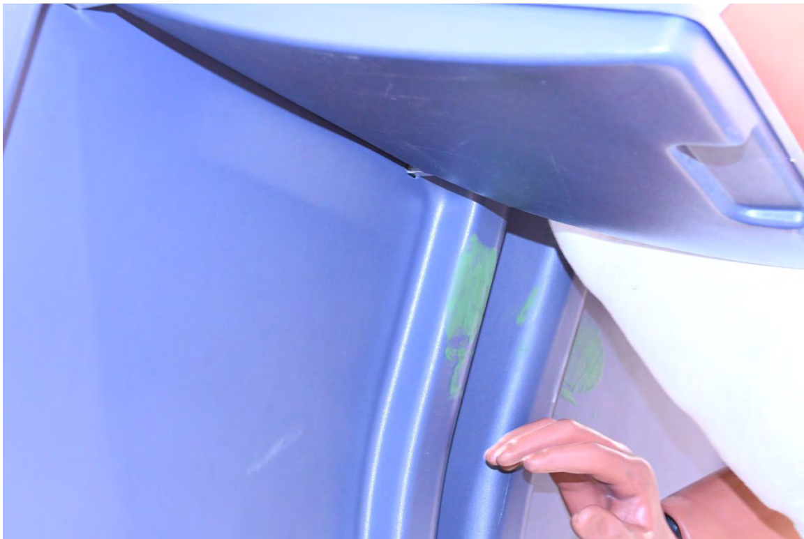
Figure A76. VP2409 Post-test Knee Contact Point on Back of Commuter Rail Seat
