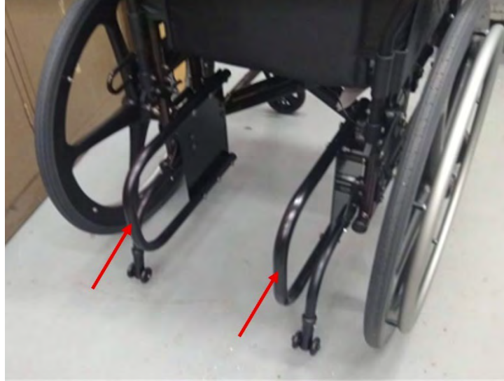
Figure 2. Example of the UDIG Prototype Hardware on a Commercial Manual Wheelchair
