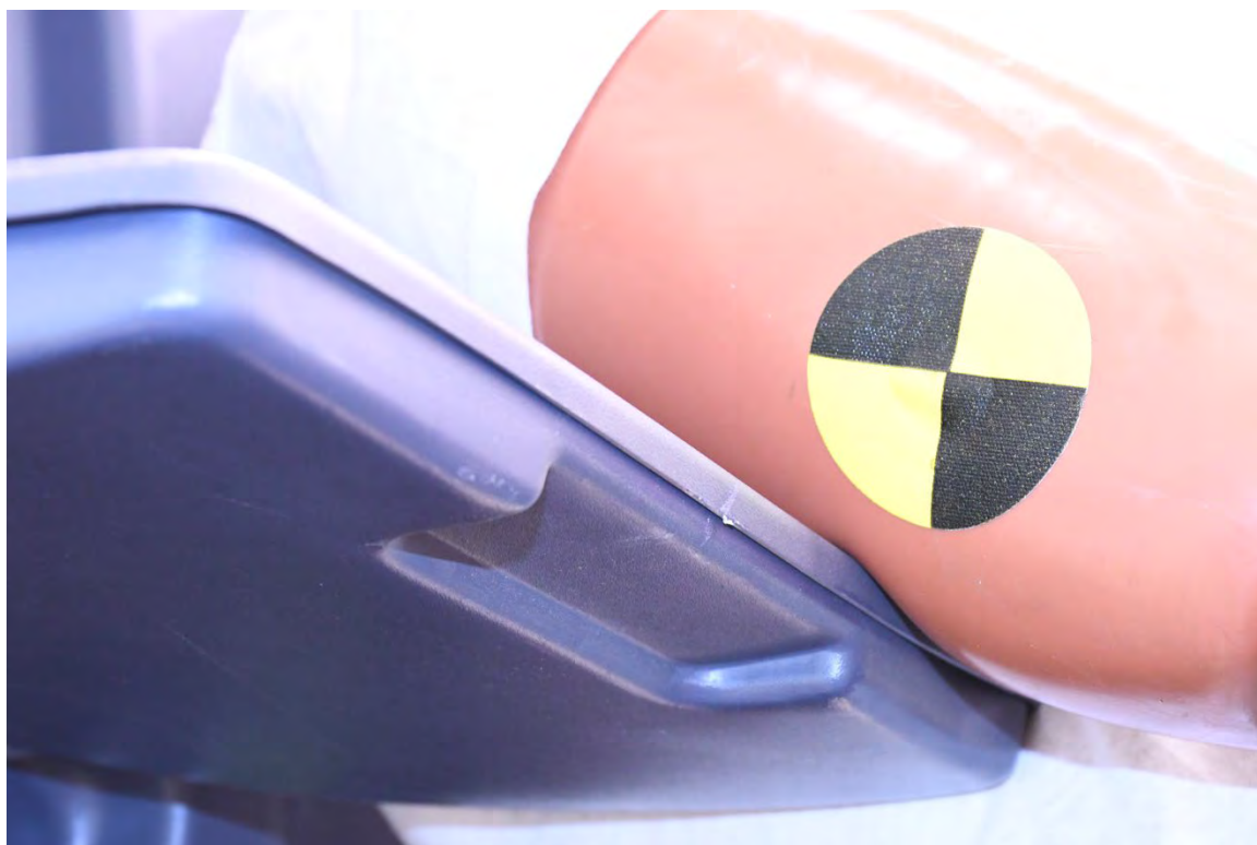
Figure A78. VP2409 Post-test Closeup of ATD Arm Contact with Commuter Rail Seat Tray
