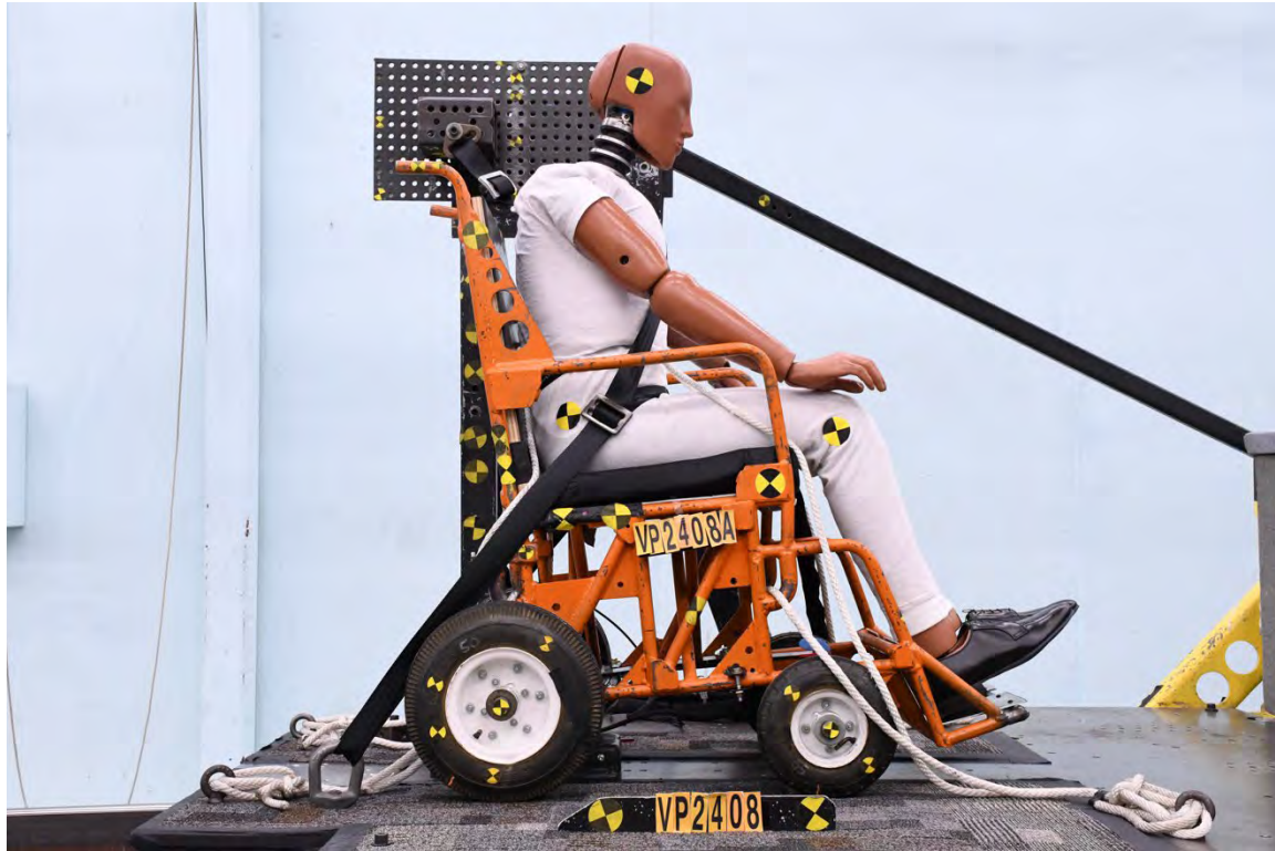
Figure A38. VP2408 Post-test Side View
