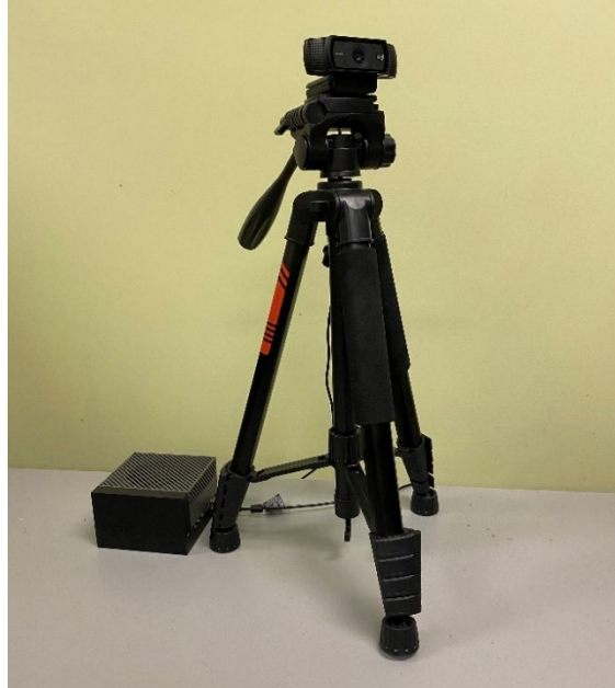
Figure 28. Real-time monitoring video capture module hardware implementation
