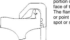
steel wheel gage (hook gage). The shank, or long flat portion of the gage must be held flat against the back face of the rim and parallel to the radius of the wheel. The flange will sit in the hook portion and will hold the tip or point of the gage clear of the tread. Gaging in a flat spot or shelled spot is not acceptable.
