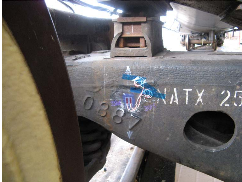
Figure 4. Strain Gages Measuring Bolster Side Bearing Loads
