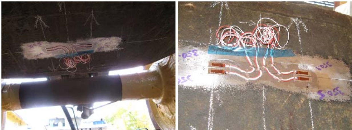
Figure 5. Strain Gages Measuring Bolster Center Bowl Load
