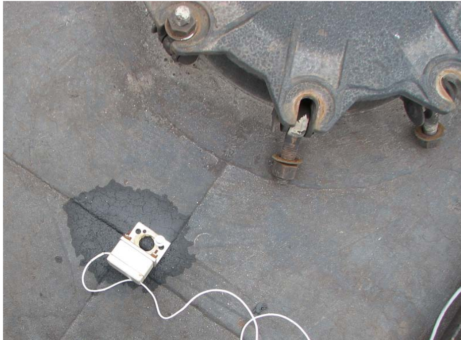
Figure 6. Triaxial Accelerometer Mounted on Top of Carbody
