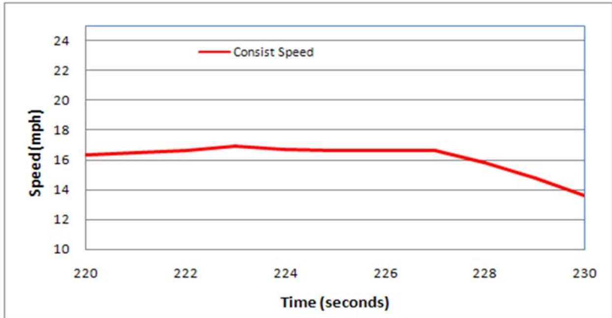
Figure 16. Deceleration of the Consist causes High Positive Longitudinal Coupler Forces
