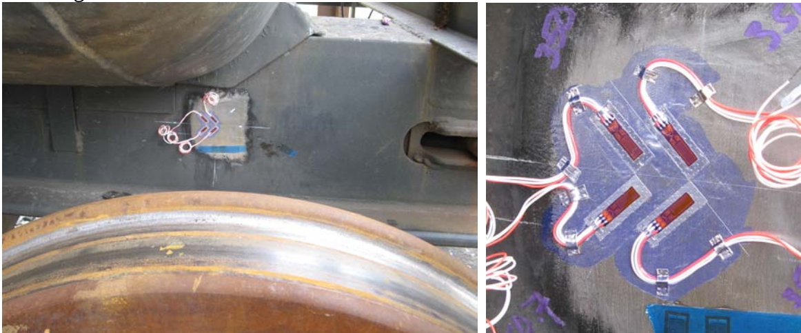
Figure 1. Shear Gages Measuring Vertical Coupler Force
