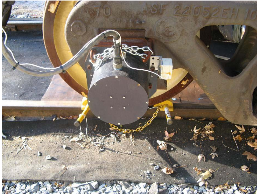
Figure 6. Vertical Accelerometer Mounted on the Axle on Both Sides of the Car
