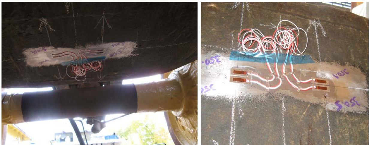
Figure 3. Strain Gages Measuring Bolster Center Bowl Load
