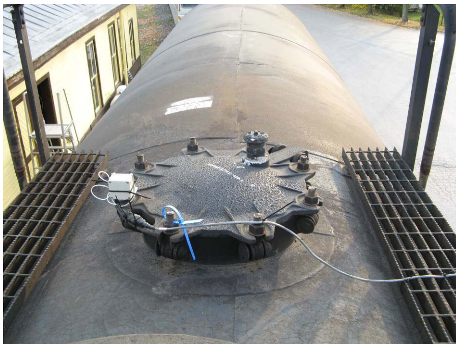
Figure 4. Triaxial Accelerometer Mounted on Top of Carbody
