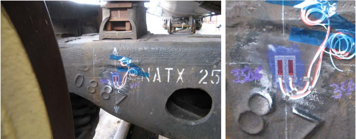
Figure 2. Strain Gages Measuring Bolster Side Bearing Loads
