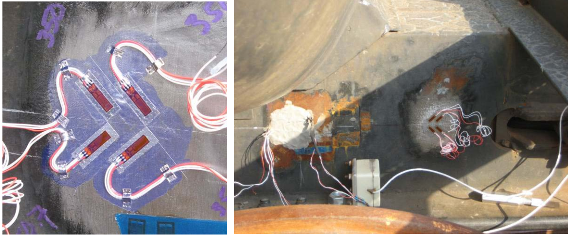
Figure 3. Shear Gages Measuring Vertical Coupler Force. Left: Close up of installation. Right: New gages on the right replace gages (covered with sealant) on the left which were then disconnected
