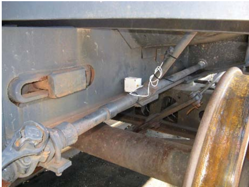
Figure 7. Vertical Accelerometer Mounted on the Stub Sill and Each End of the Car
