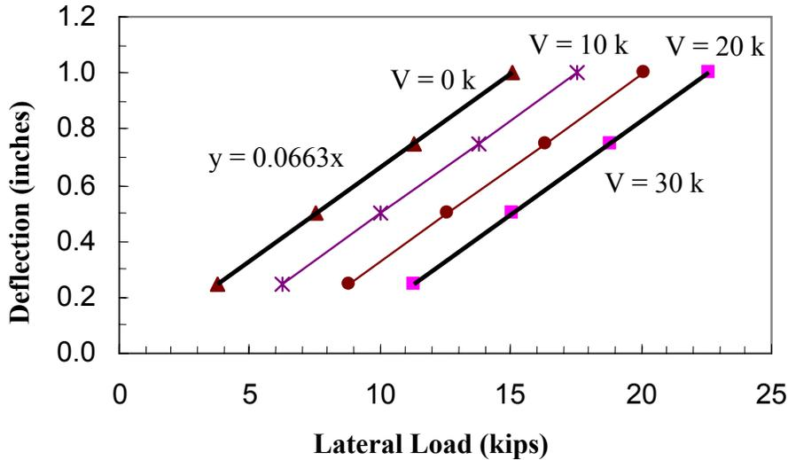
**Figure 5. Lateral load-deflection trends for different vertical loads**
