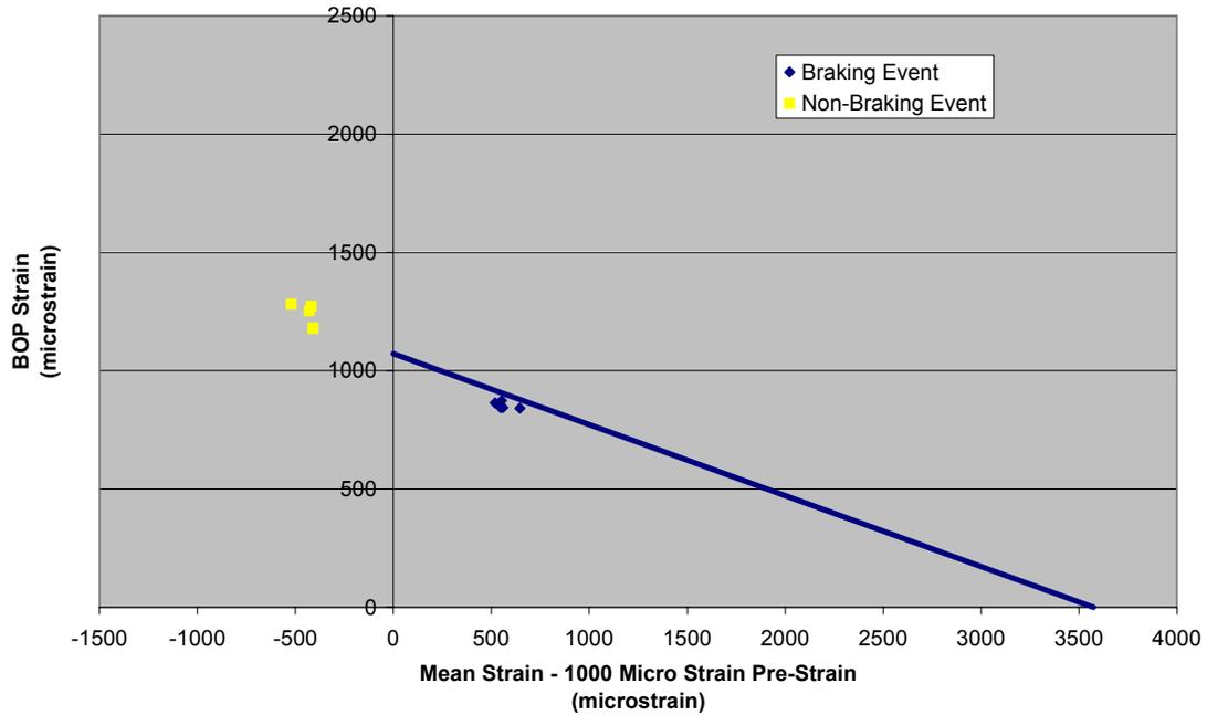
**Figure 3.70. Mean Strain versus Alternating Strain, Center WABTEC/SAB-WABCO Supplied
