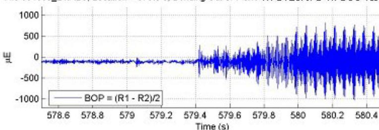
**Figure 3.78. Inception of Sustained Oscillations During Braking, Near MP AN 55 (File 061805\_24.AB3)– June 18, 2005**
