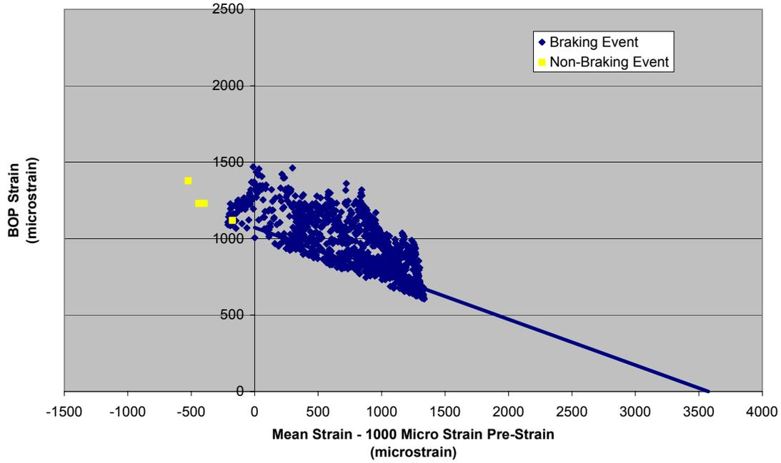
**Mean Strain vs. Alternating Strain, Center WABTEC/SAB-WABCO Disc,
