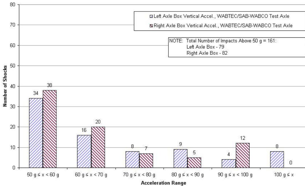
**Figure 3.6b. Distribution of Vertical Accelerations Above 50 g Measured on Instrumented Axle 1
