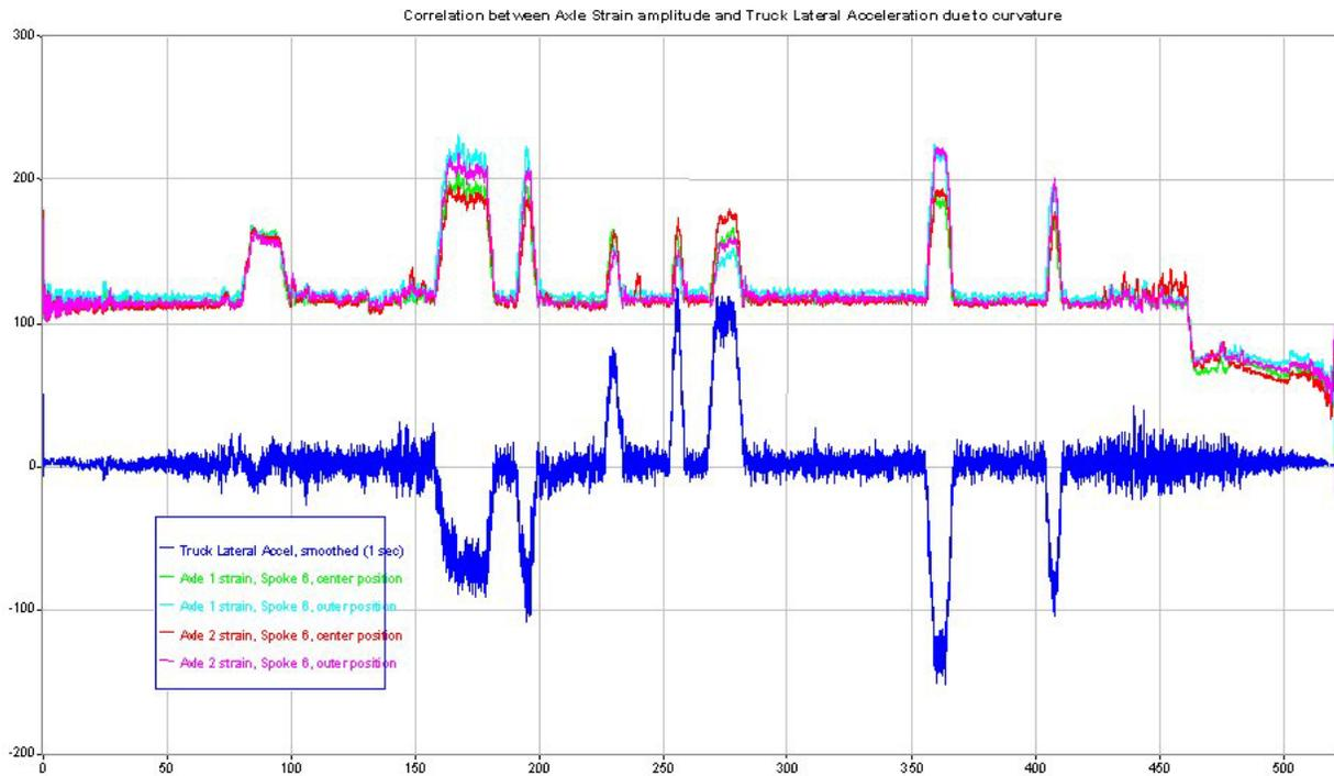
**Figure 3.52. Comparison of Truck Frame Lateral Accelerations and Axle Strains
