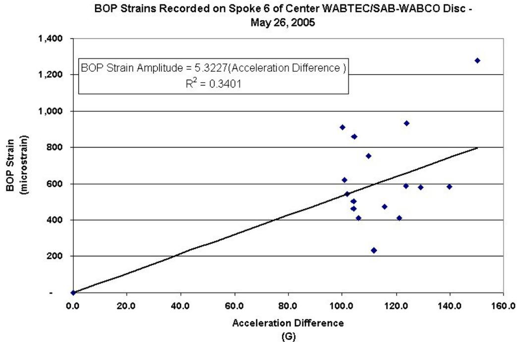
**Figure 3.33. BOP Strains as a Function of Acceleration Differences Measured on May 26, 2005**
