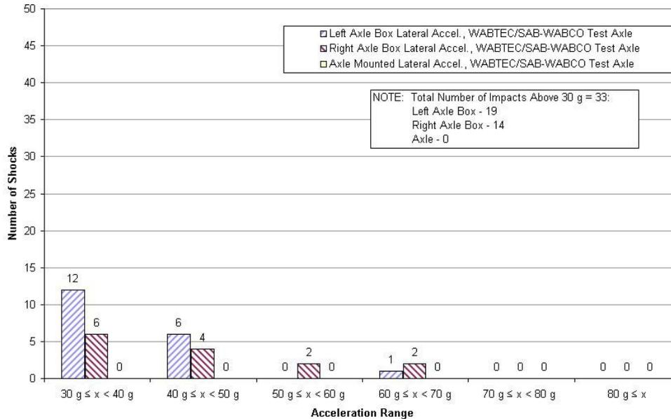
**Figure 3.26b. Distribution of Lateral Accelerations Above 30 g Measured on Instrumented Axle 1
