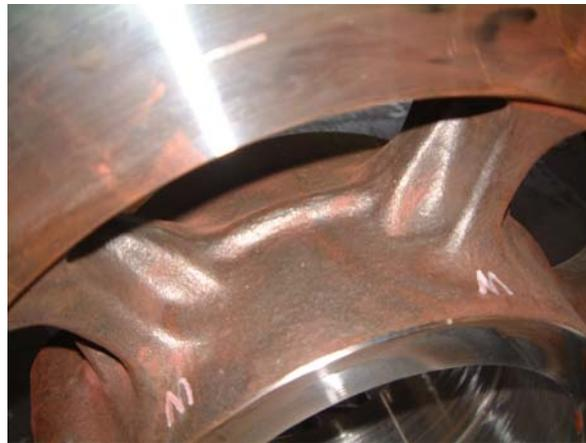
**Figure 1.5. Spokes of Brake Disc Provided by Knorr**
