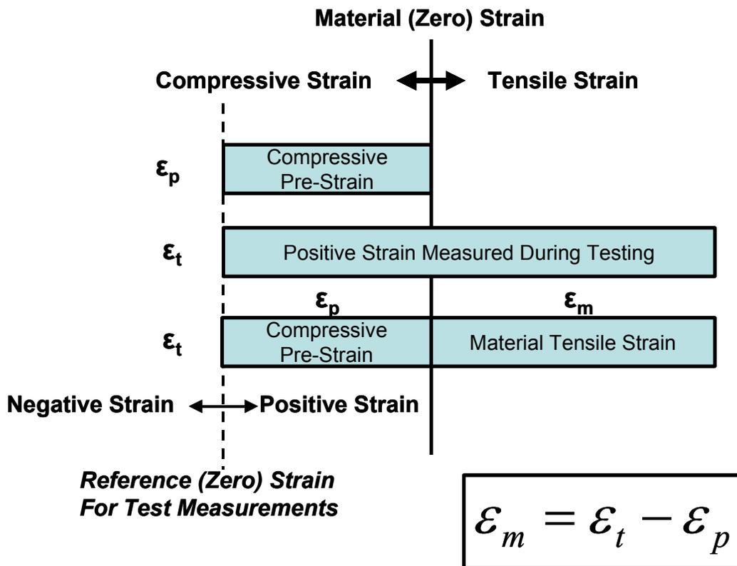
Figure 2.27. Illustration of Concept of Compressive Pre-Strain
