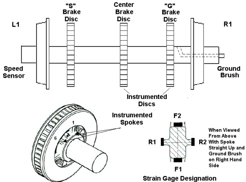
**Figure 2.3. Location of Strain Gages on WABTEC/SAB-WABCO Supplied Discs
