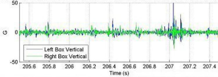
File 061705\_10.AB3, Location = 206.5 s, Truck Frame Accelerations W/ABTEC/SAB-WABCO Test Axle
