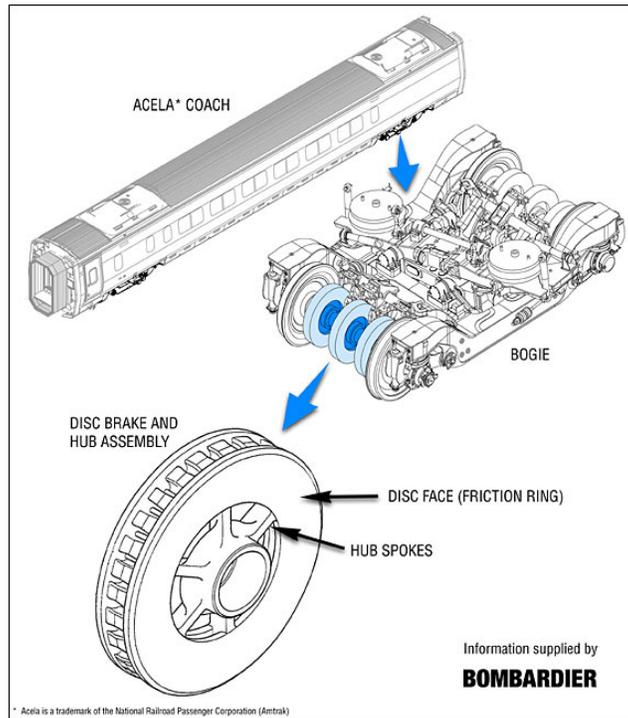
**Figure 1.1. Typical Acela Coach, Bogie and Brake Disc**
