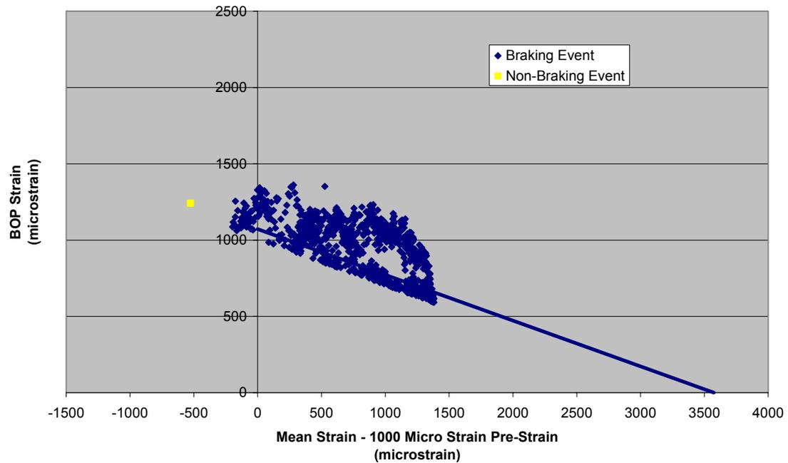
**Figure 3.72. Mean Strain versus Alternating Strain, Center WABTEC/SAB-WABCO Supplied
