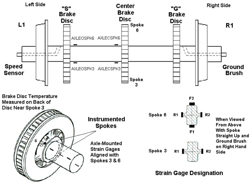
Figure 2.9a. Location of Strain Gages on WABTEC/SAB-WABCO Test Axle During Phase 3 of Acela Brake Disc Study
