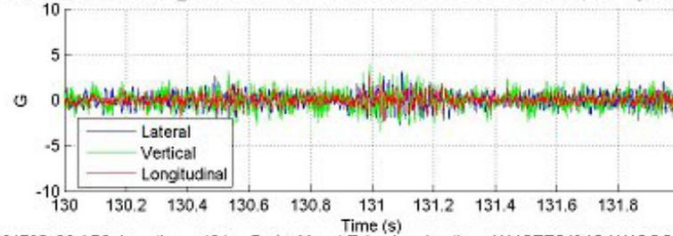
File 061705\_36.AB3, Location = 131 s, Brake Mount Tube Accelerations W/ABTEC/SAB-W/ABCO Test Axle
