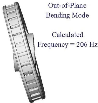
**Figure 3.1. Out-of-Plane Bending Mode Determined from FEA**
