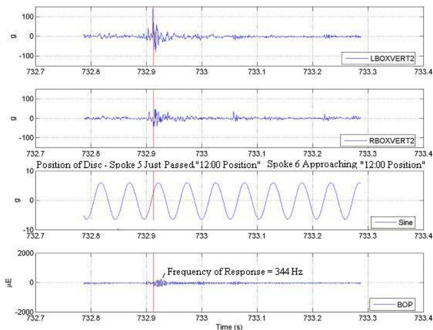
**Figure 3.49. Vertical Shock and BOP Spoke Strain Response of Knorr Brake Disc Measured Near Lane Interlocking (File 061805\_30.AB3)–June 18, 2005**
