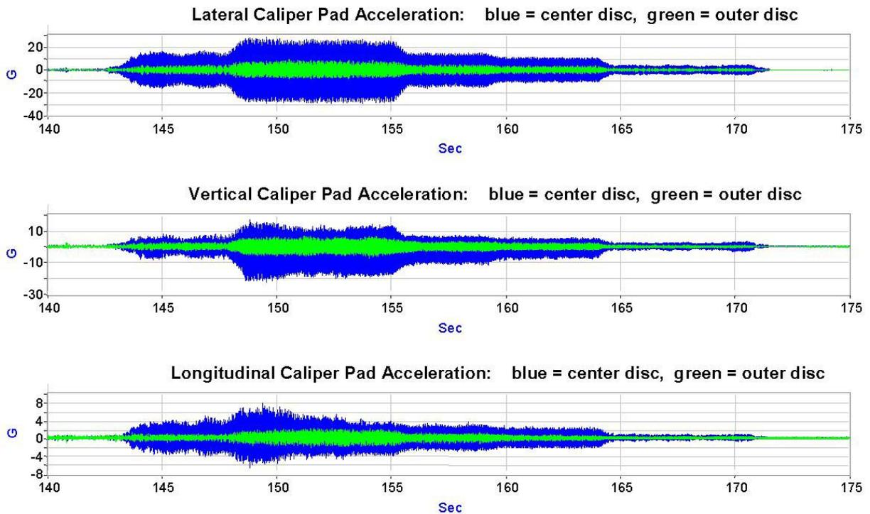
**Figure 3.17. Accelerations Measured on Center and Outer Calipers Near Pads During Brake Application with High BOP Strains (File 051705\_19.ABT)–May 17, 2005**
