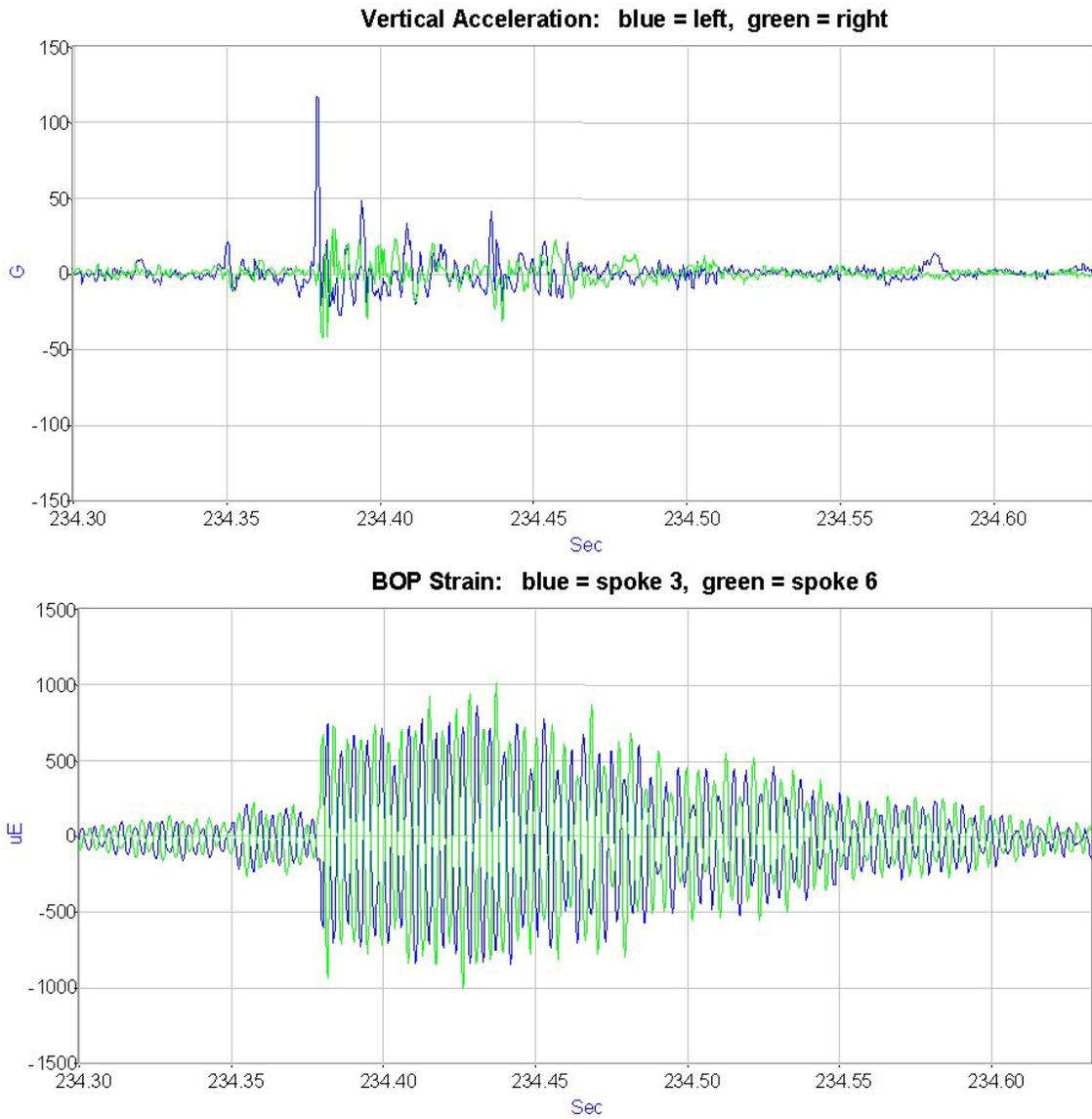
**Figure 3.30. Vertical Shock and BOP Strains Recorded on Center WABTEC/SAB-WABCO Supplied Brake Disc During Phase 2 Testing (File 052605\_18.AB2)–May 26, 2005**
