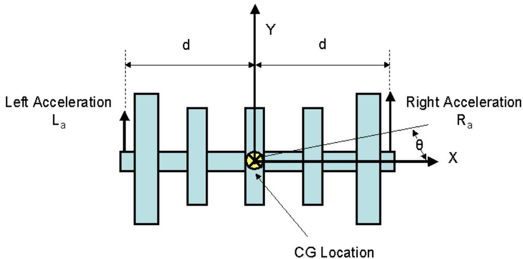
**Figure 3.35. Definition of Wheelset Acceleration Terminology**
