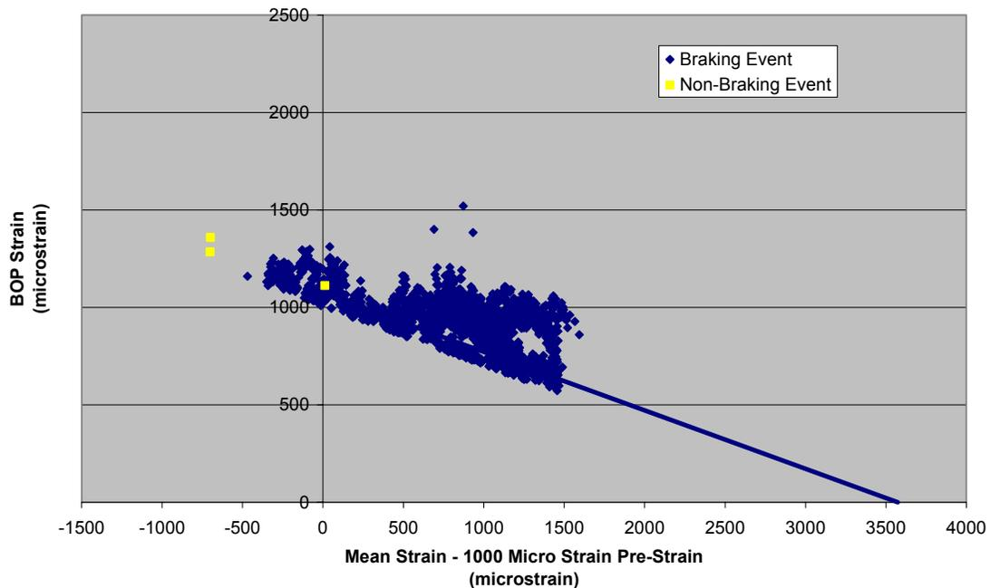
Figure 3.73. Mean Strain versus Alternating Strain, Center WABTEC/SAB-WABCO Supplied
