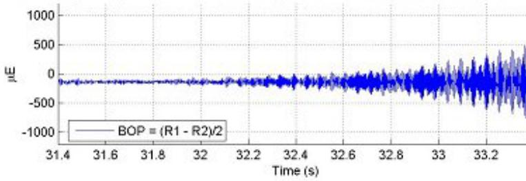
**Figure 3.77. Inception of Sustained Oscillations During Braking, Near MP AB 159 (File 061805\_07.AB3)– June 18, 2005**
