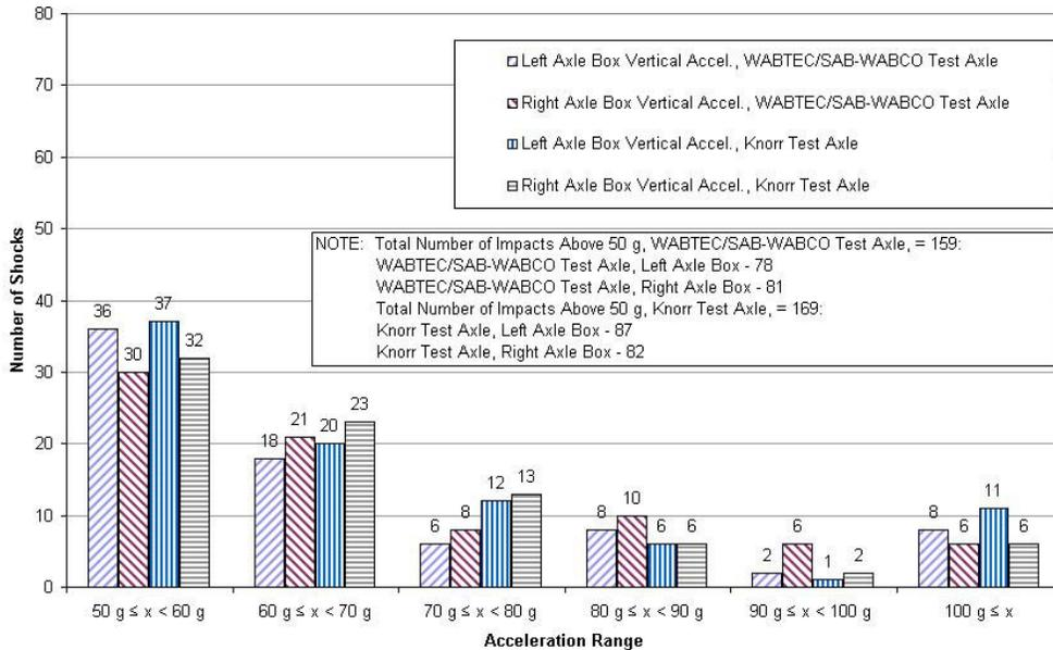
**Figure 3.46b. Distribution of Vertical Accelerations Above 50 g Measured on Instrumented Axles 1 and 2 in Lead Position—Boston, MA, to Washington, DC, on June 18, 2005**
