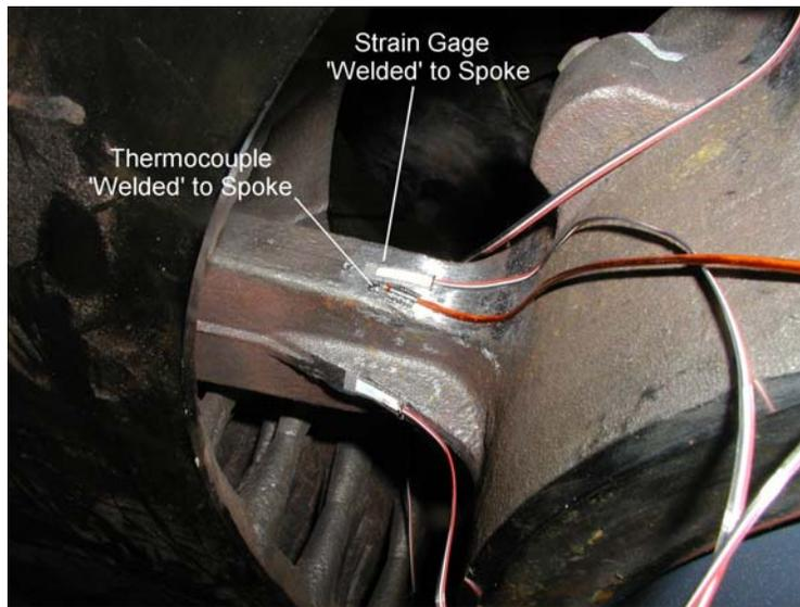
**Figure 2.19. Thermocouple Applied to Spoke on Instrumented WABTEC/SAB-WABCO Supplied Disc During Phase 1 of Acela Brake Disc Study**
