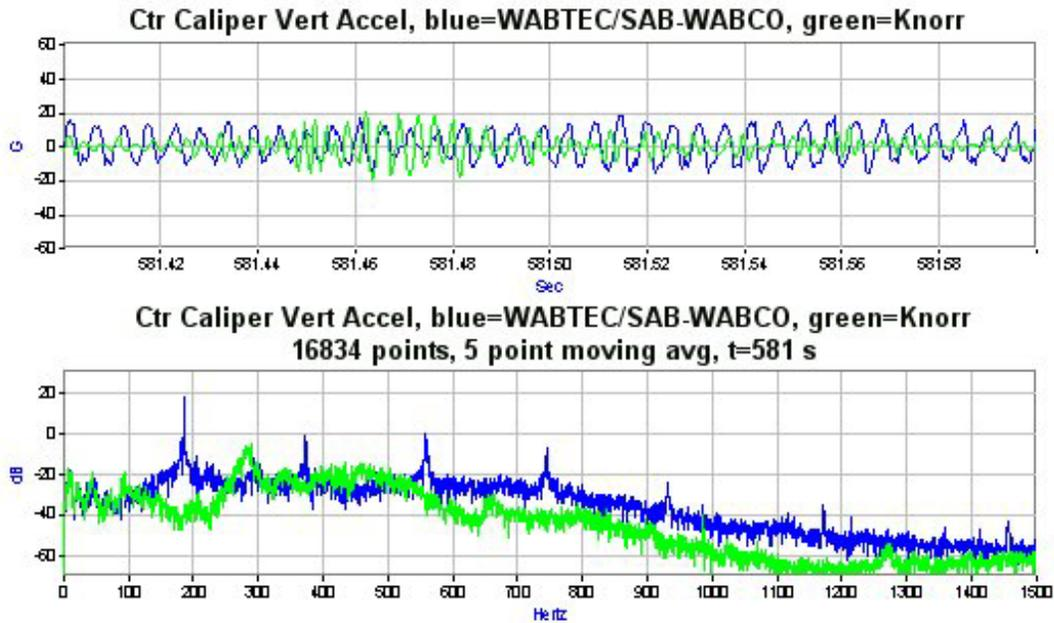
**Figure 3.59. Time History and PSD of Brake Caliper Pad Vertical Accelerations During Sustained Oscillations While Braking (File 061805\_24.AB3)–June 18, 2005**
