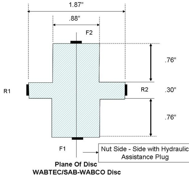
**Figure 3.45. Strain Gage Location and Cross Section Associated with Spoke of WABTEC/SAB-WABCO Supplied Brake Disc**
