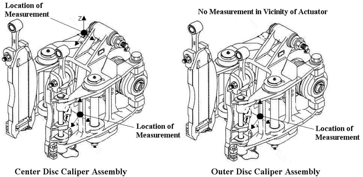
Figure 2.13. Acceleration Measurement Locations on the Caliper Assemblies
