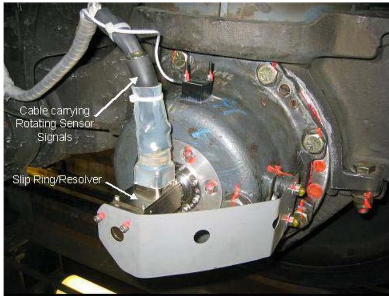
**Figure 2.22. Slip Ring/Resolver Assembly with Wheel Position Output**
