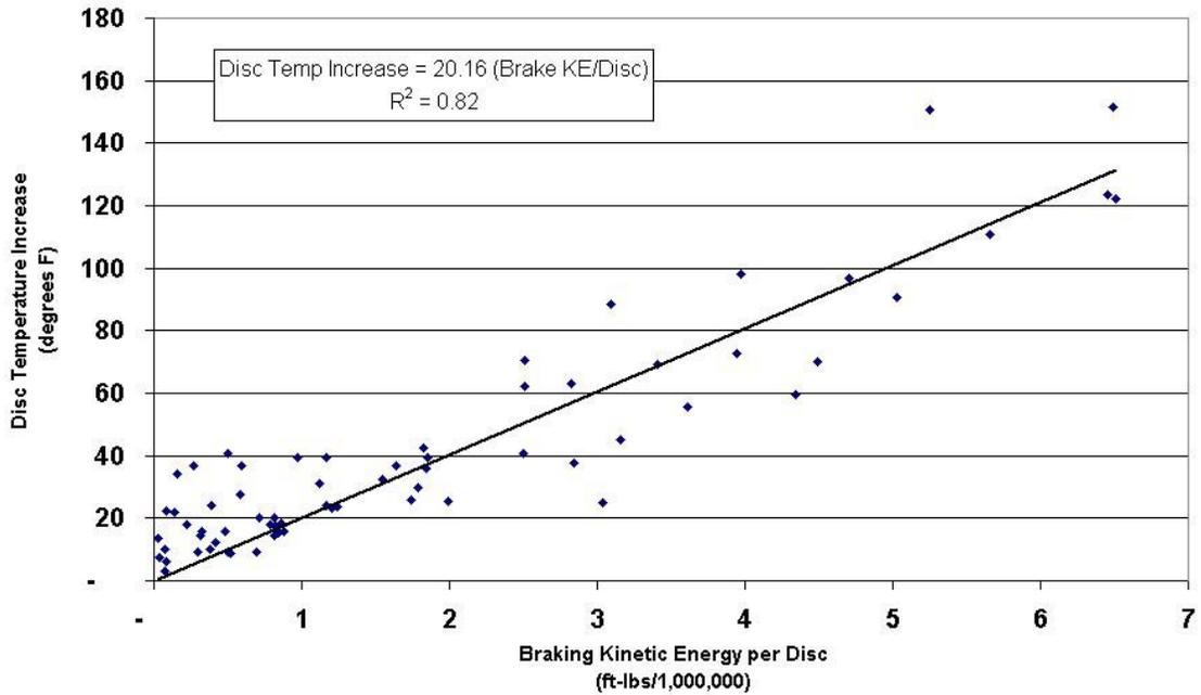
**Disc Temperature Change vs. Braking Kinetic Energy/Disc
