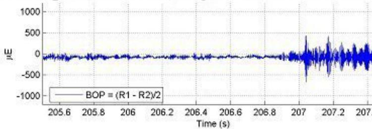
**Figure 3.75. Inception of Sustained Oscillations During Braking, Near MP AP 3.5 (File 061705\_10.AB3)– June 17, 2005**
