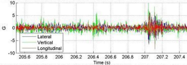
File 061705\_10.AB3, Location = 206.5 s, Brake Mount Tube Accelerations W/ABTEC/SAB-WABCO Test Axle
