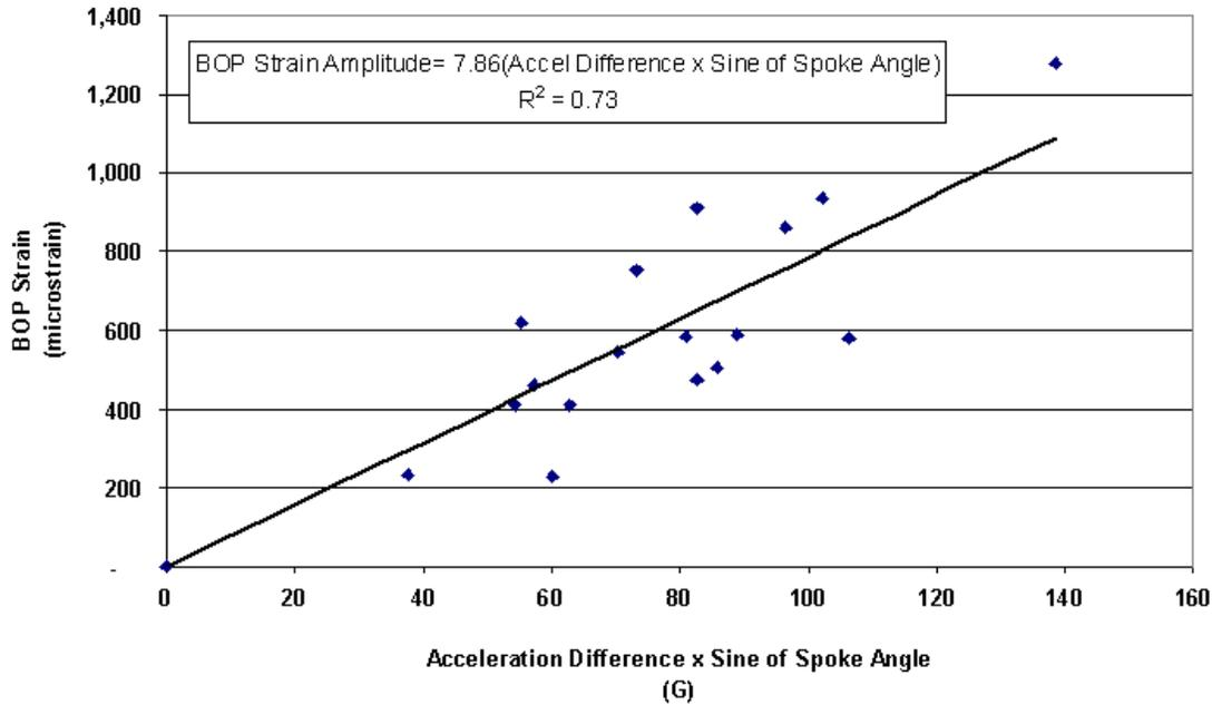
**Figure 3.34. Correlation of BOP Strain Amplitudes and Acceleration Differences
