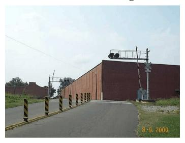
Several types of traffic channelizing devices are finding new application at highway-rail grade crossings that are equipped with flashing light signals and crossing gates. These channelizing devices, when used appropriately, can reduce the risk of a collision between a vehicle and a train by 75%! This high level of risk reduction makes traffic channelizing devices a good choice to enhance safety and greatly reduce gate violations at highway-rail grade crossings.
