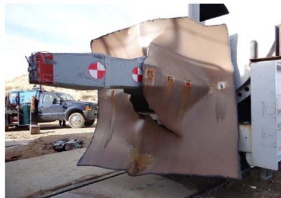
Figure 3. Post-test Photo of Interior Shell Impact Zone
