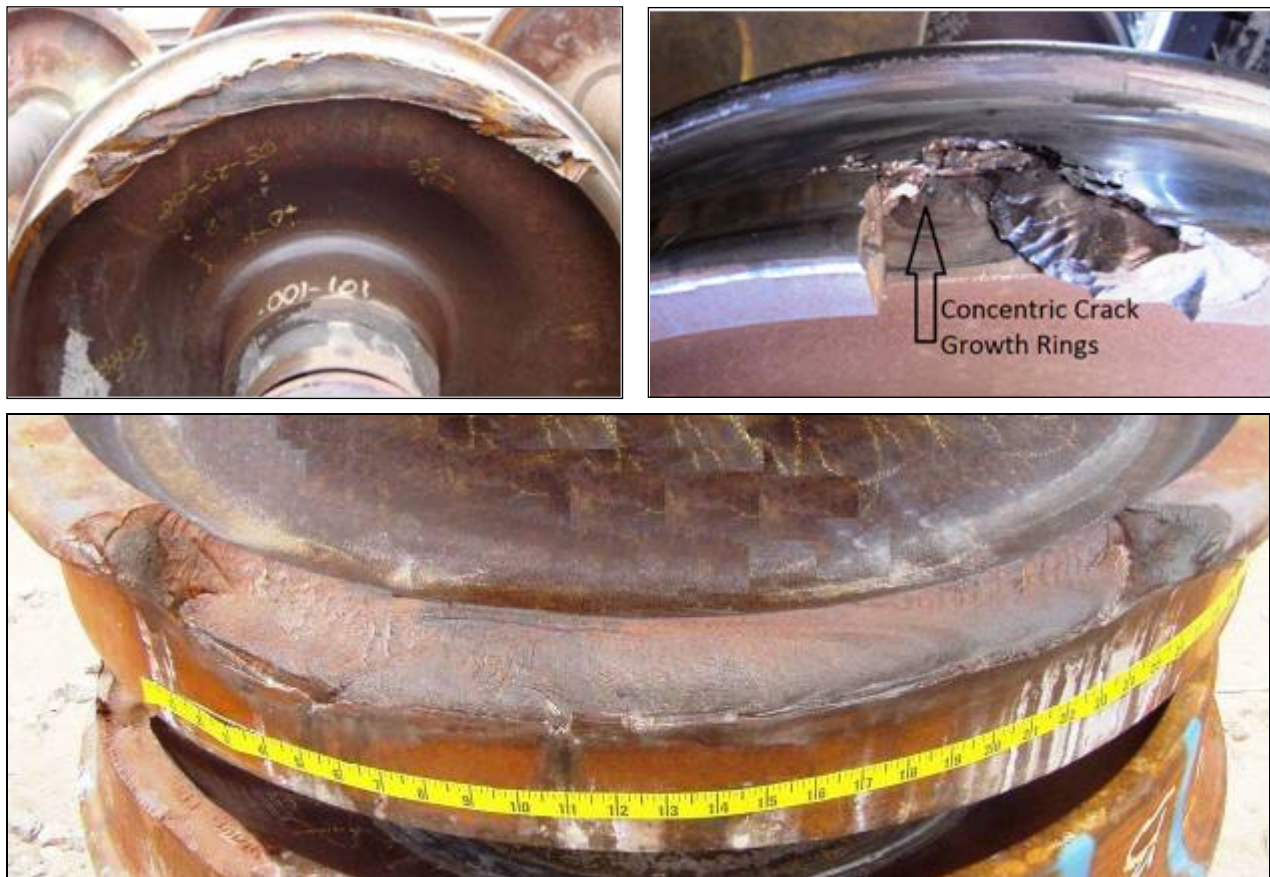
Figure 1. Typical VSR (Top Left), Shattered Rim (Top Right), and VSR Crack Resulting in a Broken Flange (Bottom)
