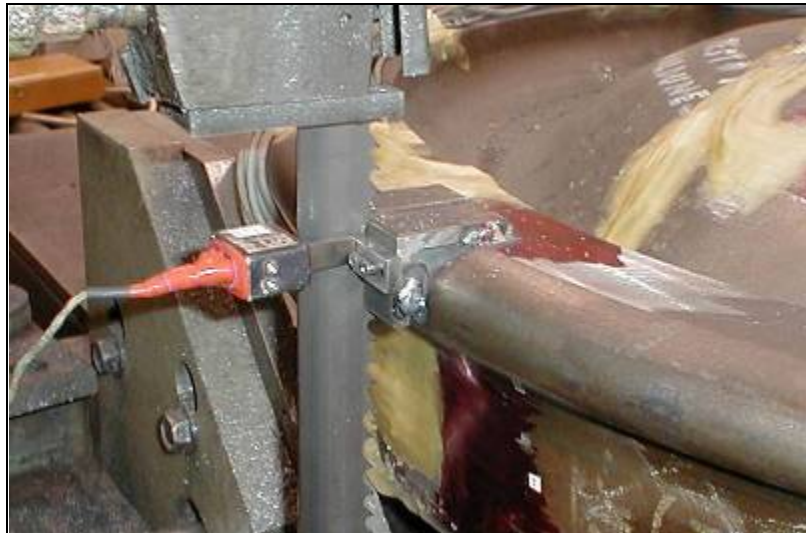
Figure 22. Photo of a Saw Cut Test
