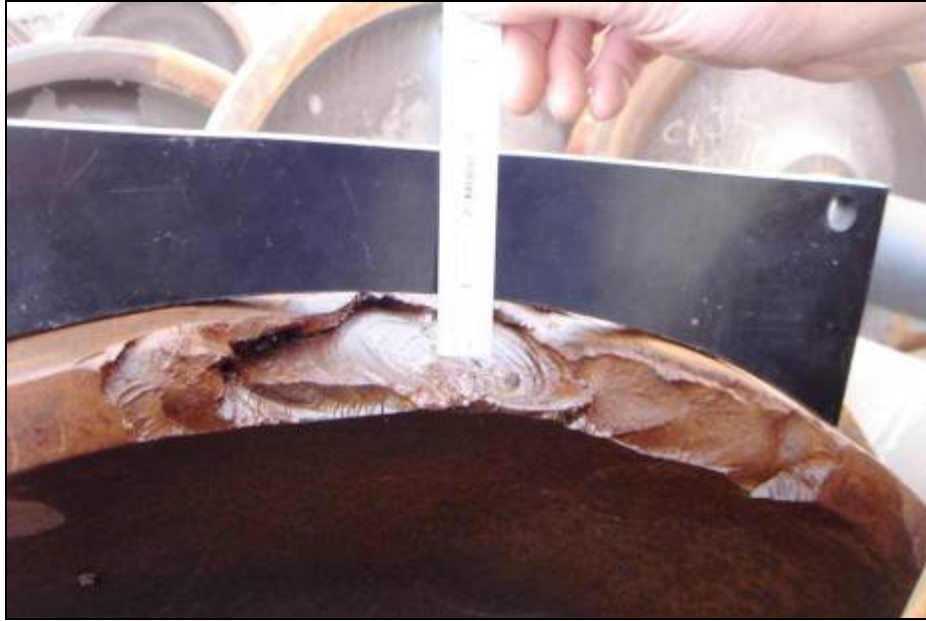
Figure 5. Shattered Rim Wheel with VSR in Combination
