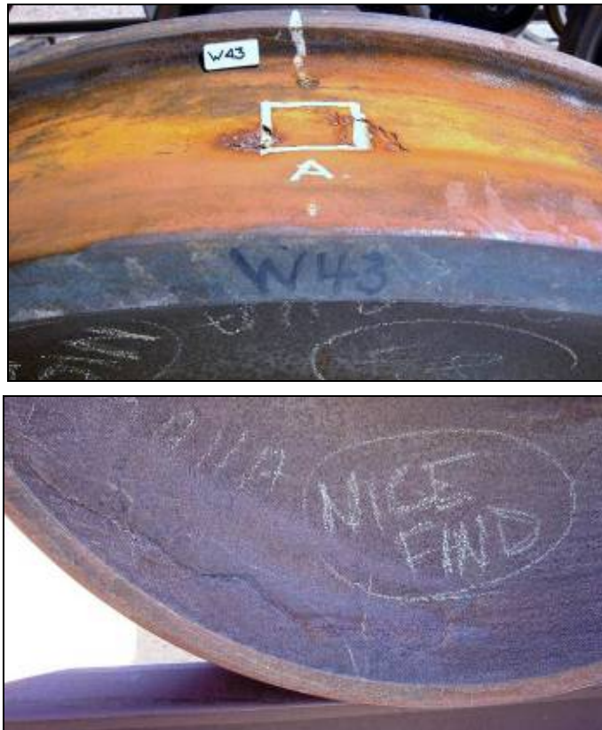
Figure 15. VSR Wheel W43 Tread (Top) and Plate (Bottom) Prior to Opening Crack
