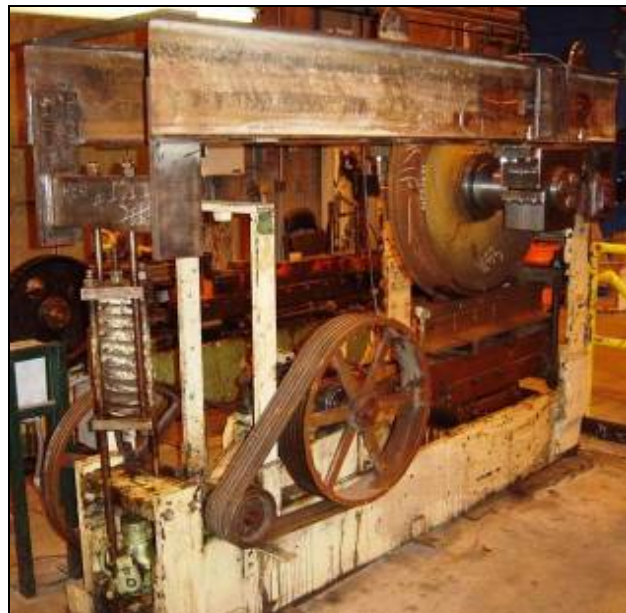
Figure 27. TTCI's Rolling Load Machine
