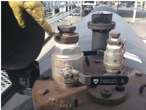
3" and 2" McKenzie UNNR Valves with Reducer Fittings and Plugs
