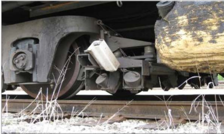
Figure 6. Production joint-bar inspection system fitted to a rail car
