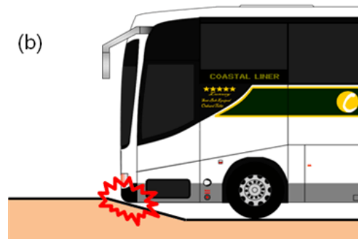
Figure 1. (a) A truck could hang up when its wheels straddle a road hump (b) The front overhang of a bus could hang up on a sudden steep incline
