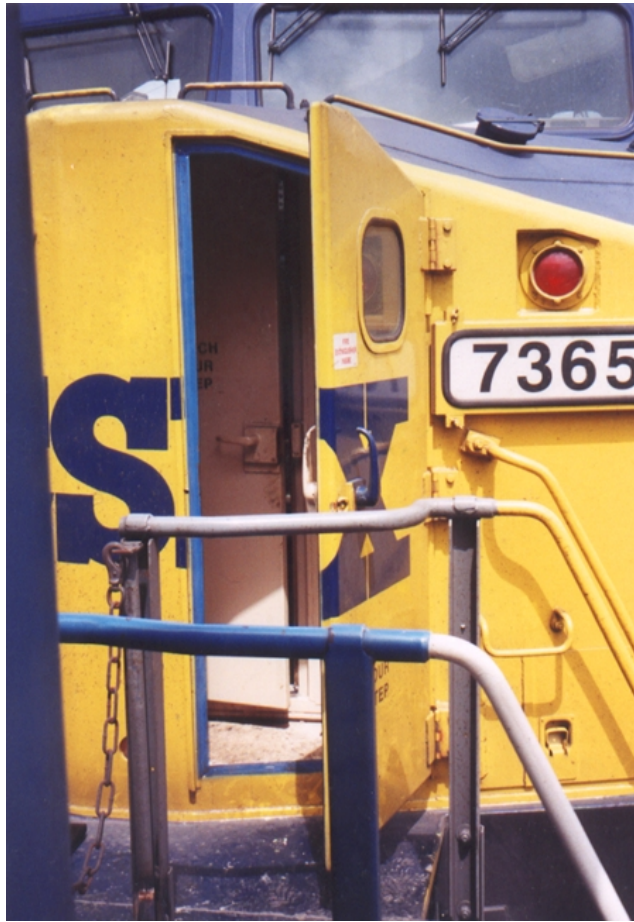
Figure 15. SD 70 MAC nose door to platform, stairs on either side
