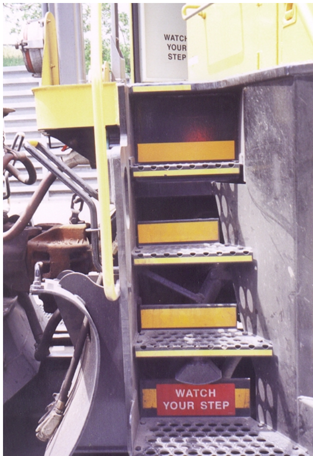
Figure 83. SD-70 MAC retroreflective step markings
