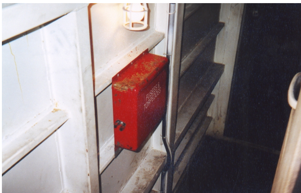
Figure 110. P32-AC emergency tools located on wall behind cab near door to engine room
