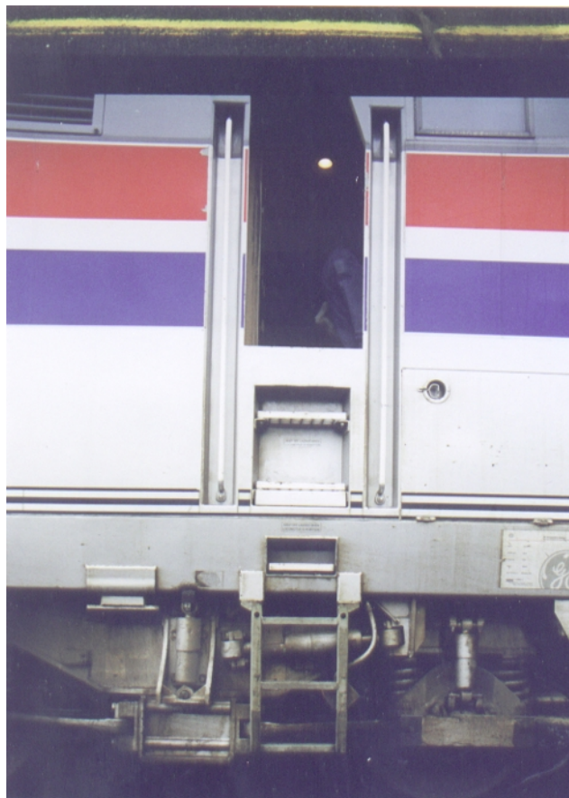
Figure 87. View of side door ladder-type steps
