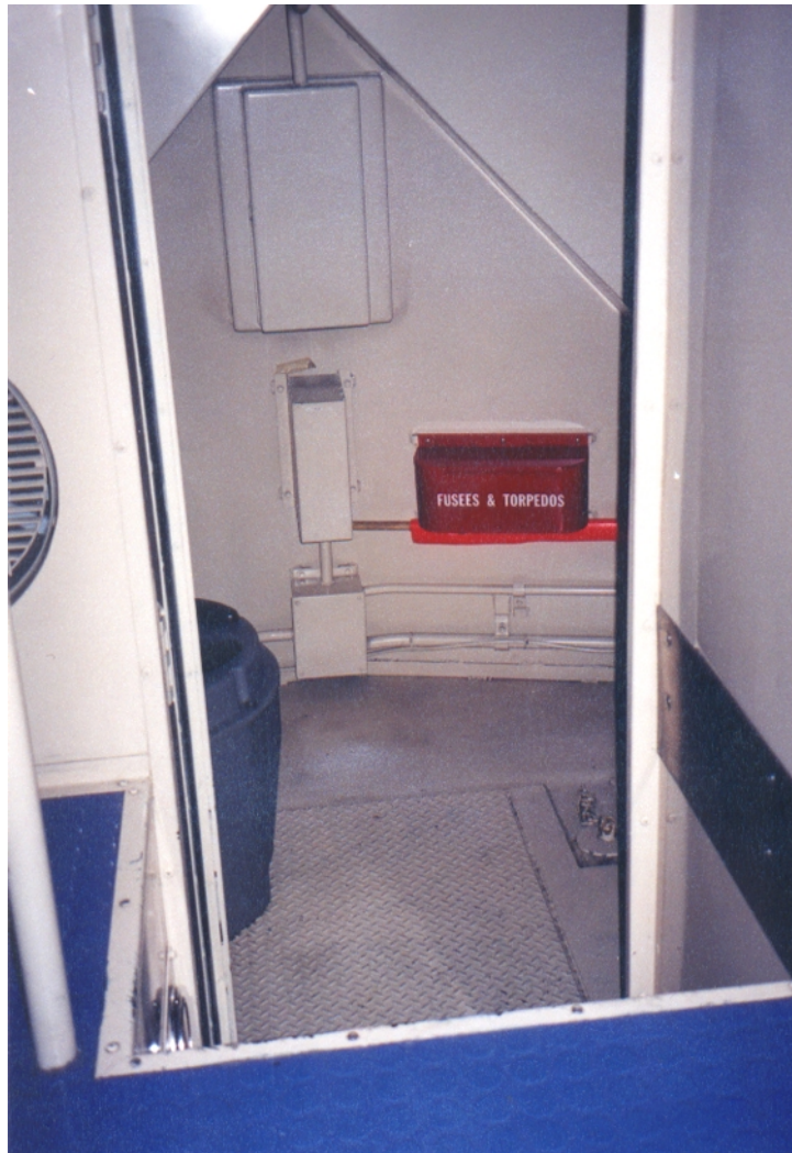
Figure 107. F40-PH3 fusees and torpedos located in nose compartment
