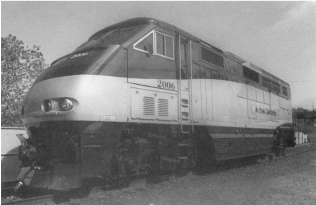
Figure 75. Exterior view of F59 passenger locomotive
