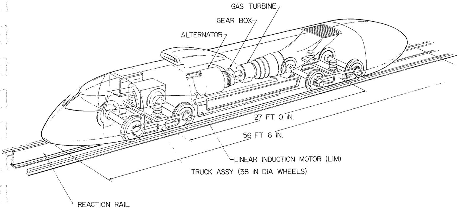
Fig. 7. — Test vehicle for linear induction motor testing.
