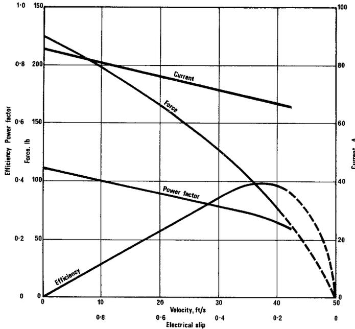
Fig. 2. Test results obtained with a small two-stator linear motor running on a vertical aluminium reaction plate
