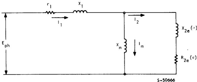
Figure 7. Equivalent Circuit of a Linear Induction Motor
