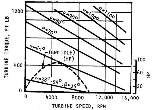
Figure 15. T64 Turbine Torque - Speed Characteristics
