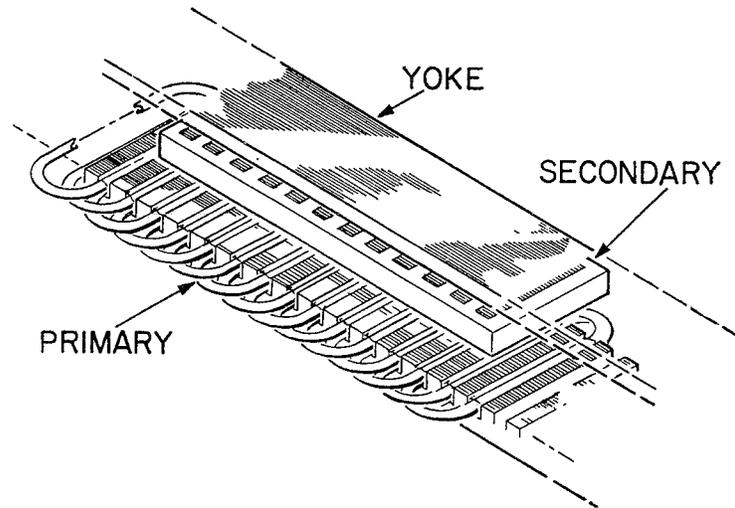
Fig. 1 b. — Single sided short secondary linear induction motor with stationary secondary yoke.
