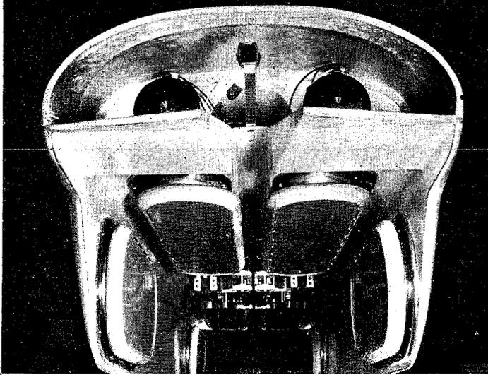
Underside of a model Hovertrain proposed by Hovercraft Development Limited. The linear motor and three-phase current collectors are in the centre of the vehicle
