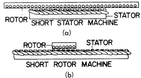
Fig. 3. Basic types of linear motor.
