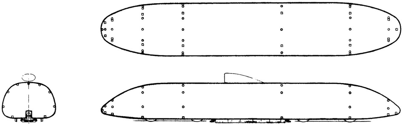
FIG. 12 LOCATIONS OF AERODYNAMIC SENSORS
