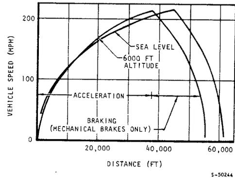
Figure 18. Speed Distance Curves
