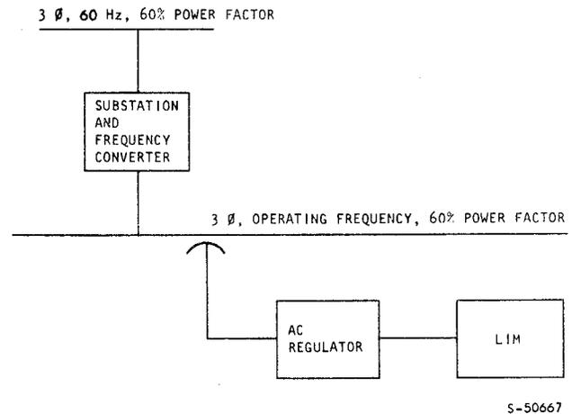
Figure 8. Constant Frequency Three-Phase Wayside Power
