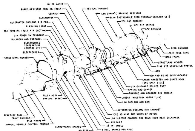
Figure 2. Component Arrangement
