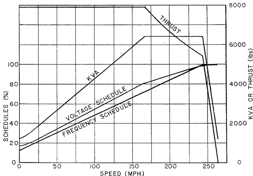
Fig. 3. — Linear induction motor performance: variable frequency and voltage.
