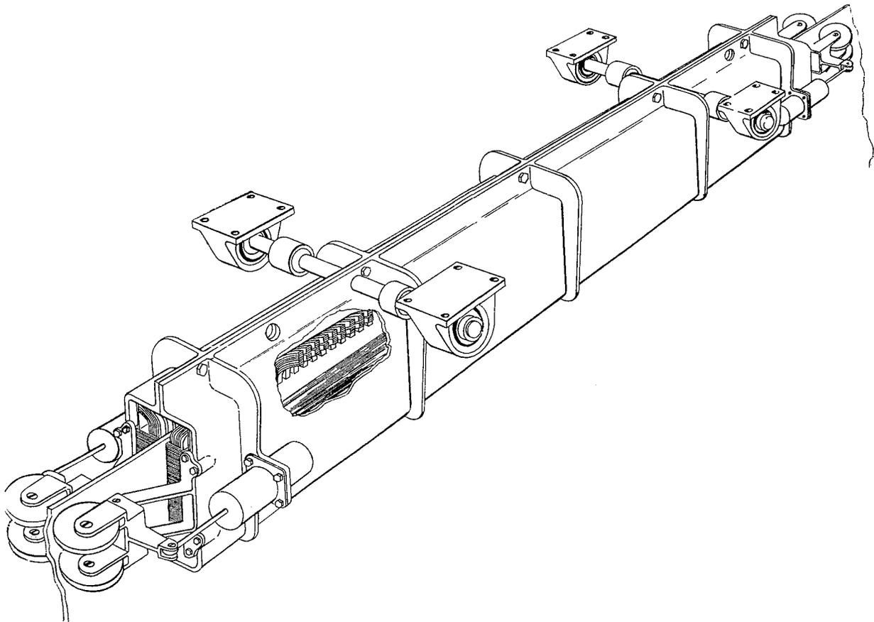
Fig. 6. — 2500 HP prototype linear induction motor.
