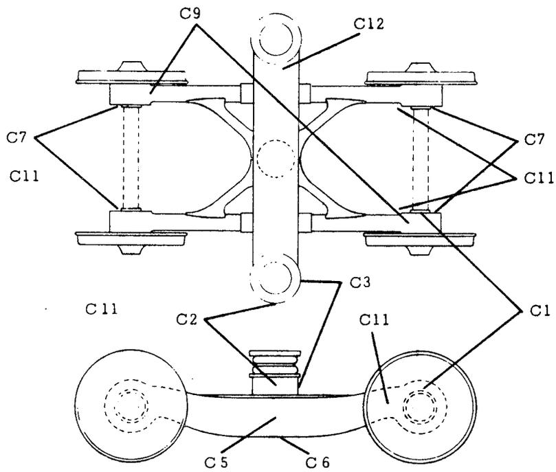
FIG. 13 LOCATIONS OF TRUCK SENSORS
