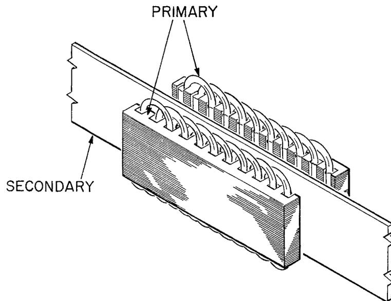
Fig. 1 d. — Double sided short primary linear induction motor.
