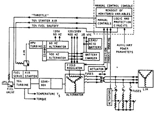
Figure 14. LIM Test Vehicle Control System
