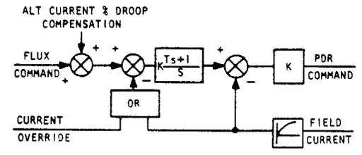
Figure 16. Alternator Field Control
