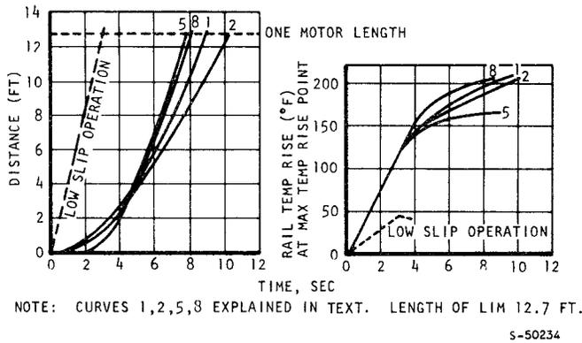
Figure 20. Reaction Rail Temperature Rise
