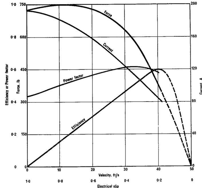
Fig. 4. Test performance of the motor used for Fig. 2 when running on a steel plate; the efficiency and power factor are significantly reduced
