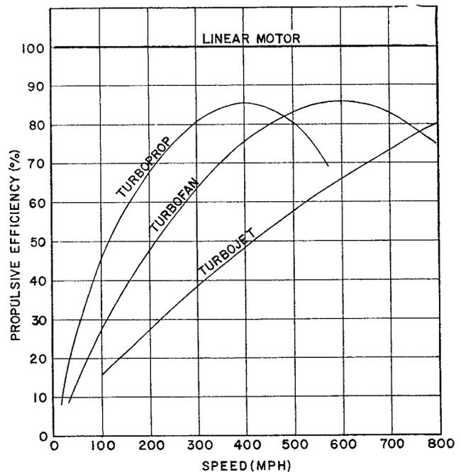
Fig. 4. — Propulsive efficiency of various propulsion systems.
