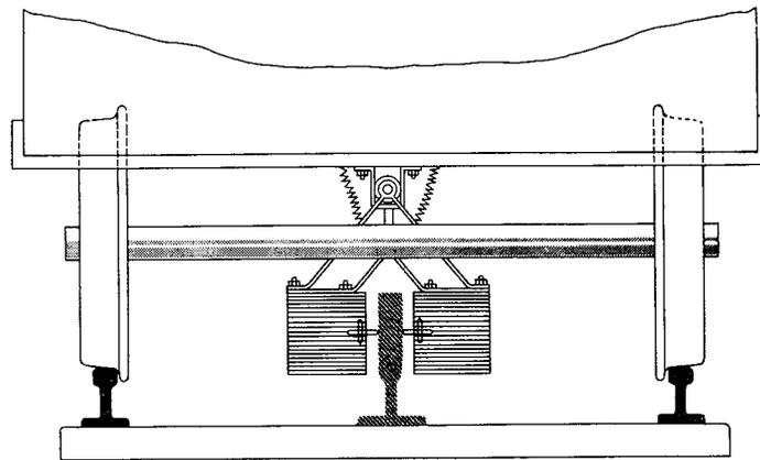
Fig. 3. Linear motor arrangement proposed by Zehden in 1905
