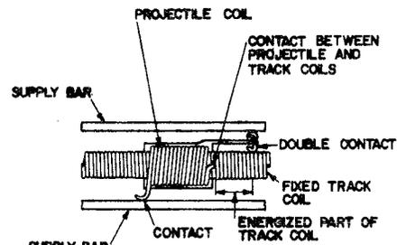
Fig. 16. The hypervelocity induction system.
