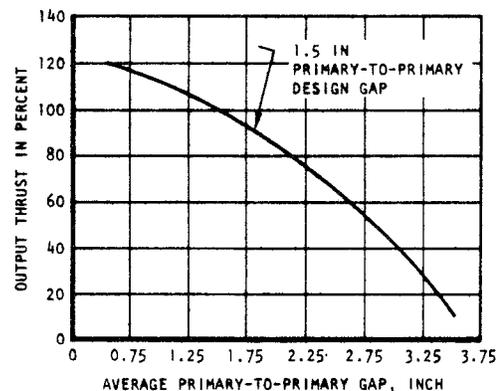
Figure 6. Output Thrust Vs Airgap
