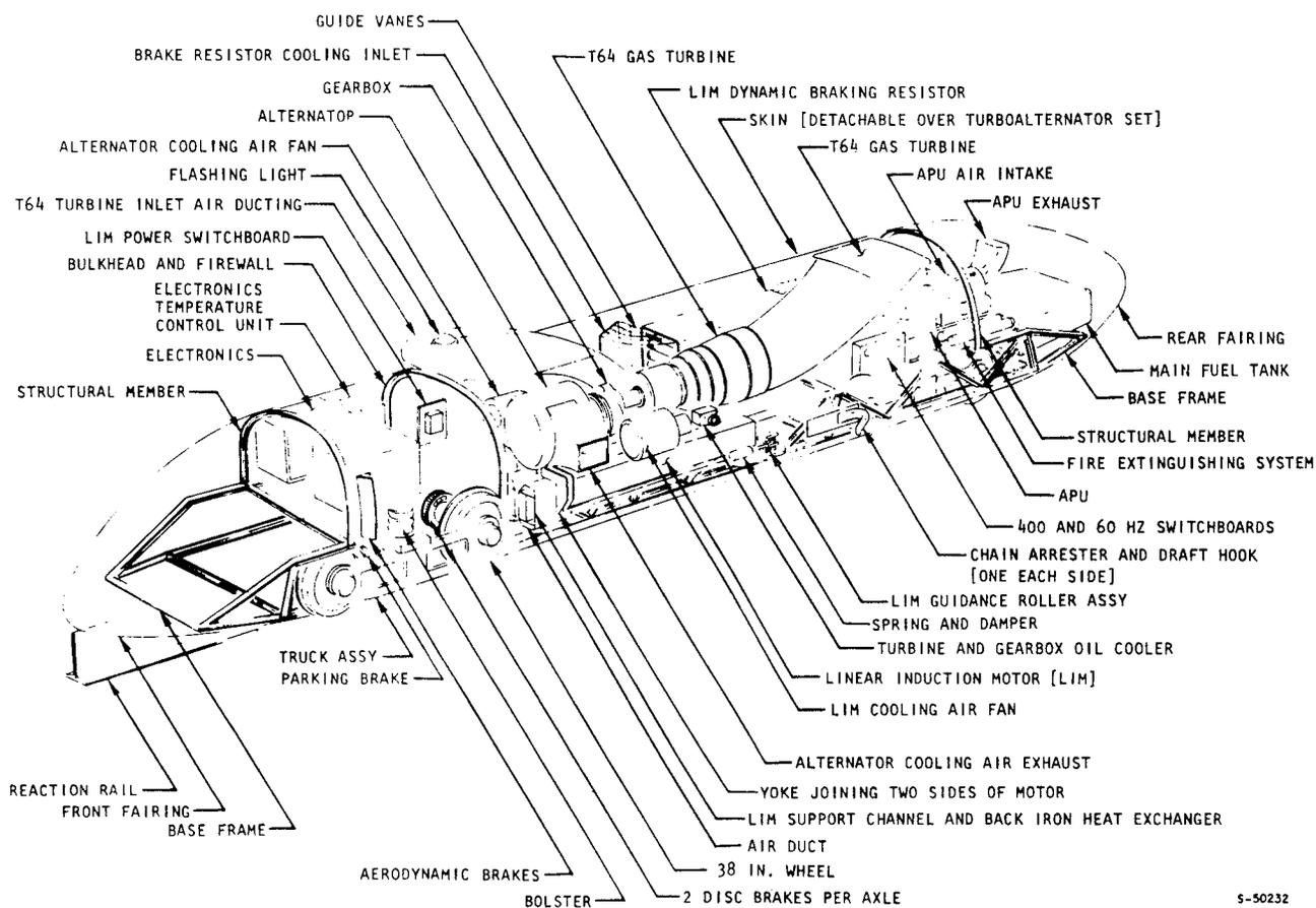
FIG. 2 GENERAL ARRANGEMENT OF HARDWARE IN LIM TEST VEHICLE
