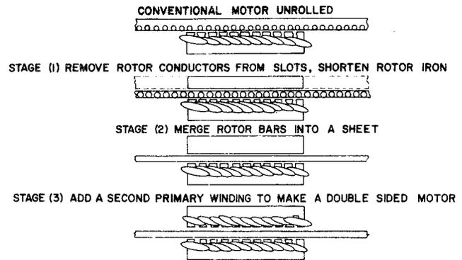
Fig. 4. Development of the "sheet-rotor" motor.
