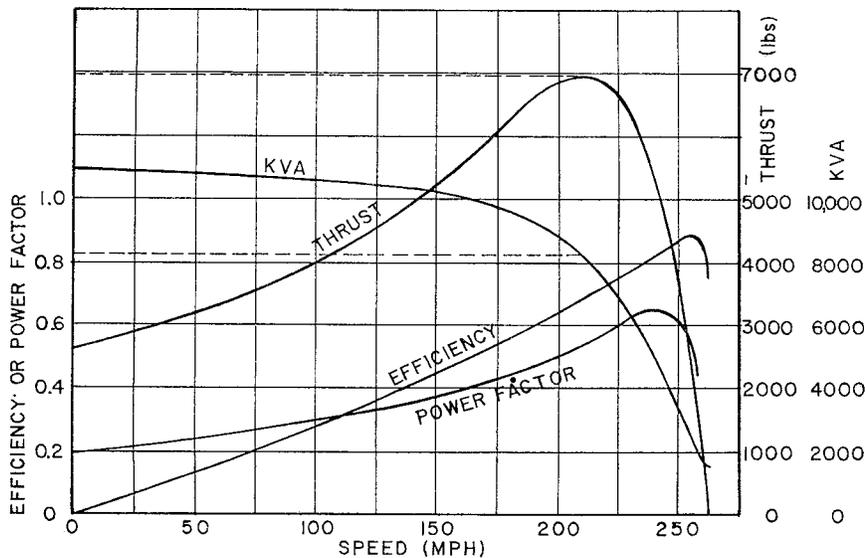
Fig. 2. — Linear induction motor performance: constant frequency and voltage.
