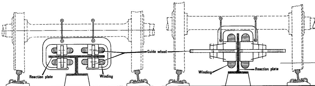
Fig. 1. Horizontal and vertical reaction plates within the space beneath a normal railway axle
