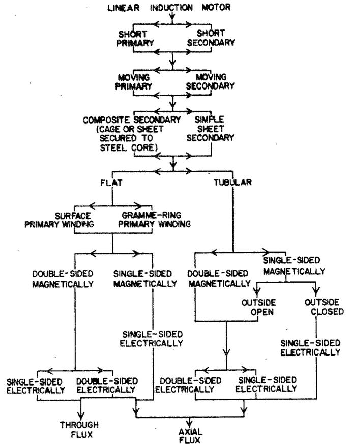
Fig. 12. Topological classification of linear induction motors.
