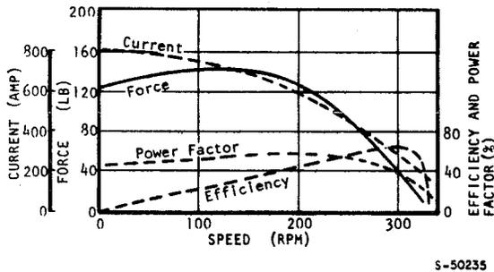
Figure 12. One Pole-Pair Dynamic Model Test Data
