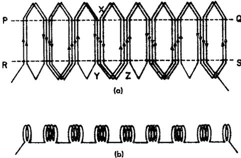
Fig. 10. End-turn advantages of tubular motor windings.
