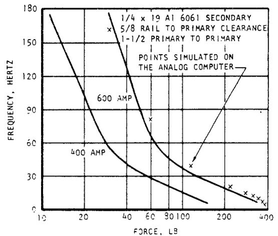
Figure 21. Locked Reaction Rail Test Data
