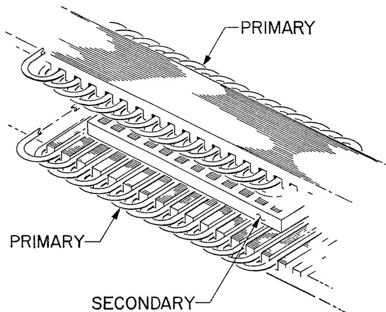
Fig. 1 c. — Double sided short secondary linear induction motor.
