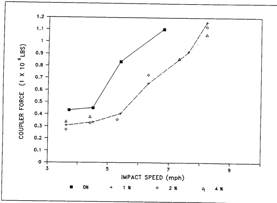
Figure 29. Coupler Force vs Impact Speed, 0% Outage, B-end Impacted
