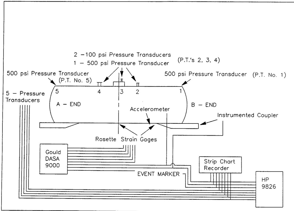
Figure 12. Instrumentation Layout
