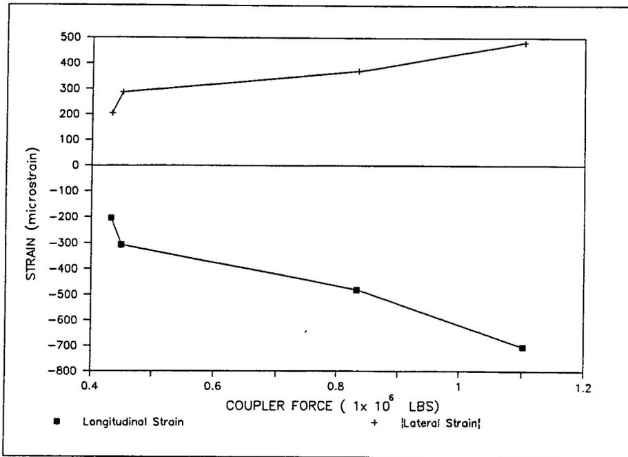
Figure 31. Longitudinal and Lateral Strains vs Coupler Force
