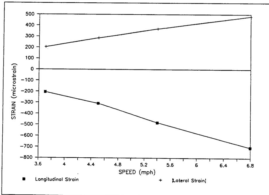
Figure 32. Longitudinal and Lateral Strains vs Impact Speed
