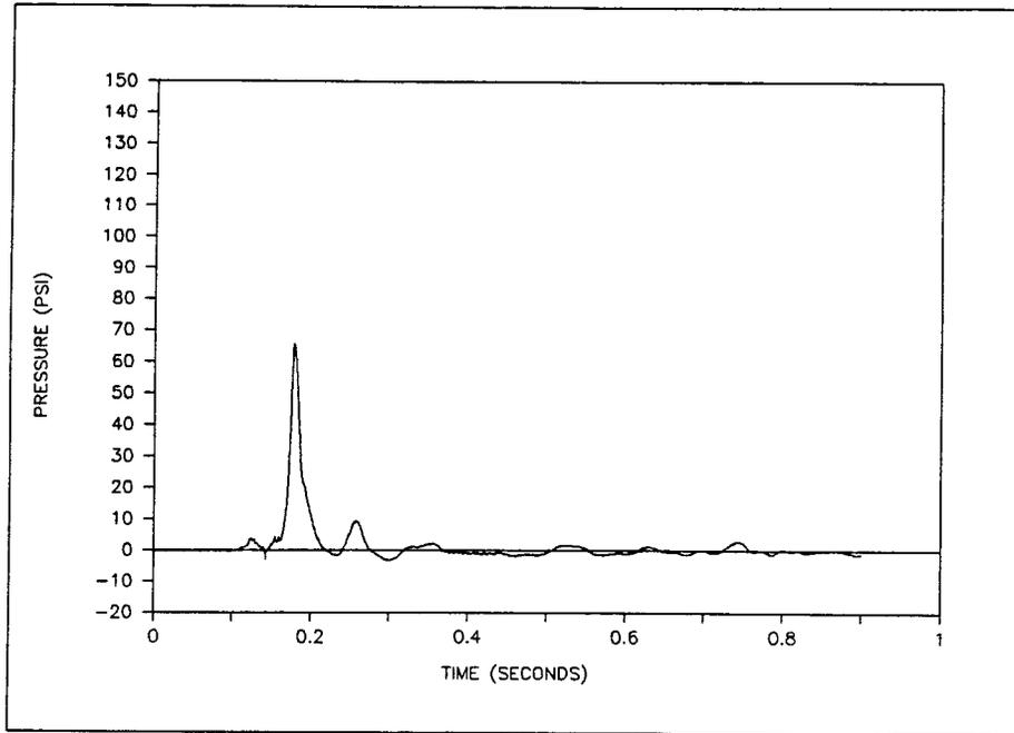
Figure 25. Surge Pressure in 2 1/2" Nozzle without SPR, 0% Outage, B-end Impacted at 5 mph
