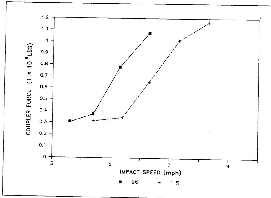
Figure 30. Coupler Force vs Impact Speed, 0% Outage, A-end Impacted
