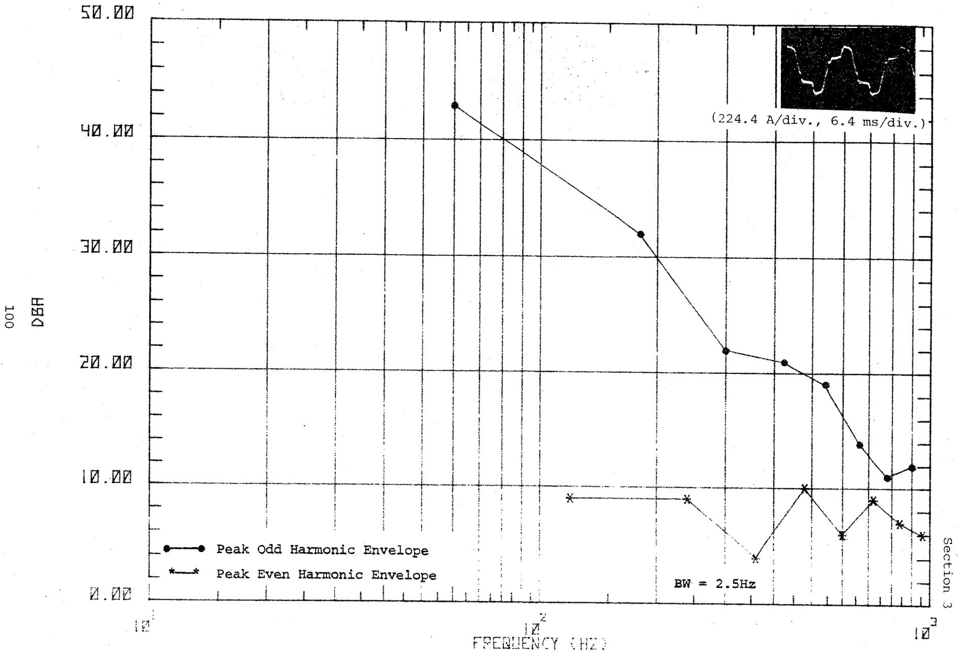
Figure 51b. Waveform and spectrum of ground side primary waveshape #2.
