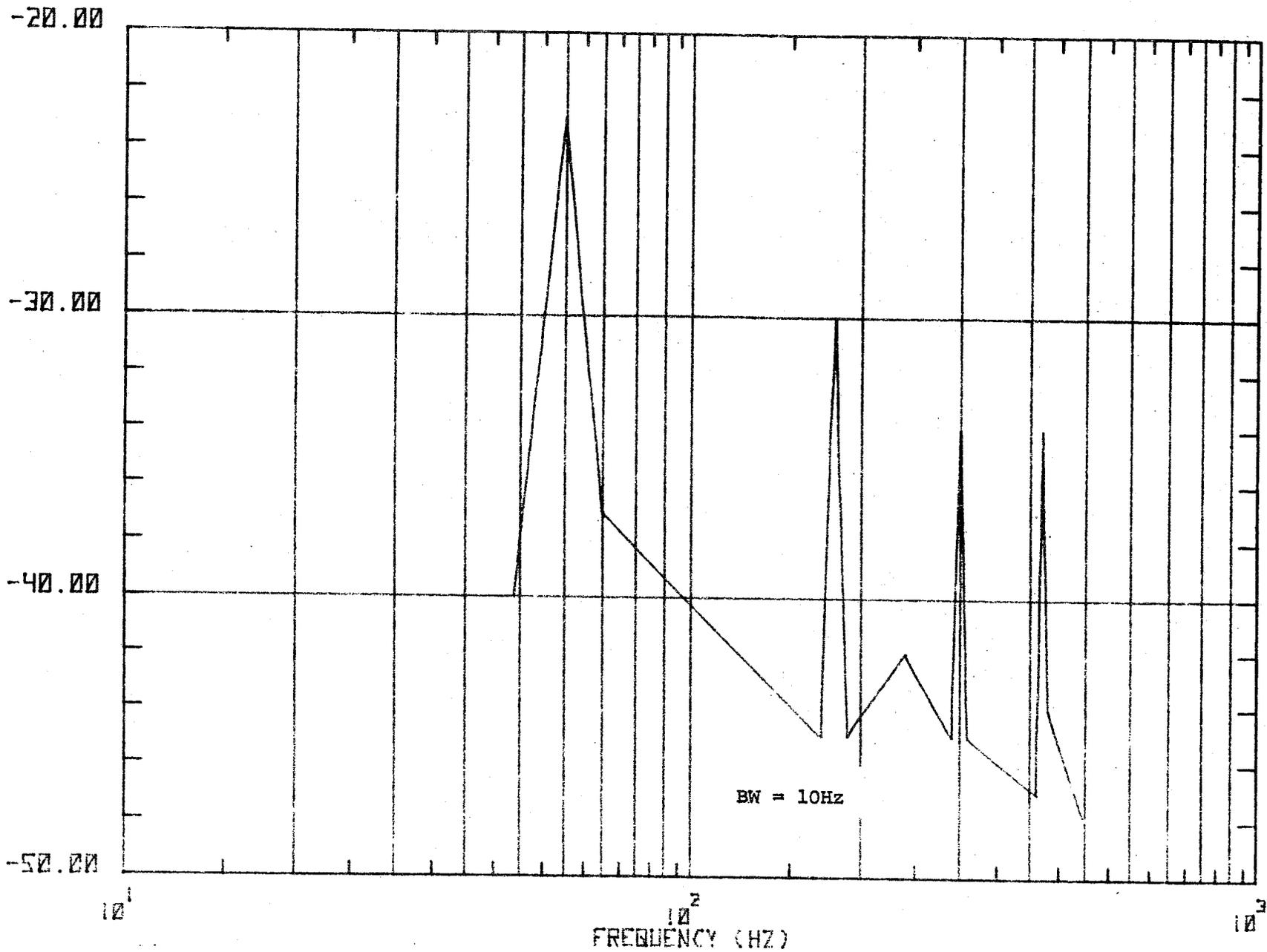
Figure 17. Spectrum of voltage across 74-volt bus with the pantograph down.
