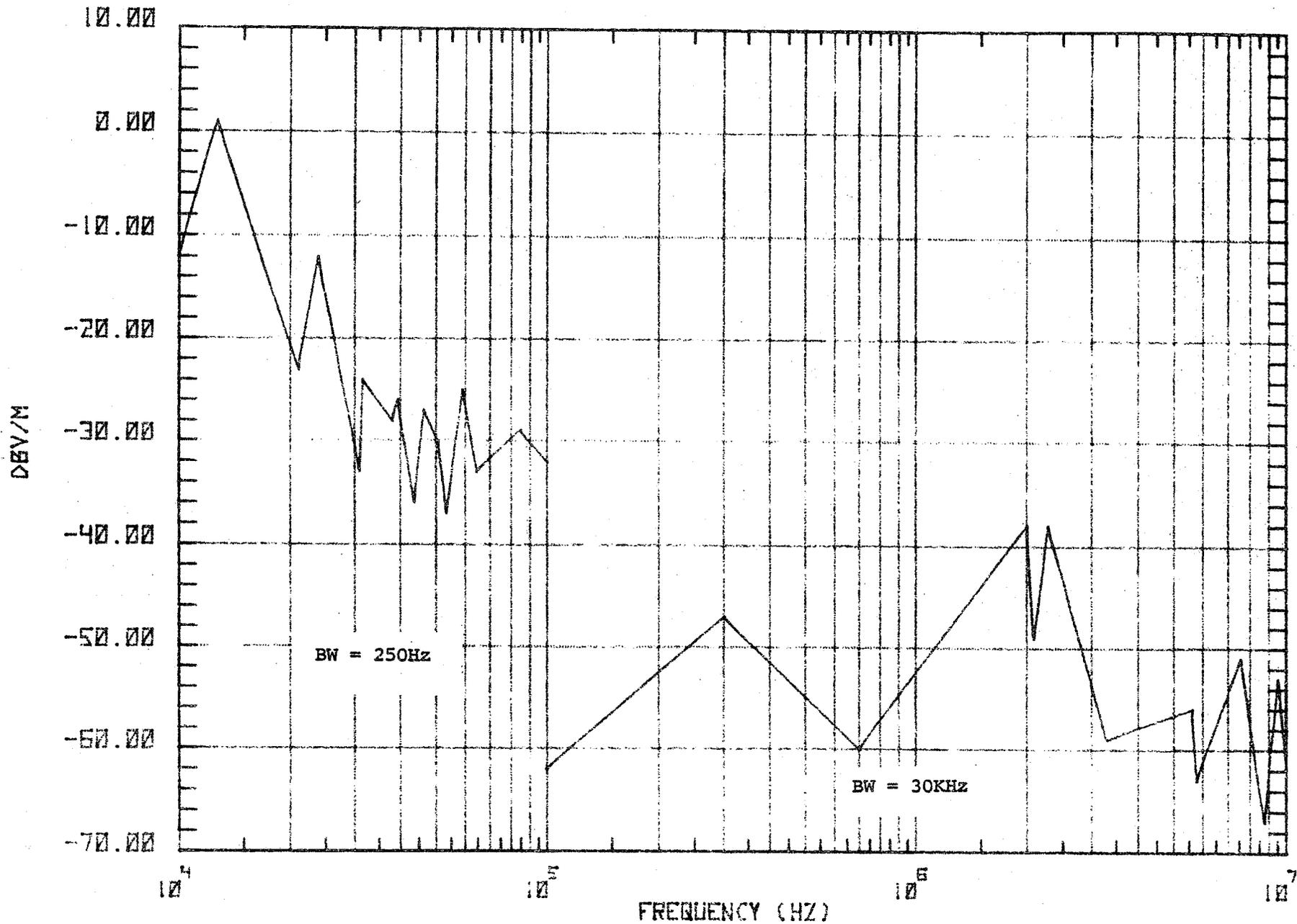
Figure 35. Spectrum of electric field strength sampled while locomotive was idling (locomotive on RTT) (Continued).
