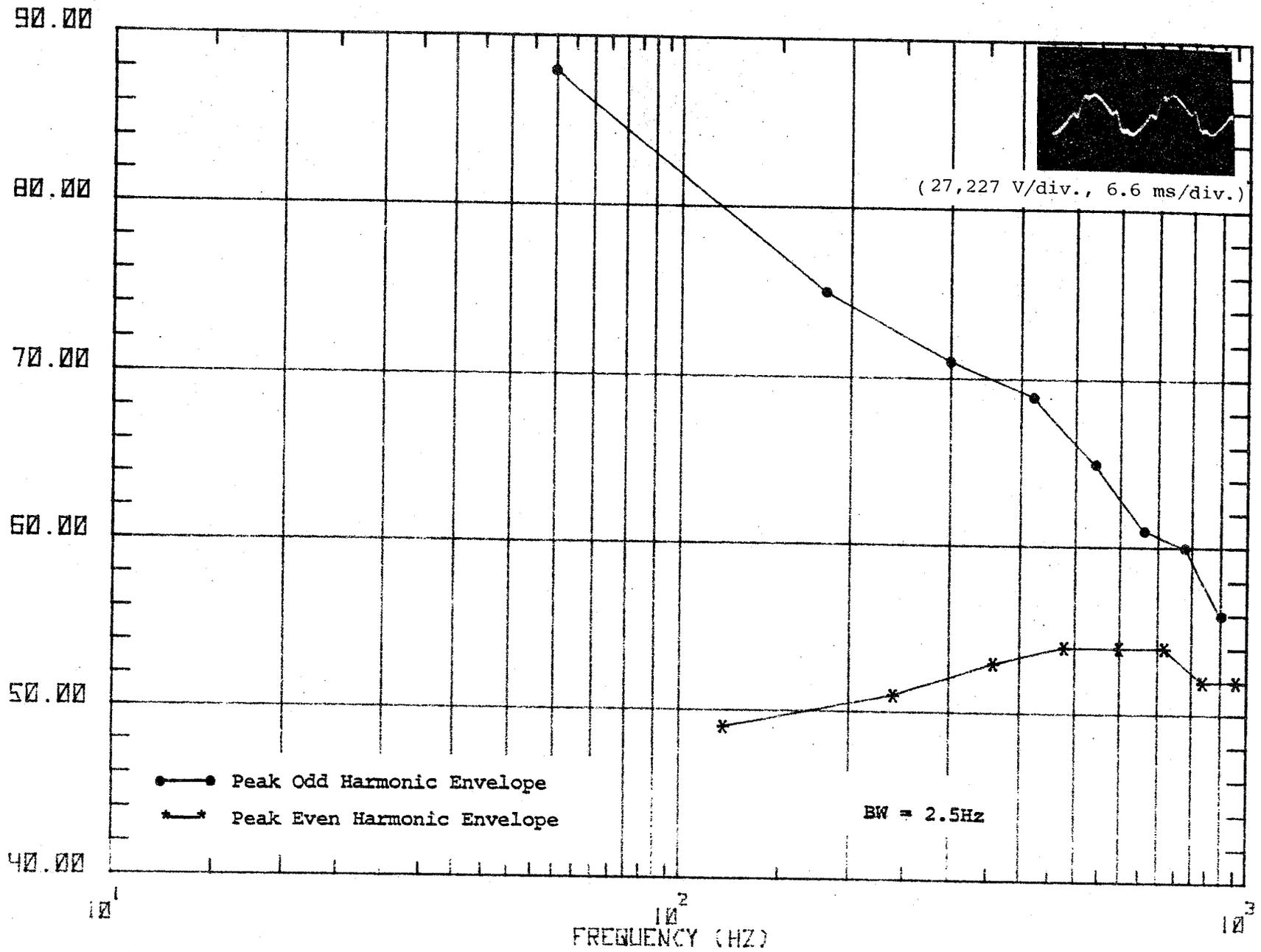
Figure 54f. Waveform and spectrum of catenary voltage sampled during 10-mph increment run, 60 to 70 mph.
