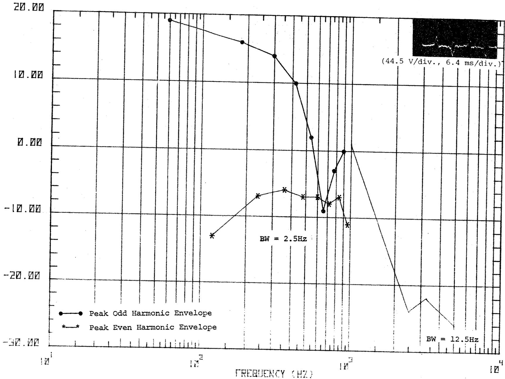
Figure 63g. Waveform and spectrum of cab signal voltage corresponding to ground side primary waveshape #7.
