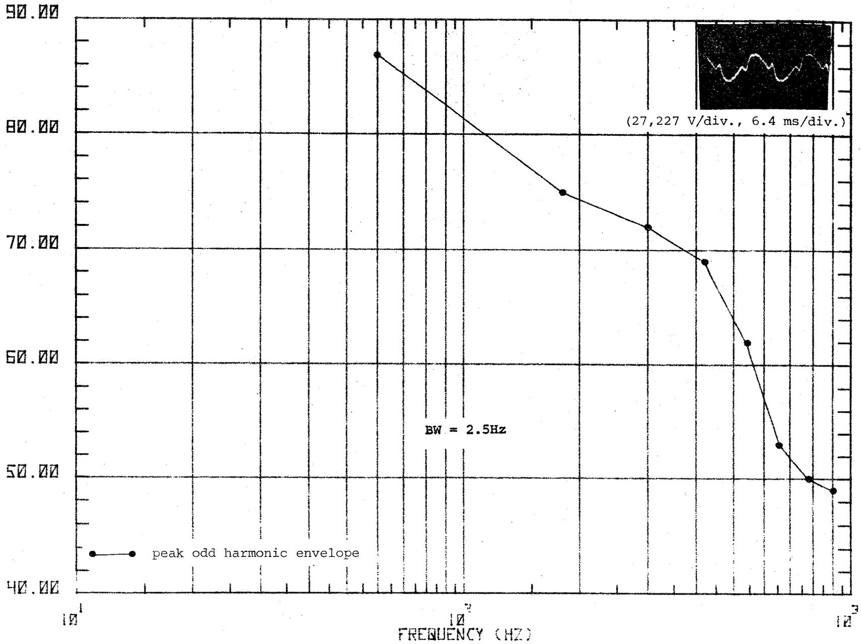
Figure 54i. Waveform and spectrum of catenary voltage sampled during 10-mph increment run, 90 to 100 mph.
