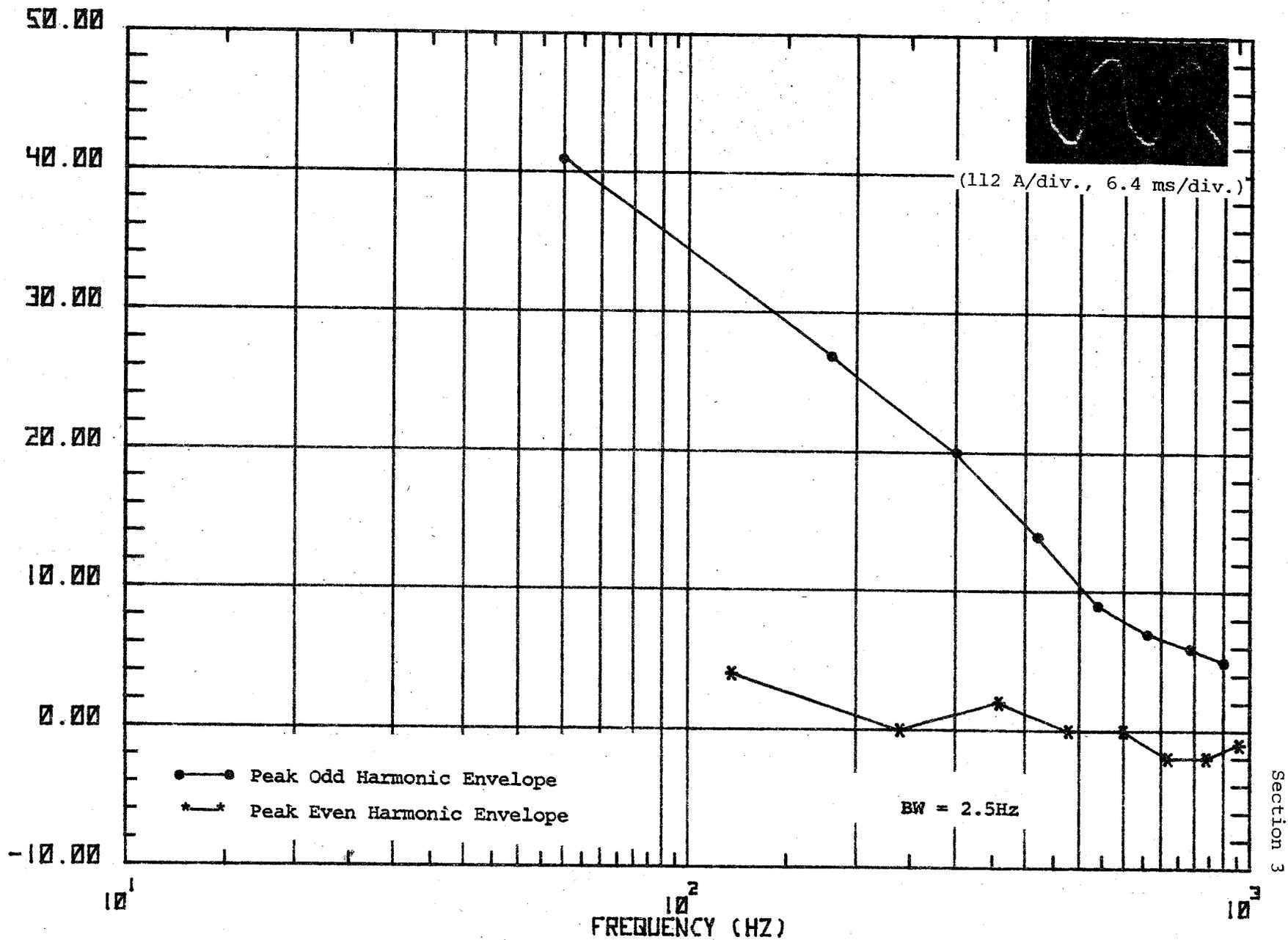
Figure 49k. Waveform and spectrum of primary current, locomotive accelerating from 110 to 115 mph.
