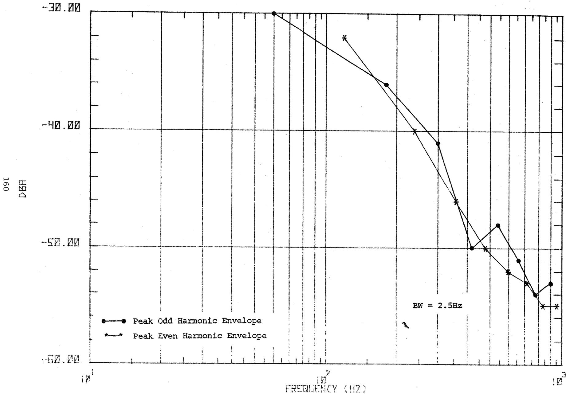
Figure 64. Spectrum of current in cab signal pickup as locomotive approaches phase break.
