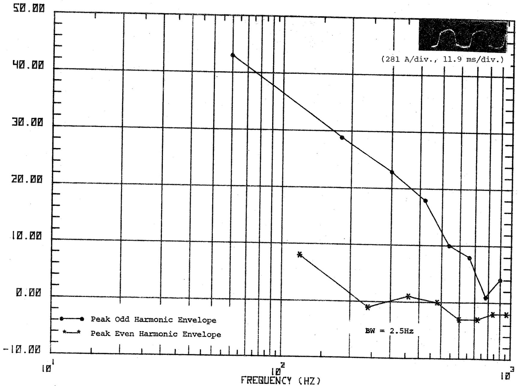
Figure 47. Waveform and spectrum of current in ground side of main transformer primary as locomotive approaches the substation.
