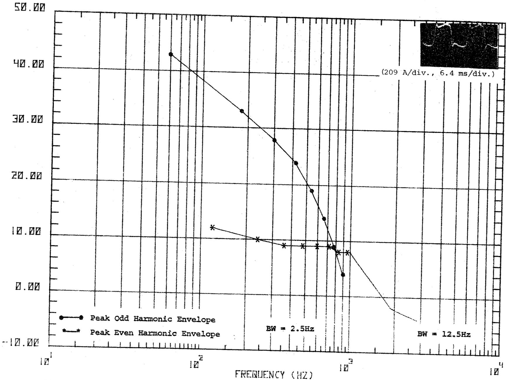
Figure 52k. Waveform and spectrum of primary current (sampled on the high side), locomotive accelerating from 100 to 110 mph.
