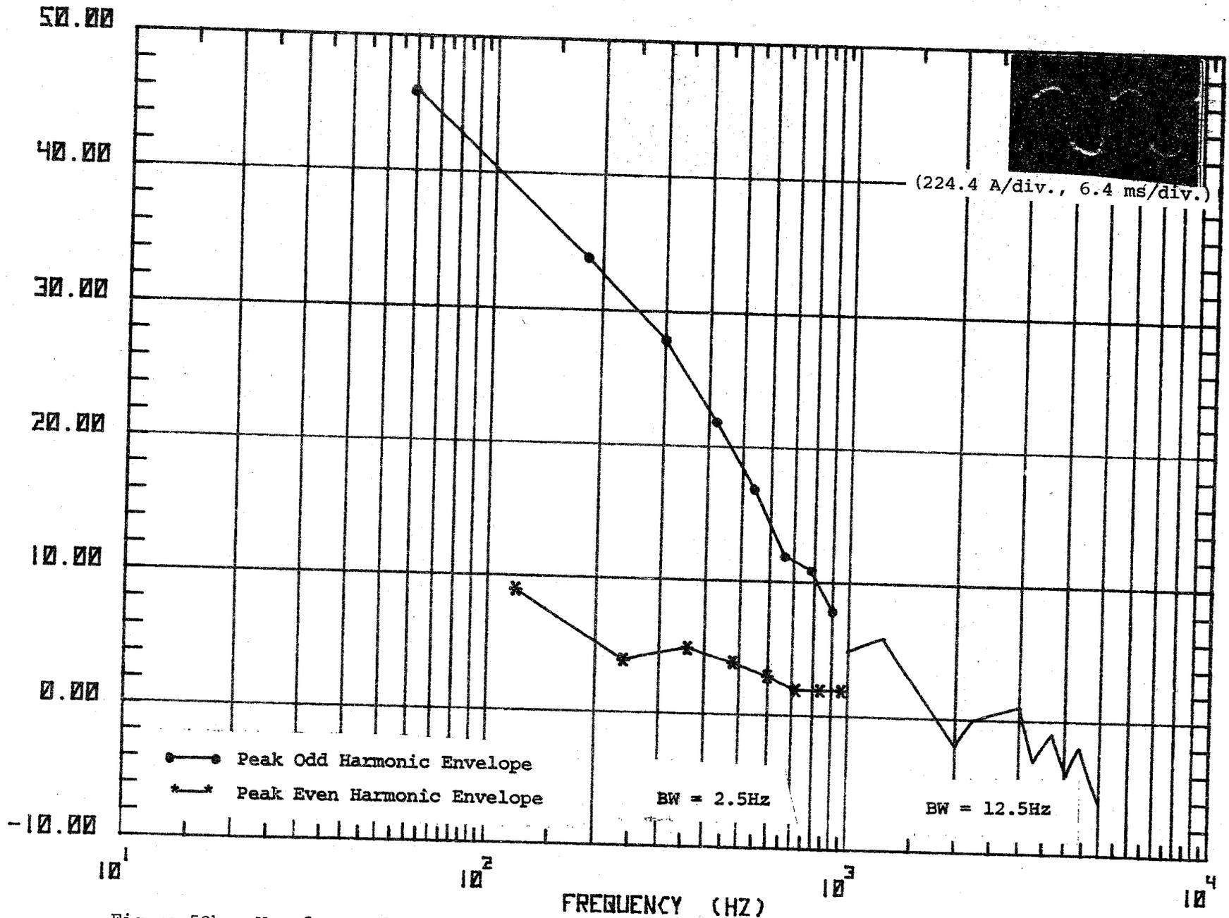
Figure 50h. Waveform and spectrum of primary current, locomotive accelerating from 70-80 mph (sample 2).
