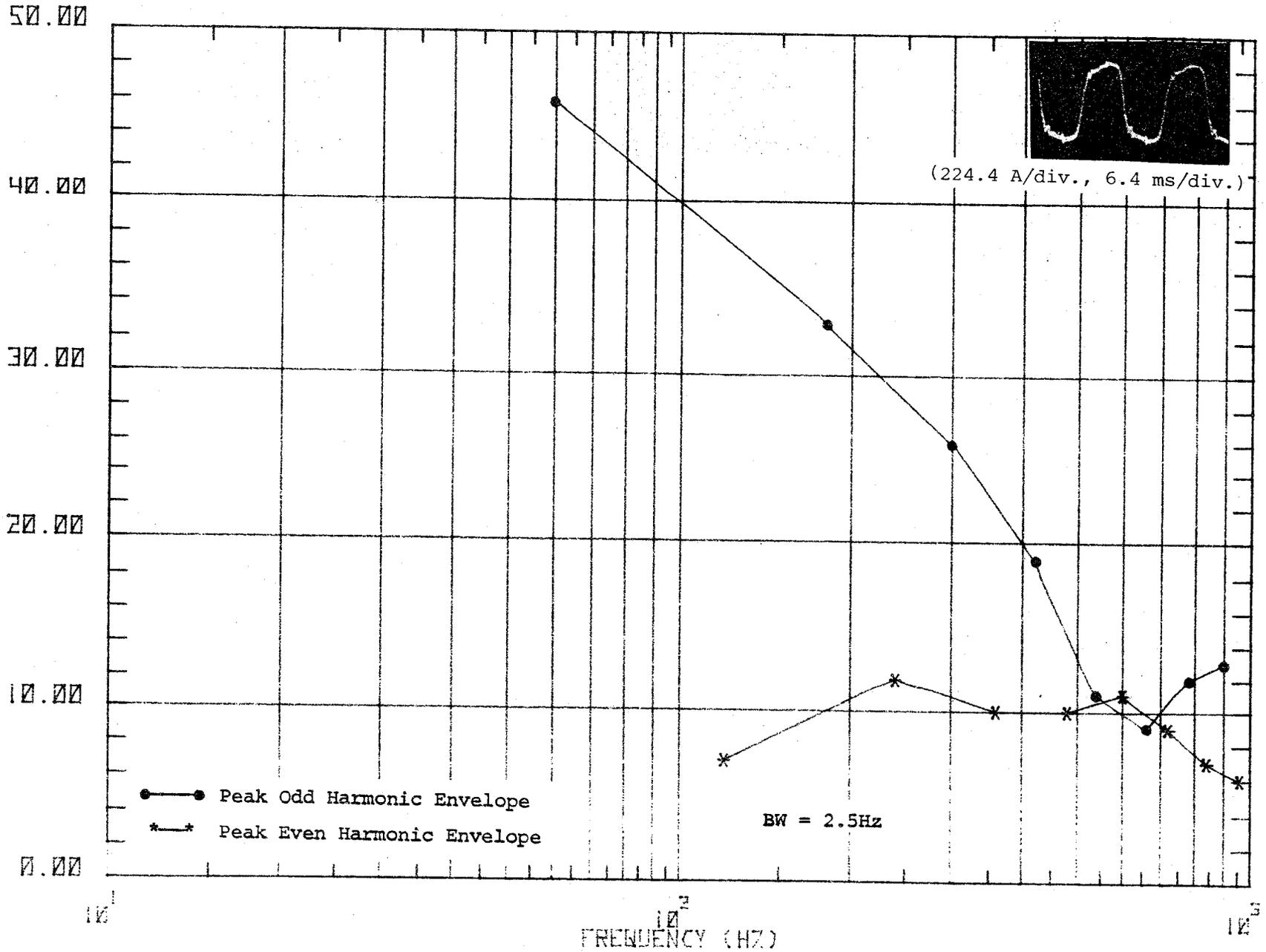
Figure 5le. Waveform and spectrum of primary current waveshape #5.
