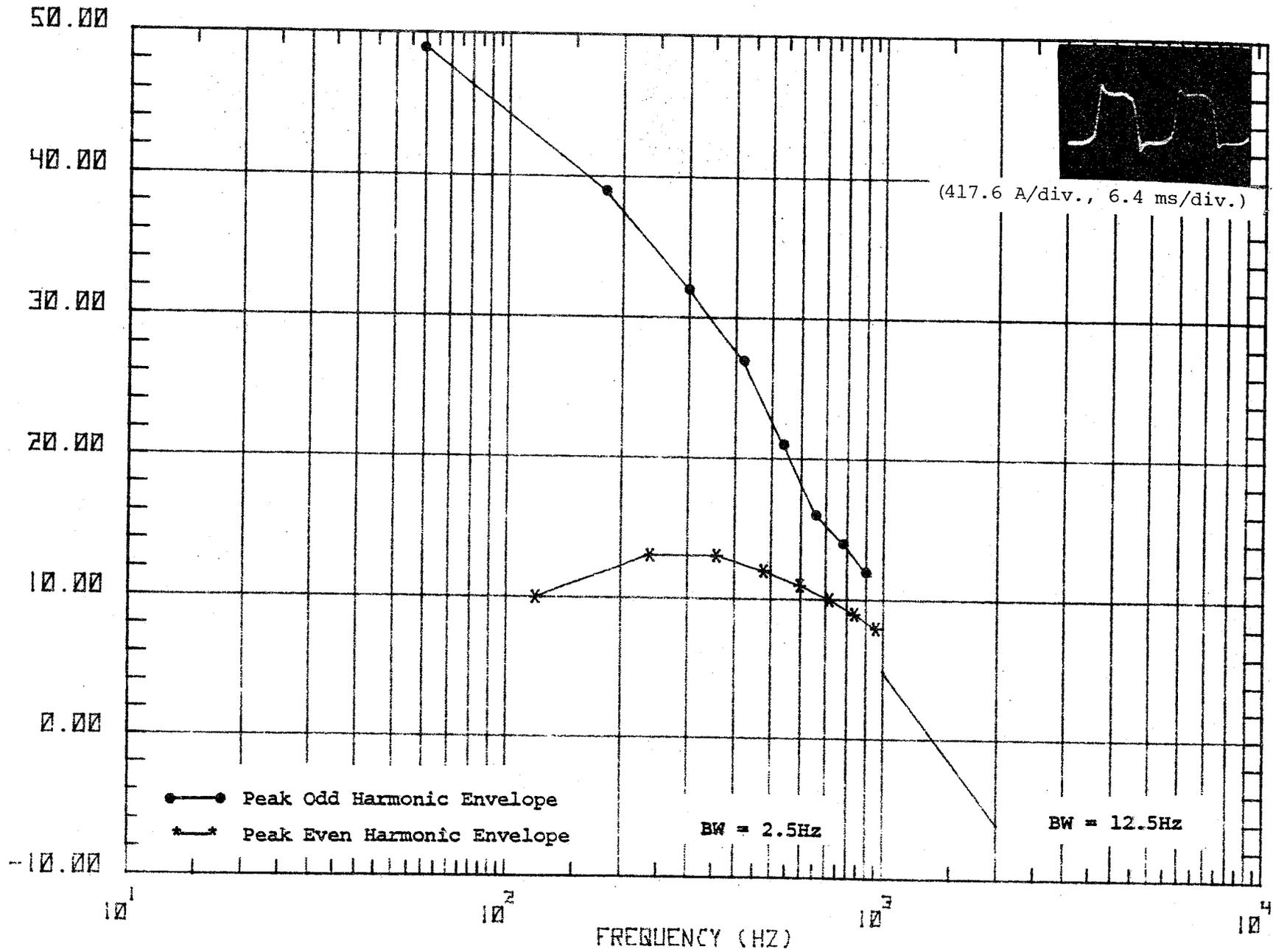
Figure 53. Waveform and spectrum of main transformer primary current (high side) sampled during a simulated revenue service run.
