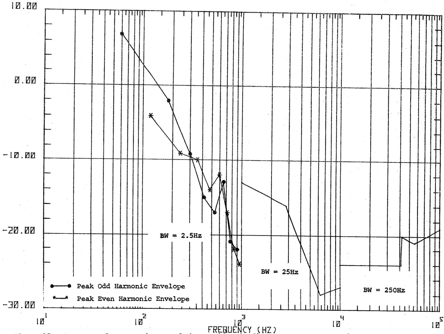
Figure 15. Spectrum of current in one of three cables leading to armature, traction motors off.
