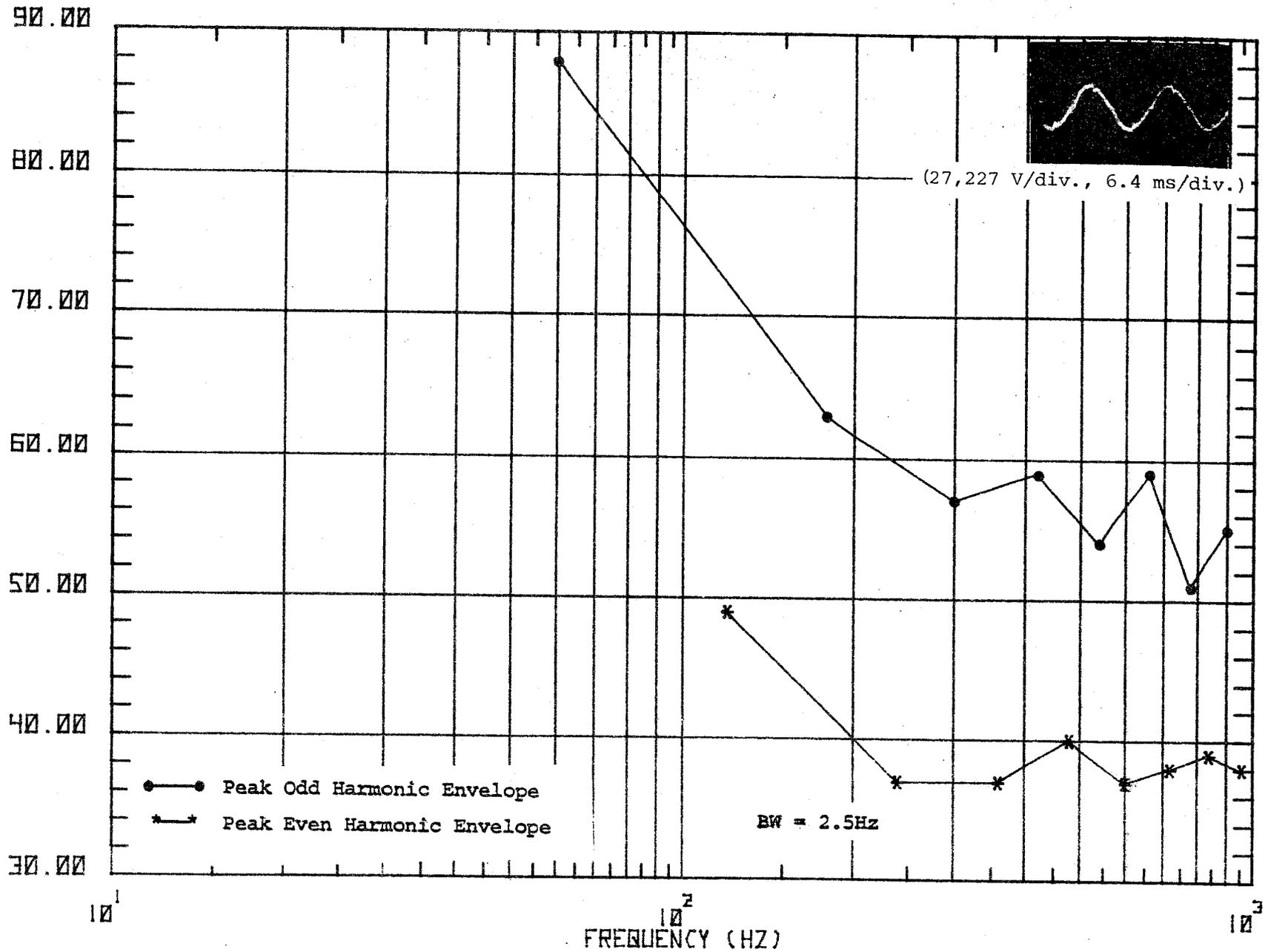
Figure 54a. Waveform and spectrum of catenary voltage sampled during 10-mph increment run, 10 to 20 mph.
