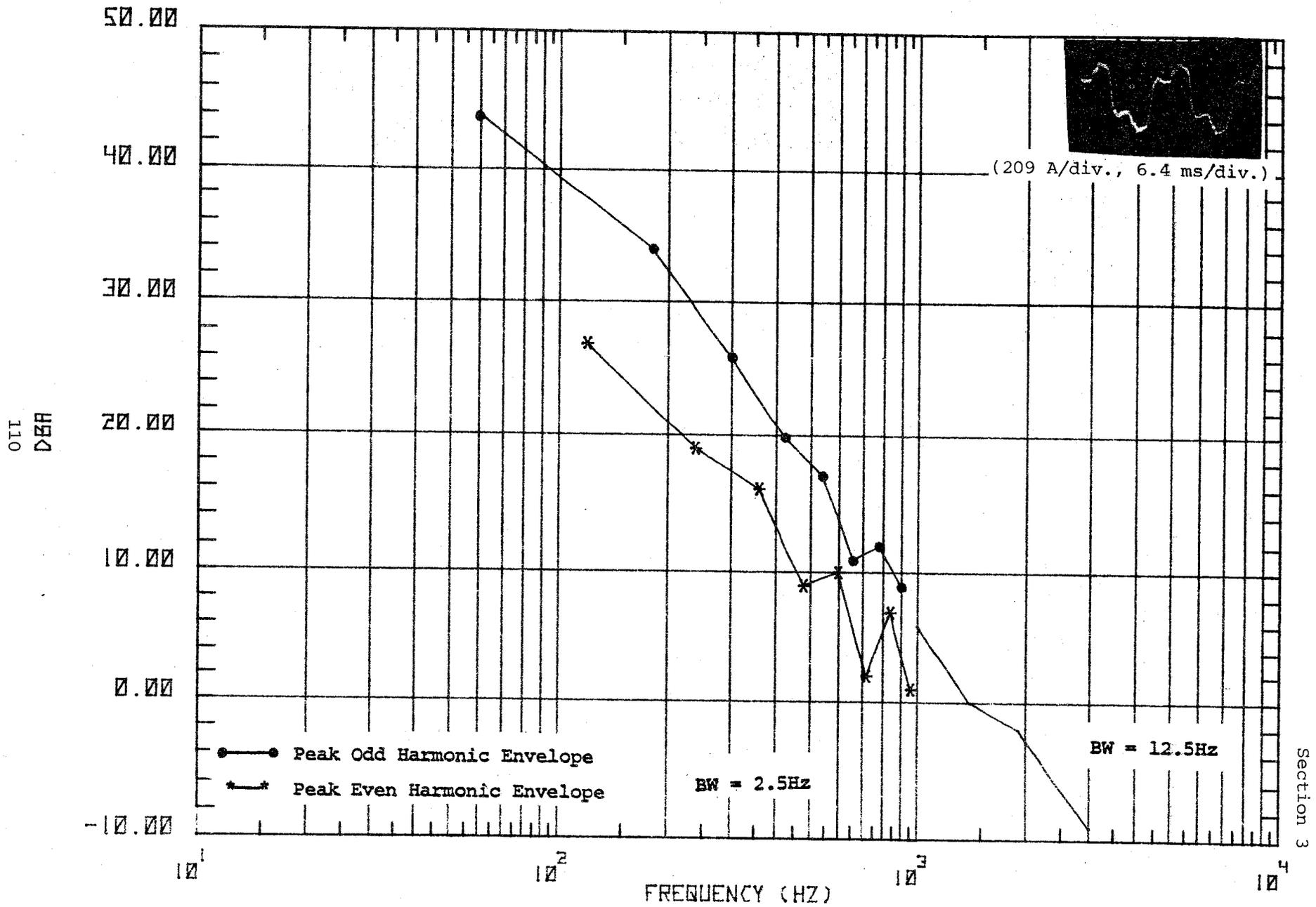
Figure 52d. Waveform and spectrum of primary current (sampled on the high side), locomotive accelerating from 30 to 40 mph.
