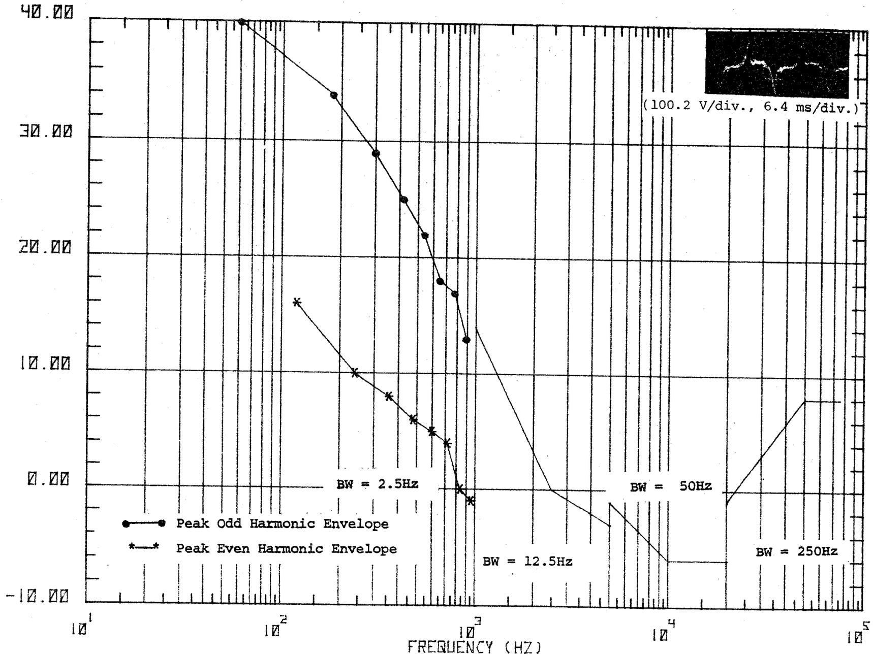
Figure 59. Waveform and spectrum of voltage across 74-volt bus as train runs simulated revenue service run.
