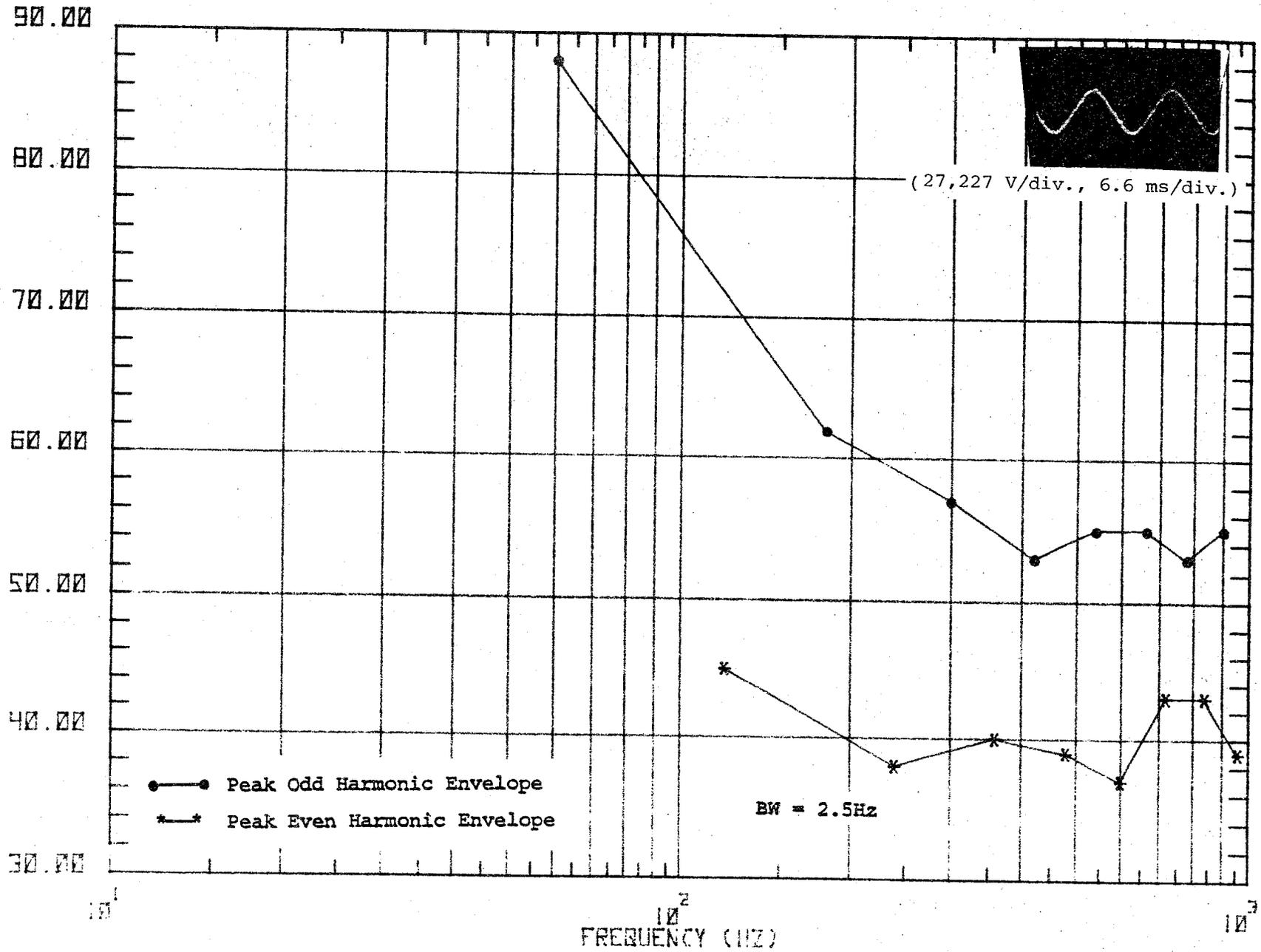
Figure 54c. Waveform and spectrum of catenary voltage sampled during 10-mph increment run, 30 to 40 mph.
