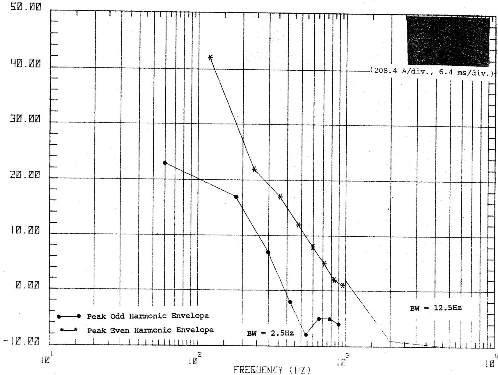
Figure 57g. Waveform and spectrum of armature current (ac) corresponding to primary current waveshape #7.
