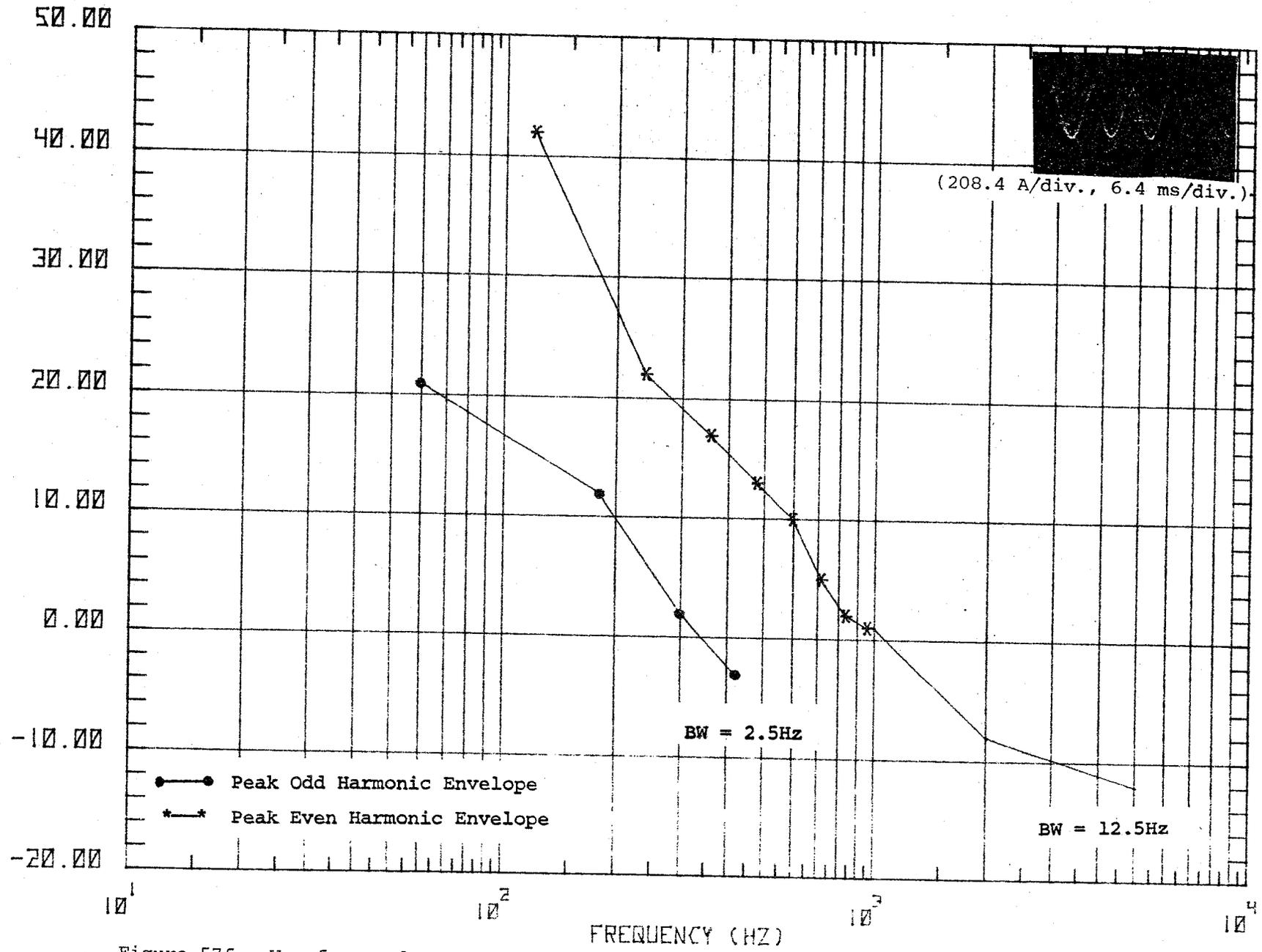
Figure 57f. Waveform and spectrum of armature current (ac) corresponding to primary current waveshape #6.
