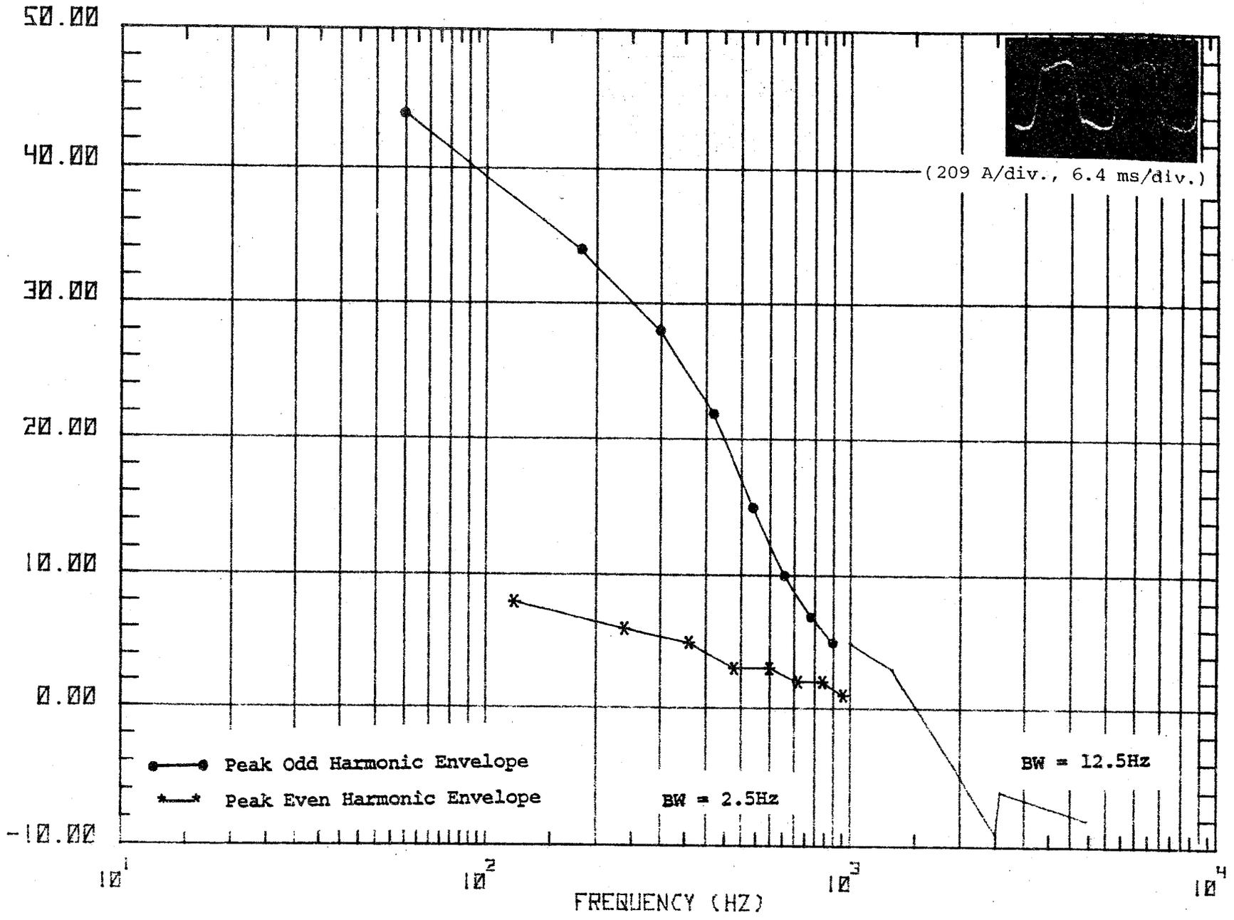
Figure 52h. Waveform and spectrum of primary current (sampled on the high side), locomotive accelerating from 70 to 80 mph.
