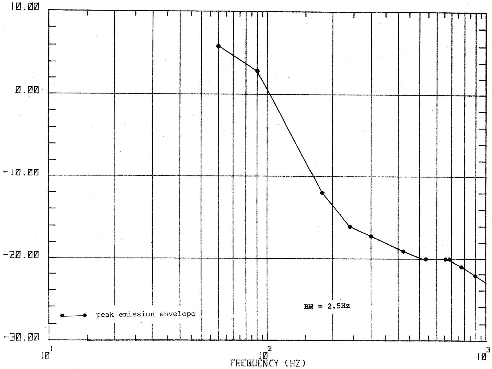
Figure 45. Spectrum of magnetic field strength, locomotive moving at 19 miles per hour.
