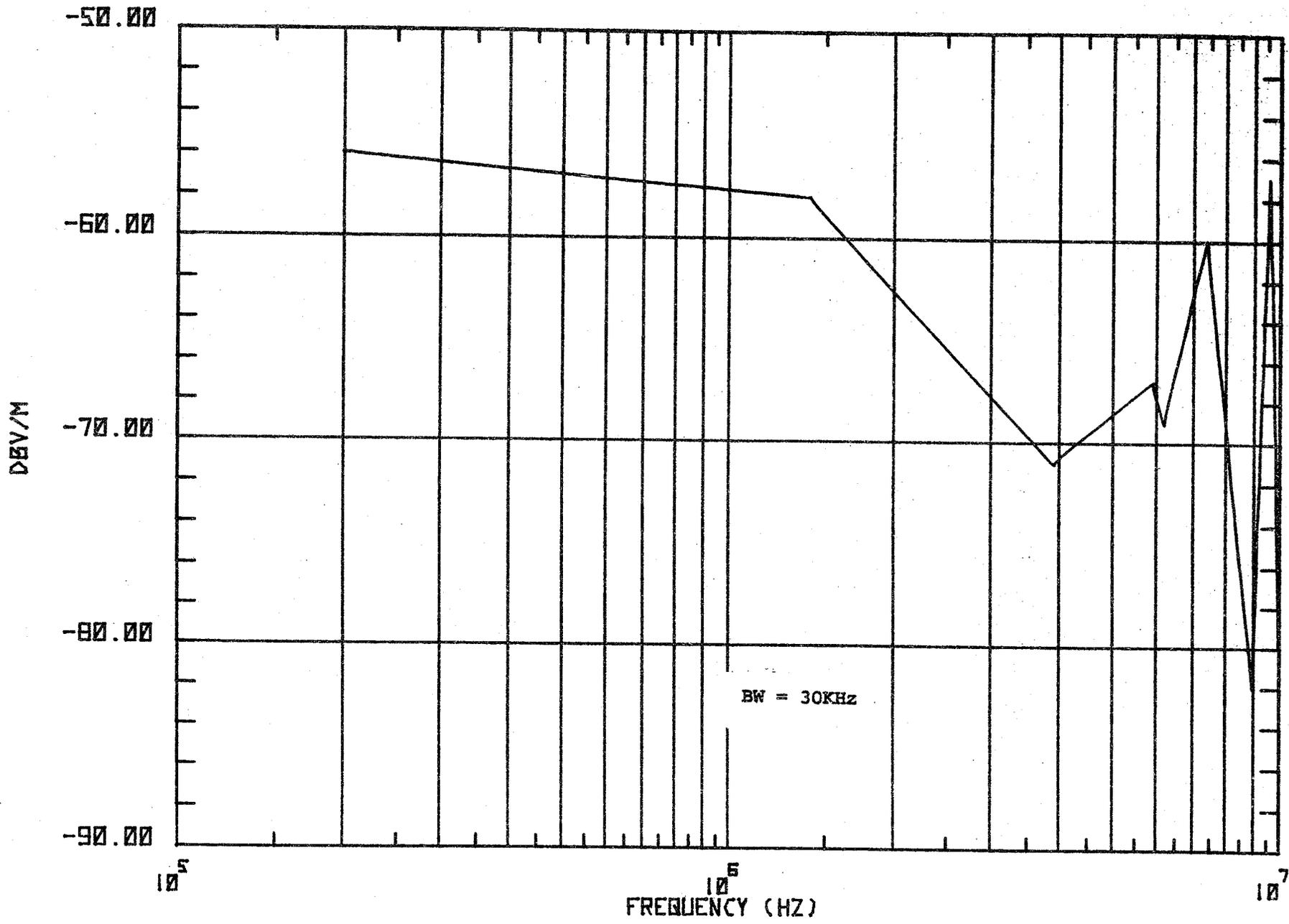
Figure 36. Spectrum of electric field strength sampled while locomotive coasted (Continued).
