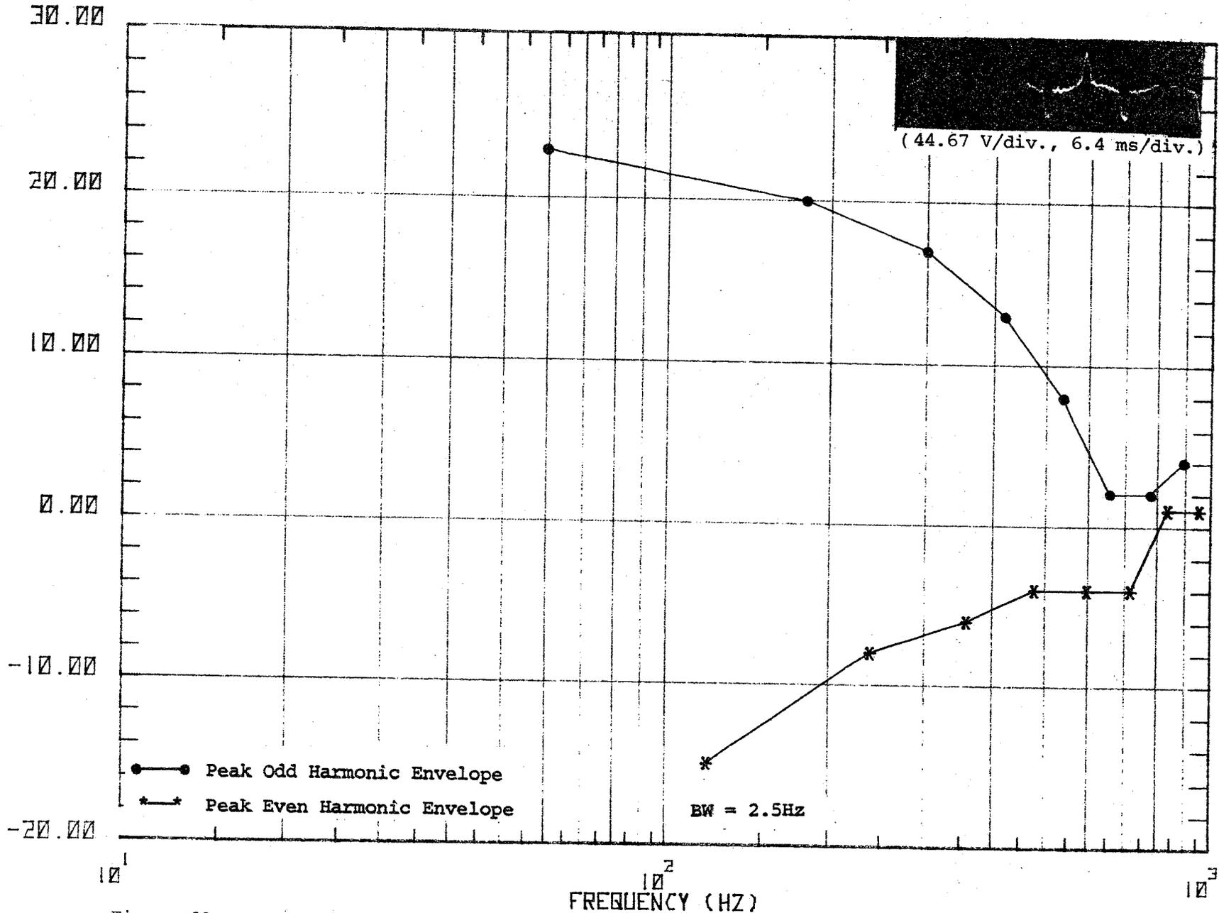
Figure 62. Waveform and spectrum of cab signal voltage sampled just after locomotive passed through phase break.
