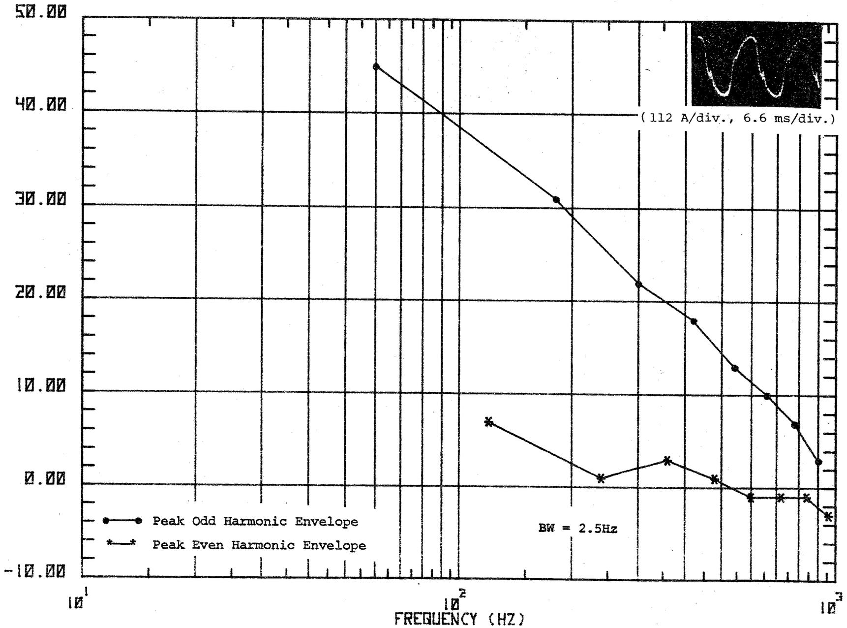
Figure 49f. Waveform and spectrum of primary current, locomotive accelerating from 60-70 mph.
