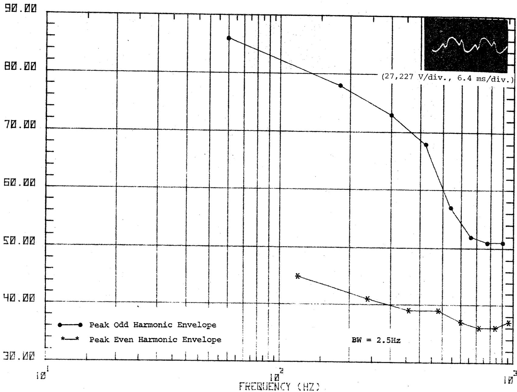
Figure 54g. Waveform and spectrum of catenary voltage sampled during 10-mph increment run, 70 to 80 mph.
