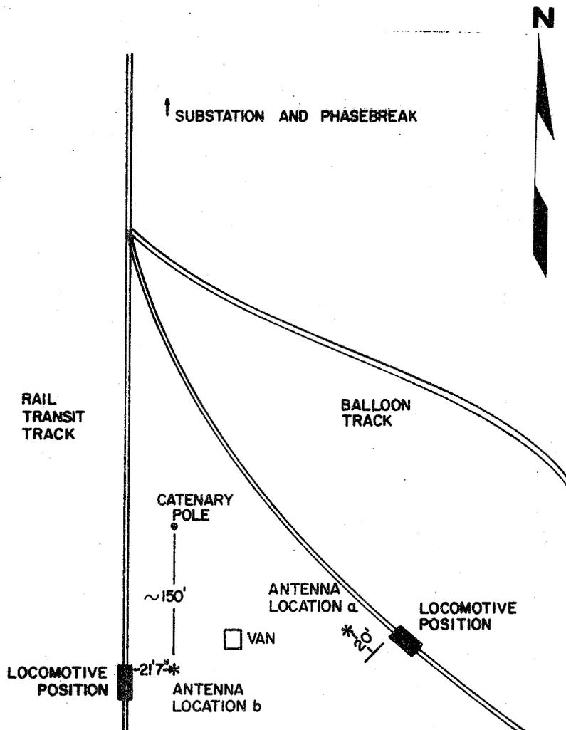
Figure 30. Electric field strength measurement locations.
