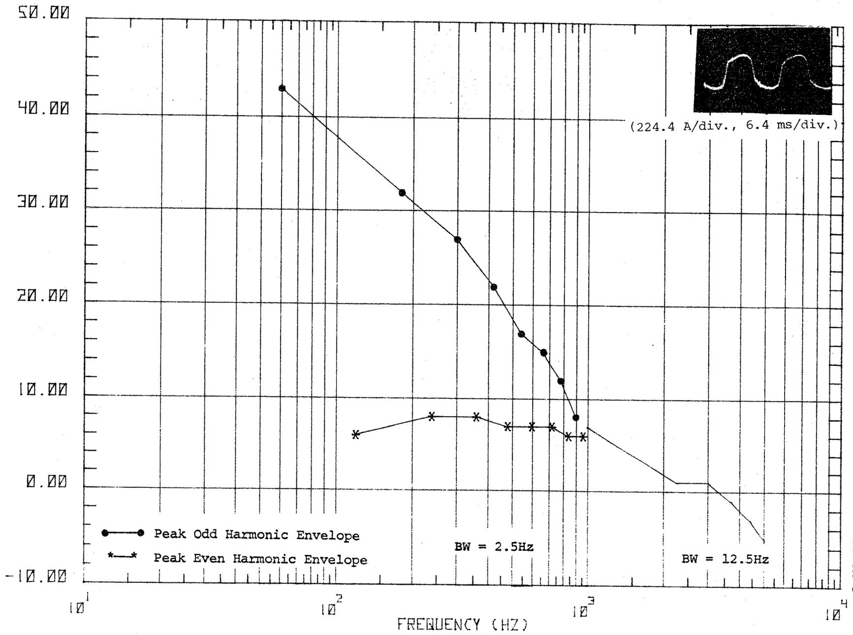
Figure 50k. Waveform and spectrum of primary current, locomotive accelerating from 100-110 mph (sample 2).
