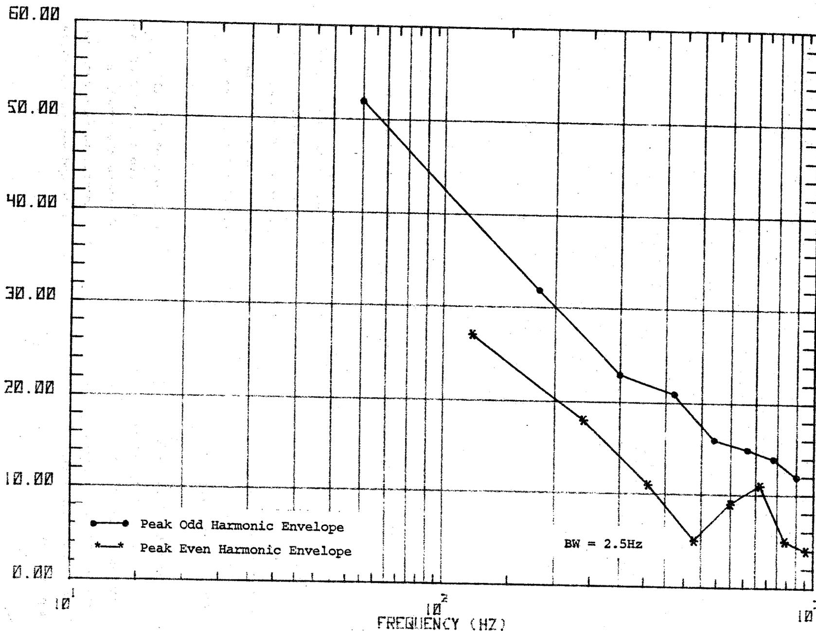
Figure 14. Spectrum of the current in one of three cables leading to armature, locomotive traveling at over 100 mph.
