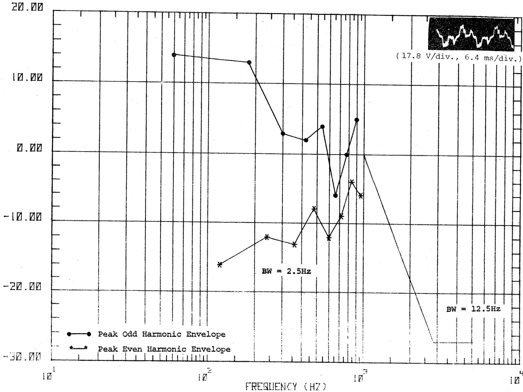
Figure 63b. Waveform and spectrum of cab signal voltage corresponding to ground side primary current waveshape #2.
