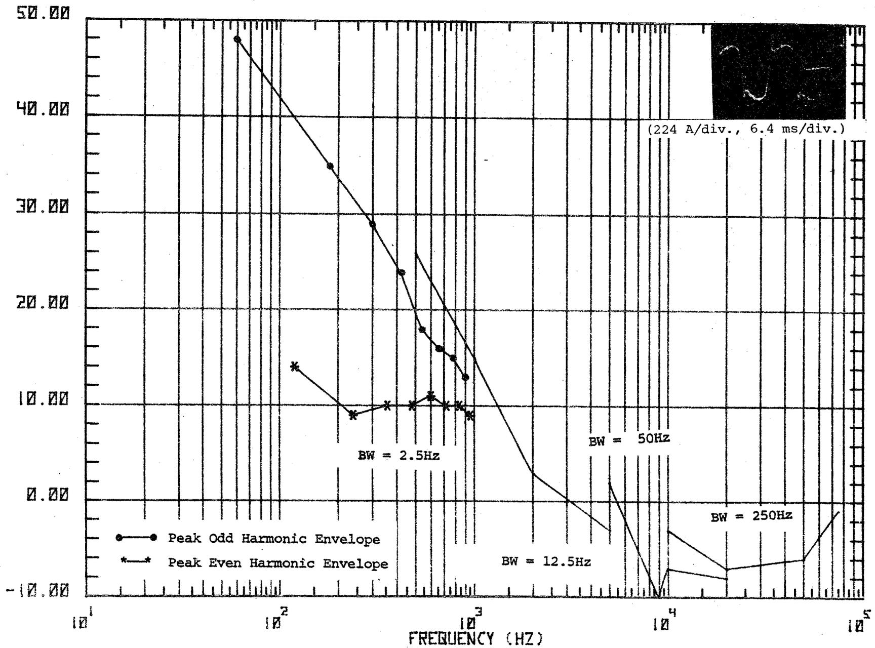
Figure 46. Waveform and spectrum of current in main transformer primary (ground side).
