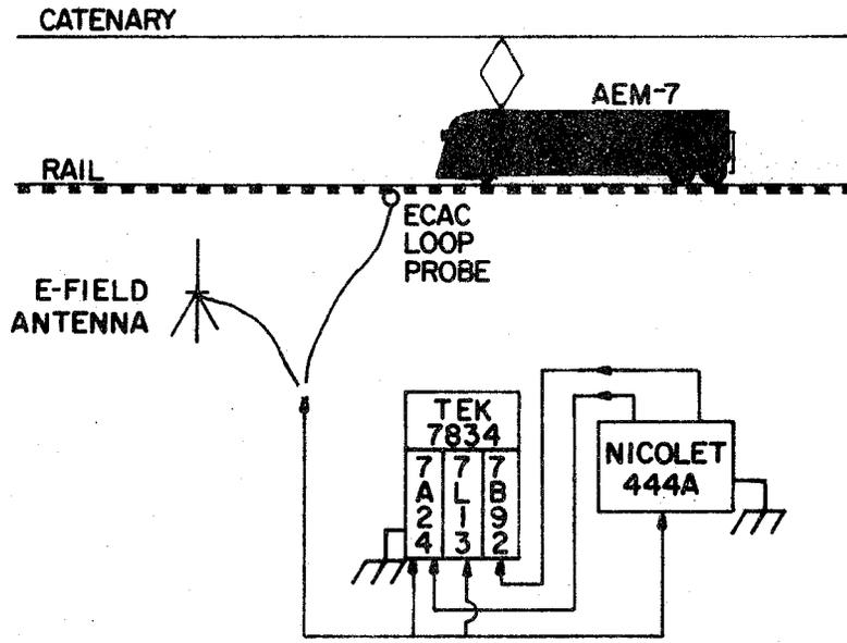
Figure 6. Real-time wayside measurement equipment setup.
