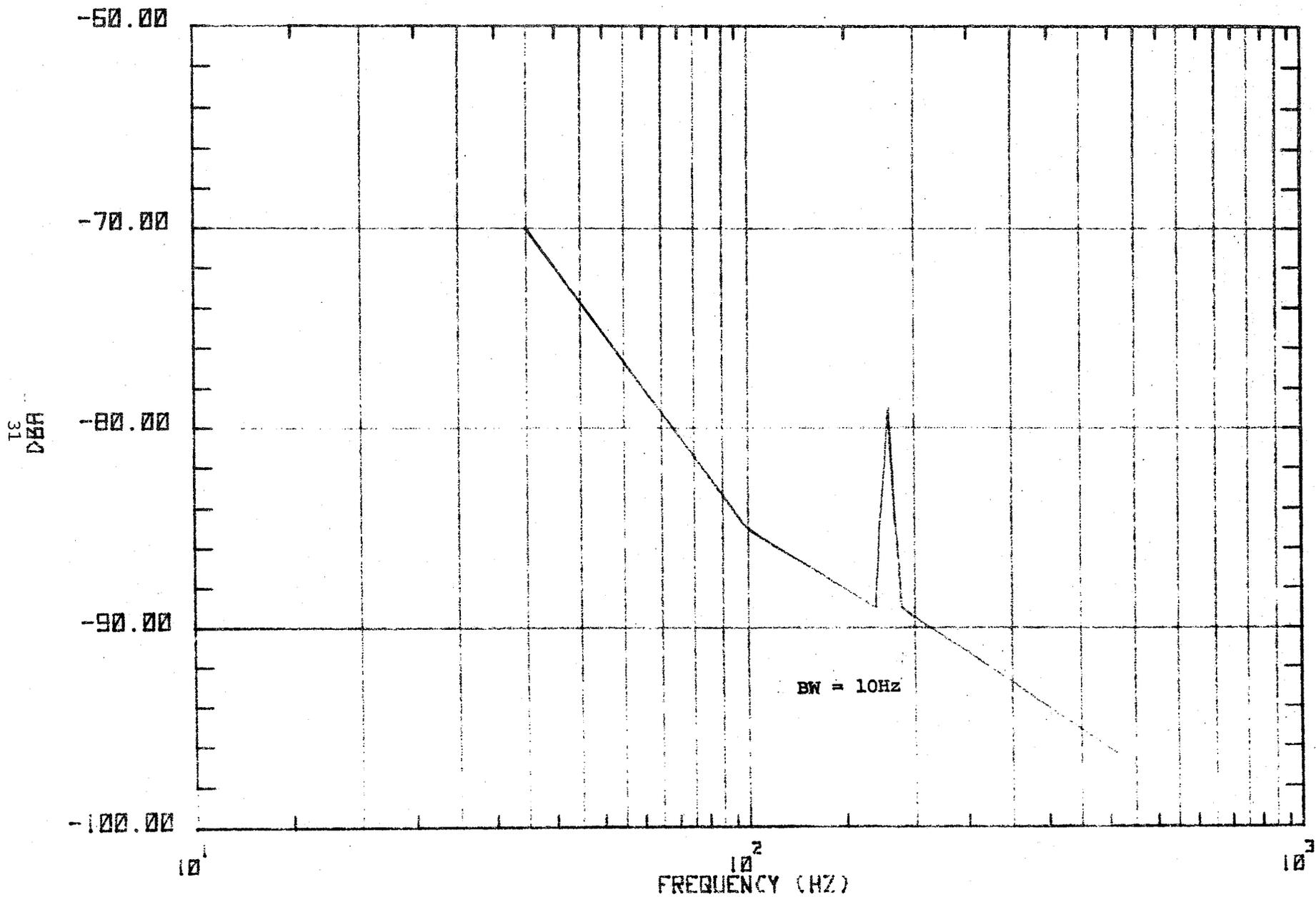
Figure 16. Spectrum of current in cab signal pickup, pantograph down.
