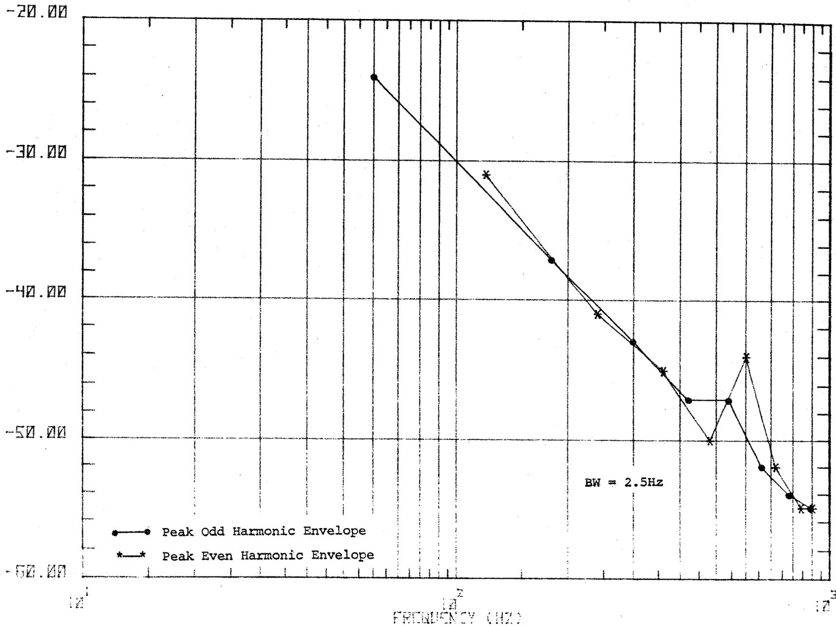
Figure 65. Spectrum of current in cab signal pickup as locomotive approaches phase break.
