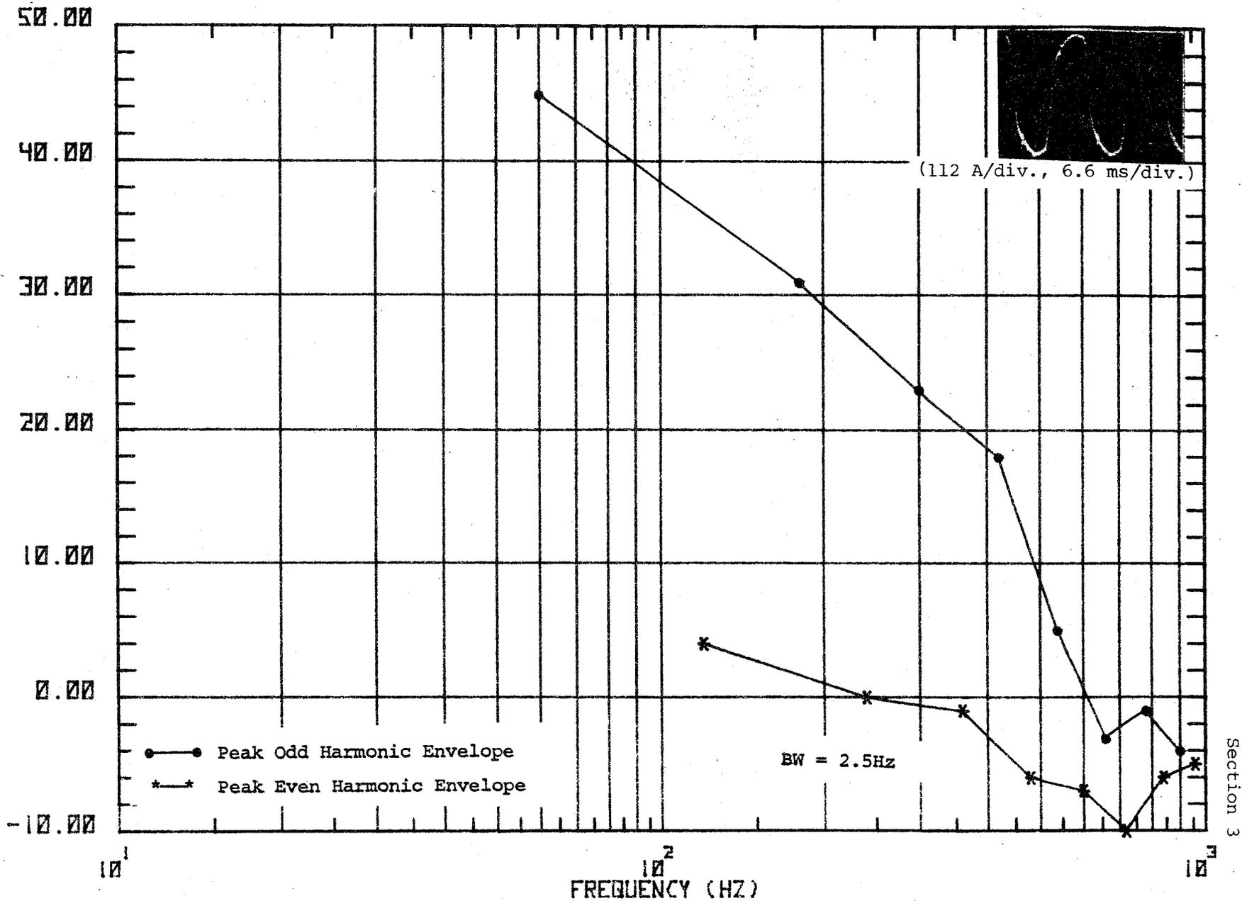
Figure 49g. Waveform and spectrum of primary current, locomotive accelerating from 70-80 mph.
