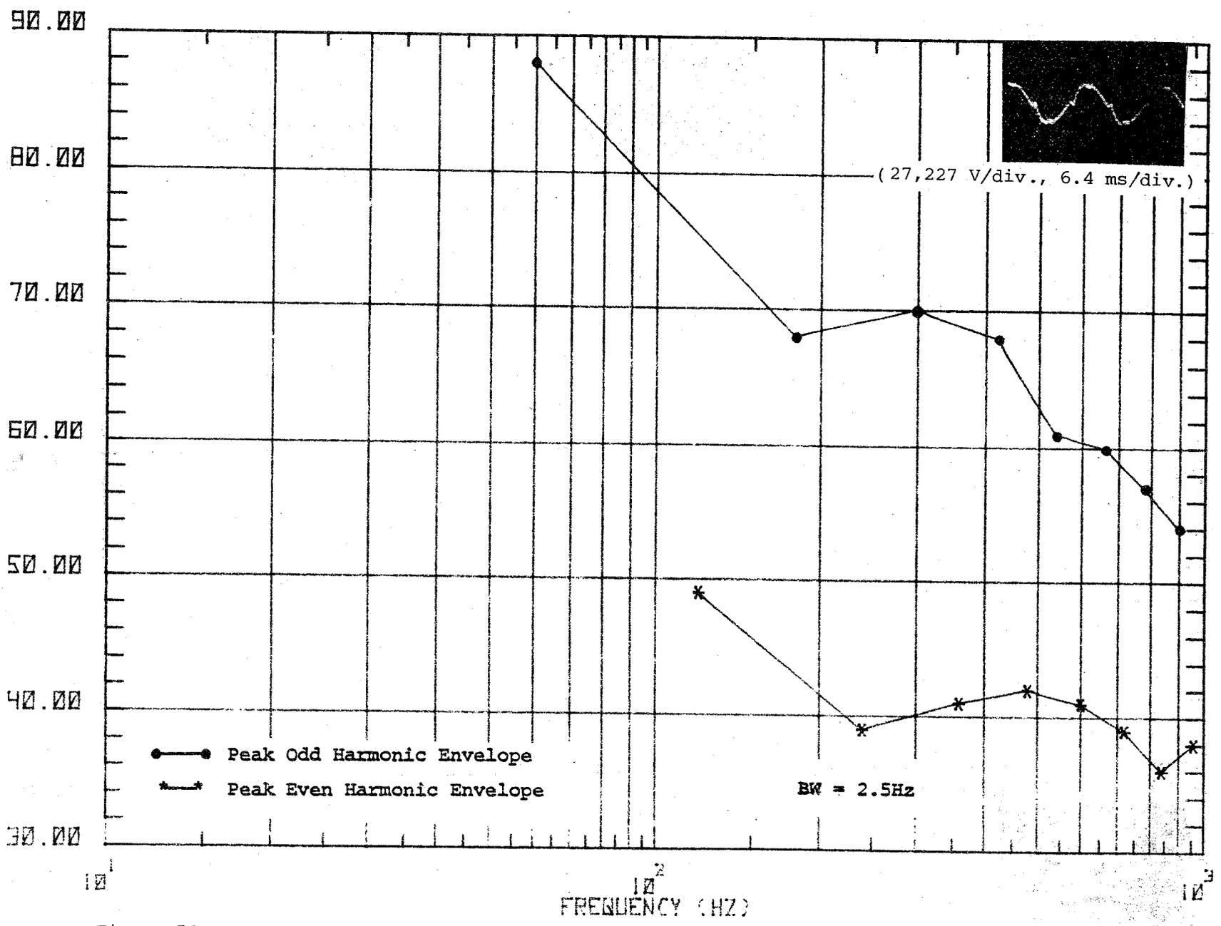
Figure 54e. Waveform and spectrum of catenary voltage sampled during 10-mph increment run, 50 to 60 mph.
