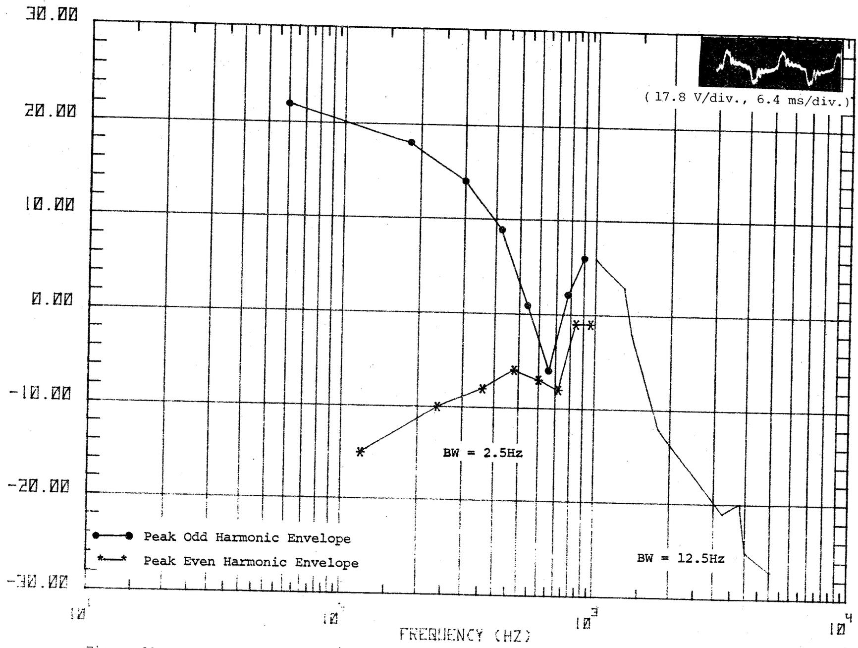
Figure 63e. Waveform and spectrum of cab signal voltage corresponding to ground side primary current waveshape #5.
