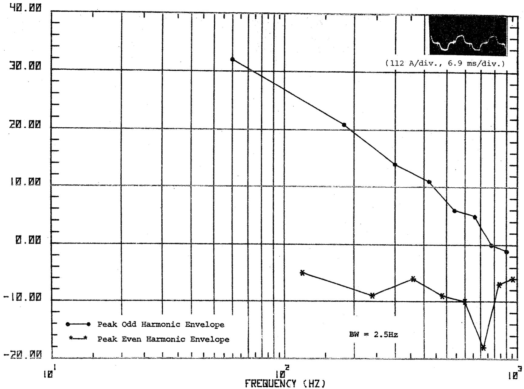
Figure 49a. Waveform and spectrum of primary current, locomotive accelerating from 10-20 mph.
