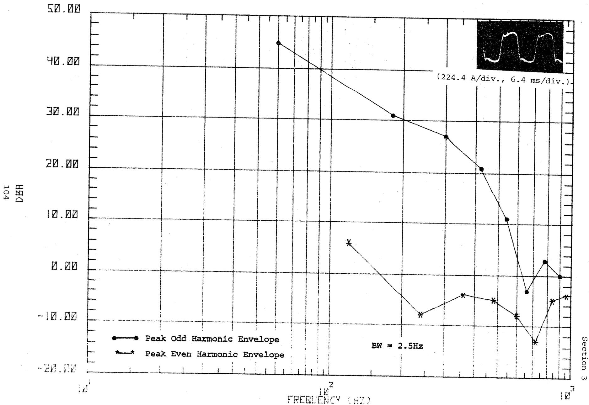
Figure 51f. Waveform and spectrum of ground side primary waveshape #6.
