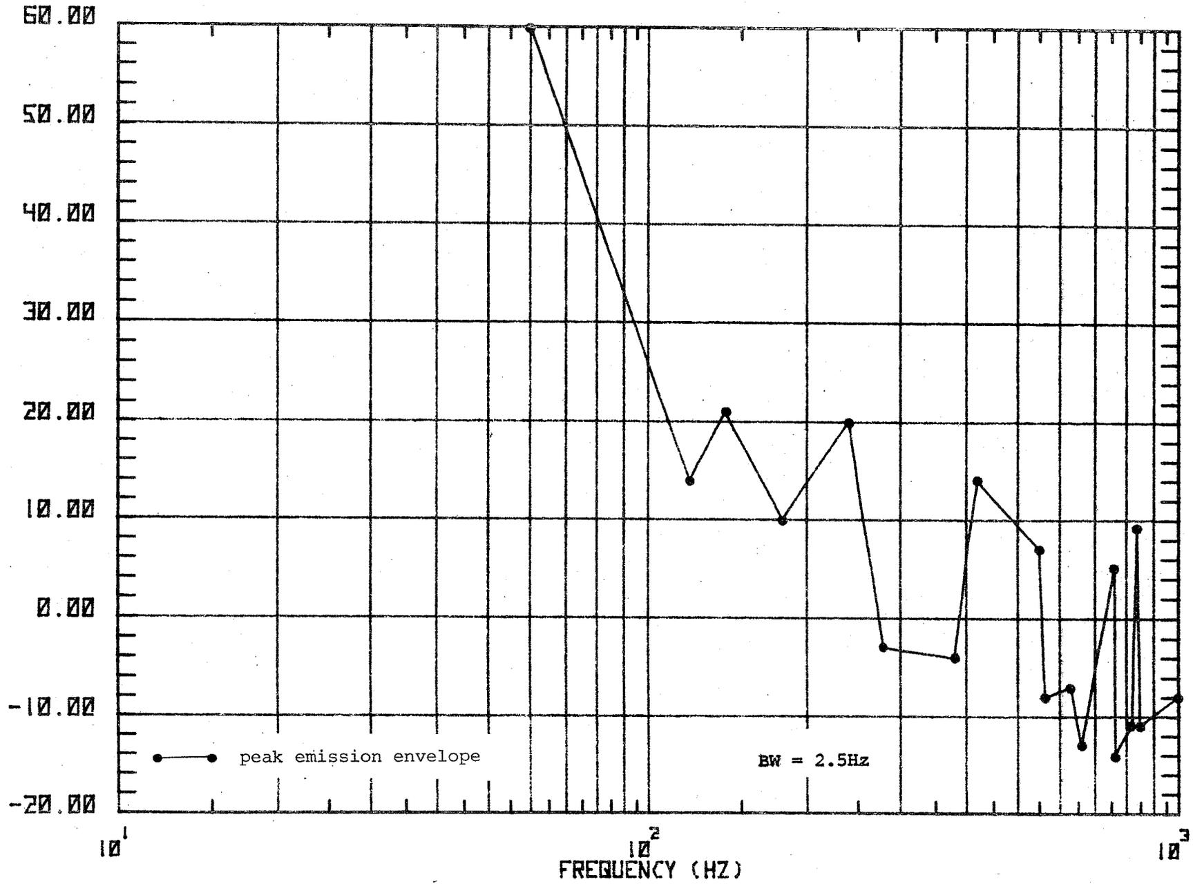
Figure 34. Spectrum of electric field strength, locomotive idling (sample 2).
