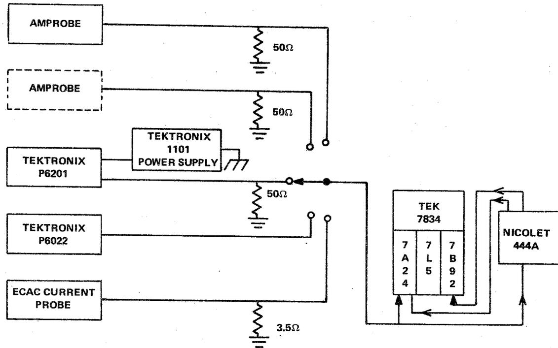
Figure 5. Real-time on board measurement equipment setup.
