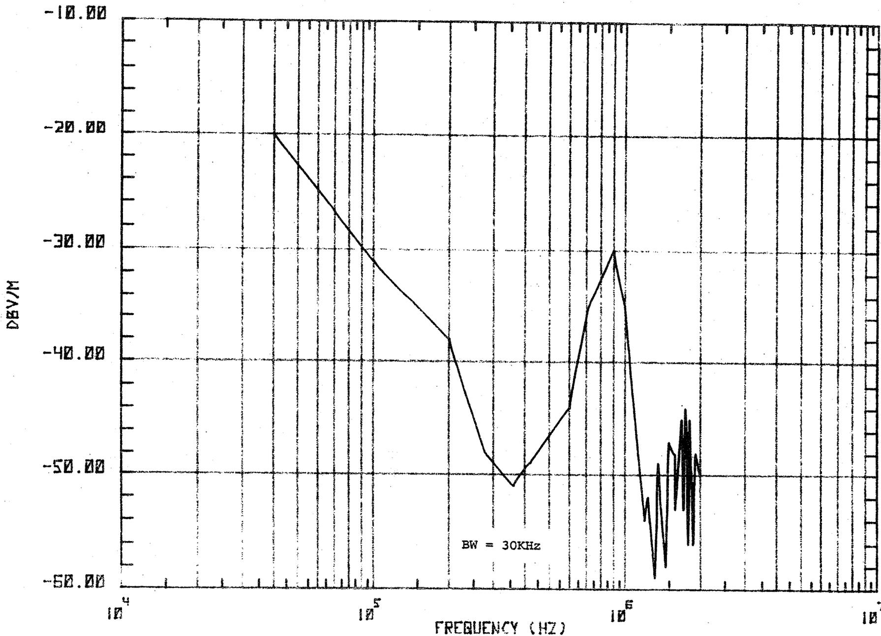
Figure 31. Spectrum of electric field strength of the ambient environment.
