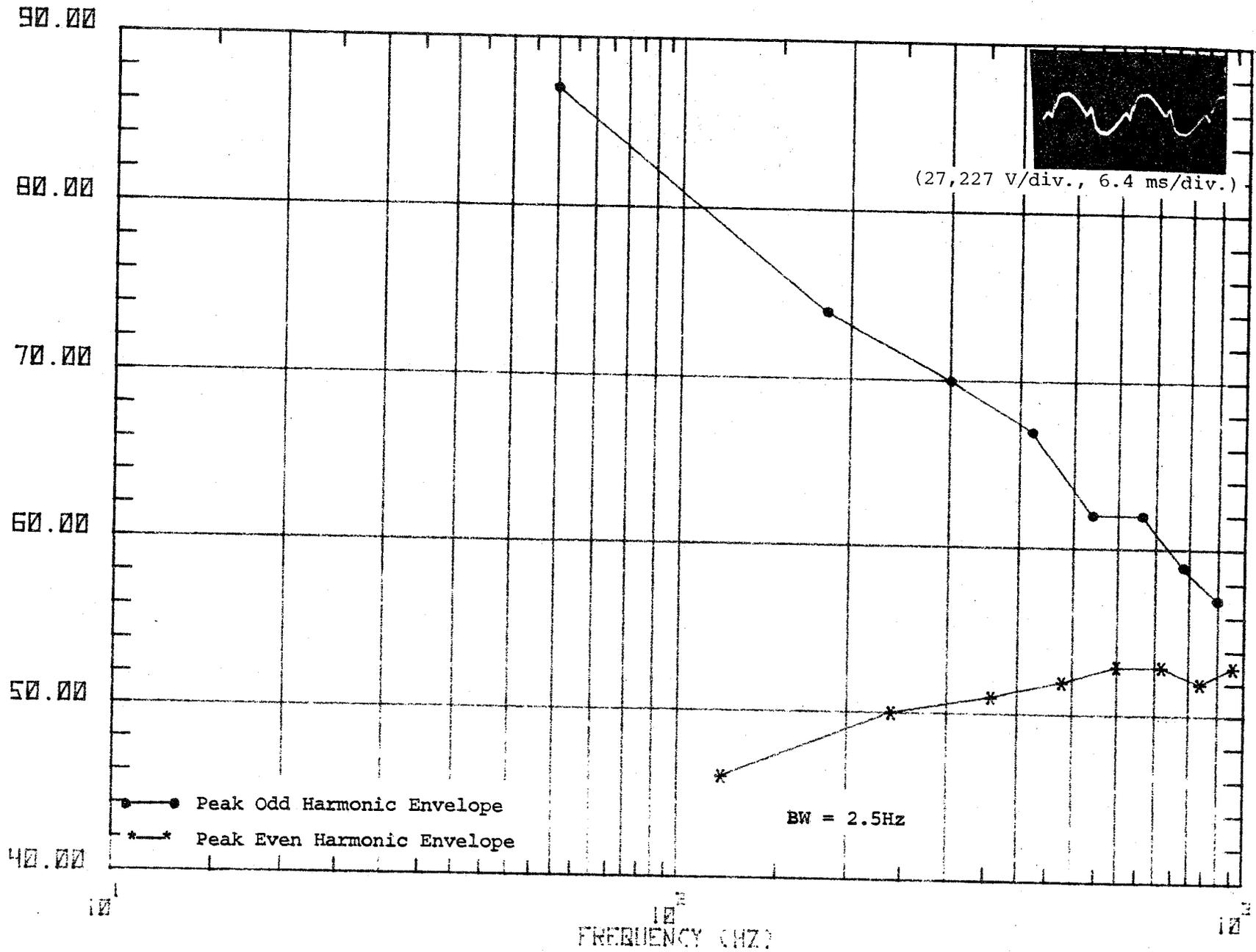
Figure 54k. Waveform and spectrum of catenary voltage sampled during 10-mph increment run, 110 to 115 mph.
