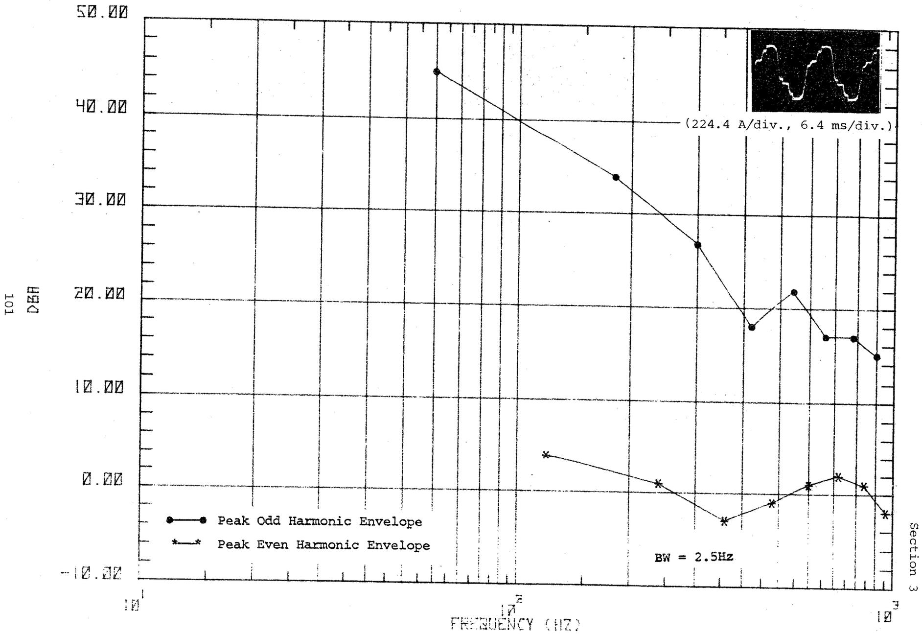
Figure 51c. Waveform and spectrum of primary current waveshape #3.
