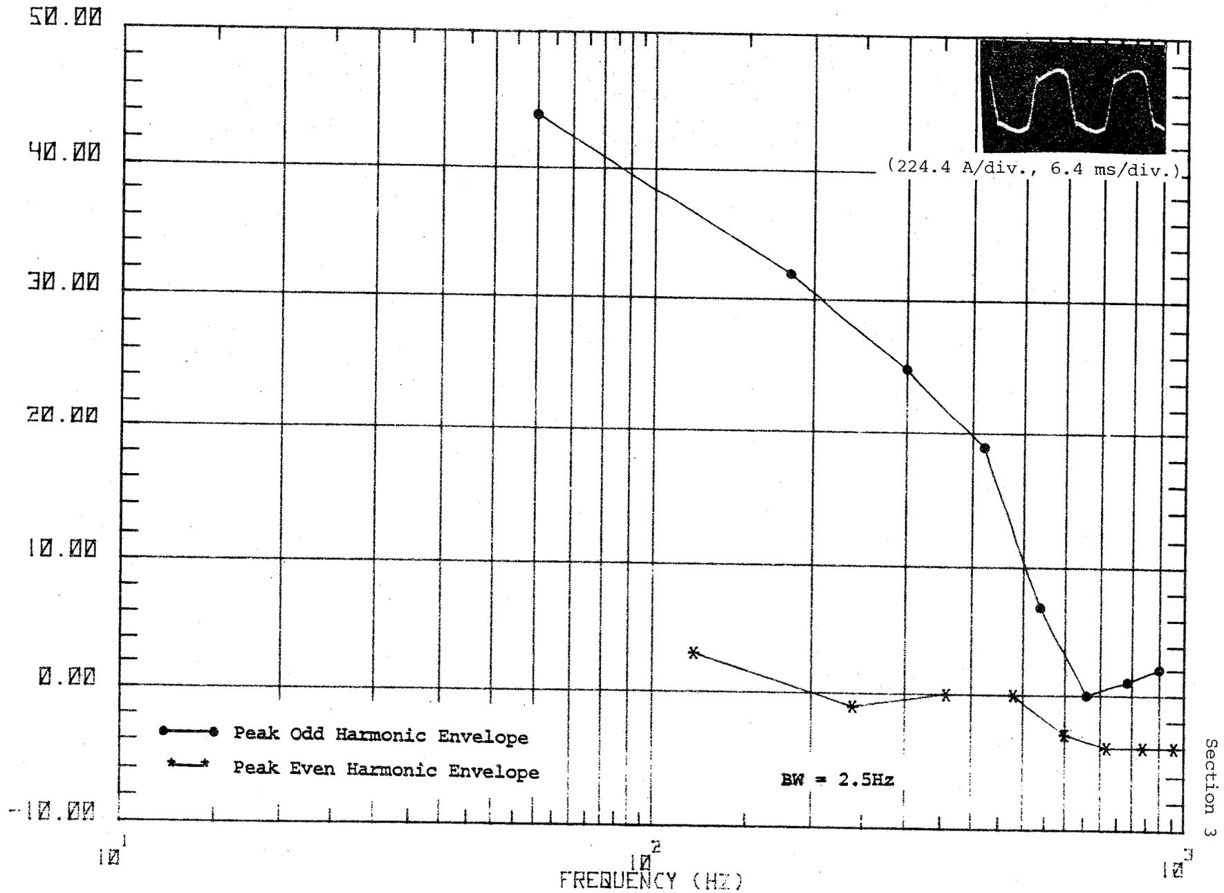
Figure 51g. Waveform and spectrum of ground side primary current waveshape #7.
