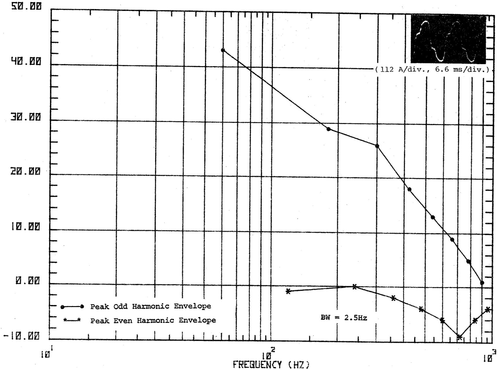
Figure 49e. Waveform and spectrum of primary current, locomotive accelerating from 50-60 mph.
