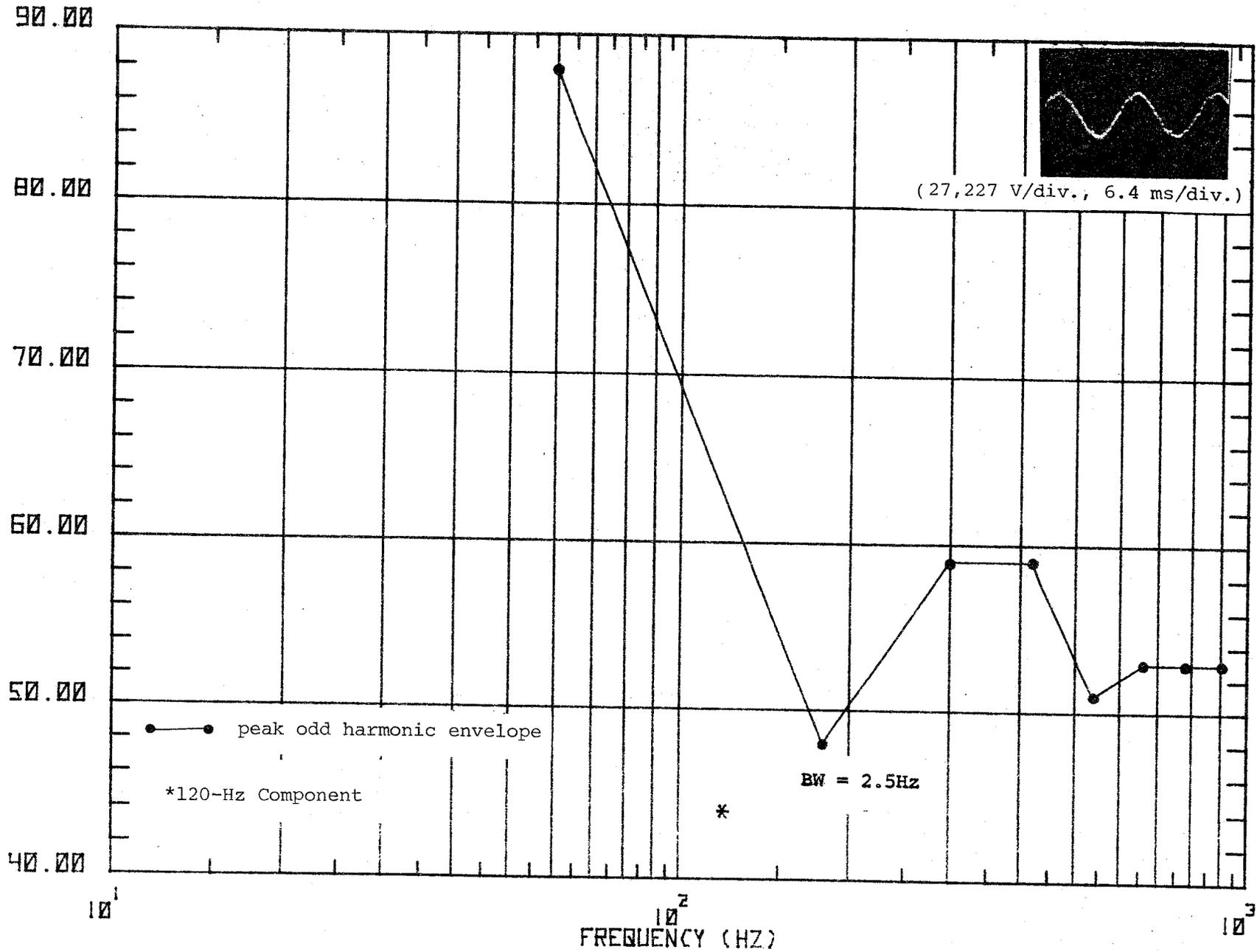
Figure 54b. Waveform and spectrum of catenary voltage sampled during 10-mph increment run, 20 to 30 mph.
