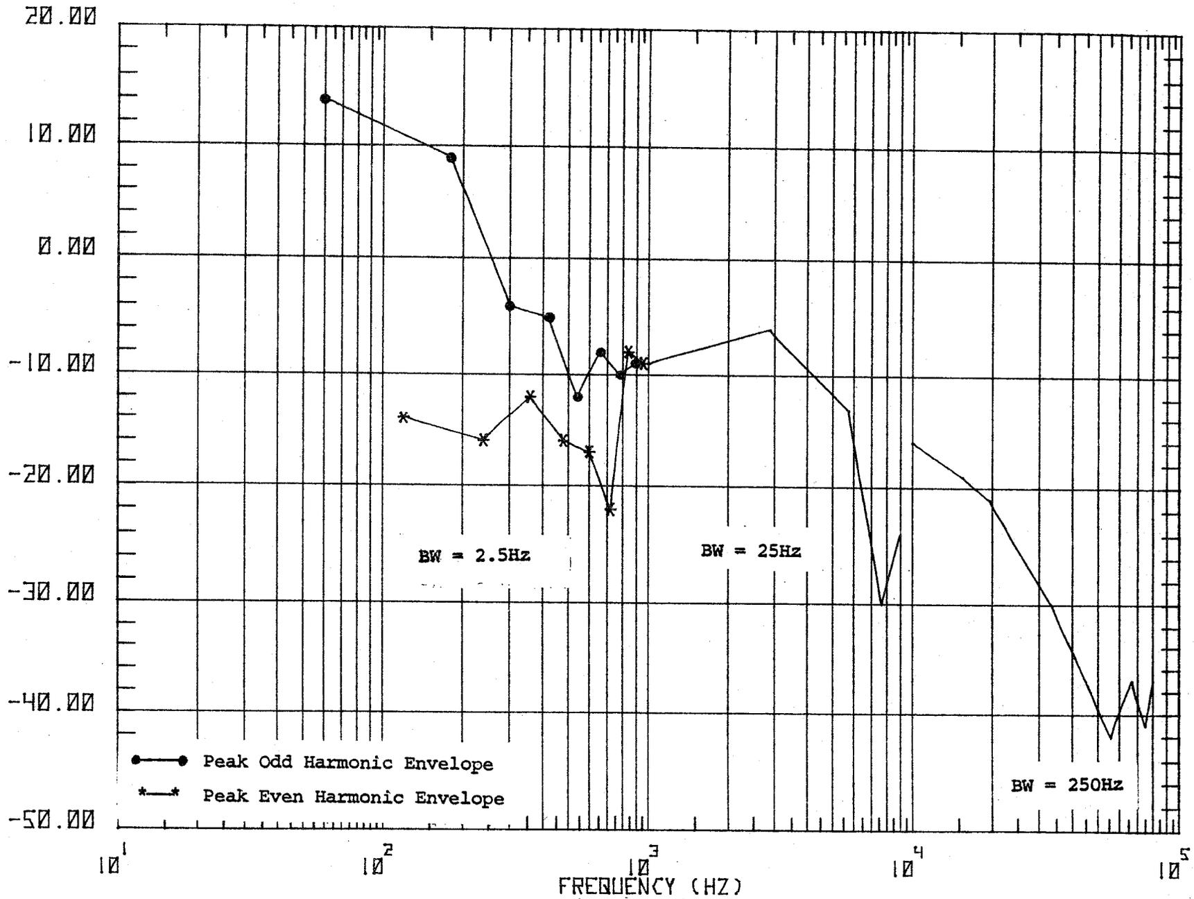
Figure 9. Spectrum of ground side primary current sampled while locomotive was traveling at slow speed.
