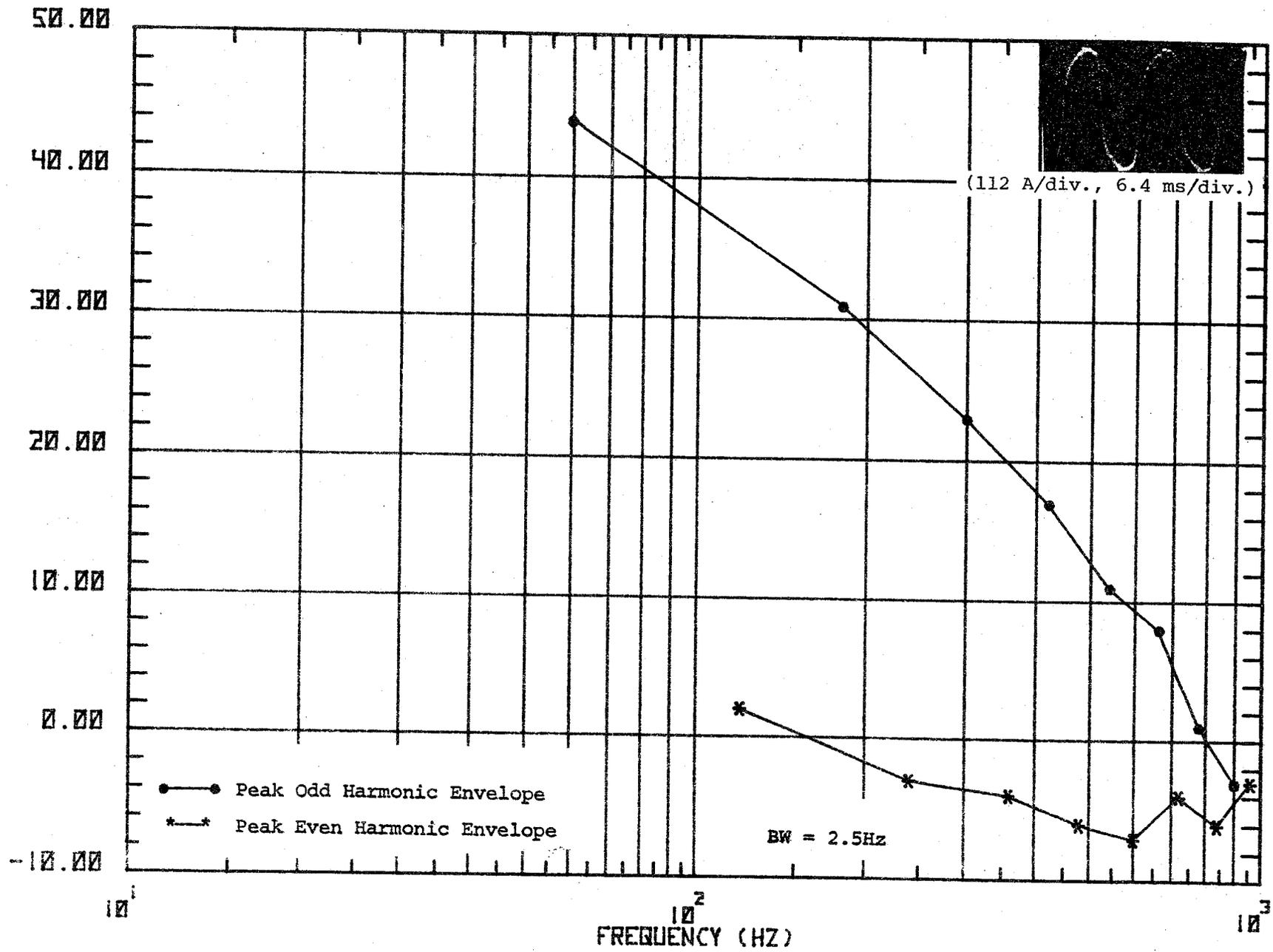
Figure 49h. Waveform and spectrum of primary current, locomotive accelerating from 80-90 mph.
