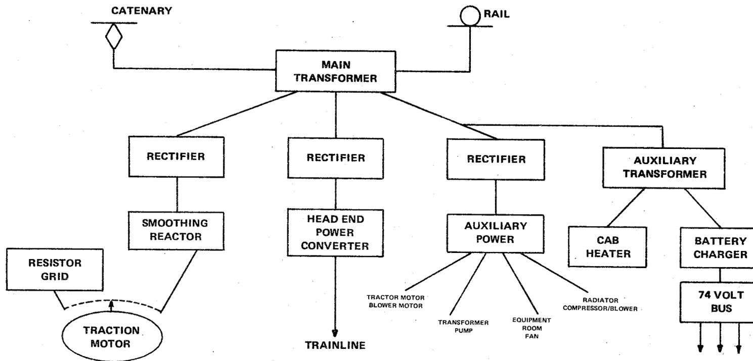
Figure 1. Block diagram of the major electrical systems on an AEM-7 locomotive.
