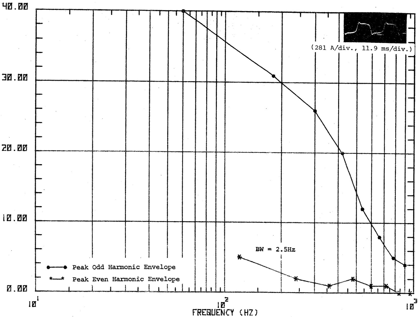
Figure 48. Waveform and spectrum of primary current (ground side) as locomotive passes substation.
