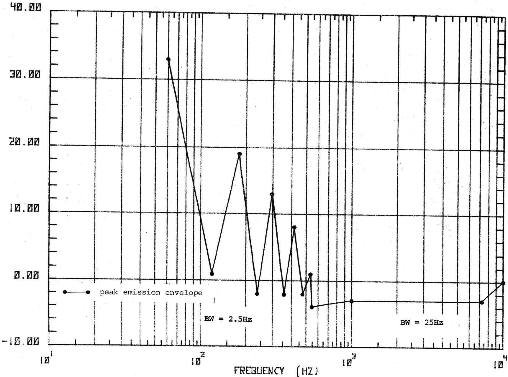
Figure 28. Spectrum of current in one rail as locomotive passes measurement location.
