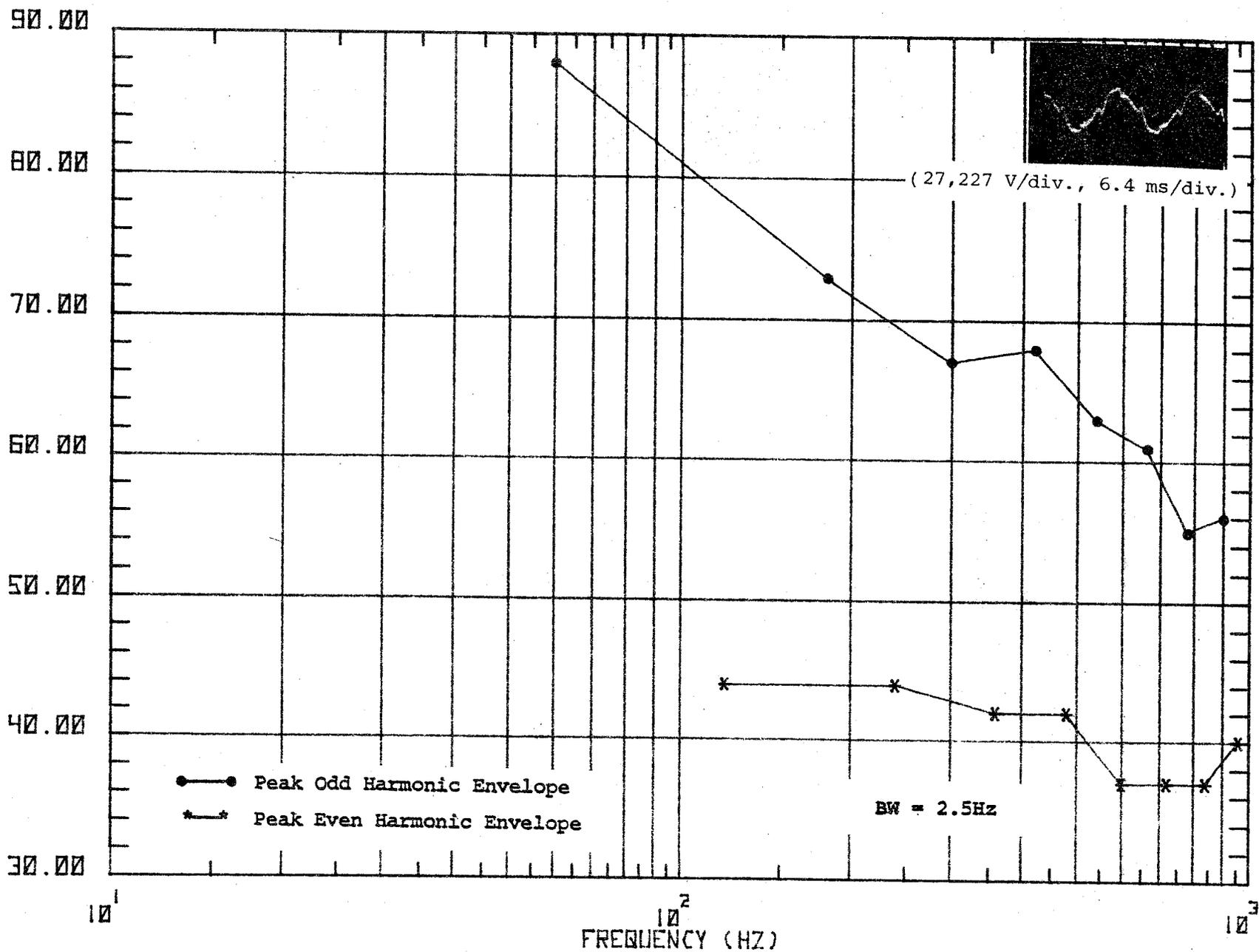
Figure 54d. Waveform and spectrum of catenary voltage sampled during 10-mph increment run, 40 to 50 mph.
