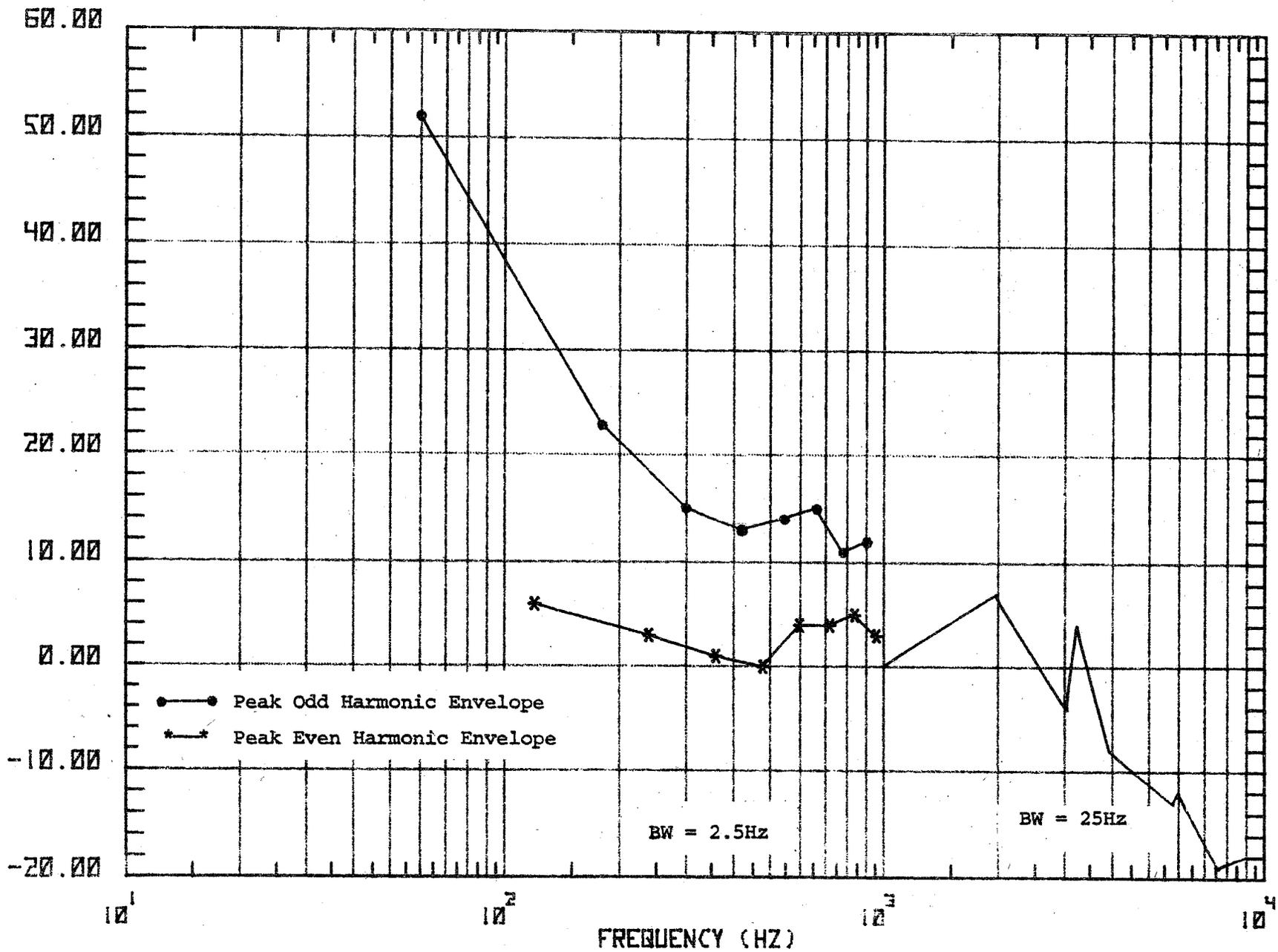
Figure 35. Spectrum of electric field strength sampled while locomotive was idling (locomotive on RTT).
