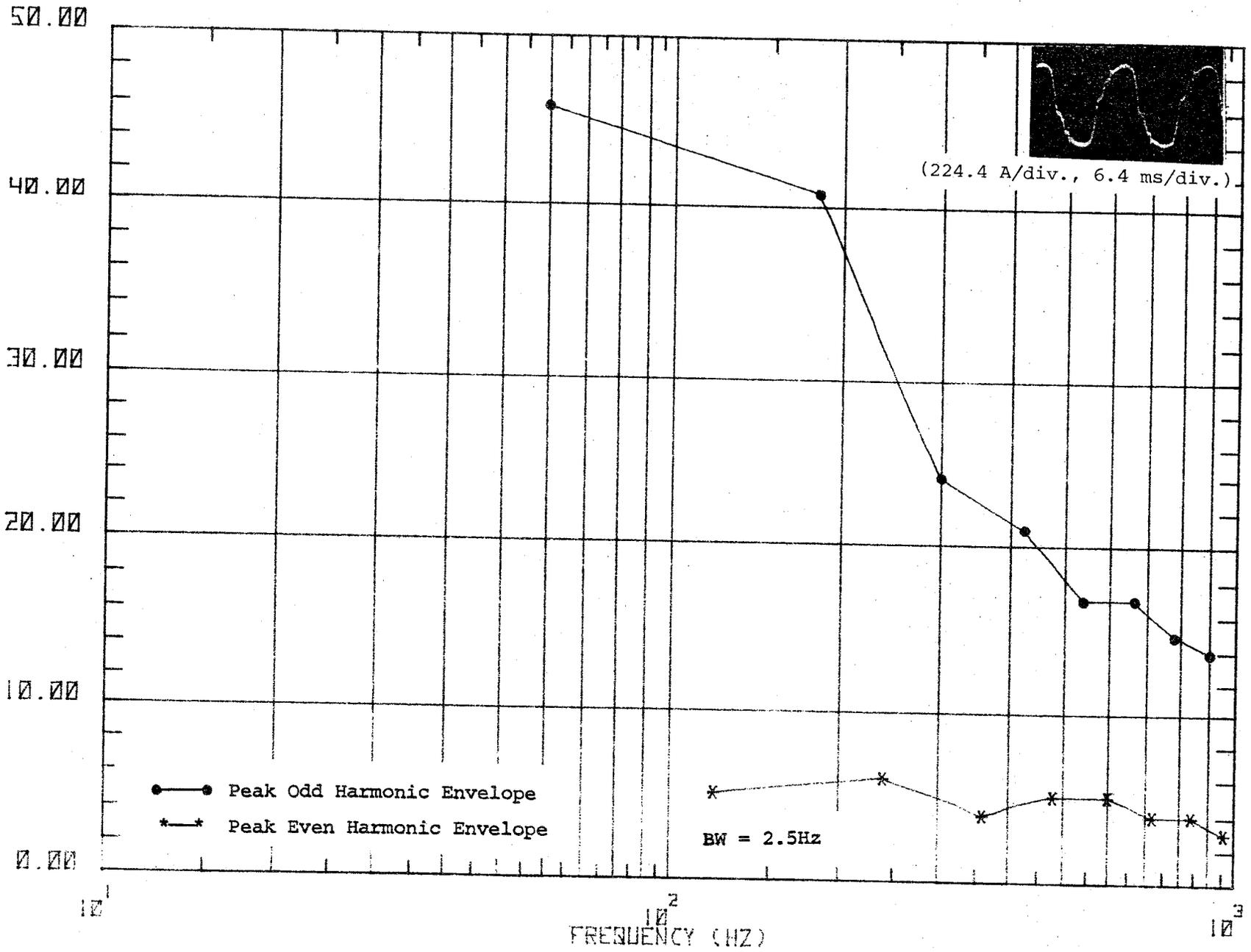
Figure 5ld. Waveform and spectrum of ground side primary current waveshape #4.
