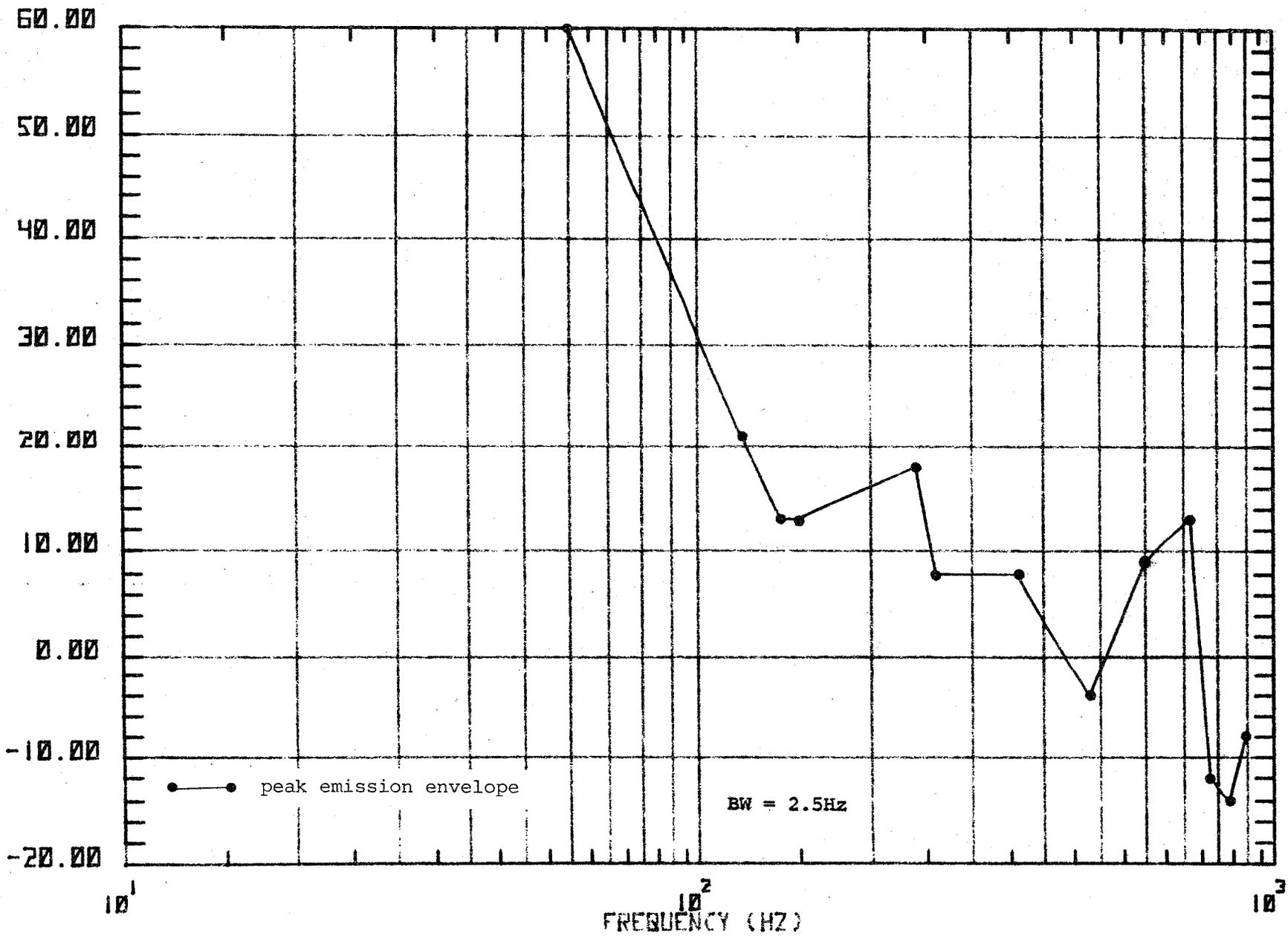
Figure 33. Spectrum of electric field strength, locomotive idling (sample 1).
