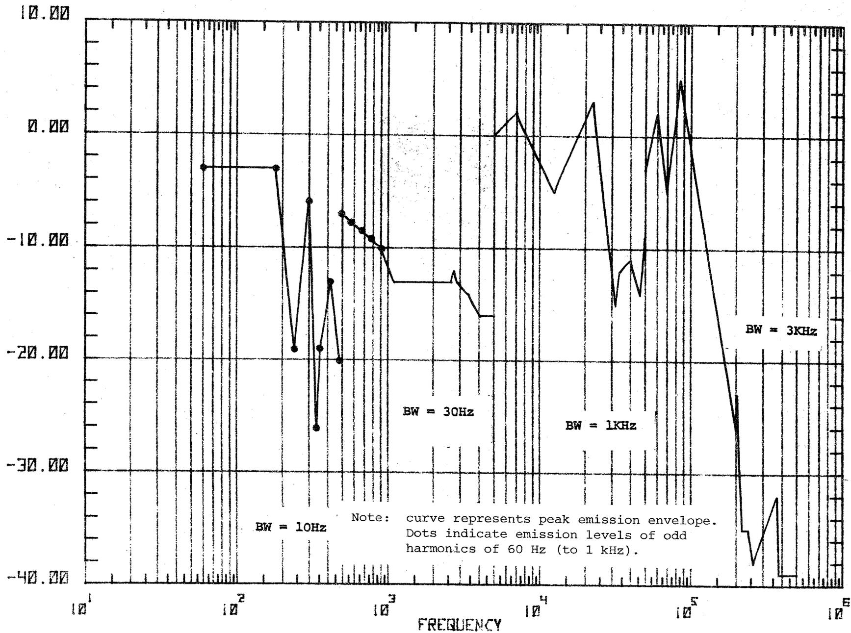
Figure 20. Spectrum of voltage across 74-volt bus (corresponding to Figure 19).
