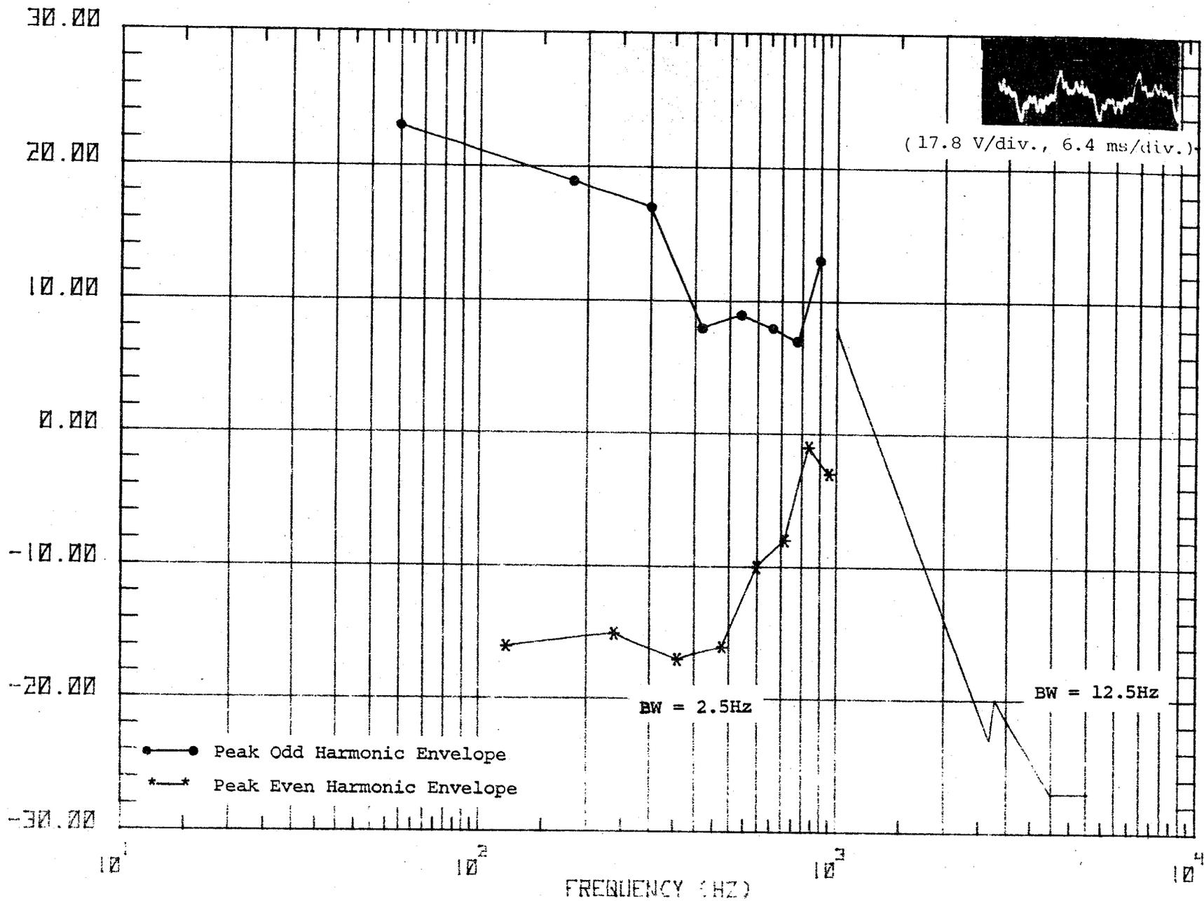
Figure 63c. Waveform and spectrum of cab signal voltage corresponding to ground side primary current waveshape #3.
