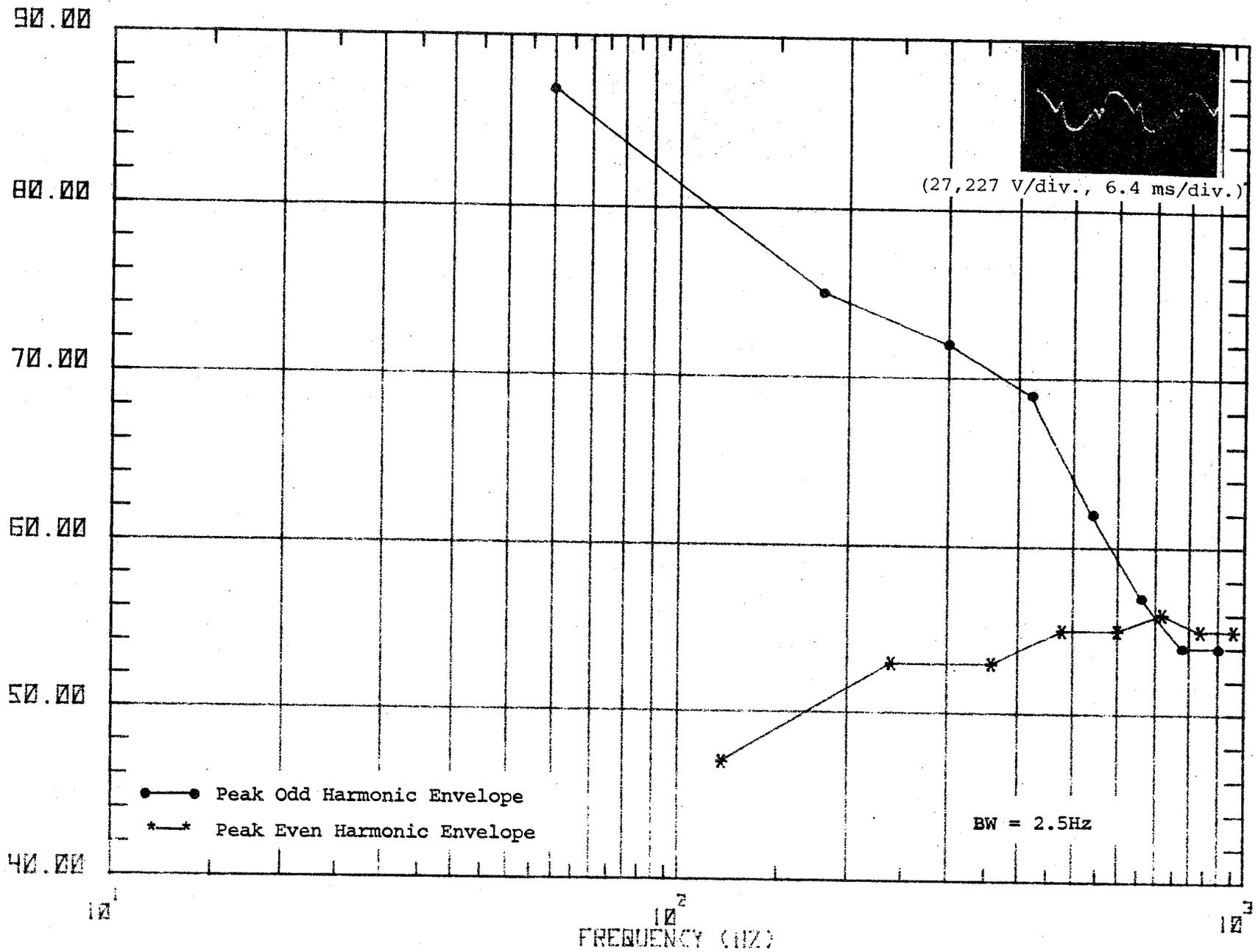
Figure 54j. Waveform and spectrum of catenary voltage sampled during 10-mph increment run, 100 to 110 mph.
