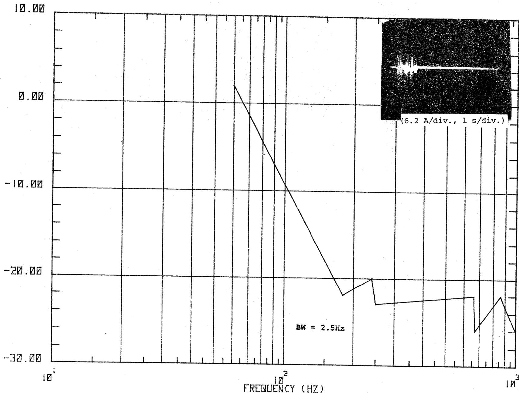
Figure 44. Waveform and spectrum of magnetic field strength recorded at third location, probe perpendicular to rails.
