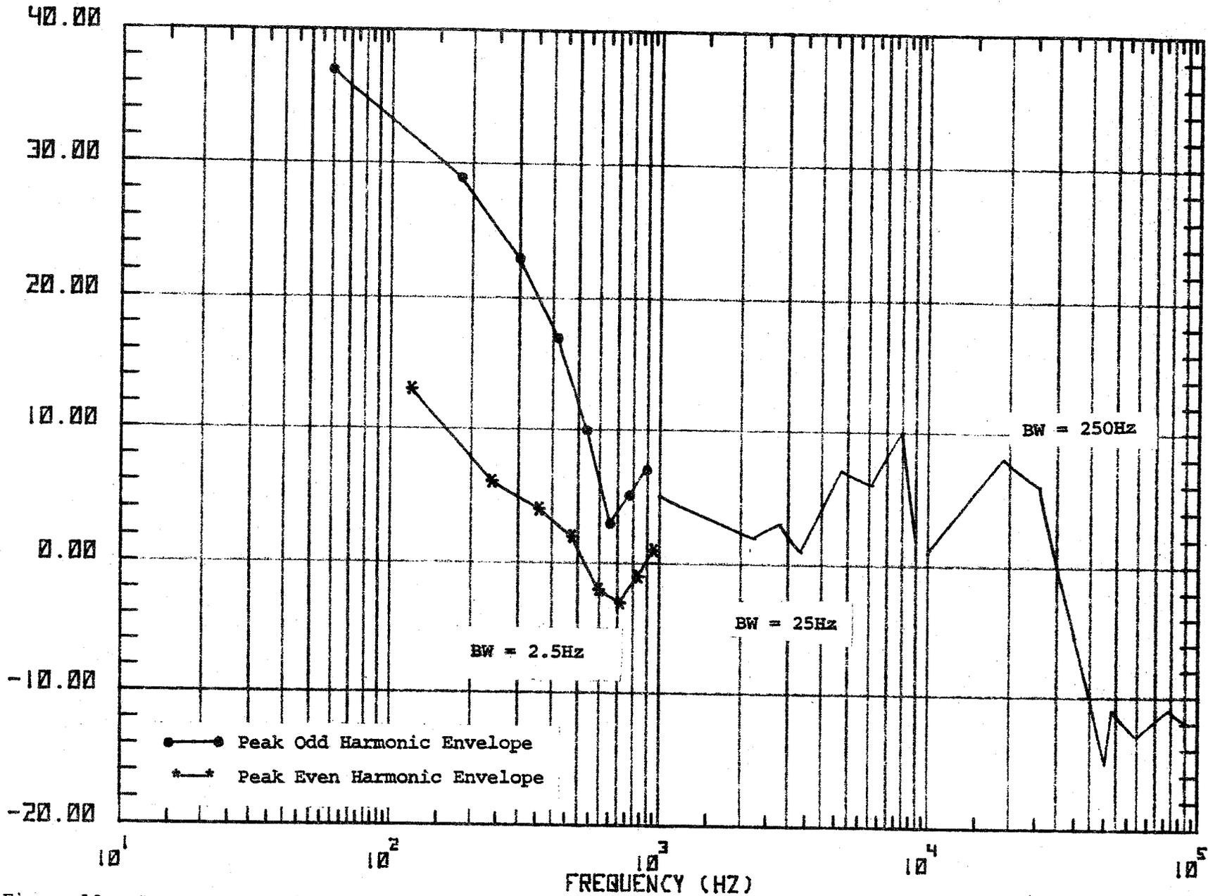
Figure 10. Spectrum of primary current sampled while locomotive was traveling at high speed.
