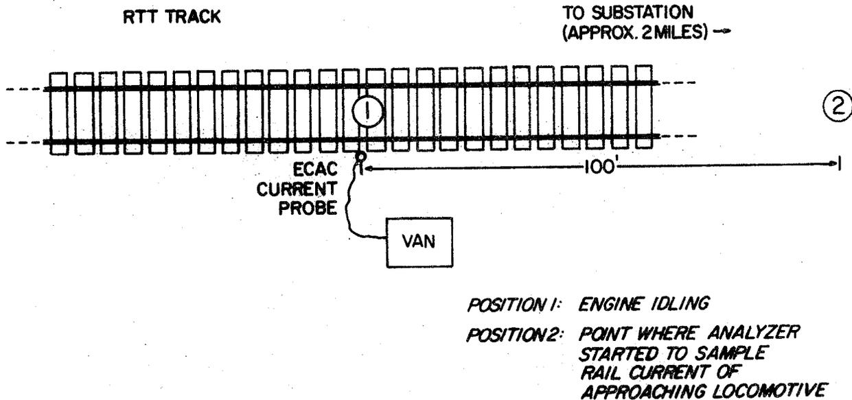
Figure 25. Rail current measurement location.
