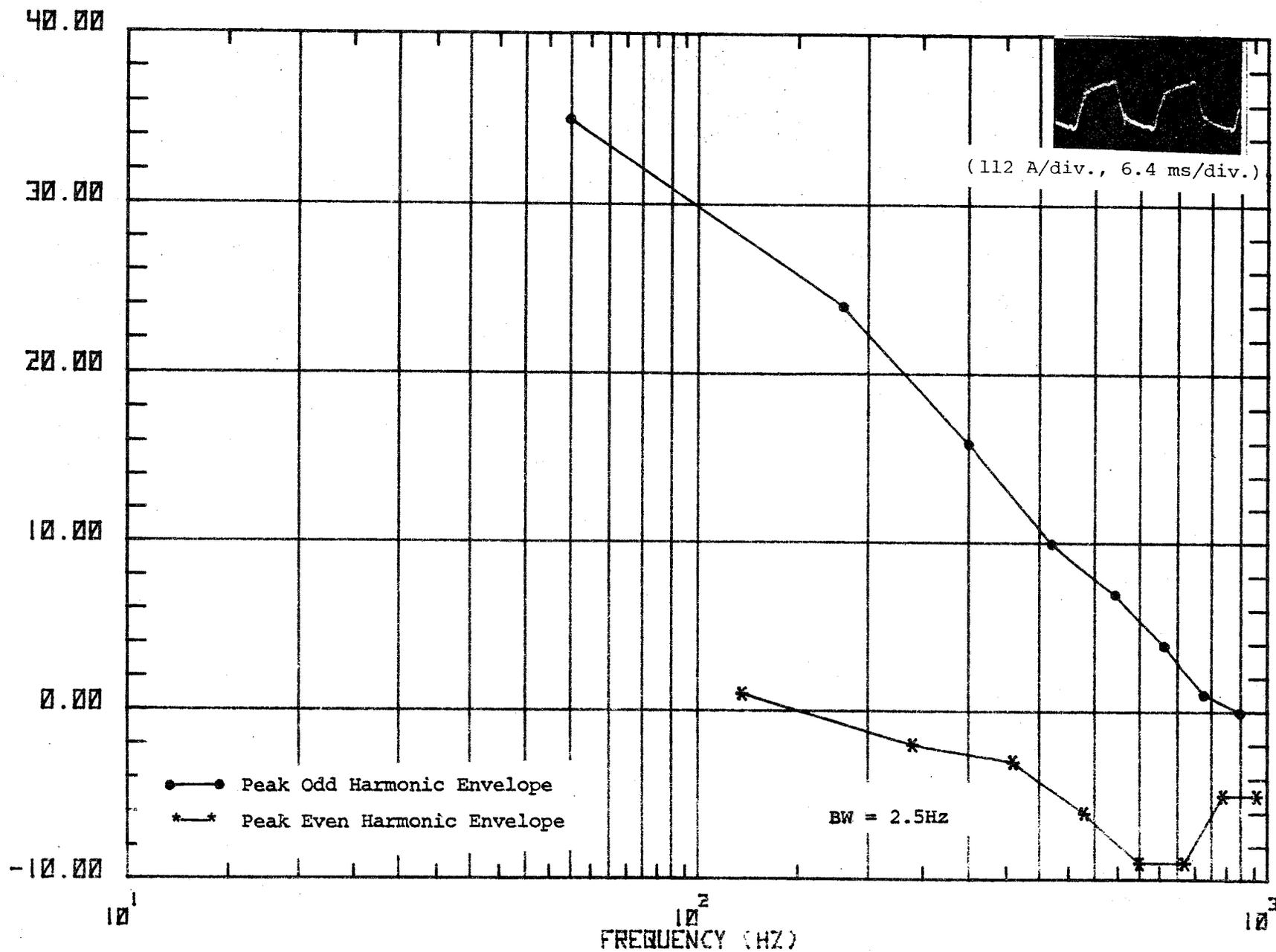
Figure 49c. Waveform and spectrum of primary current, locomotive accelerating from 30-40 mph.
