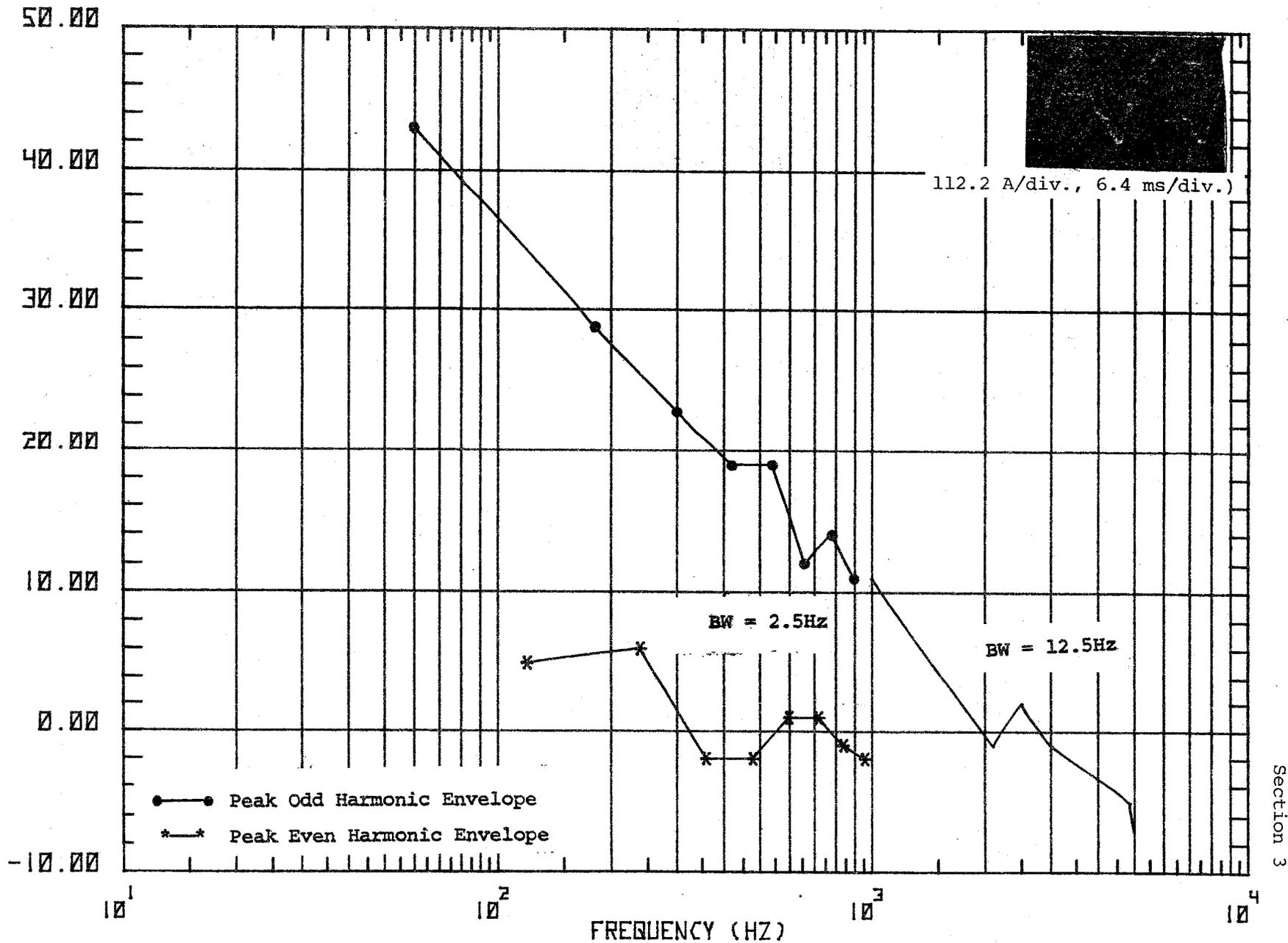
Figure 50d. Waveform and spectrum of primary current, locomotive accelerating from 30-40 mph (sample 2).
