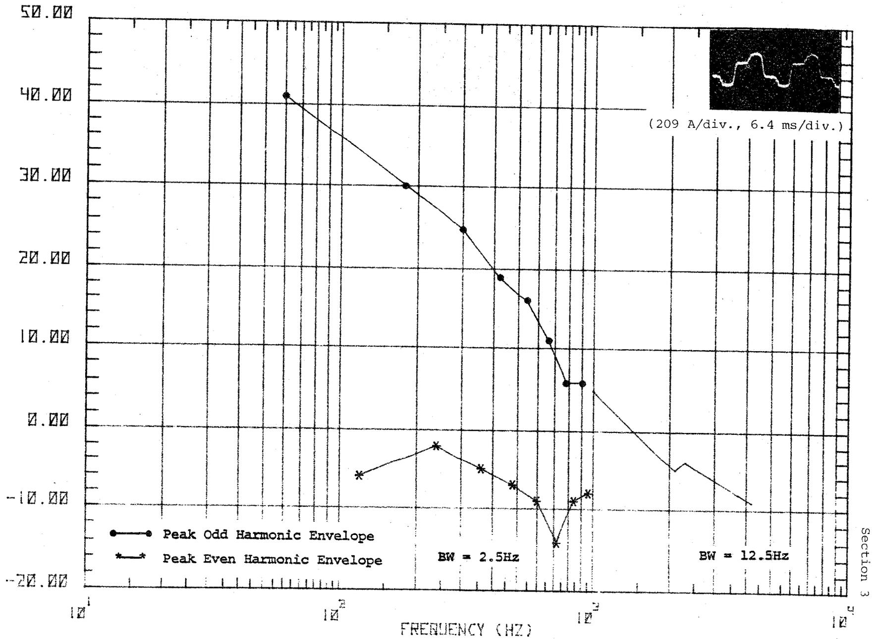
Figure 52e. Waveform and spectrum of primary current (sampled on the high side), locomotive accelerating from 40 to 50 mph.
