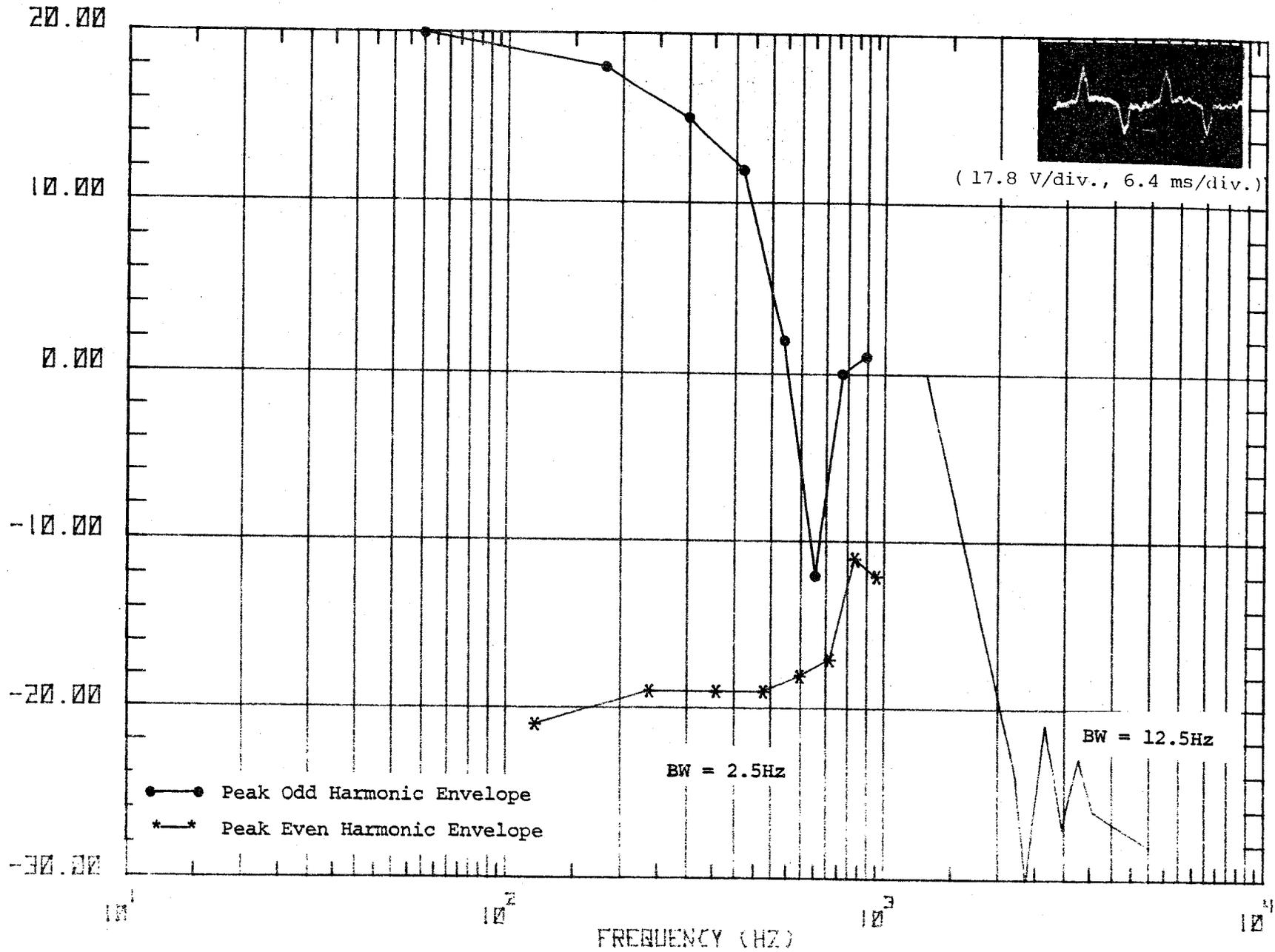
Figure 63f. Waveform and spectrum of cab signal voltage corresponding to ground side primary current waveshape #6.
