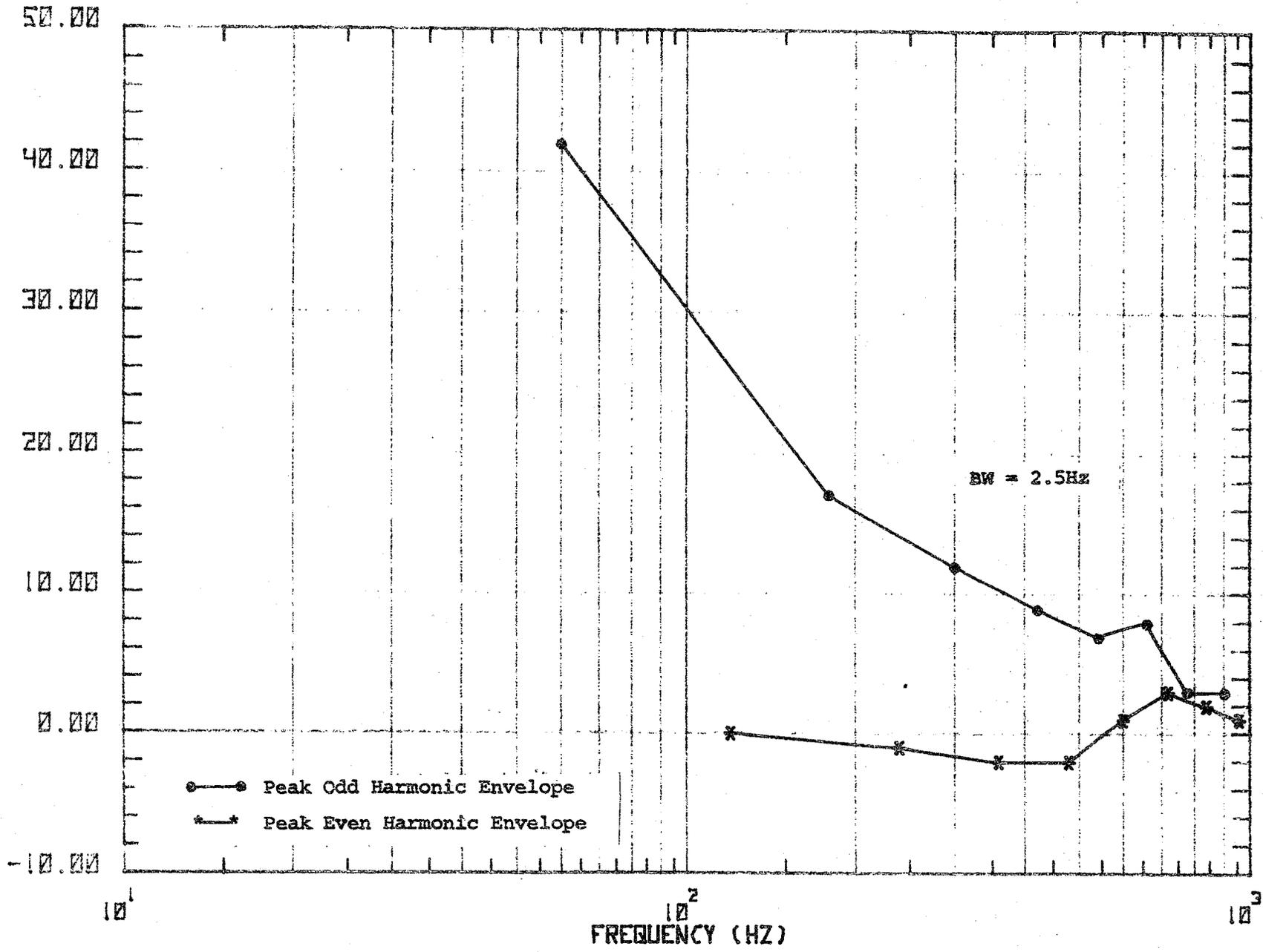
Figure 36. Spectrum of electric field strength sampled while locomotive coasted.
