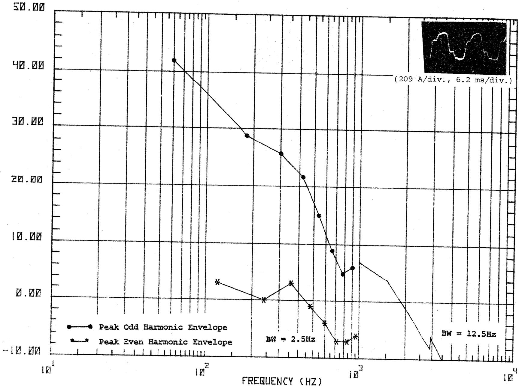
Figure 52f. Waveform and spectrum of primary current (sampled on the high side), locomotive accelerating from 50 to 60 mph.
