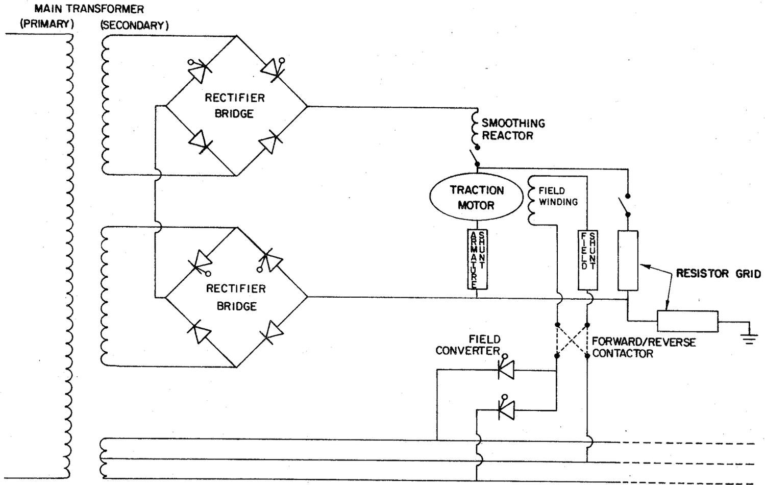
Figure 2. Simplified diagram of one traction motor circuit.
