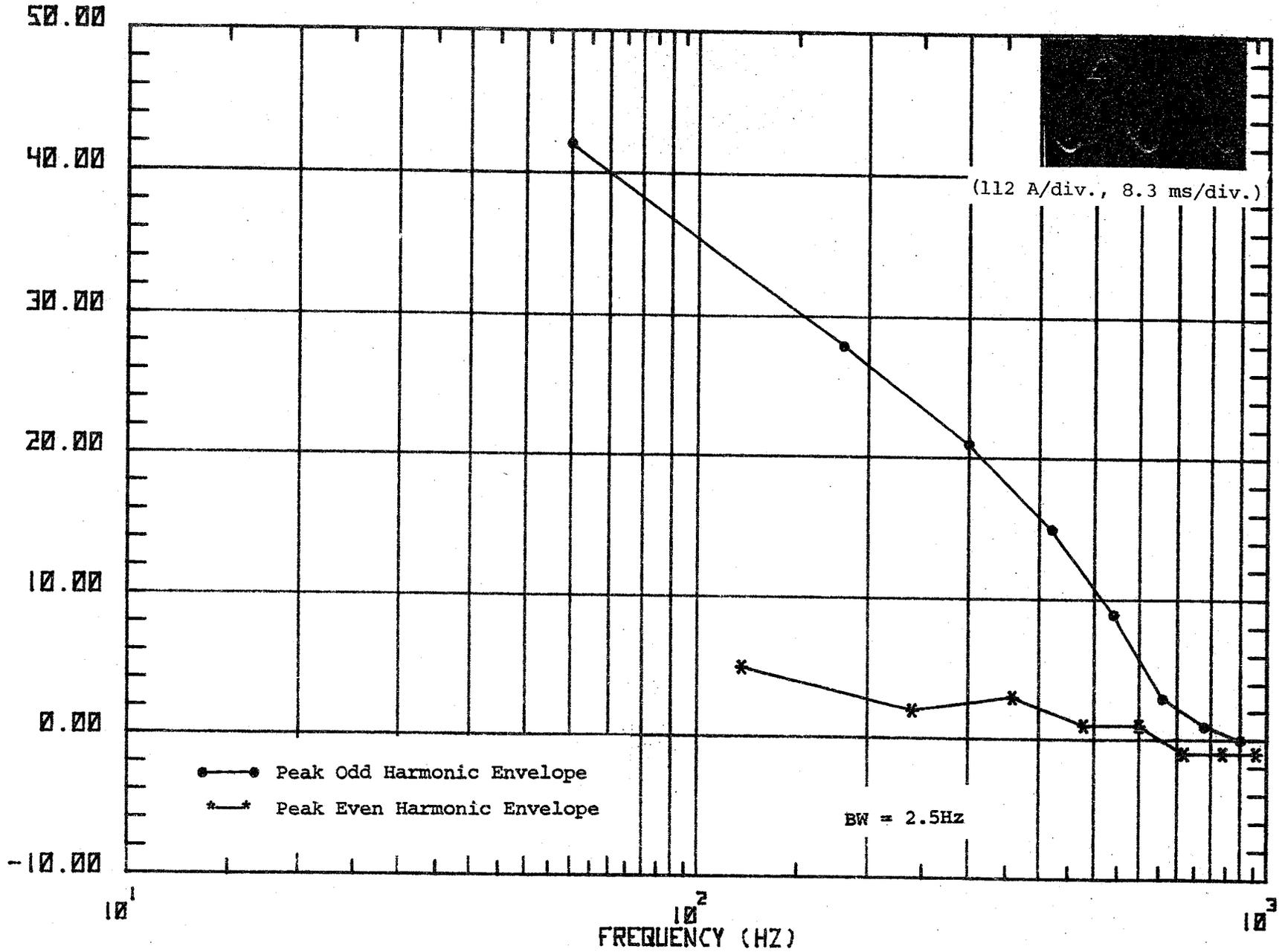
Figure 49j. Waveform and spectrum of primary current, locomotive accelerating from 100-110 mph.
