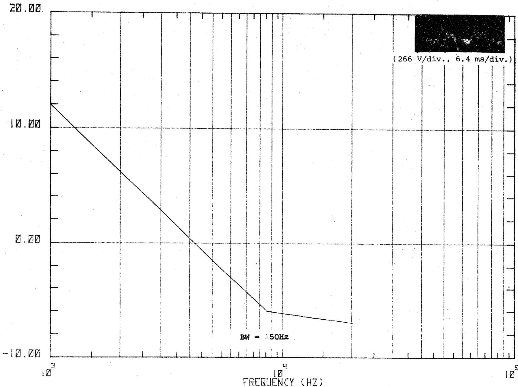
Figure 60. Waveform and spectrum of voltage across 74-volt bus recorded as locomotive accelerated from 0 mph (recorded on direct channel).
