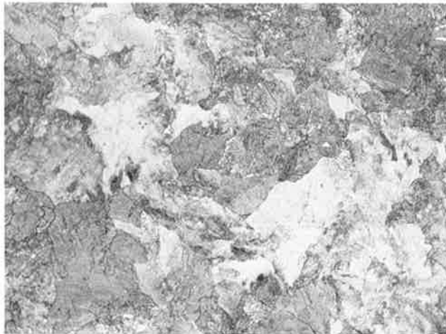
A. 1075 PLATE PEARLITIC MICROSTRUCTURE (500X)
