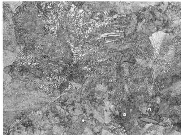
B. 112-LB RAIL MICROSTRUCTURE (500X)
