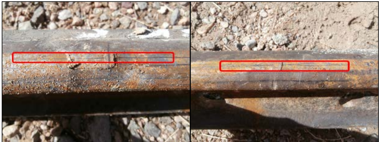
Figure 20. Post-Test Metal Flow for an Untreated (left) and a Post-Hardened (right) Joint Bar
