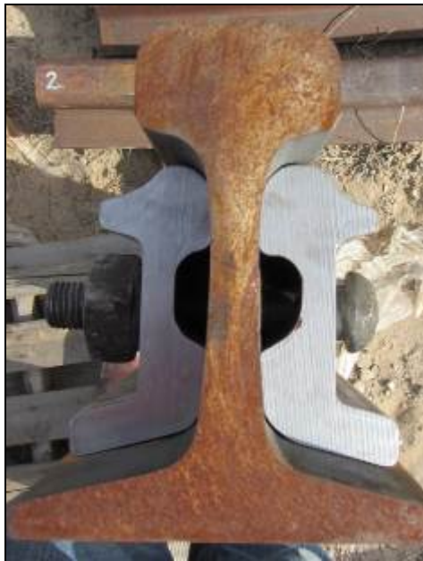
Figure 36. Example Prototype Joint Bar Design
