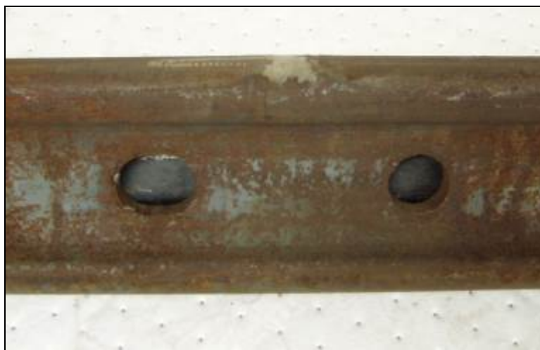
Figure 30. Area of Interest/Stress Concentration Location
