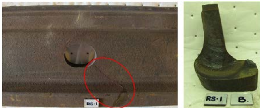
Figure 2. Joint Bar Bolt Hole Crack
