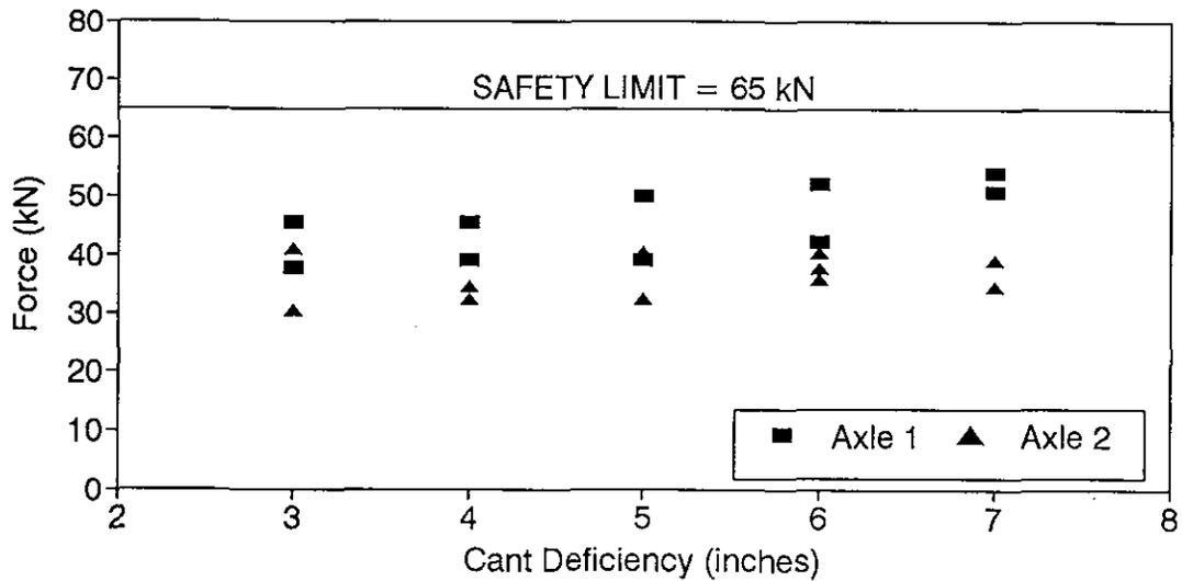
**Figure 5.2: Peak Net Axle Lateral Forces During Cant Deficiency Runs**
