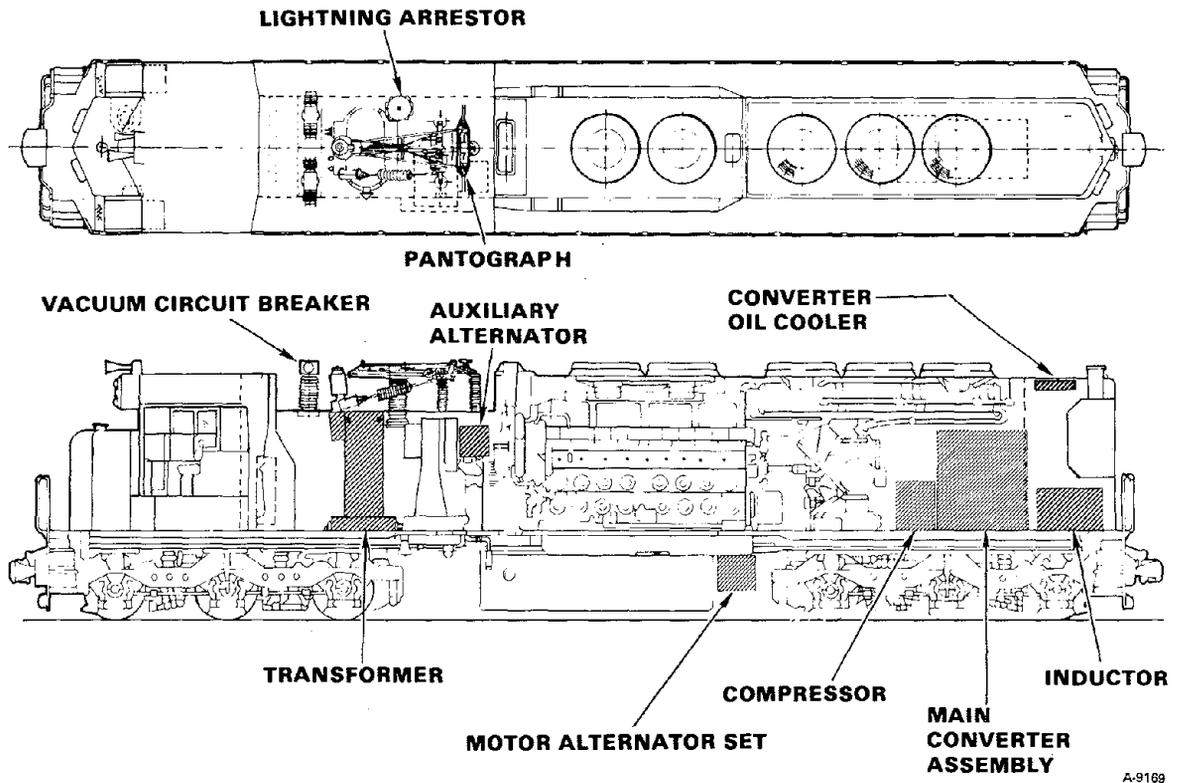
Figure 3. 50-kv DML, Equipment Layout
