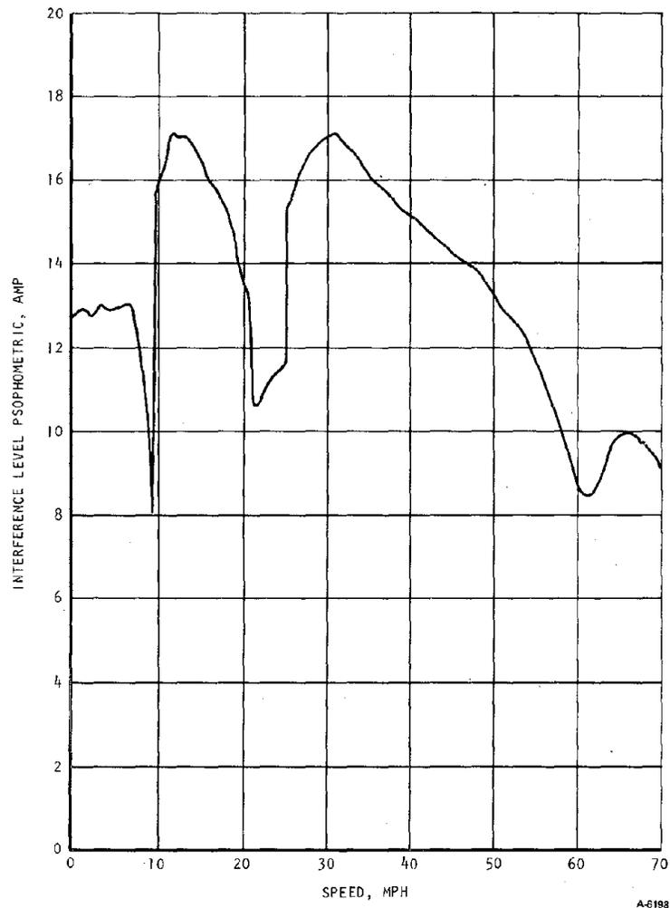
Figure 8. Variation of Psophometric Current with Speed
