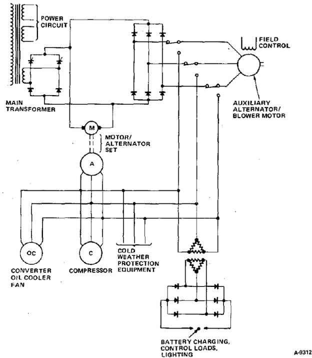
Figure 9. DML Auxiliaries Scheme
