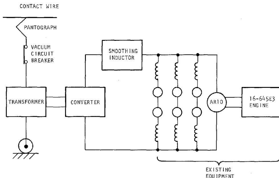
Figure 2. Simplified DML System Diagram
