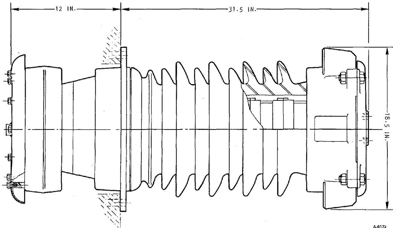
Figure 14. Typical Lightning Arrester
