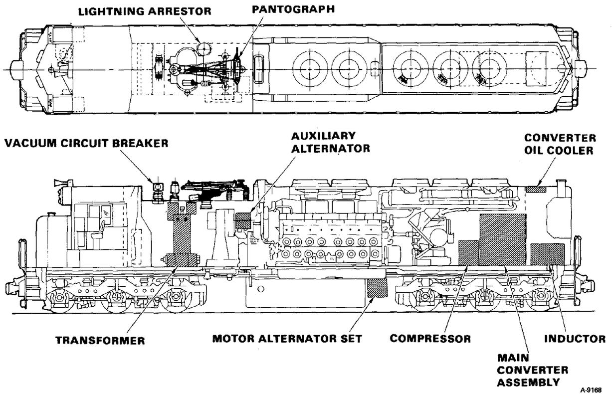
Figure 4. 25-kv DML, Equipment Layout
