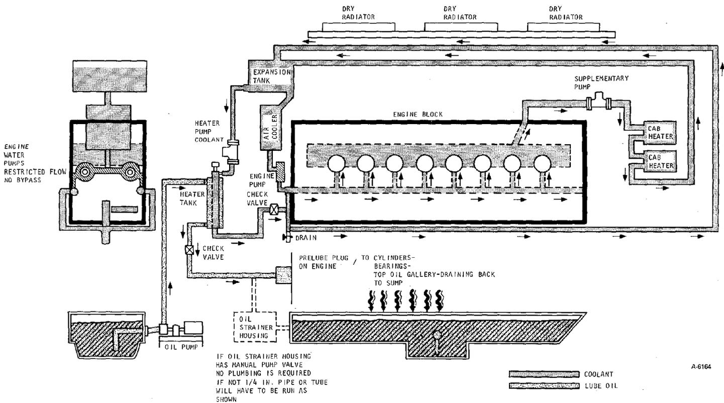
Figure 17. Typical Kim Hotstart Two-Fluid System
