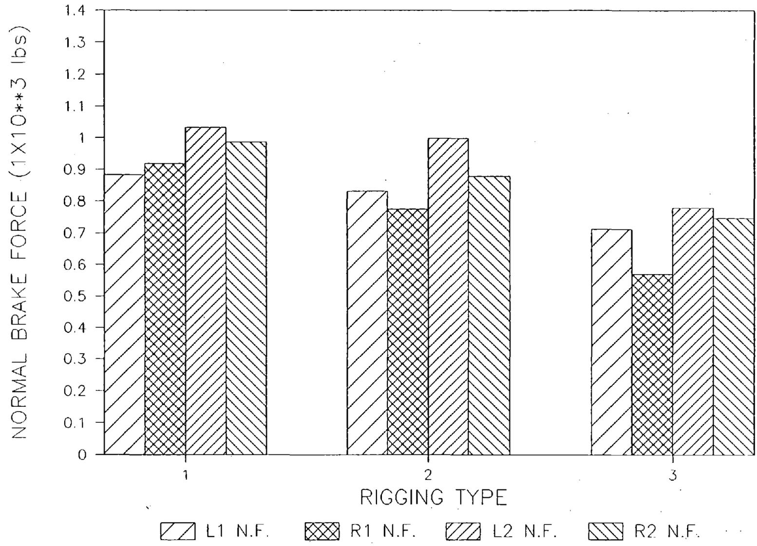
B-END TRUCK NORMAL FORCES FOR 20 MPH, 50 PSI TEST CONDITIONS
