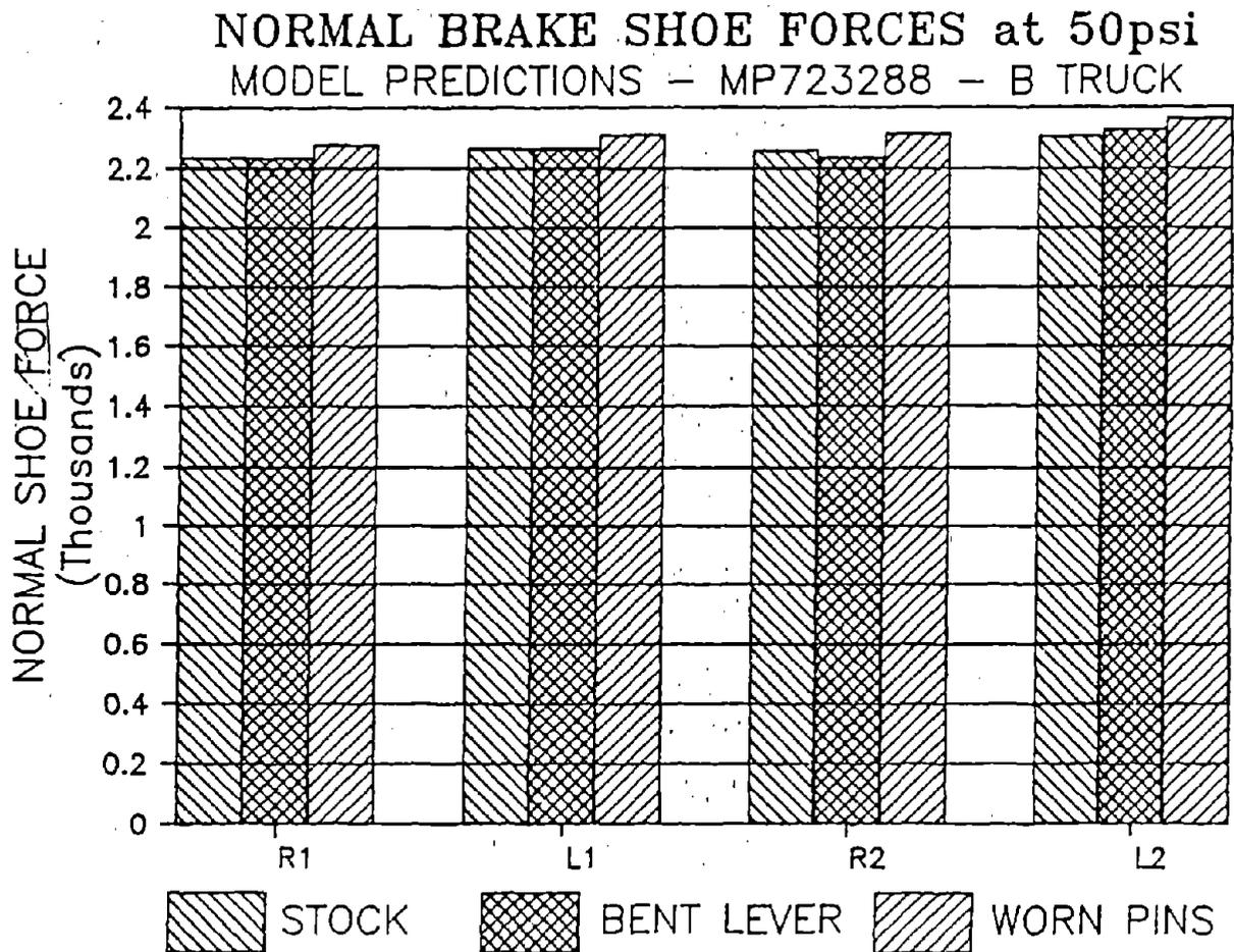
**Figure 8. Comparison of Brake Force Normal Forces, Stock Condition, Bent Live Lever, Worn Pins, Worn Live and Dead Levers**
