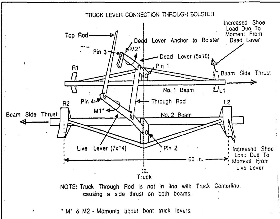
Figure 11. Truck Lever And Brake Beam Arrangement
