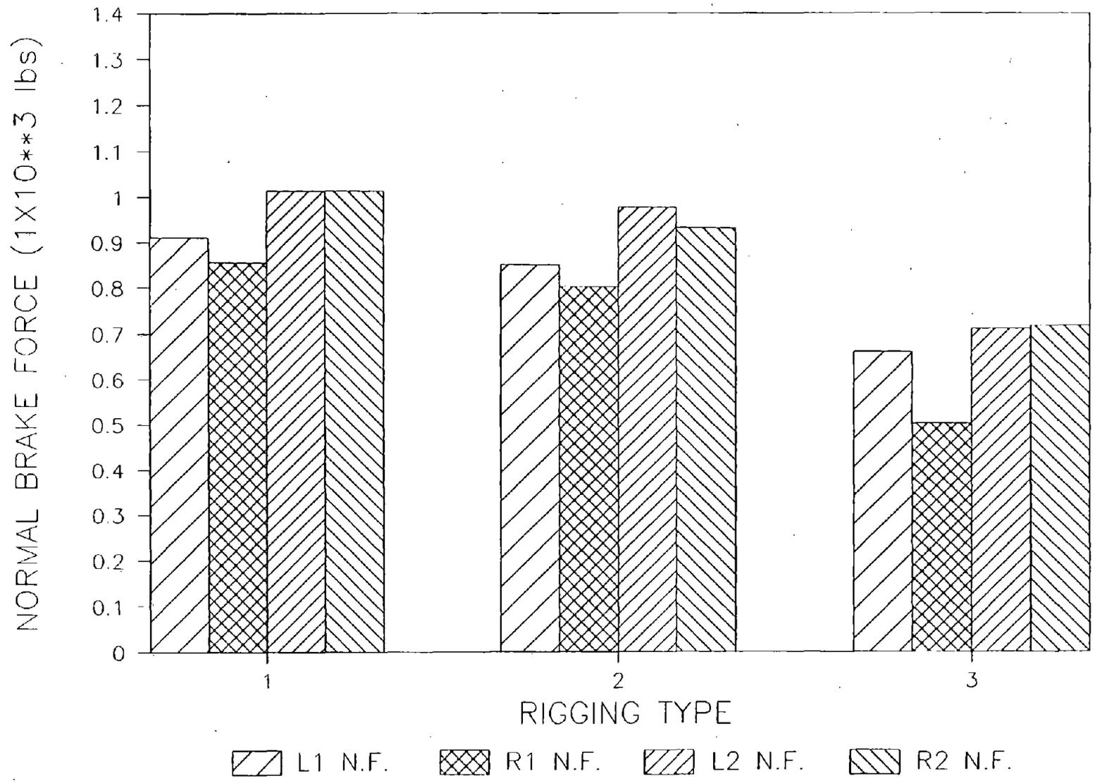
B-END TRUCK NORMAL FORCES FOR 50 MPH, 25 PSI TEST CONDITIONS
