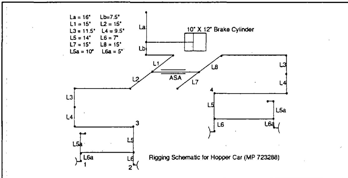
Figure 10. Brake Rigging Dimensions
