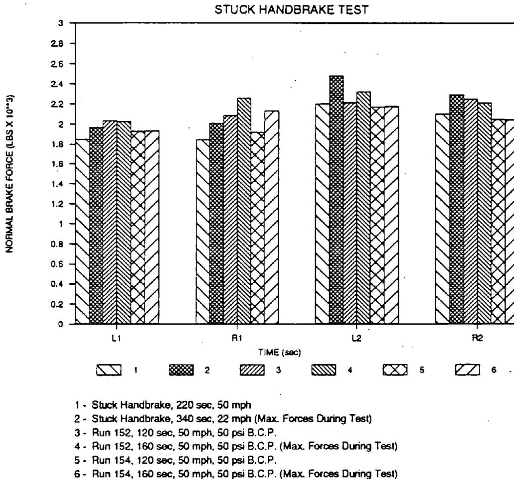
**Figure 48. Handbrake Forces vs Drag Braking Forces For Runs 152 and 154**
