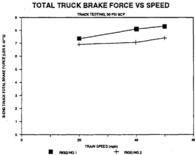
**Figure 45. B-end Truck Total Normal Brake Force Measured After 120 Seconds**
