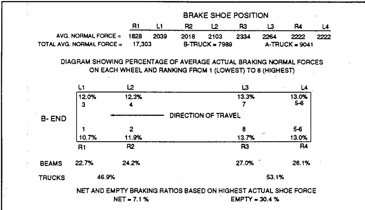
**Figure 2. Distribution Of Brake Forces For B-End Leading**
