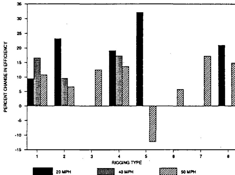
**Figure 32. Percent Change In Efficiency Between 25- and 50-psi BCP**
