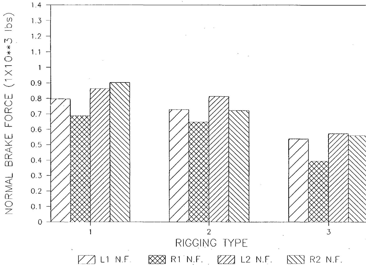
B-END TRUCK NORMAL FORCES. FOR 40 MPH, 25 PSI TEST CONDITIONS
