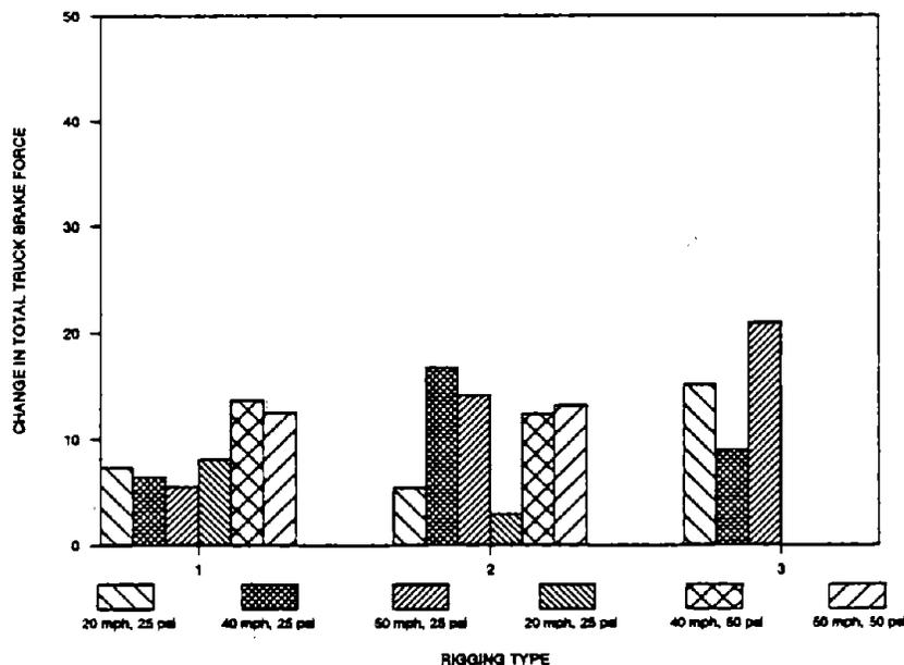
**Figure 46. Change in Total Brake Force Measured Between 40 and 120 Seconds, Track Testing**
