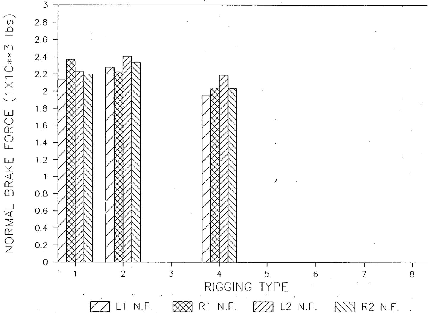
B-END TRUCK PIN AND NORMAL FORCES FOR 20 MPH, 25 PSI TEST CONDITIONS
