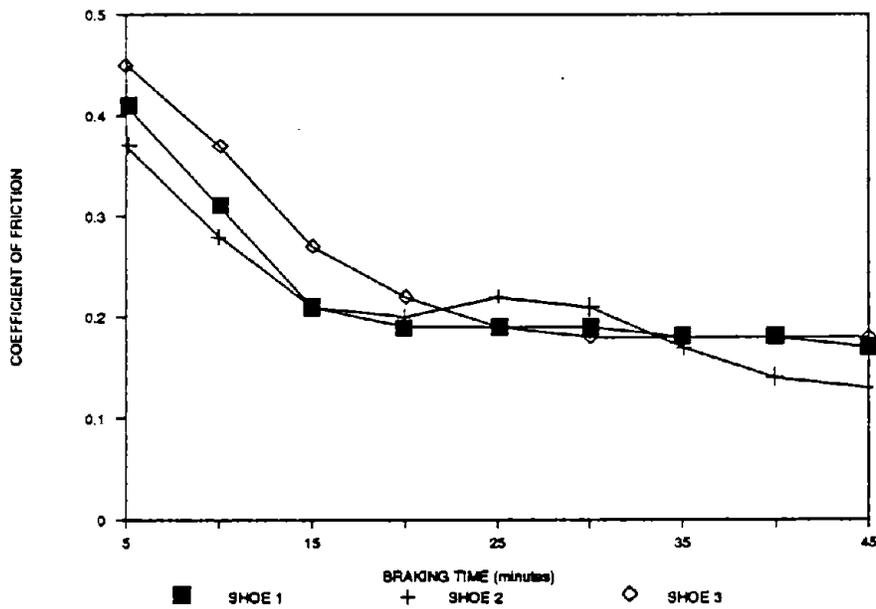
Figure 50. Brake Shoe Coefficient Of Friction vs Time, Brand B Shoes
