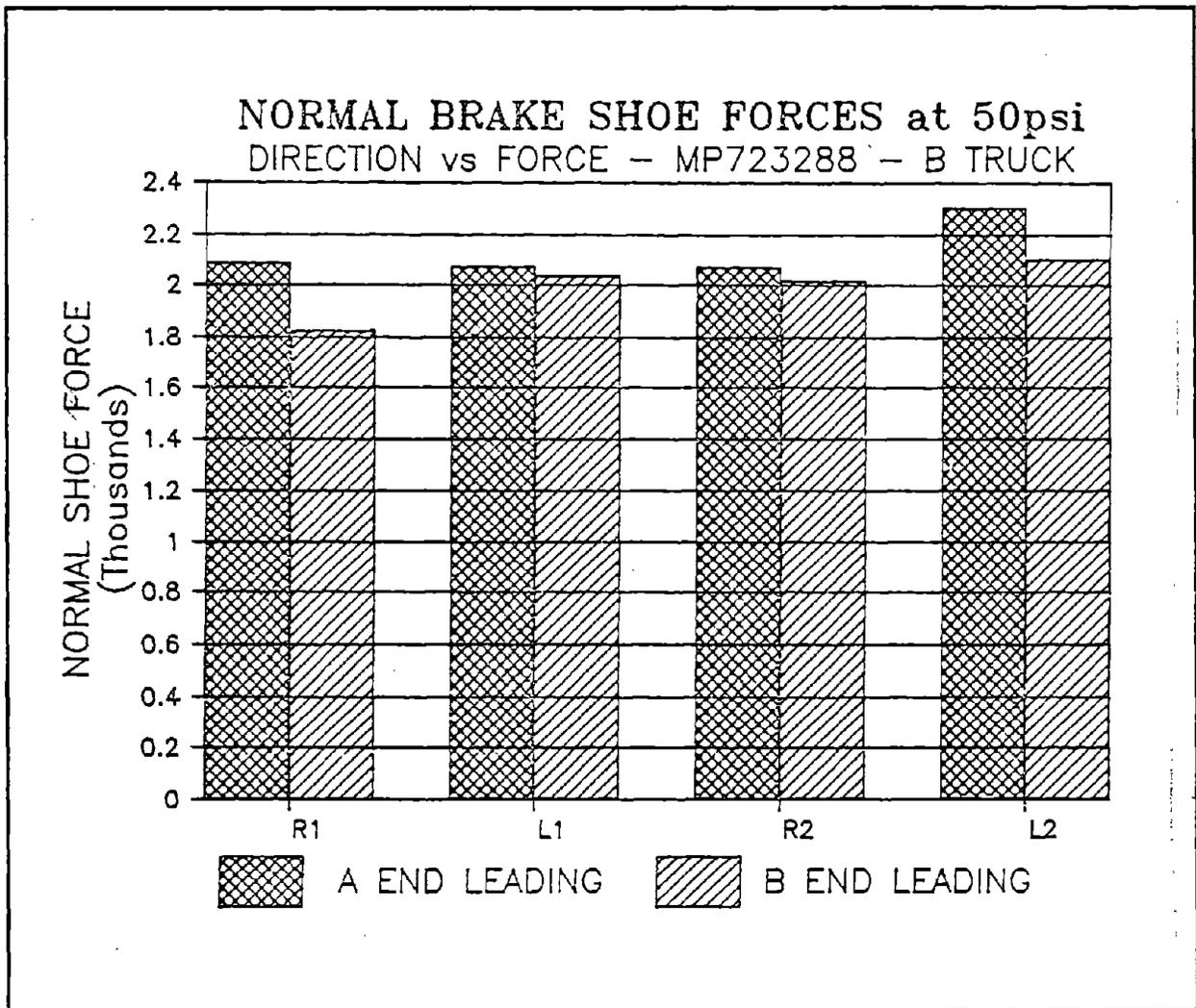
Figure 1. Average Brake Shoe Forces Measured During Previous Tests
