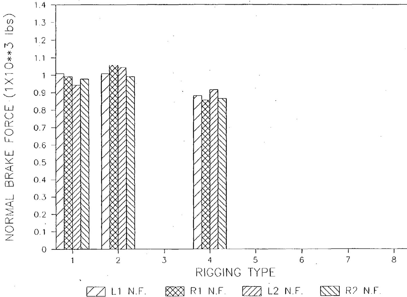
B-END TRUCK NORMAL FORCES FOR 50 MPH, 25 PSI TEST CONDITIONS
