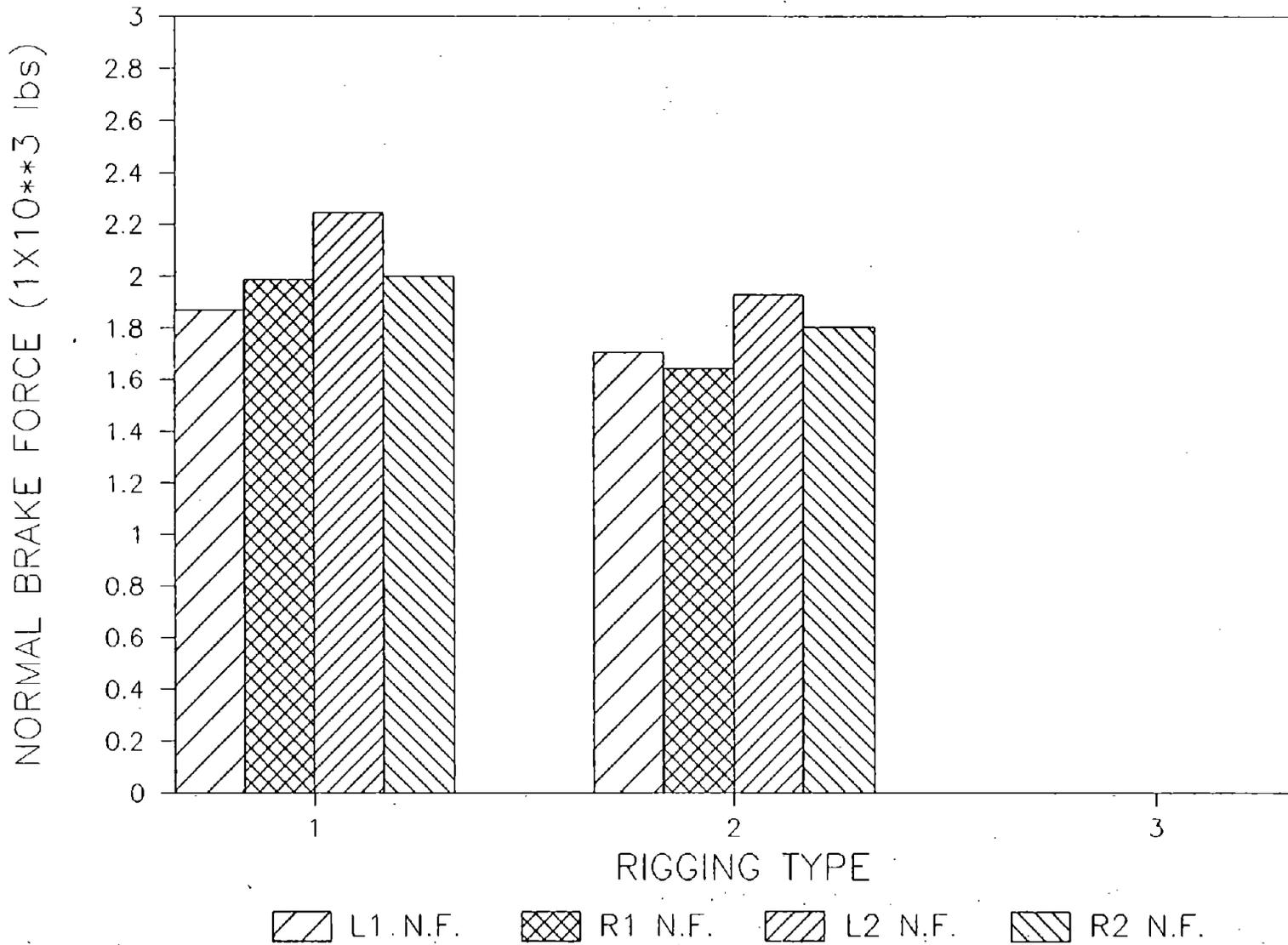
B-END TRUCK NORMAL FORCES FOR 50 MPH, 50 PSI TEST CONDITIONS
