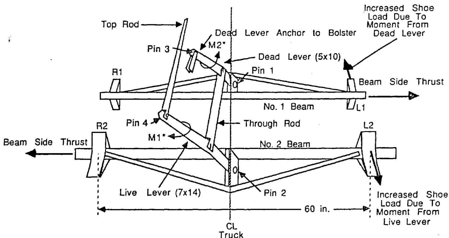
NOTE: Truck Through Rod is not in line with Truck Centerline, causing a side thrust on both beams.
