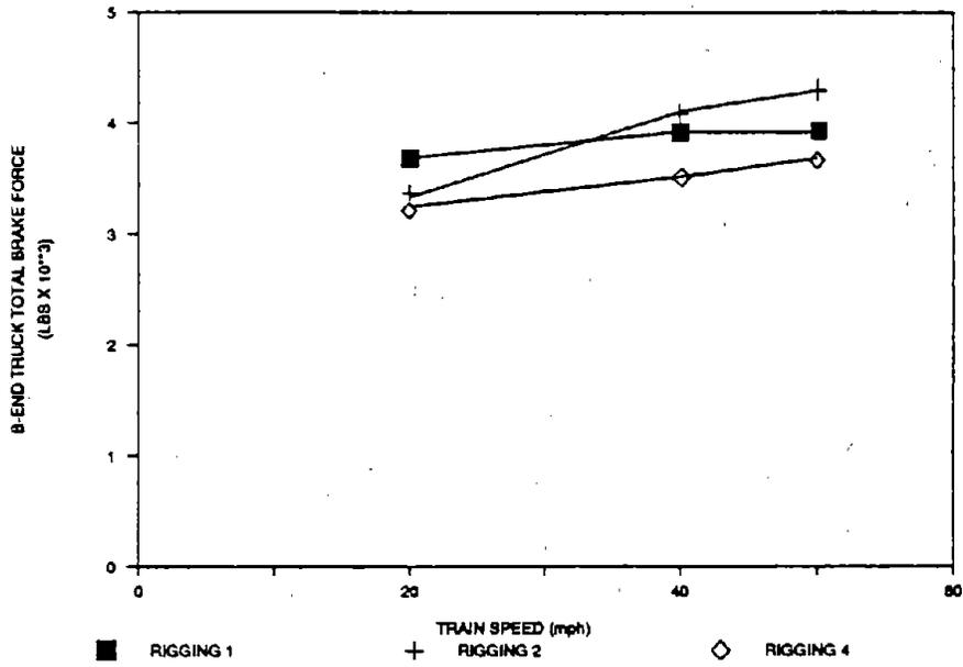
**Figure 21. B-end Truck Total Normal Brake Force vs Running Speed 25-psi BCP, Testing on RDU**
