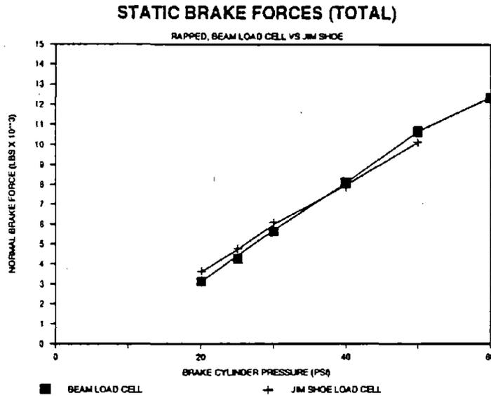
**Figure 38. Rapped B-end Truck Brake Forces Measured with Instrumented Brake Heads and Static Load Cells**
