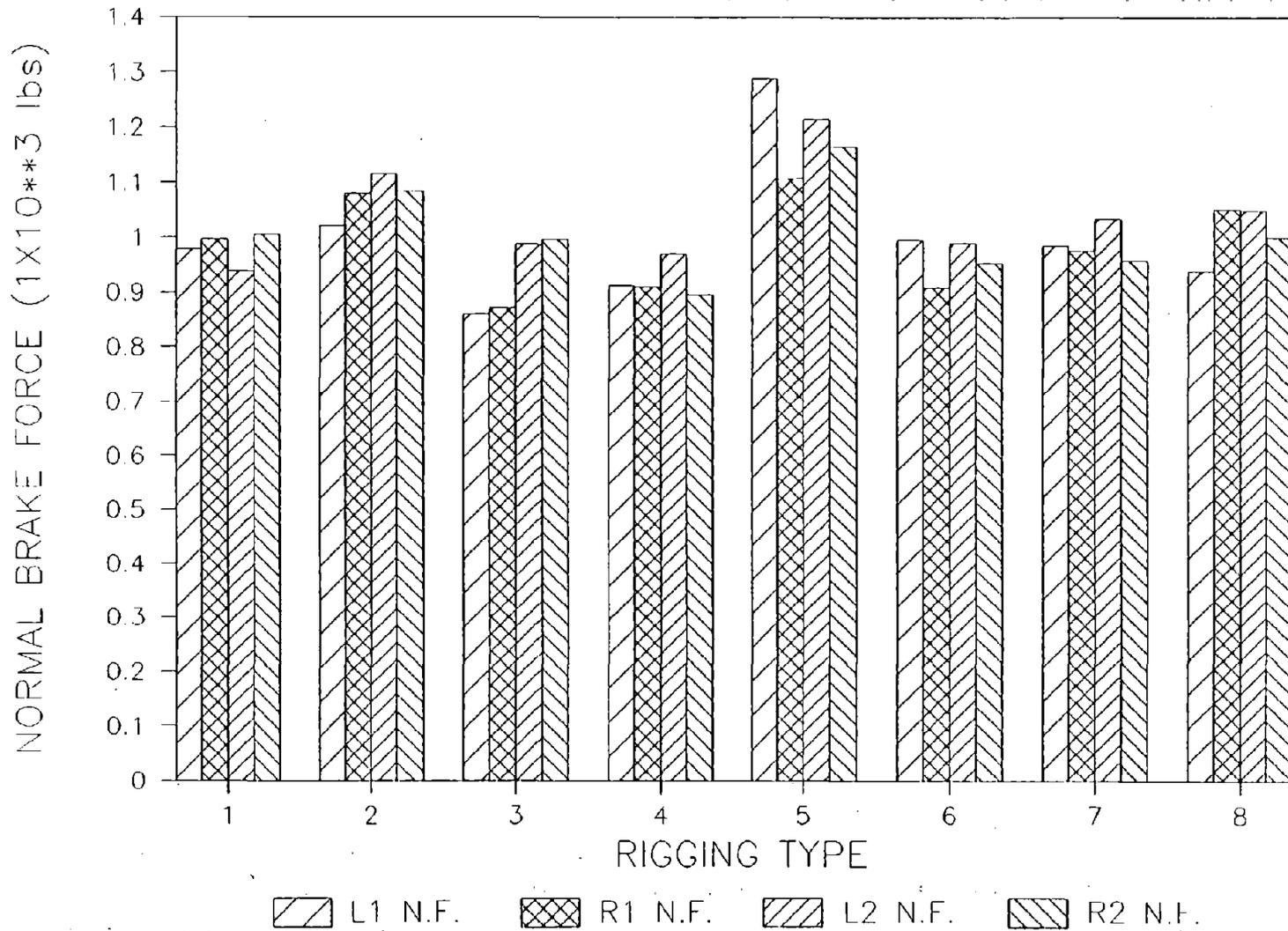
B-END TRUCK NORMAL FORCES FOR 20 MPH, 50 PSI TEST CONDITIONS
