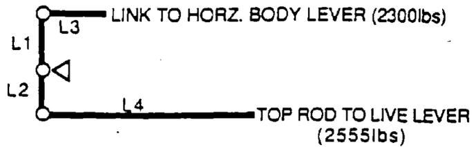
30 DEGREE ANGULARITY OF VERTICAL BODY LEVER.
