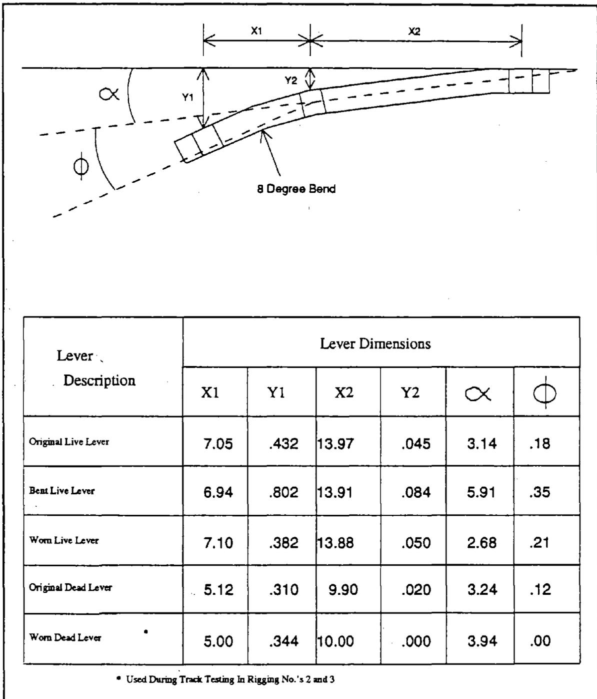
**Figure 18. Rigging Lever Dimensions -- Continued**
