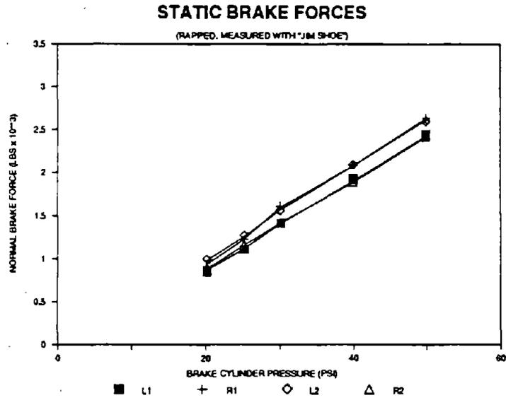
**Figure 36. Rapped Brake Forces Measured with Static Load Cells**
