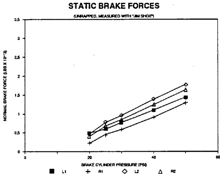
**Figure 35. Unrapped Brake Forces Measured with Static Load Cells**
