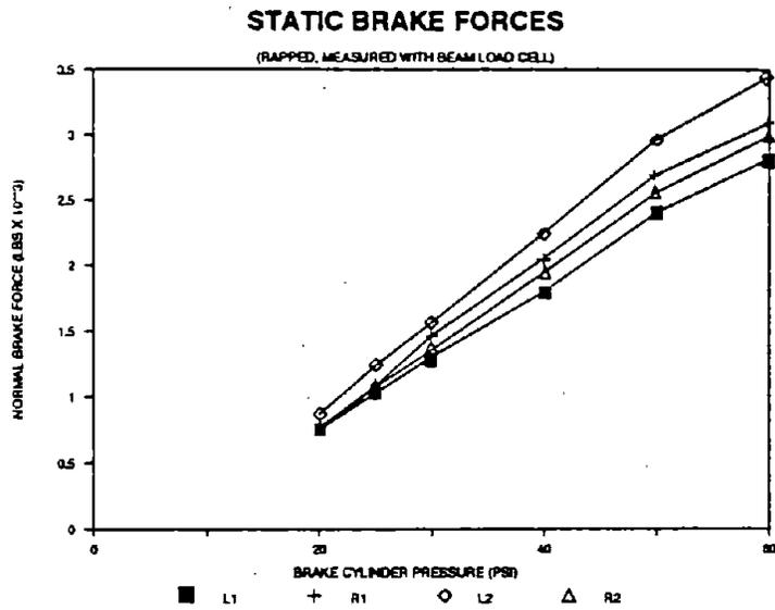
**Figure 34. Rapped Brake Forces Measured with Instrumented Brake Heads**
