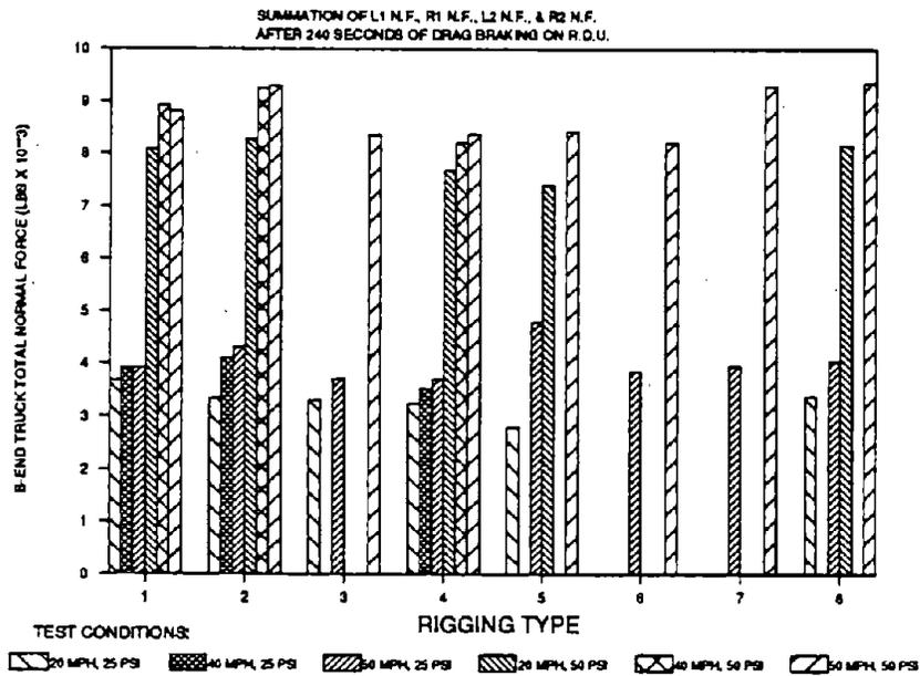
**Figure 20. B-end Truck Total Normal Brake Force Measured After 240 Seconds**
