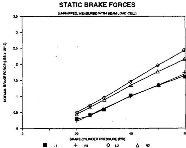
**Figure 33. Unrapped Brake Forces
