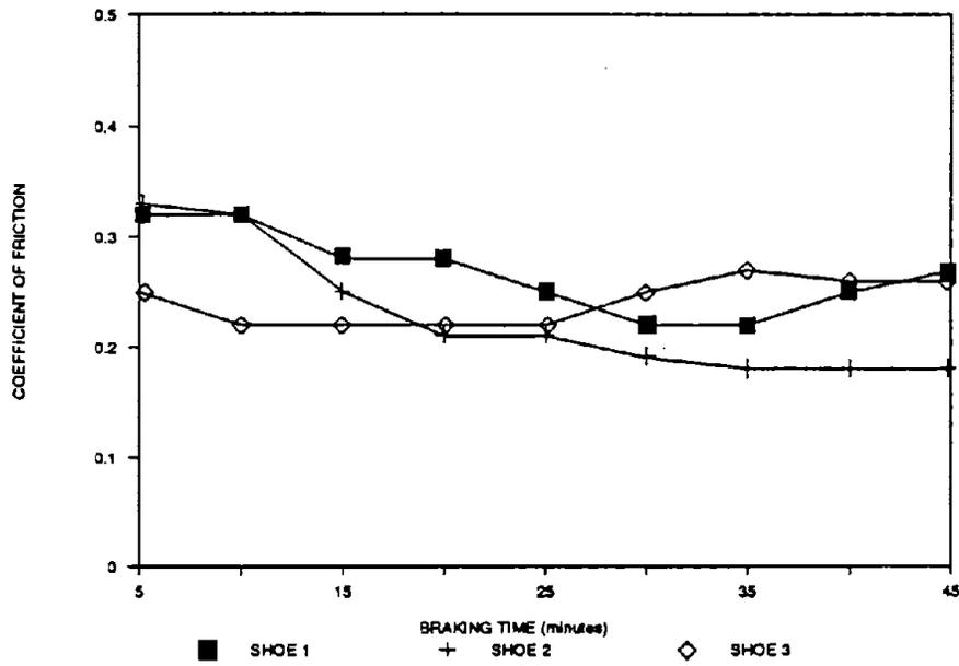
Figure 49. Brake Shoe Coefficient Of Friction vs Time, Brand A Shoes
