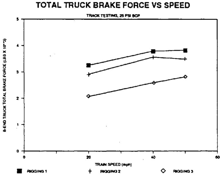
**Figure 44. B-end Truck Total Normal Brake Force Measured After 120 Seconds**
