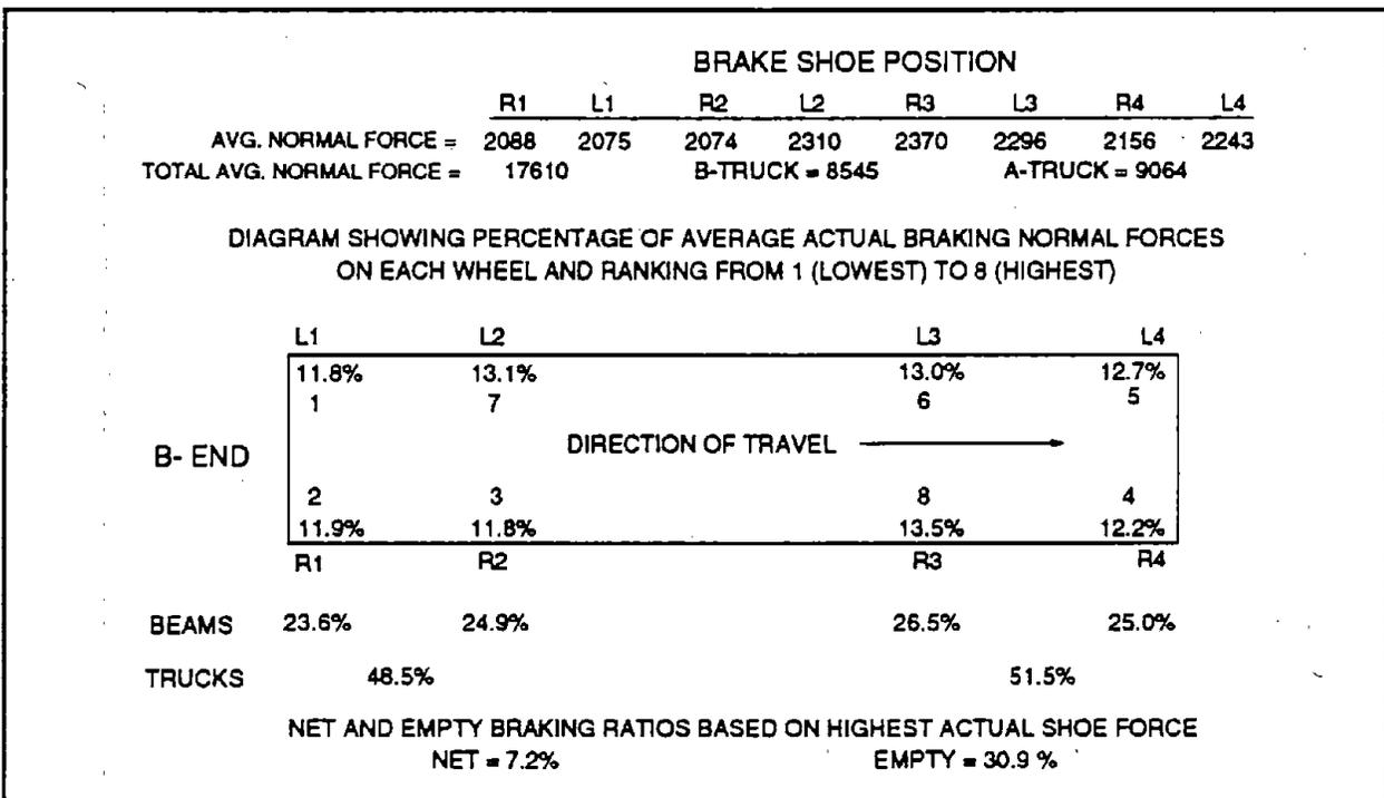
**Figure 3. Distribution Of Brake Forces For A-End Leading**
