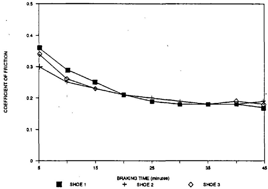
**Figure 51. Brake Shoe Coefficient Of Friction vs Time, Brand C Shoes**
