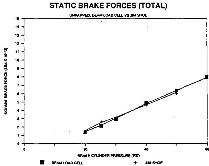
**Figure 37. Unrapped B-end Truck Brake Force Measured with Instrumented Brake Heads and Static Load Cells**
