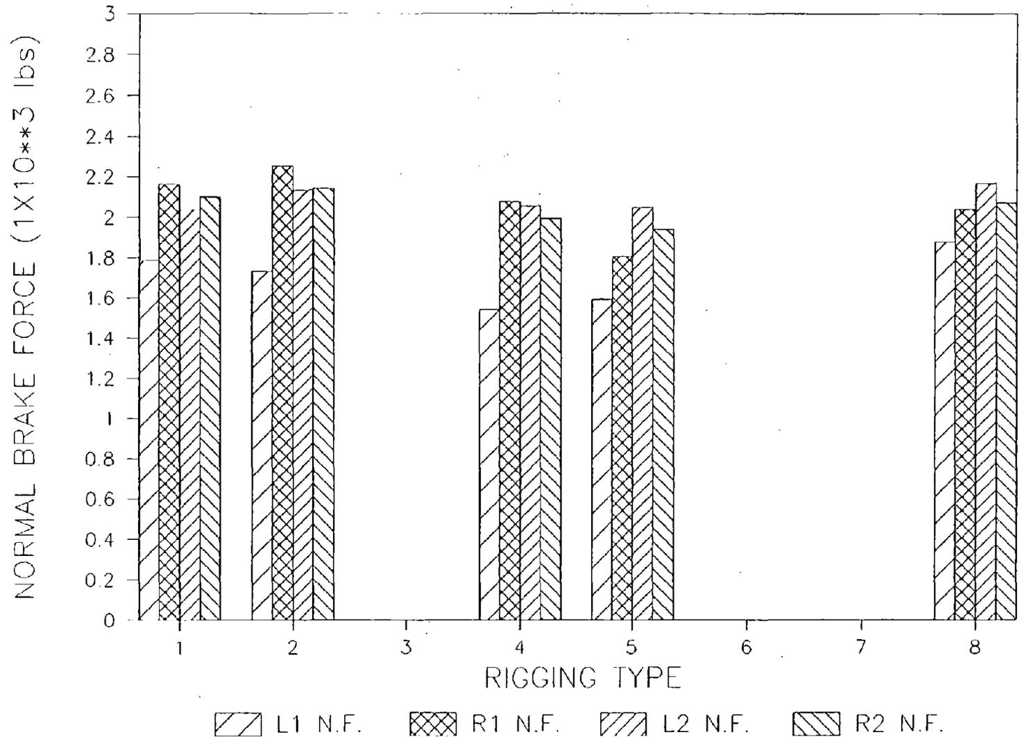
B-END TRUCK NORMAL FORCES FOR 40 MPH, 50 PSI TEST CONDITIONS
