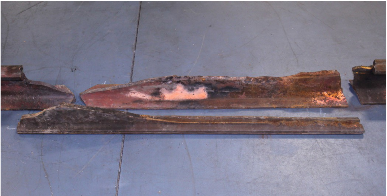
Figure 2: Photograph of the broken rail sections laid out end-to-end
