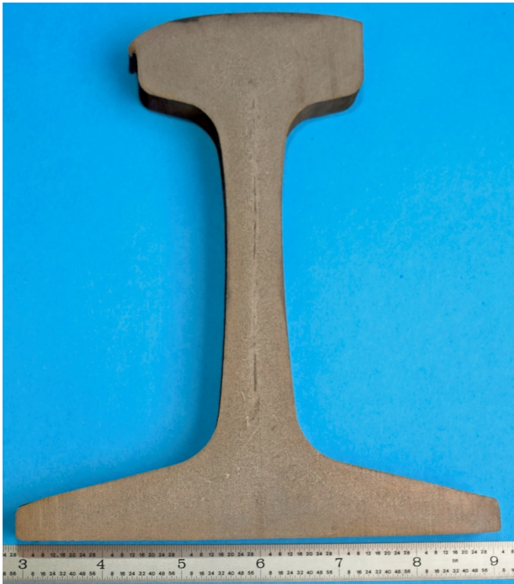
Figure 8: Macroetch showing centerline segregation
