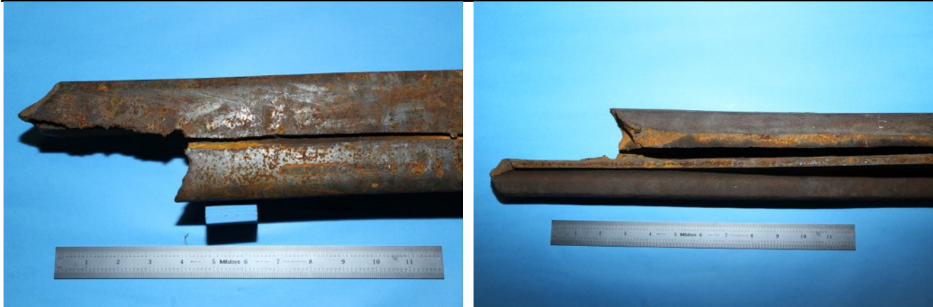
Figure 3: Photographs of a section of rail split vertically through the head.
