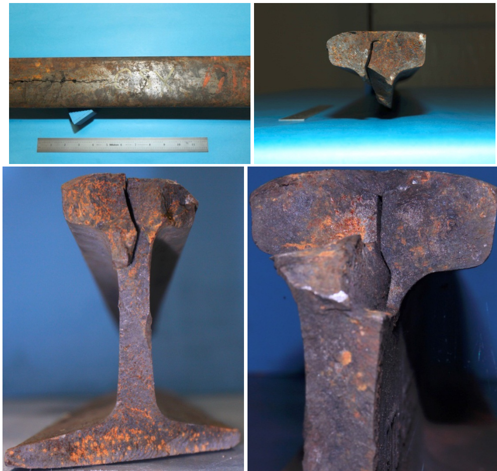
Figure 4: Head widening is visible near the right (Top Left) as a cross-sectional view of the VHS (Top Right and Bottom Left and Right)
