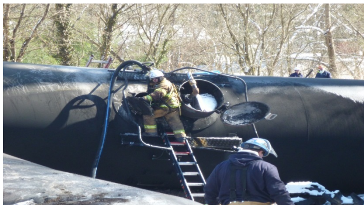
Figure 6: Inspecting a tank car after the fires stopped burning.
