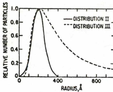
Figure 5.5. Two particle-size distribution used for the calculation of the emissivity of carbon particles. [ ]
