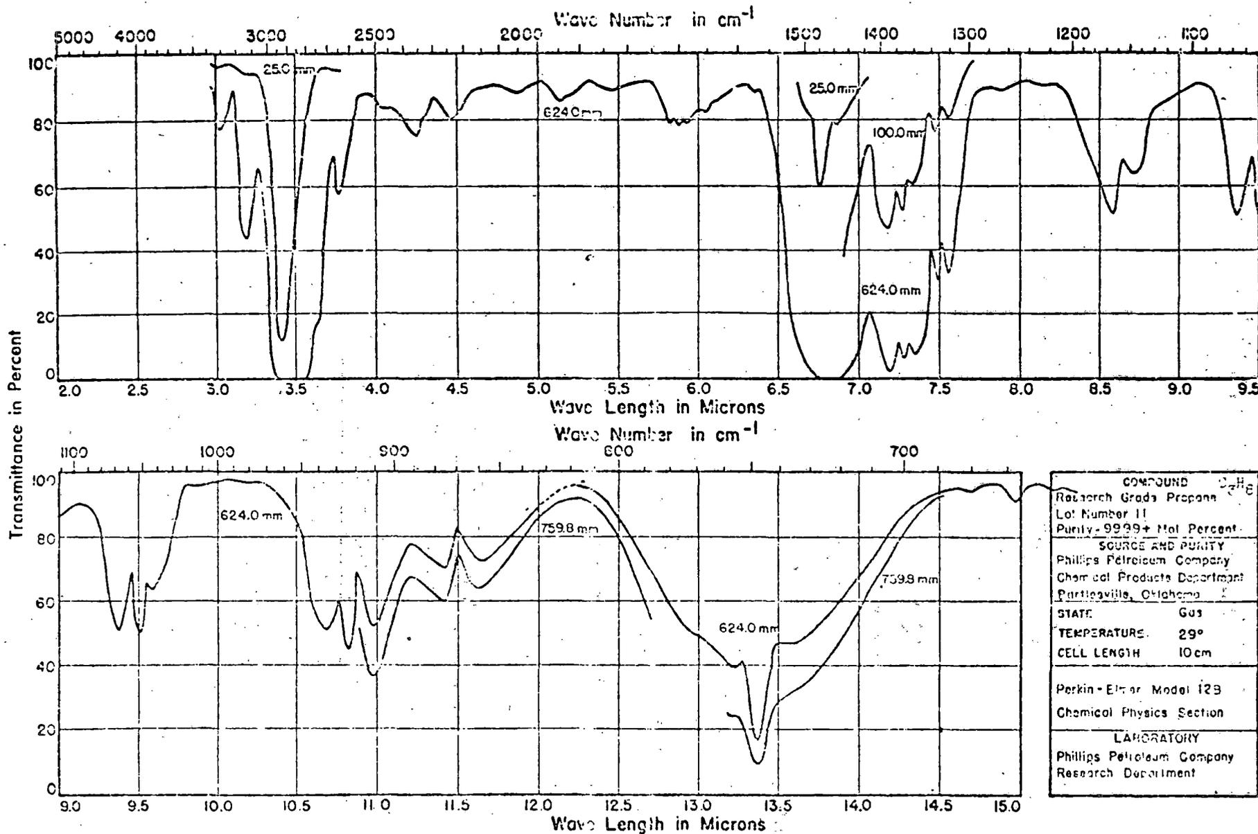
Figure 5.3 Spectral transmittance of propane gas through 10 cm long cell at room temperature.
