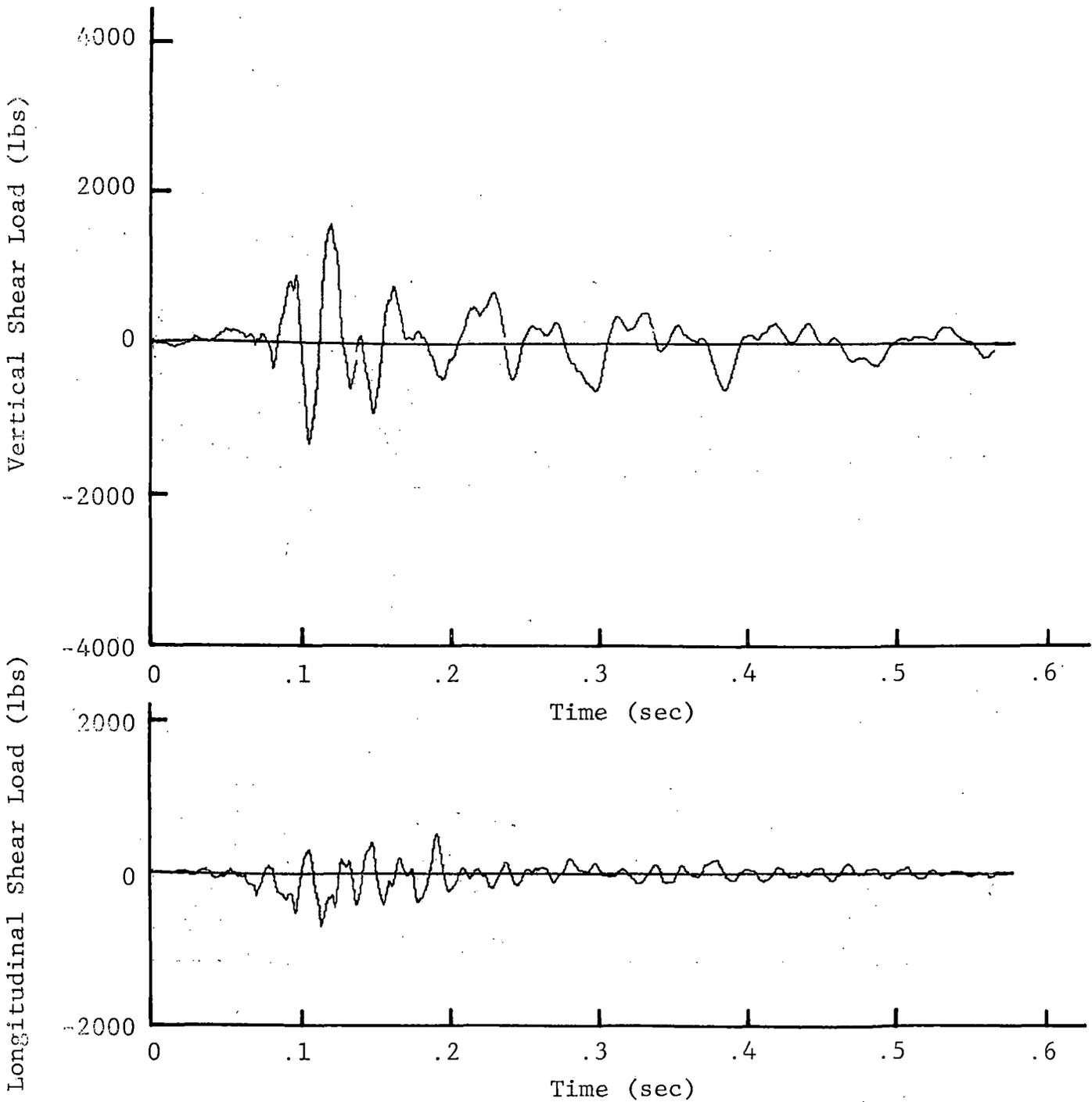
Figure 21 VERTICAL AND LONGITUDINAL SHEAR LOADS ON SIDE SILL FROM SHIELD SUPPORT ANGLE, RIGID TUBE SUPPORT, IMPACT NO. 5, 6.31 MPH (NOTE: POSITIVE LOAD IS DOWN OR FORWARD)
