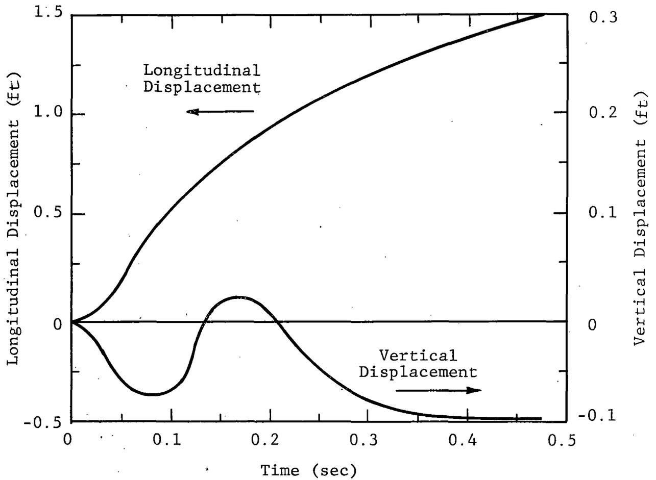
Figure 24 LONGITUDINAL AND VERTICAL DISPLACEMENT OF STRUCK CAR ON ANVIL CAR TEST, 7.04 MPH IMPACT SPEED
