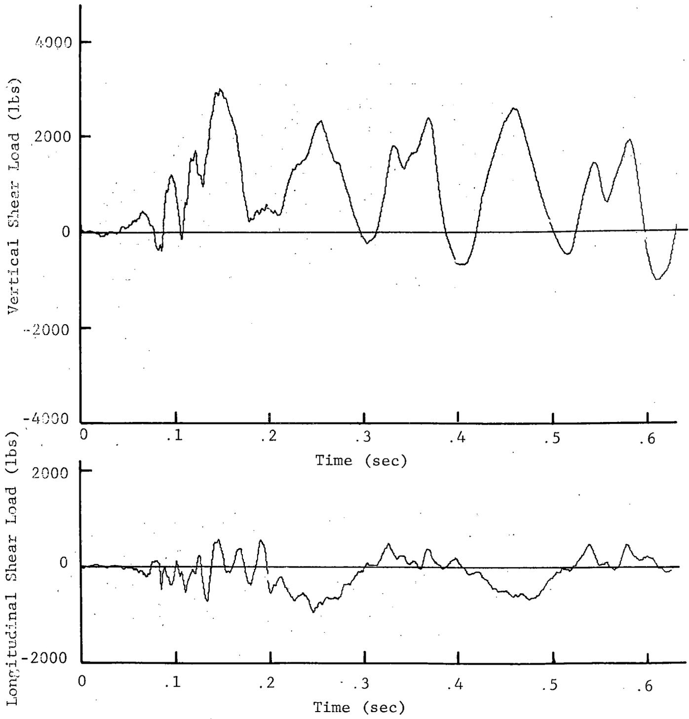
Figure 18 VERTICAL AND LONGITUDINAL SHEAR LOADS ON SIDE SILL FROM SHIELD SUPPORT ANGLE, FLEXIBLE STRAP SUPPORT, IMPACT NO. 5, 6.29 MPH (NOTE: POSITIVE LOAD IS DOWN OR FORWARD)
