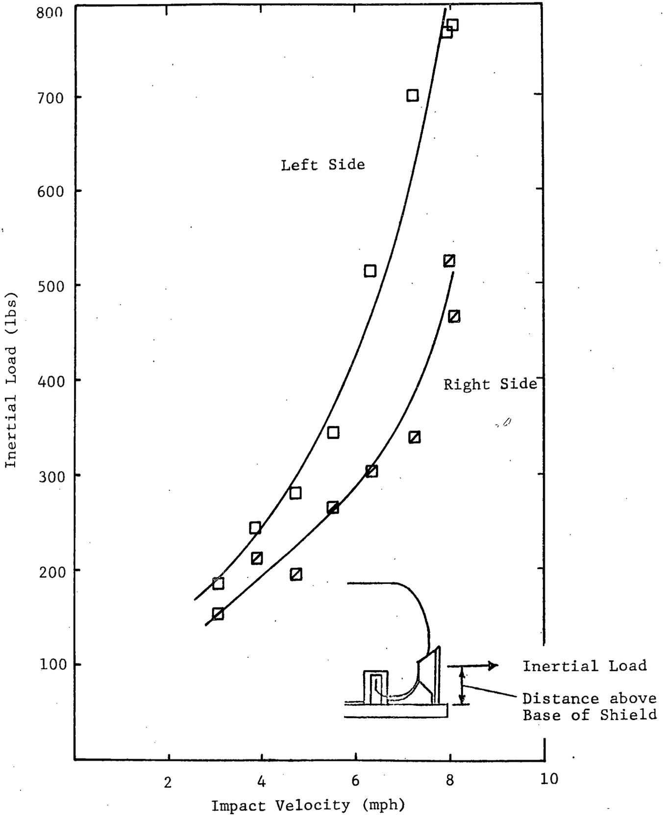
Figure 14 MAXIMUM LONGITUDINAL INERTIAL LOAD ACTING THROUGH STRAP SHIELD SUPPORTS
