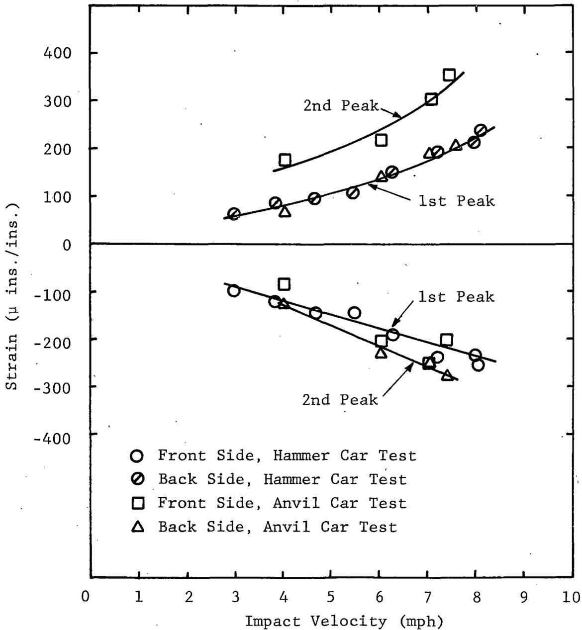
Figure 27 HORIZONTAL STRAINS MEASURED ON LEFT SIDE OF SHIELD, COMPARISON OF HAMMER CAR AND ANVIL CAR TEST DATA
