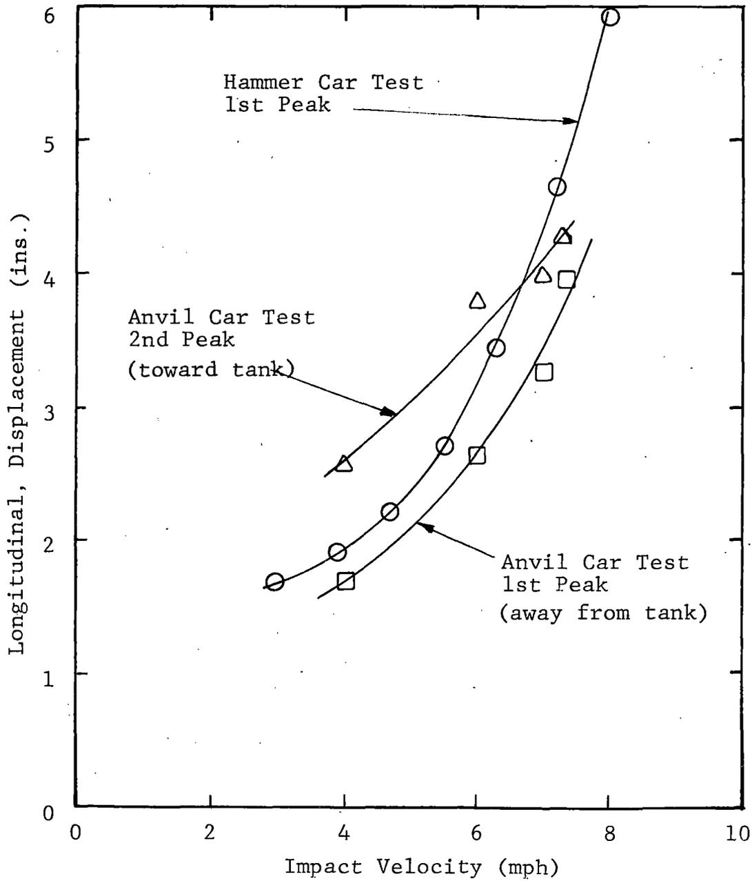
Figure 23 LONGITUDINAL DISPLACEMENT (AWAY FROM CAR) OF TOP CENTER OF SHIELD, COMPARISON OF HAMMER CAR AND ANVIL CAR TEST DATA
