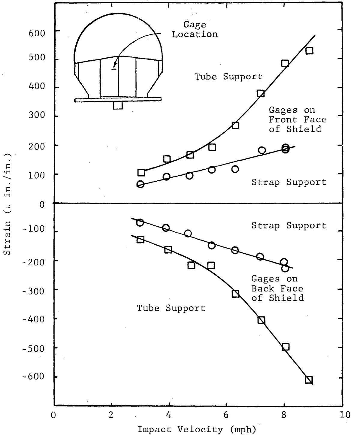
Figure 12 MAXIMUM HORIZONTAL STRAINS MEASURED ON GAGES AT CENTER OF SHIELD
