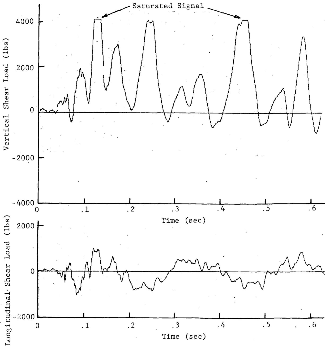
Figure 19 VERTICAL AND LONGITUDINAL SHEAR LOADS ON SIDE SILL FROM SHIELD SUPPORT ANGLE, FLEXIBLE STRAP SUPPORT, IMPACT NO. 7, 7.98 MPH (NOTE: POSITIVE LOAD IS DOWN OR FORWARD)
