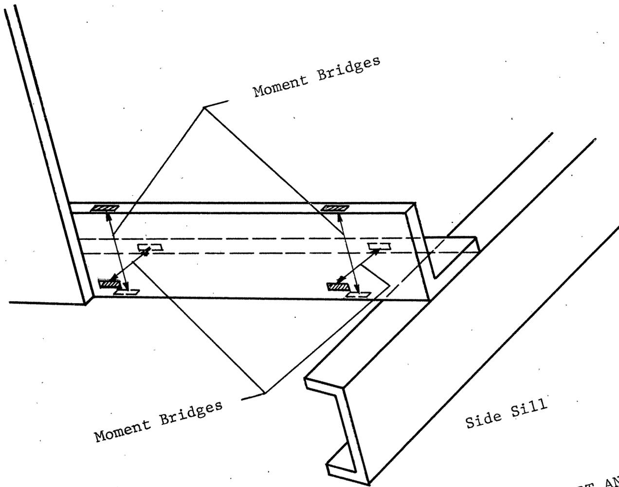
Figure 9 STRAIN GAGE PLACEMENT ON HEAD SHIELD SUPPORT ANGLE,
