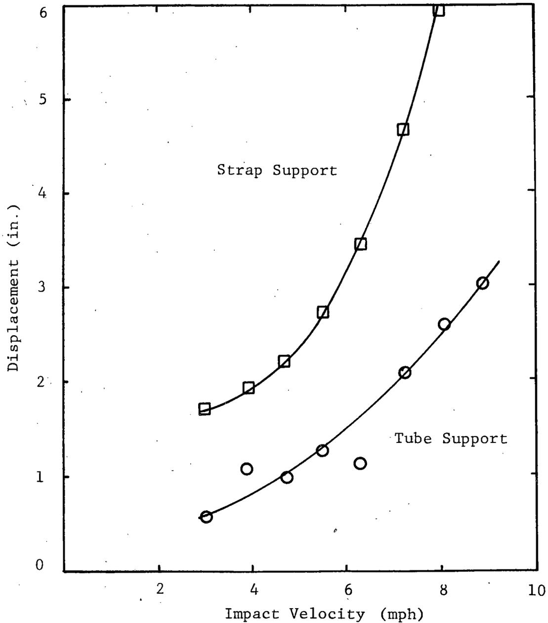
Figure 11 MAXIMUM LONGITUDINAL DISPLACEMENT (AWAY FROM CAR) OF TOP CENTER OF SHIELD
