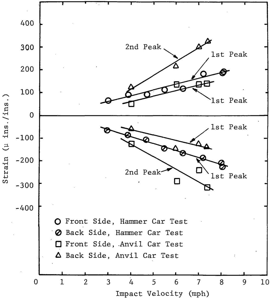
Figure 26 HORIZONTAL STRAINS MEASURED ON GAGES AT CENTER OF SHIELD, COMPARISON OF HAMMER CAR AND ANVIL CAR TEST DATA
