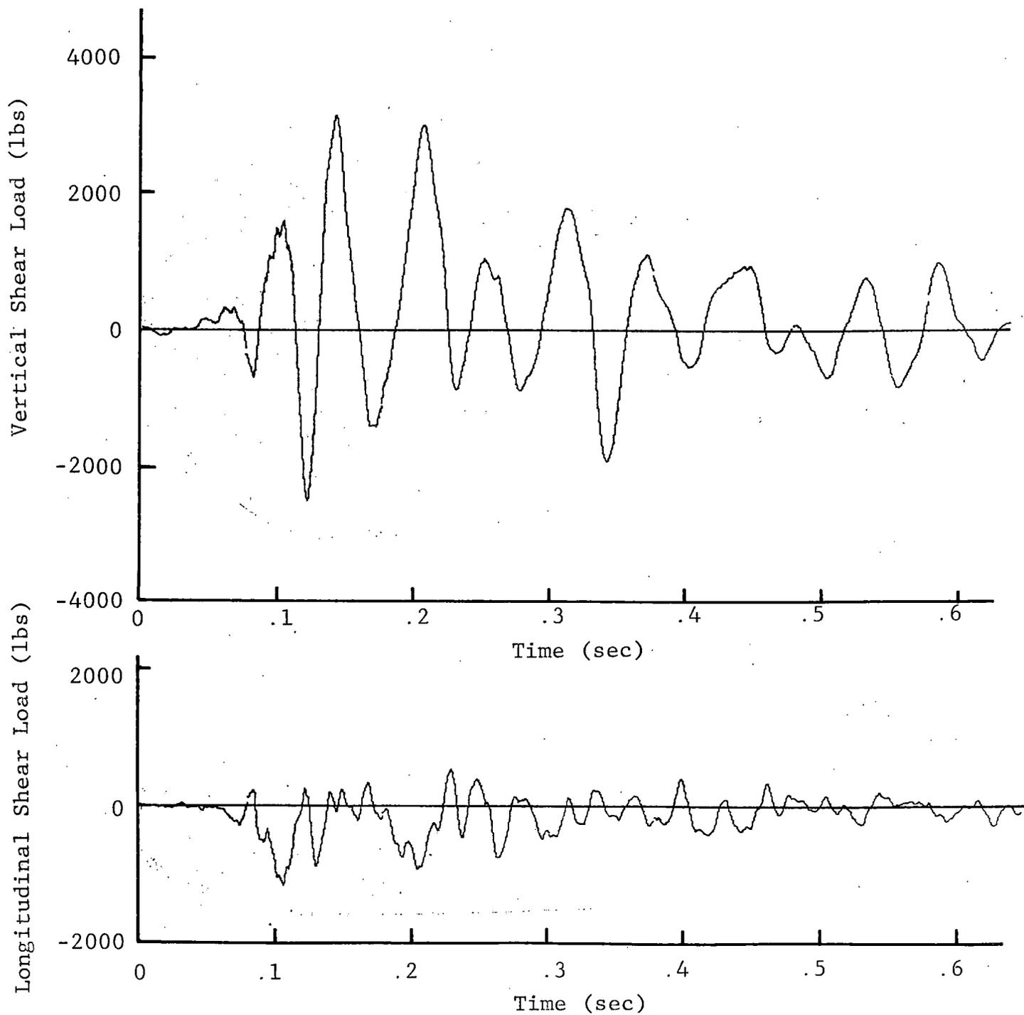
Figure 22 VERTICAL AND LONGITUDINAL SHEAR LOADS ON SIDE SILL FROM SHIELD SUPPORT ANGLE, RIGID TUBE SUPPORT, IMPACT NO. 7, 8.06 MPH (NOTE: POSITIVE LOAD IS DOWN OR FORWARD)
