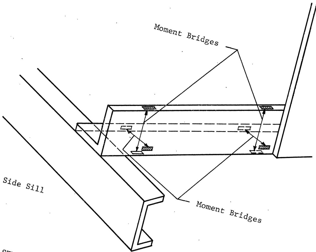
Figure 8 STRAIN GAGE PLACEMENT ON HEAD SHIELD SUPPORT ANGLE, LEFT SIDE OF CAR
