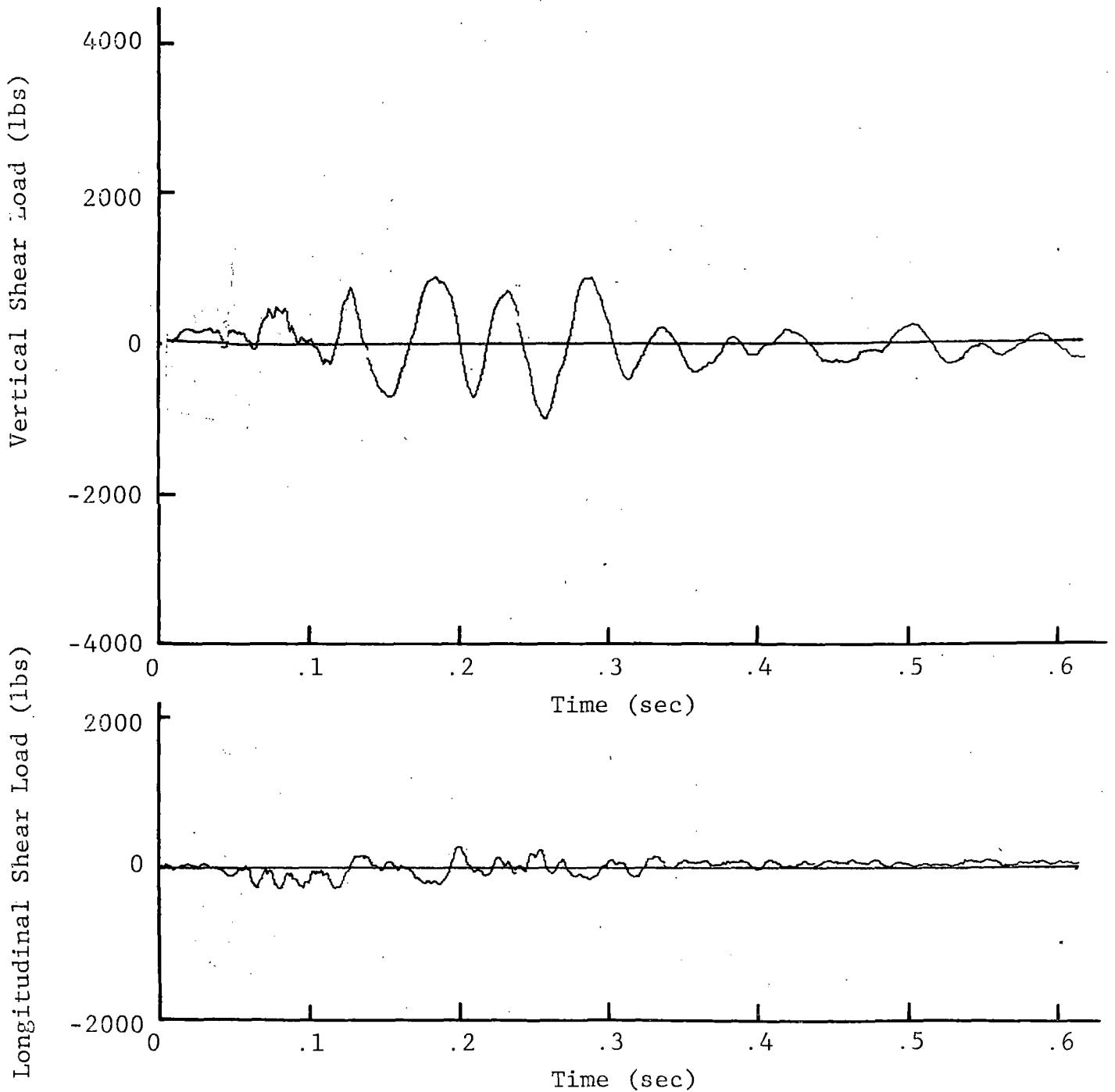
Figure 20 VERTICAL AND LONGITUDINAL SHEAR LOADS ON SIDE SILL FROM SHIELD SUPPORT ANGLE, RIGID TUBE SUPPORT, IMPACT NO. 3, 4.74 MPH (NOTE: POSITIVE LOAD IS DOWN OR FORWARD)
