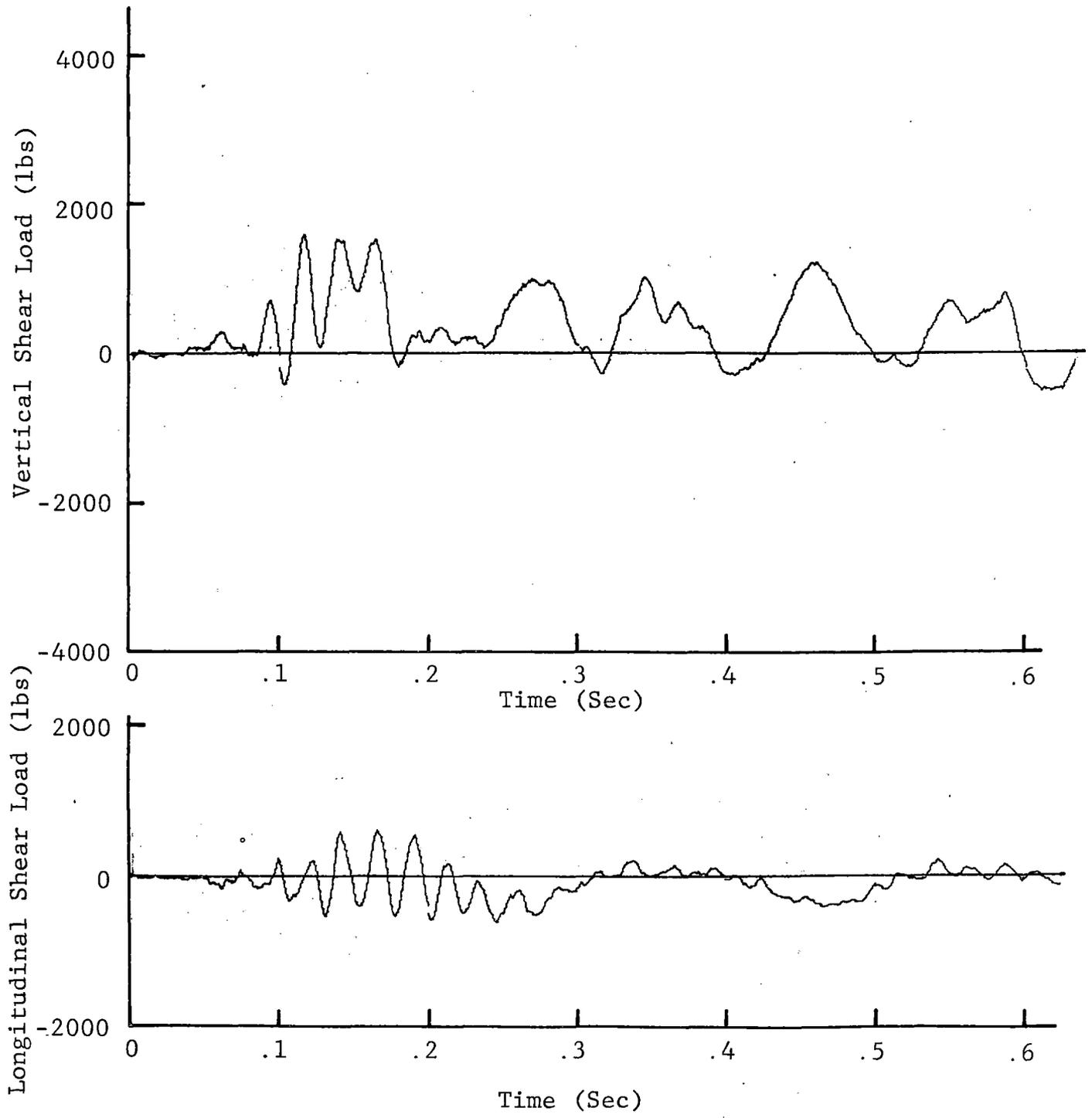
Figure 17 VERTICAL AND LONGITUDINAL SHEAR LOADS ON SIDE SILL FROM SHIELD SUPPORT ANGLE FLEXIBLE STRAP SUPPORT, IMPACT NO. 3, 4.68 MPH (NOTE: POSITIVE LOAD IS DOWN OR FORWARD)
