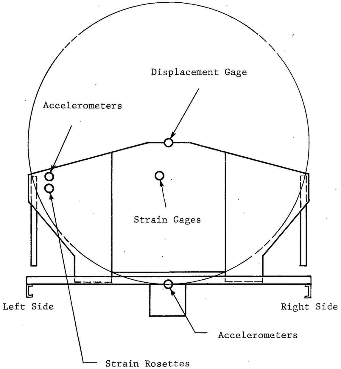
Figure 6 TRANSDUCER LOCATIONS FRONT VIEW OF SHIELD
