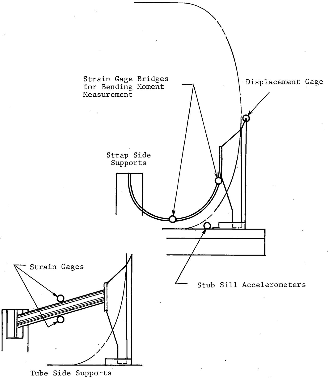
Figure 7 TRANSDUCER LOCATIONS SIDE VIEW OF SHIELD AND CAR
