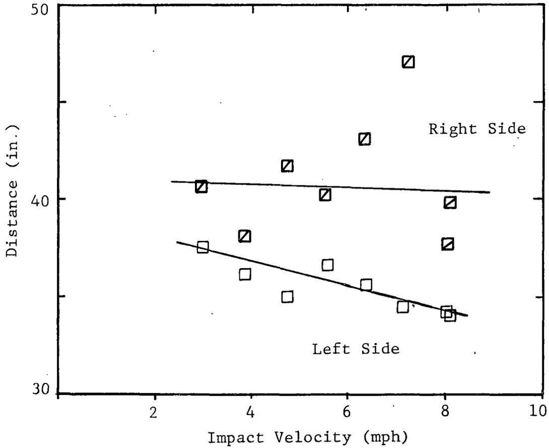
Figure 15 DISTANCE ABOVE BASE OF SHIELD FOR LINE-OF-ACTION OF LONGITUDINAL INERTIAL LOAD, STRAP SUPPORT FOR SHIELD
