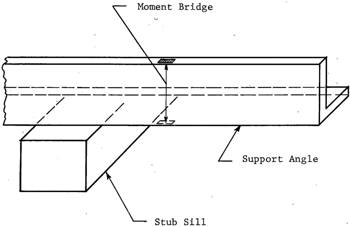
Figure 10 STRAIN GAGE PLACEMENT ON HEAD SHIELD SUPPORT ANGLE NEAR CENTER OF CAR
