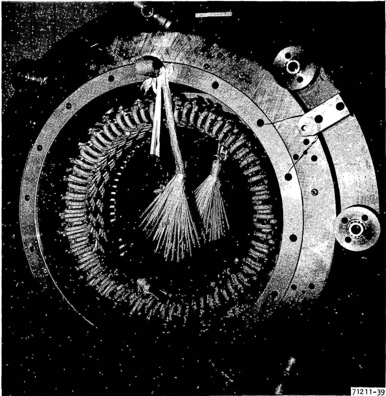
Figure 5-9. Support Arrangement for Installation of Last 15 Coils
