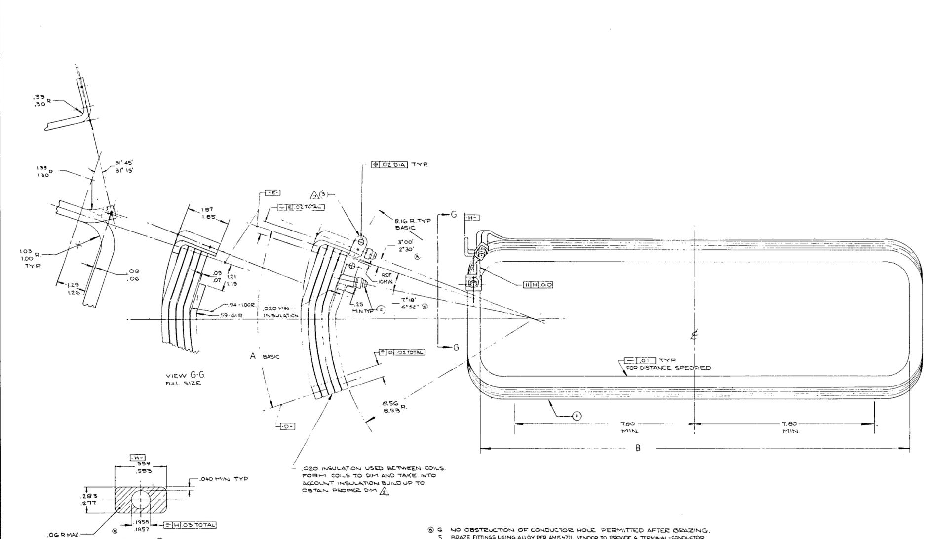
WEIGHT OF CONDUCTOR TO BE .483-495 LBS/FT AT ANY SECTION, NOMINAL COPPER AREA TO BE .124 IN<sup>2</sup> AND NOMINAL HOLE AREA TO BE .0285 IN<sup>2</sup>
