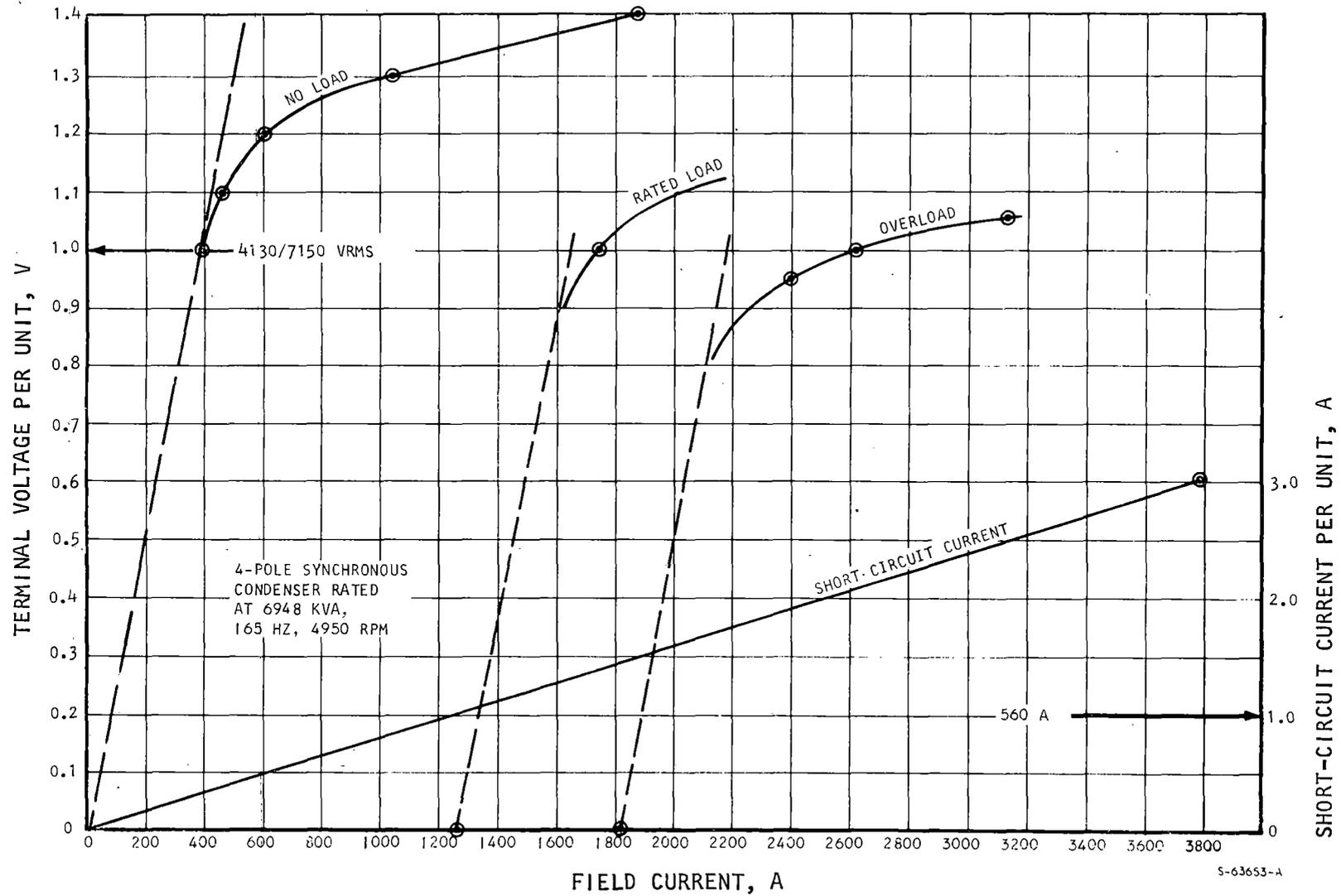
Figure 3-2. Load/No-Load Saturation and Short-Circuit Current Performance (Calculated)
