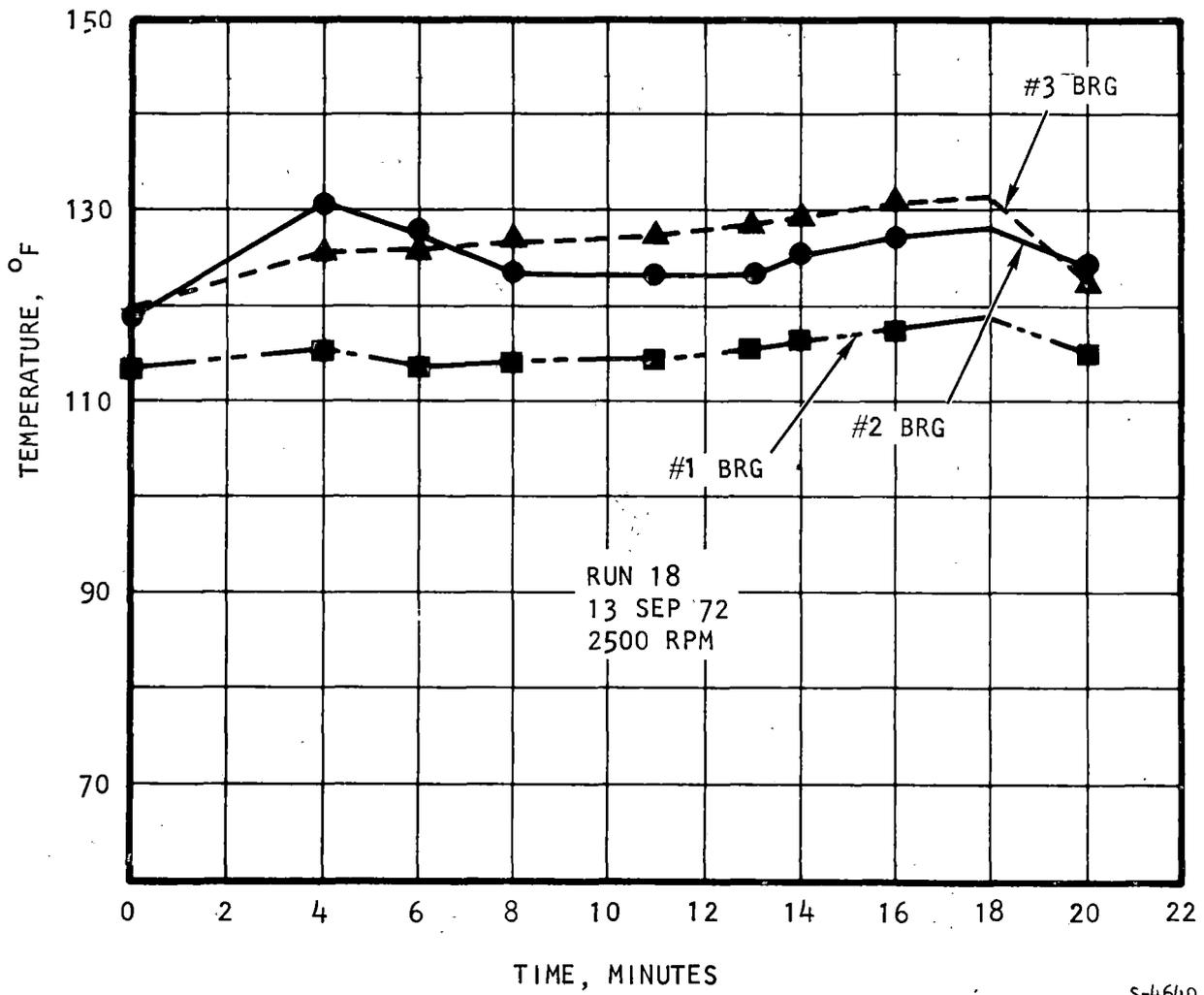
Figure 7-8. Bearing Temperatures at End of Test Run
