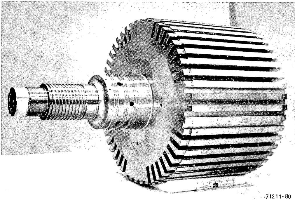
Figure 5-2. Finished Machined Rotor Core
