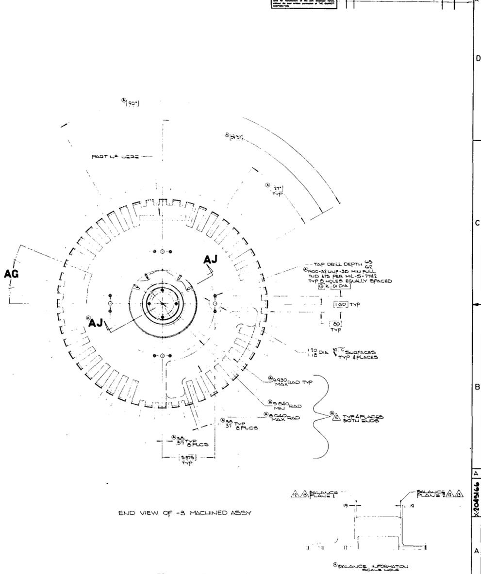
Figure 9-5. Assembly Drawing 2045166, Rotor Core Assembly (Page 2 of 2)
