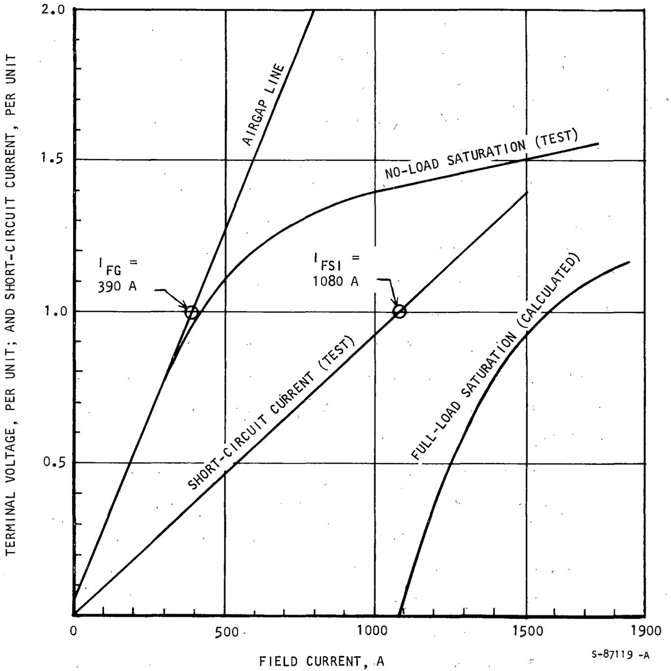
Figure 7-15. No-Load Saturation, Short-Circuit Current, and Full-Load Saturation Tests
