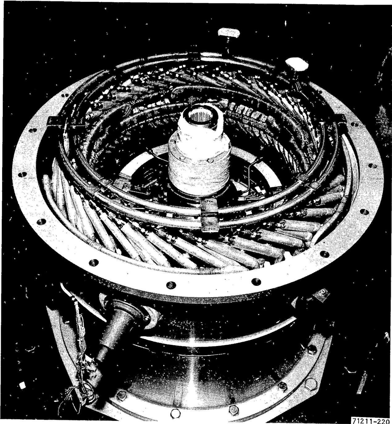
Figure 5-12. Stator Coil Coolant Transfer Tube and Manifold Assembly (Prior to Shrinking Installation)
