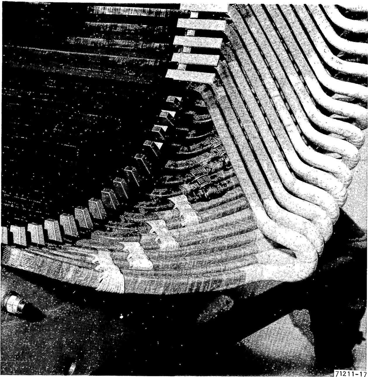
Figure 5-8. Stator Stack and Coil Assembly -
