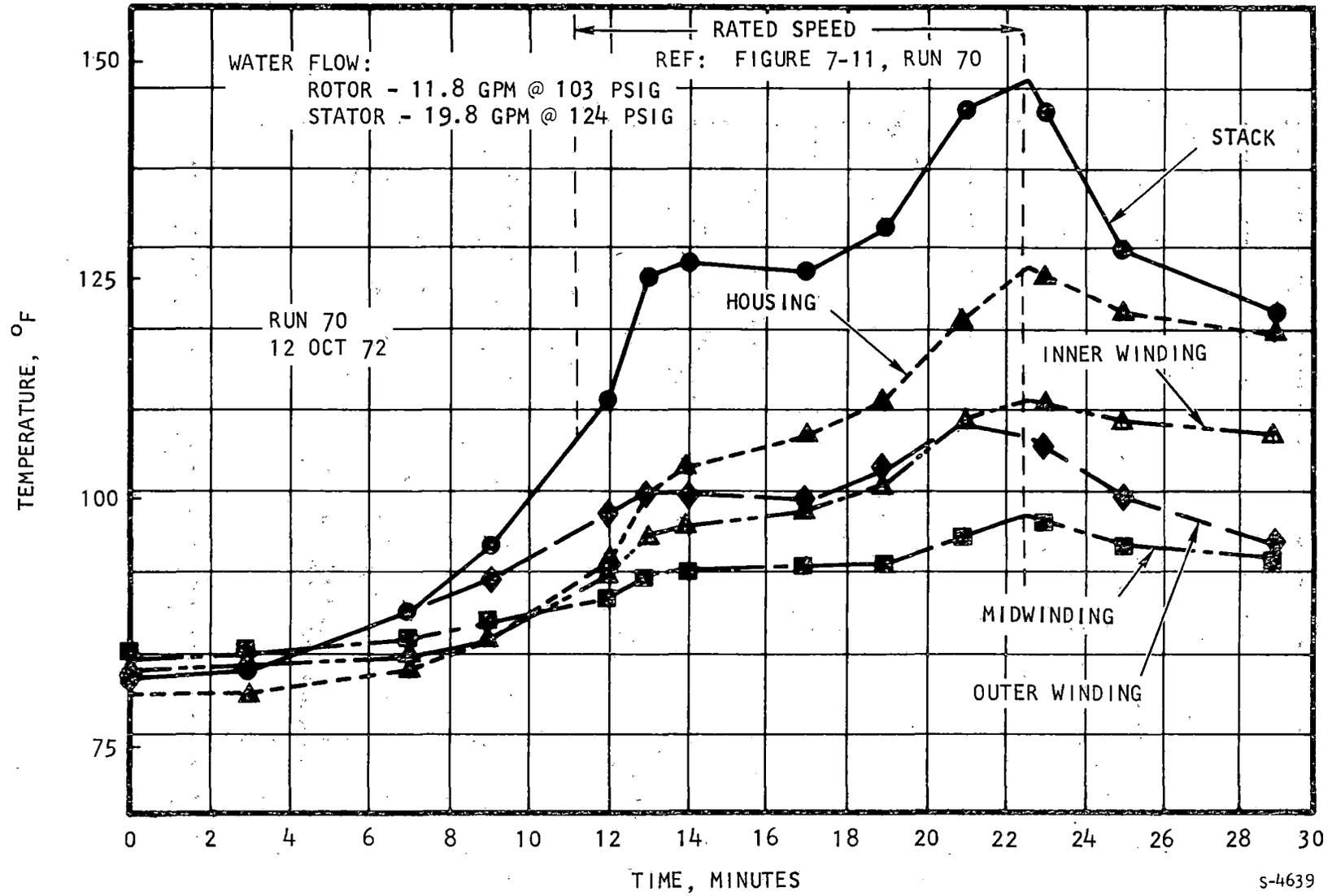
Figure 7-10. Coolant Water Temperature vs Running Time
