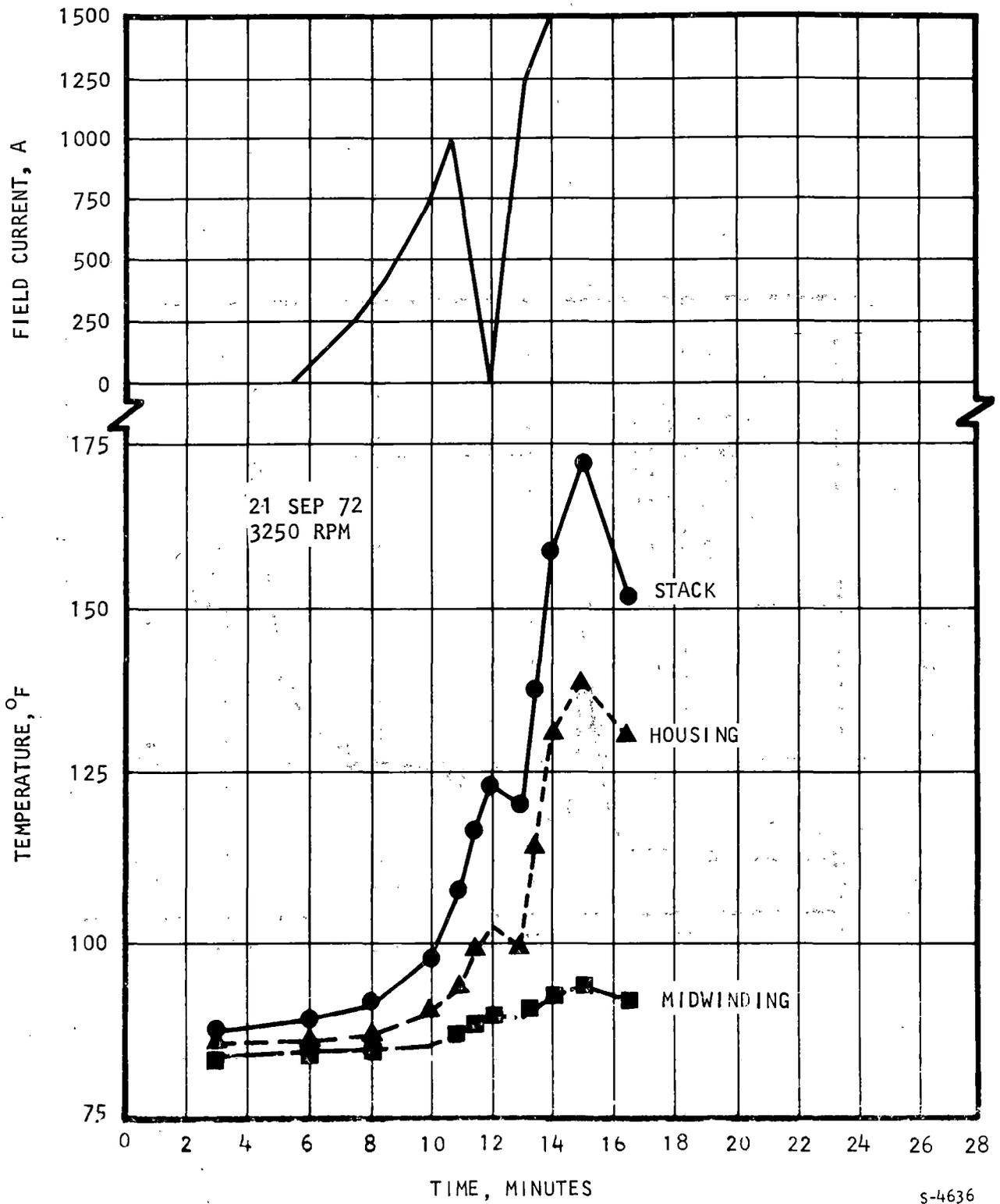
Figure 7-13. No-Load Saturation Test, Run 48
