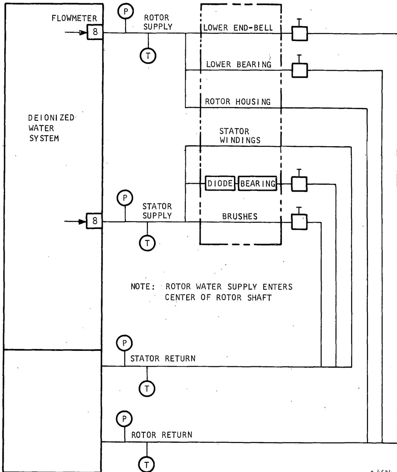
Figure 7-17. Cooling Water System Schematic
