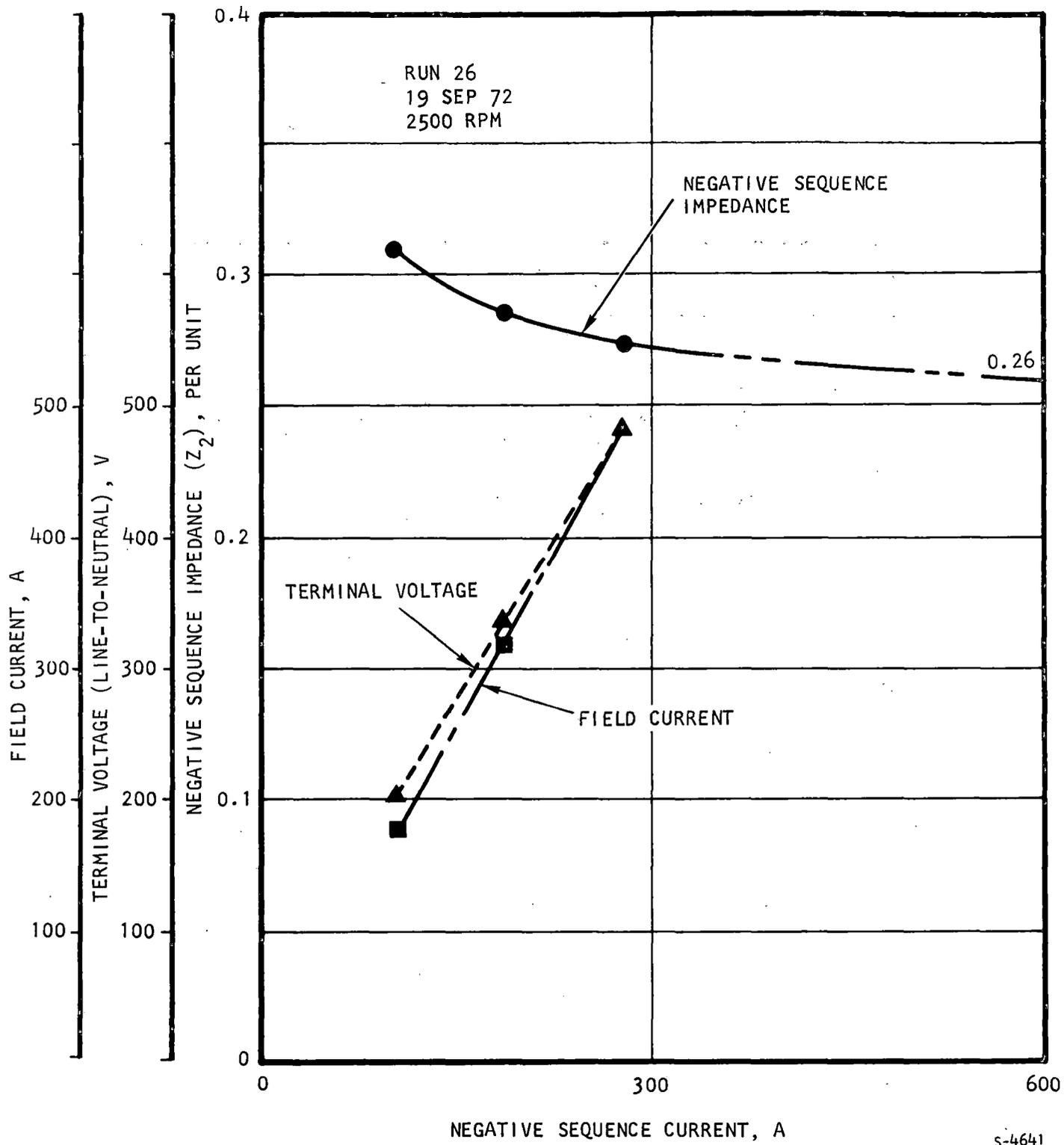
Figure 7-7. Negative Sequence Impedance Test at One-Half Rated Speed
