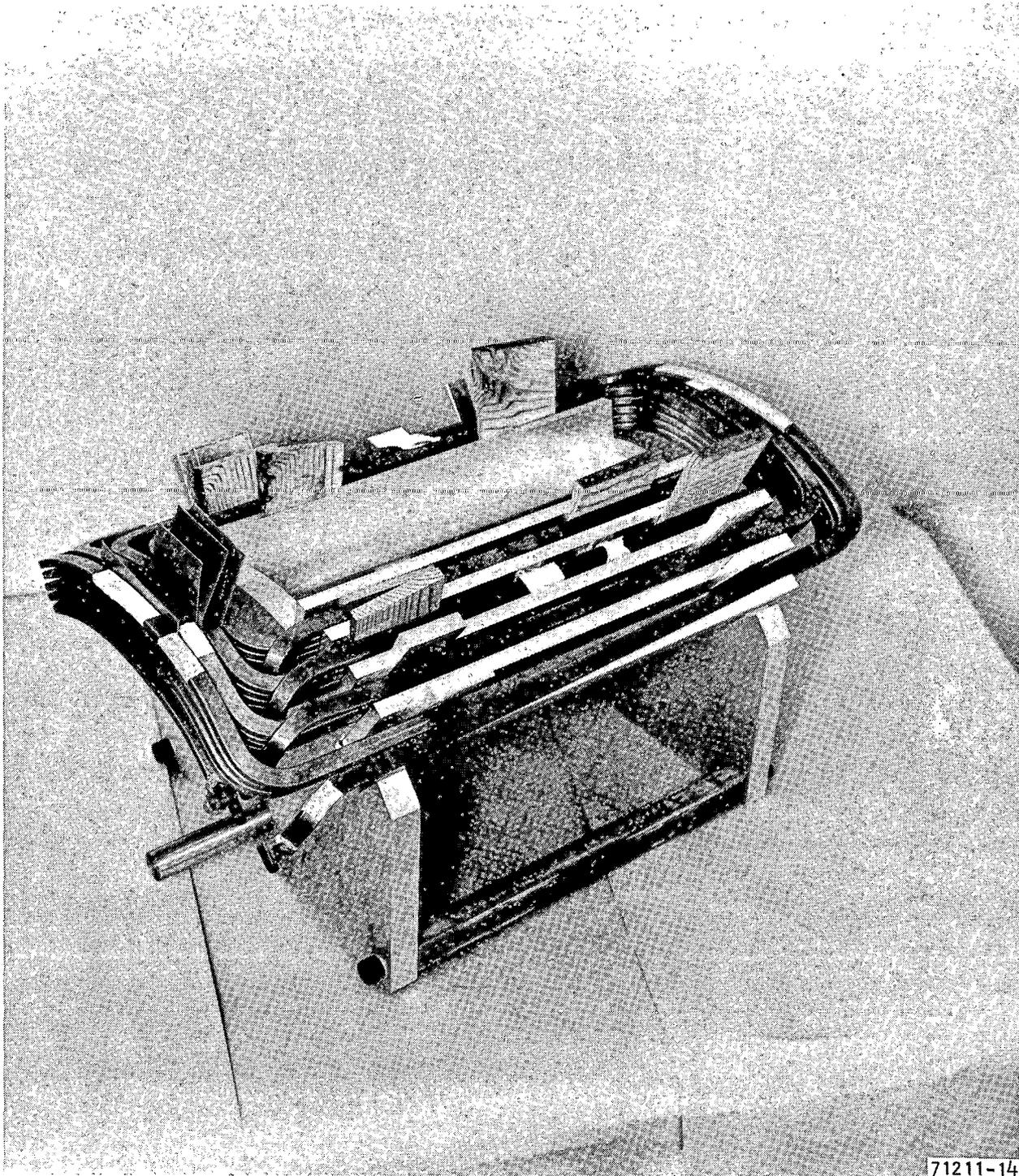
Figure 5-4. Rotor Coils in Inspection Fixture
