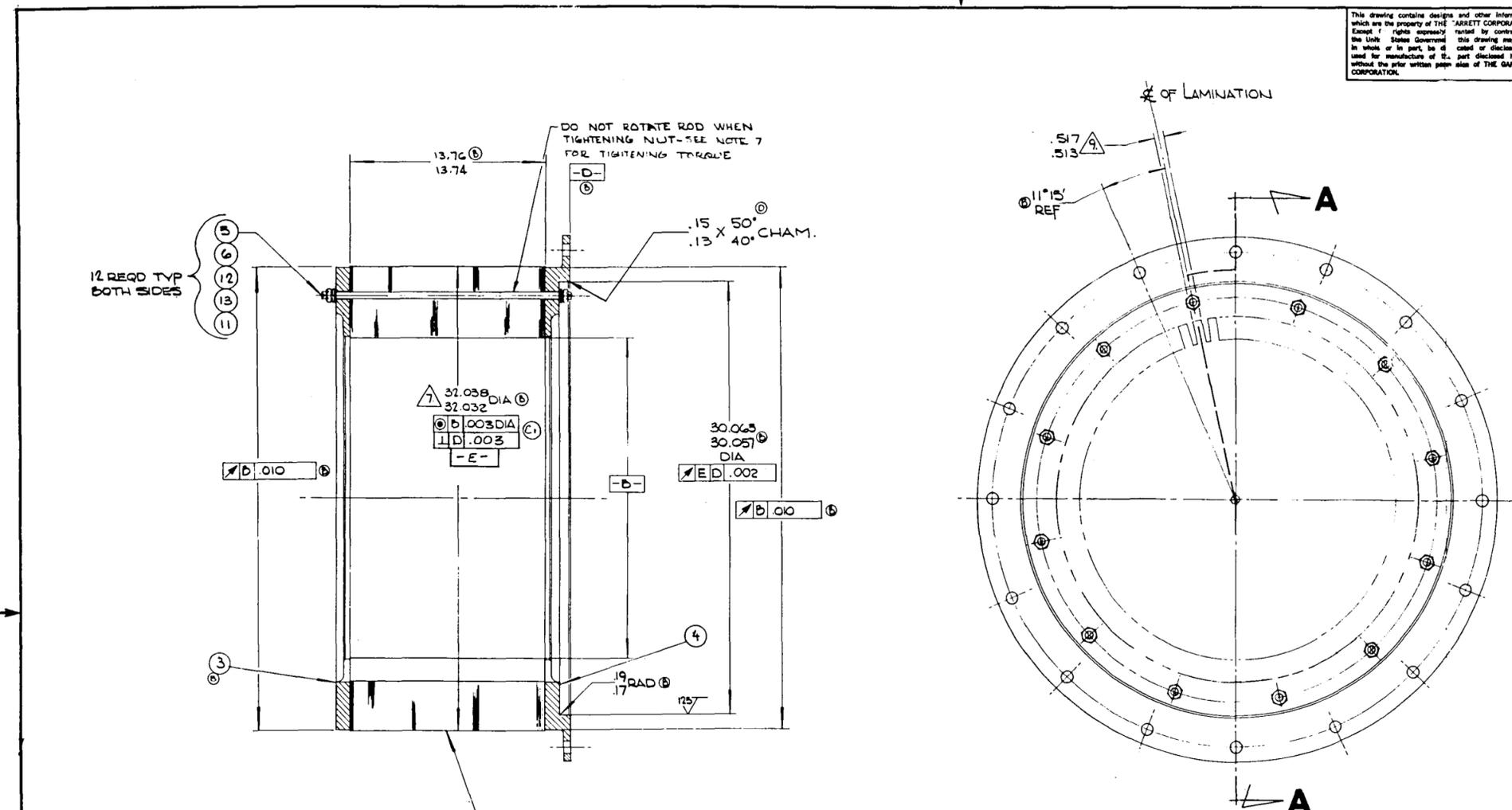
Figure 9-3. Assembly Drawing 2045162, Stator Stack Assembly
