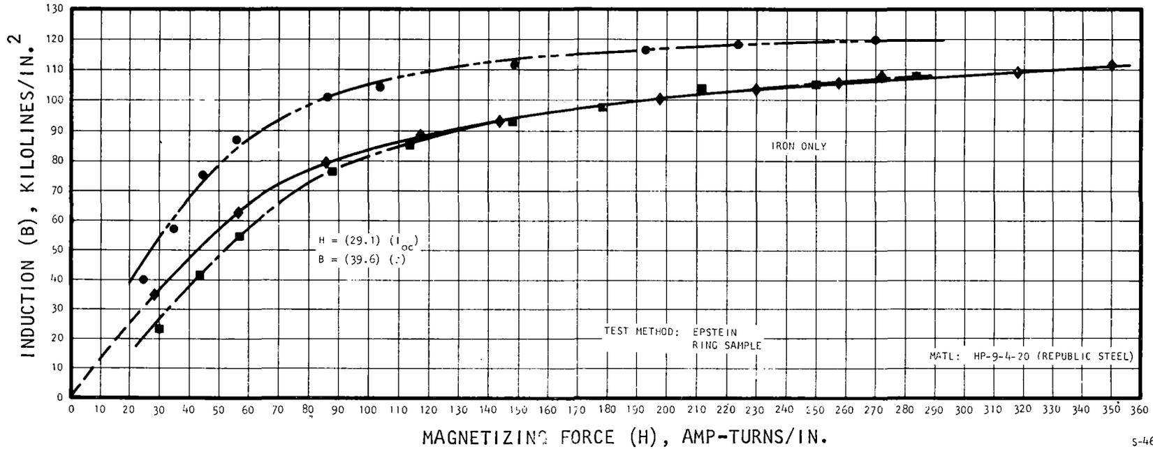
Figure 4-1. Rotor Core Material Magnetic Properties, LIMRV vs TLRV
