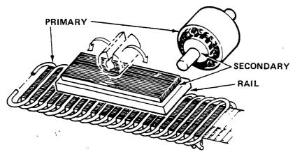
Figure 10. Principle of Single-Sided Linear Electric Motor
