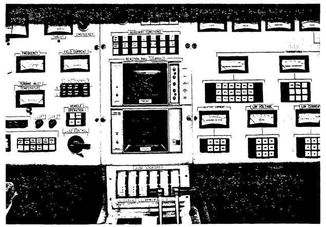
Figure 12, LIMRV Instrument: Van Remote Control Panel.
