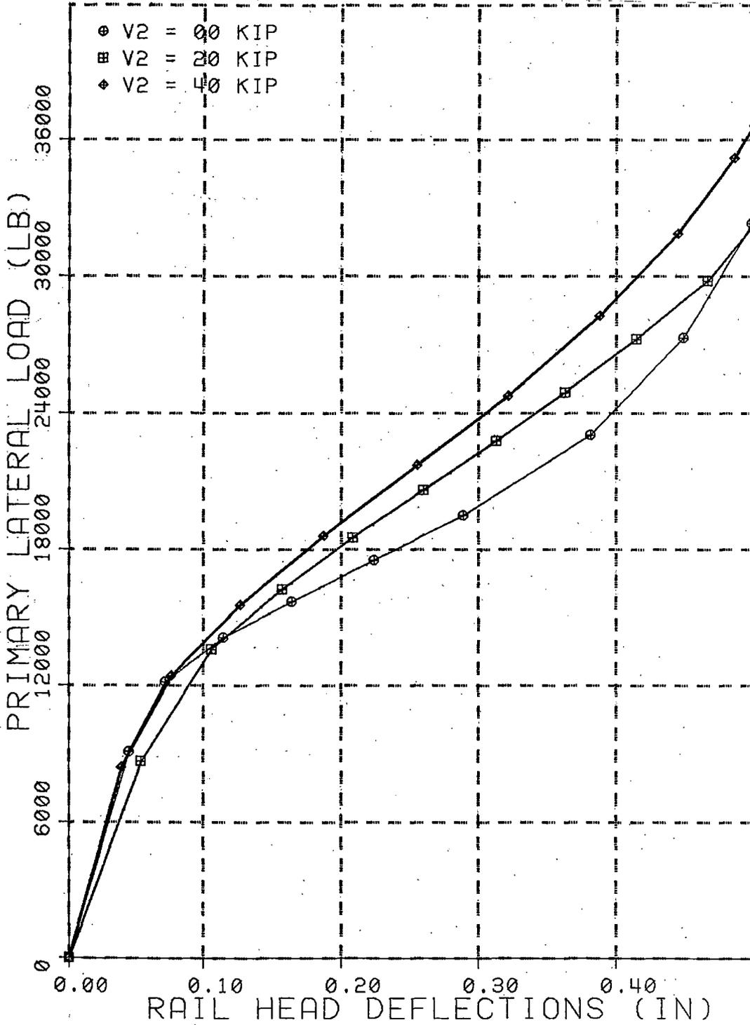
FIGURE 17. RAIL HEAD DEFLECTION VS PRIMARY LATERAL LOAD, FOR VARIOUS ADJACENT VERTICAL LOADS AND CONSTANT 20 KIP PRIMARY VERTICAL LOAD.
