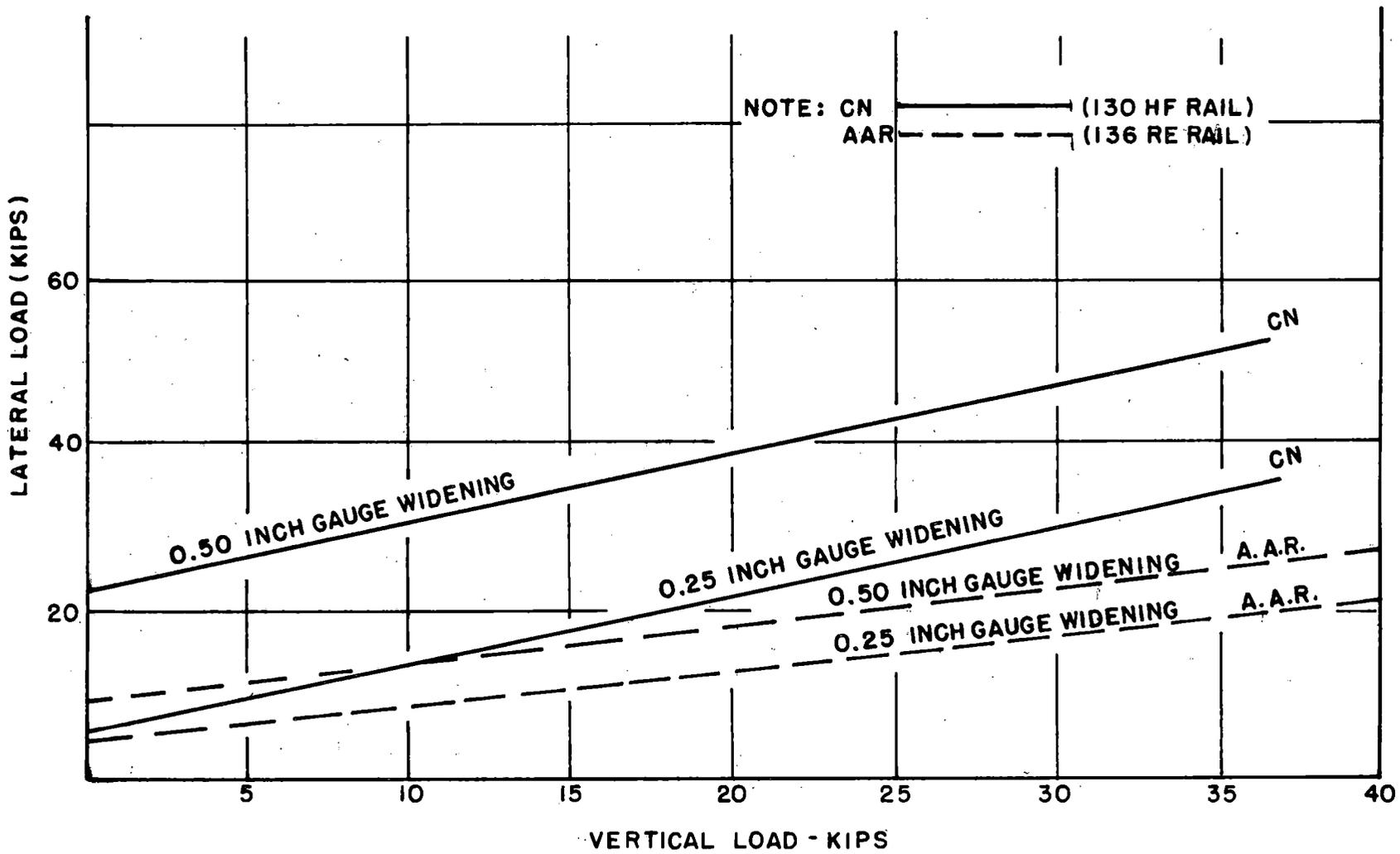
FIGURE II. LATERAL VS. VERTICAL RAIL LOADS - COMPARISON BETWEEN A.A.R. AND CANADIAN NATIONAL (7) TEST DATA
