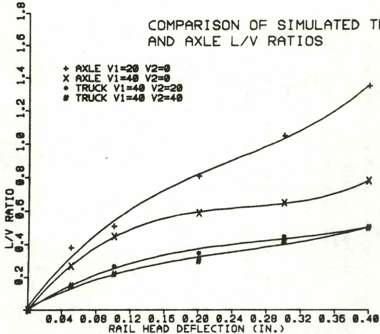
FIGURE 20. RAIL HEAD DEFLECTIONS VS SIMULATED SINGLE
