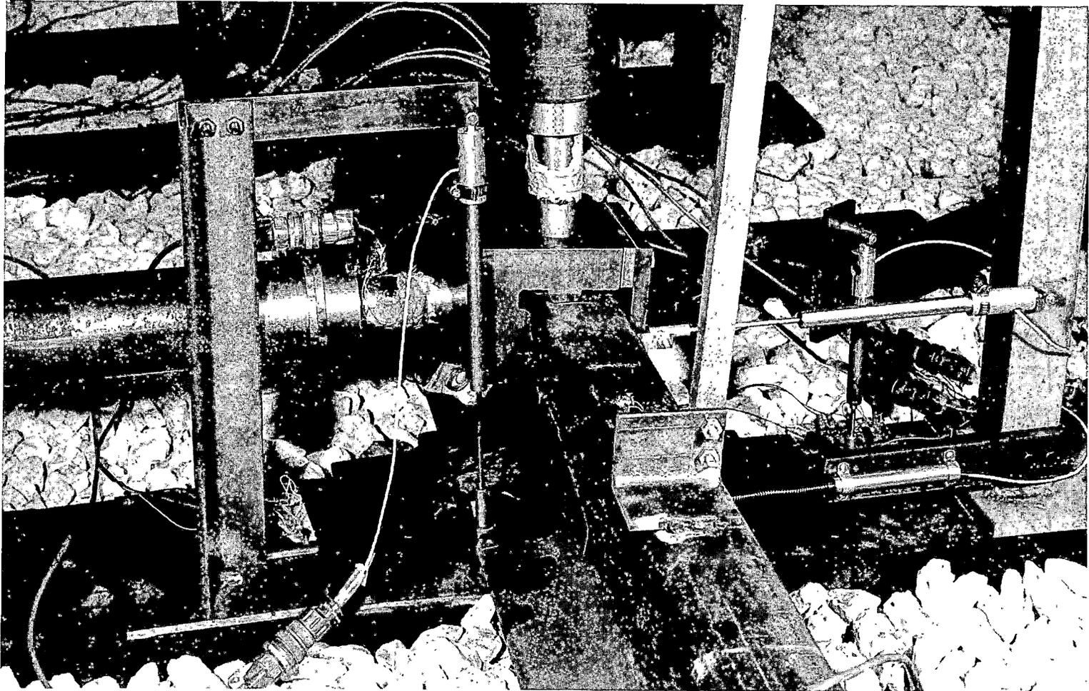
Figure 6. Typical Measurement Location for Rail Deflections: Railhead Lateral and Rail Base Lateral/Vertical.
