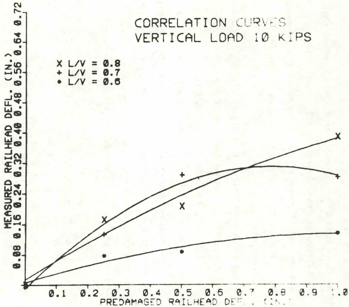
FIGURE 15. MEASURED VS. PREDAMAGED RAILHEAD DEFLECTION AT VARIOUS L/V LOADING RATIOS, AT CONSTANT VERTICAL LOAD OF 10 KIPS.
