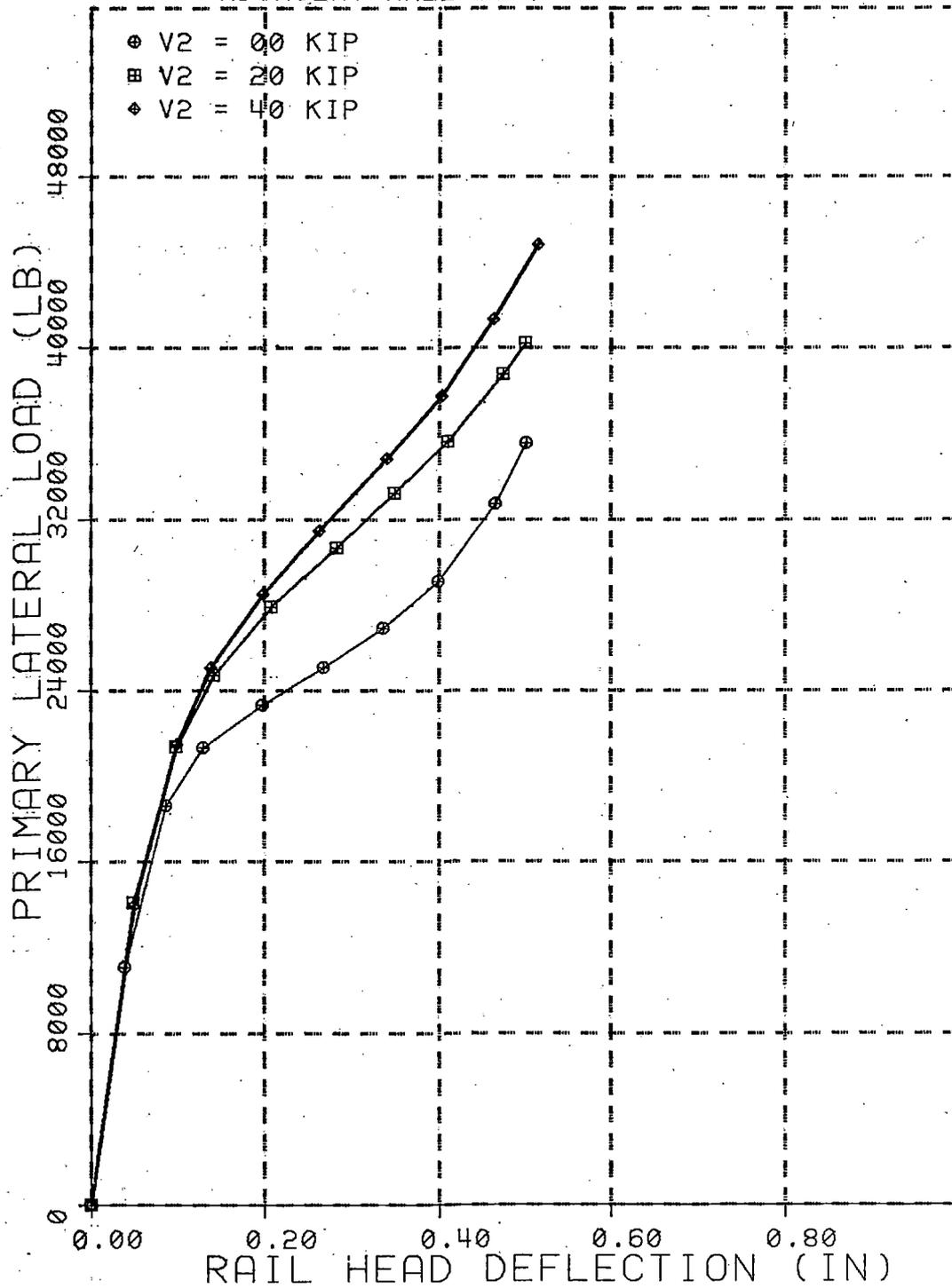
FIGURE 18. RAIL HEAD DEFLECTION VS PRIMARY LATERAL LOADS, FOR VARIOUS ADJACENT VERTICAL LOADS AND CONSTANT 40 KIP PRIMARY VERTICAL LOAD.
