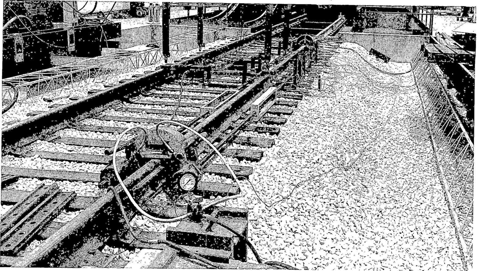
Figure 27. Test Set-Up for Longitudinal Load Tests, Showing Hydraulic Rail Puller in Position.
