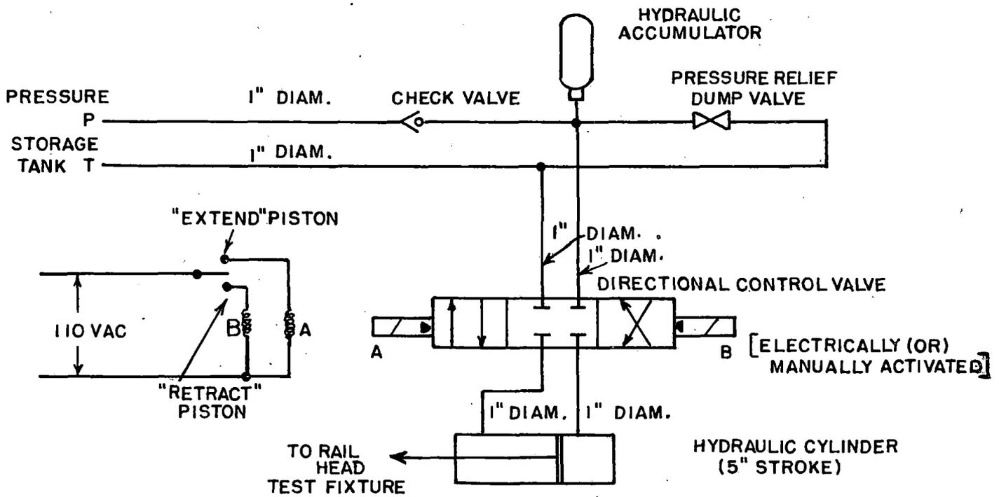
FIGURE 22. SCHEMATIC DIAGRAM FOR HYDRAULIC IMPULSE LOADING SYSTEM
