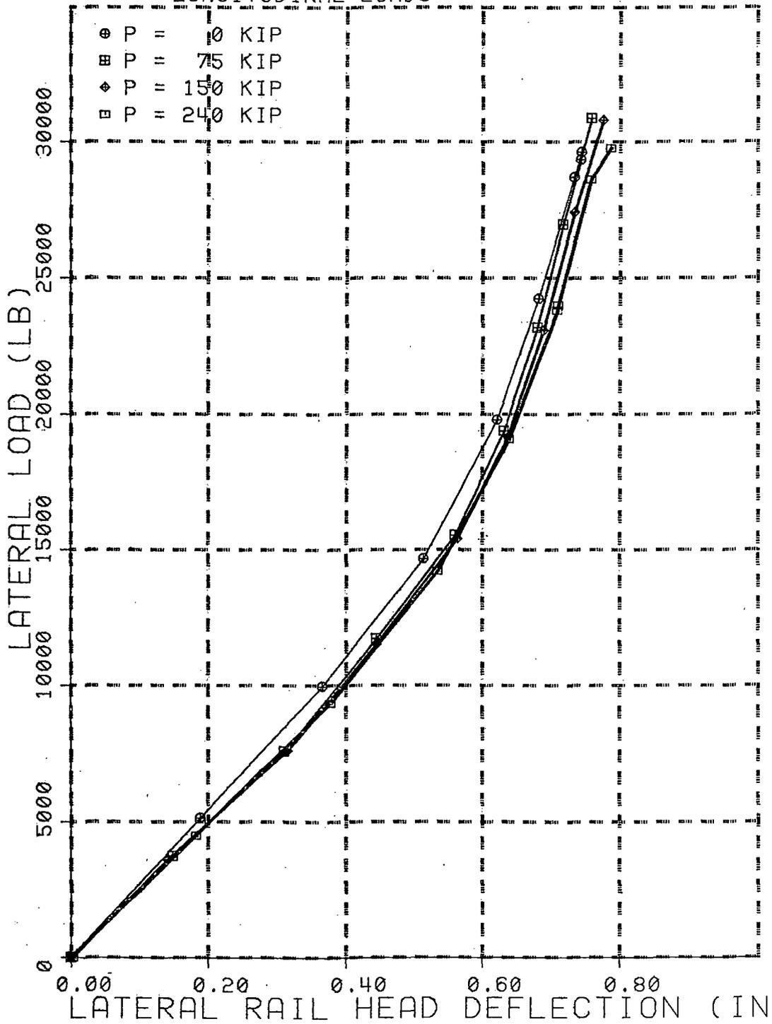
FIGURE 30. LATERAL RAIL HEAD DEFLECTION VS LATERAL LOAD, FOR VARIOUS LONGITUDINAL LOADS AND ZERO VERTICAL LOAD.
