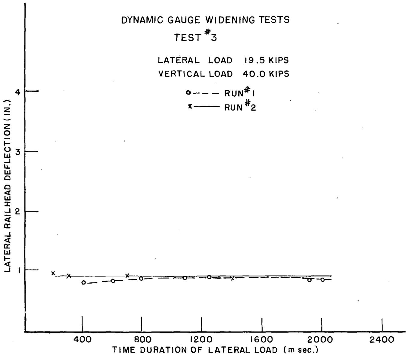
FIGURE 25. LATERAL RAILHEAD DEFLECTIONS VS. TIME DURATIONS OF A 19.5 Kip LATERAL IMPULSE LOAD, FOR A CONSTANT 40 Kip VERTICAL LOAD.
