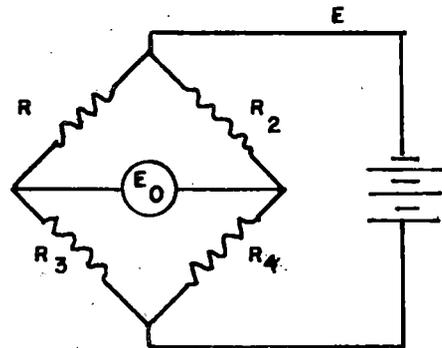
FIGURE 7. SCHEMATIC SHOWING RAIL-MOUNTED STRAIN GAUGE ORIENTATIONS AND ELECTRICAL BRIDGE MEASUREMENT CIRCUITRY.
