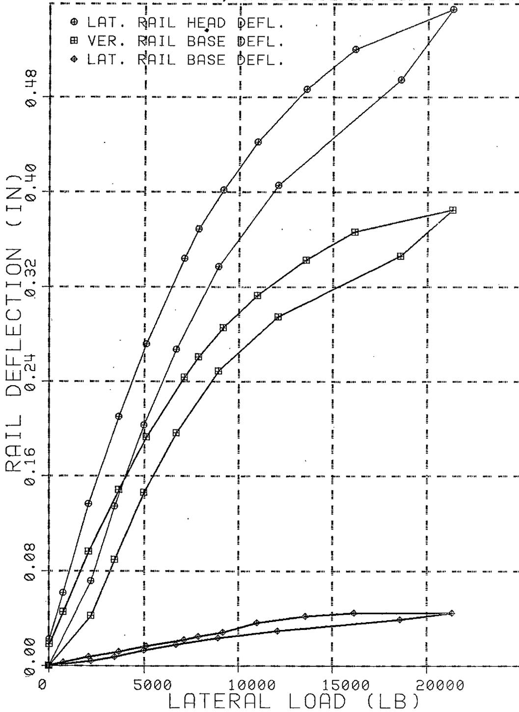
FIGURE 10. GRAPH SHOWING VARIOUS RAIL DEFECTIONS VS LATERAL LOADS, FOR ZERO VERTICAL LOAD.
