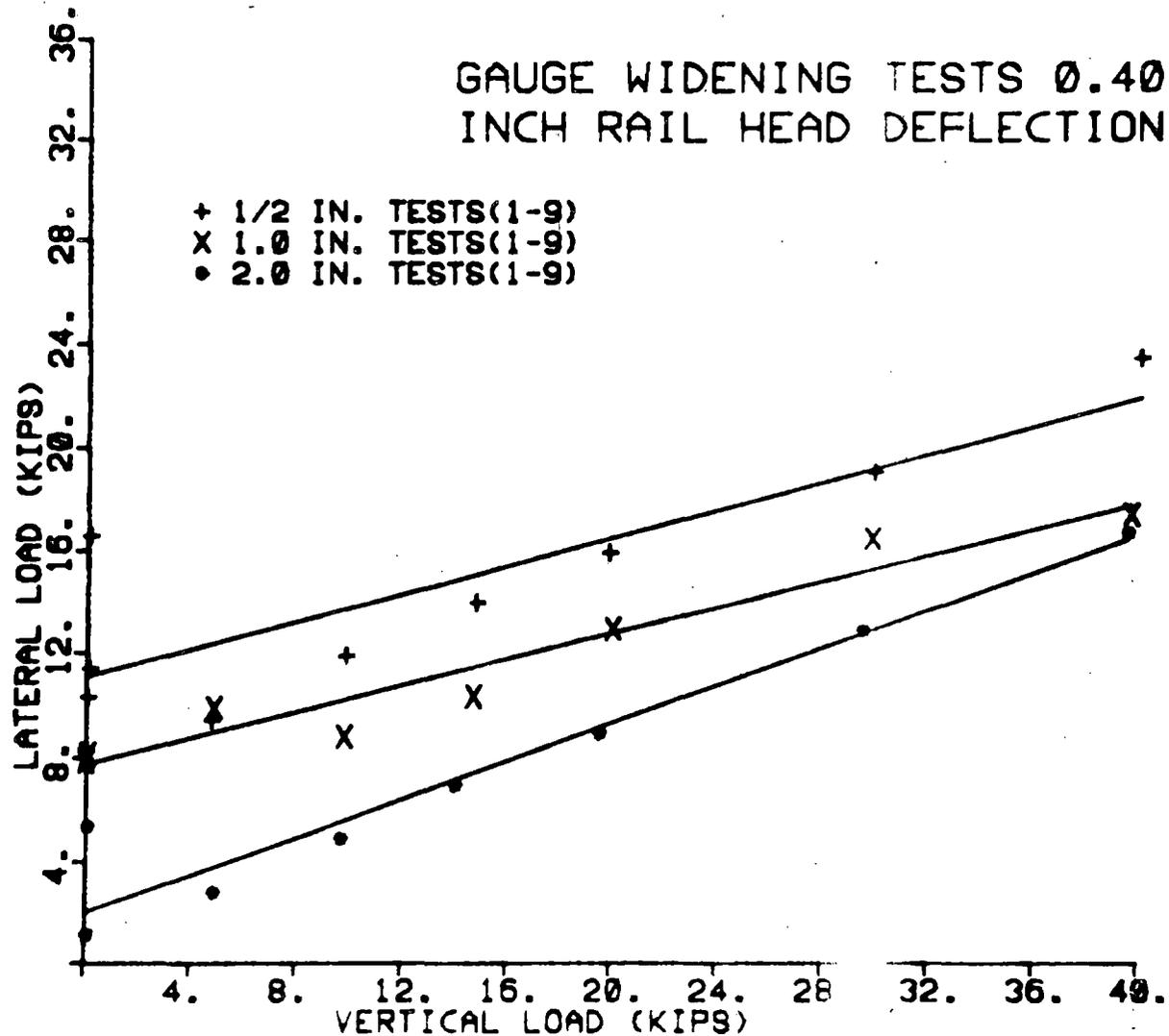
FIGURE 13. LATERAL VS VERTICAL RAIL LOADS FOR 0.40 INCH
