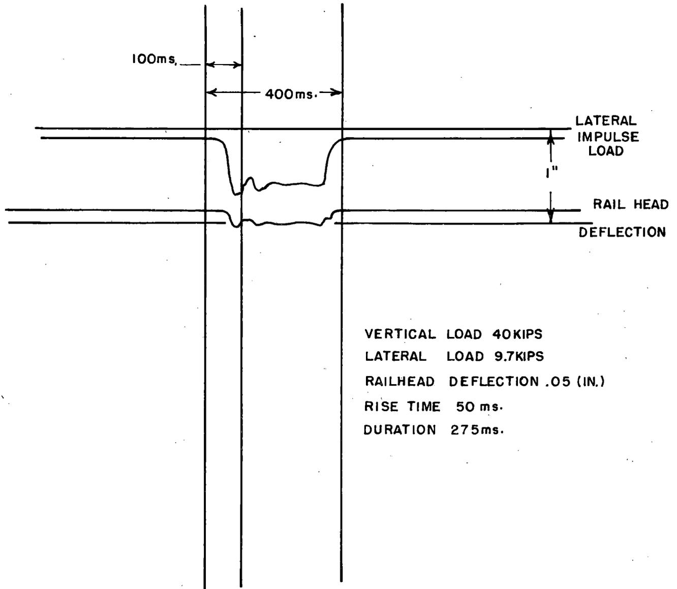
FIGURE 26. RECORDING OSCILLOGRAPH TRACE SHOWING WAVEFORMS OF 9.7 Kip LATERAL IMPULSE LOAD, AND RESULTING 0.05 INCH EAST RAILHEAD DEFLECTION, FOR A CONSTANT 40 Kip VERTICAL LOAD.
