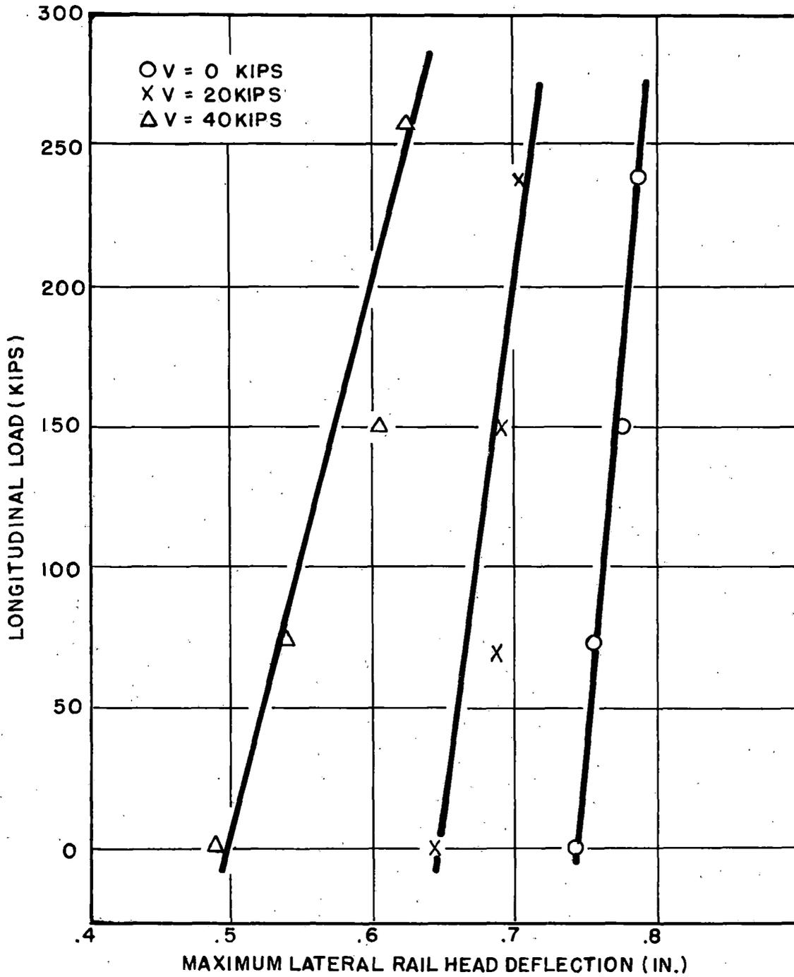
FIGURE 31. MAXIMUM LATERAL RAIL HEAD DEFLECTION VS. LONGITUDINAL LOAD, FOR VARIOUS VERTICAL LOADS AND CONSTANT 30 KIP LATERAL LOAD.
