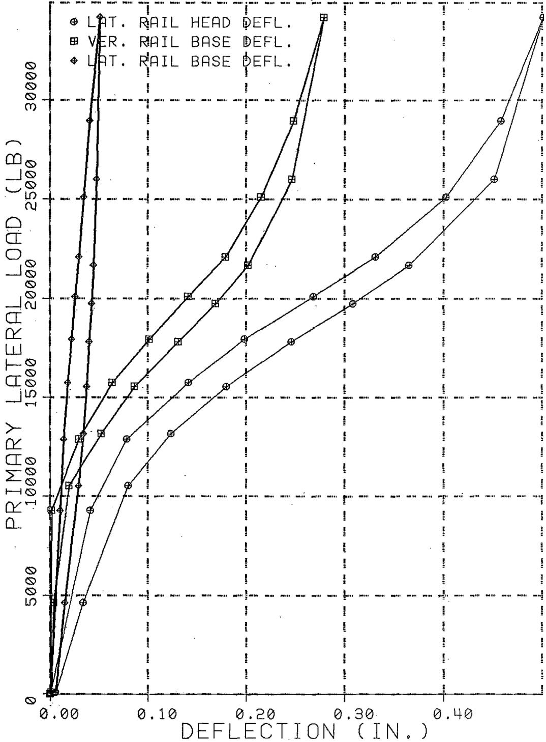
FIGURE 16. RAIL HEAD DEFLECTION VS PRIMARY LATERAL LOAD, FOR CONSTANT 20 KIP PRIMARY VERTICAL AND 10 KIP ADJACENT VERTICAL LOAD
