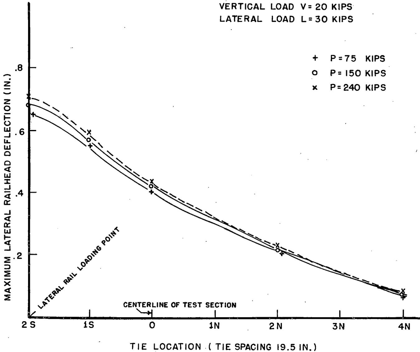
FIGURE 33. MAXIMUM LATERAL RAILHEAD DEFLECTION VS. MEASUREMENT LOCATION, FOR VARIOUS LONGITUDINAL LOADS, AND CONSTANT 20 KIP VERTICAL AND 30 KIP LATERAL LOADS.
