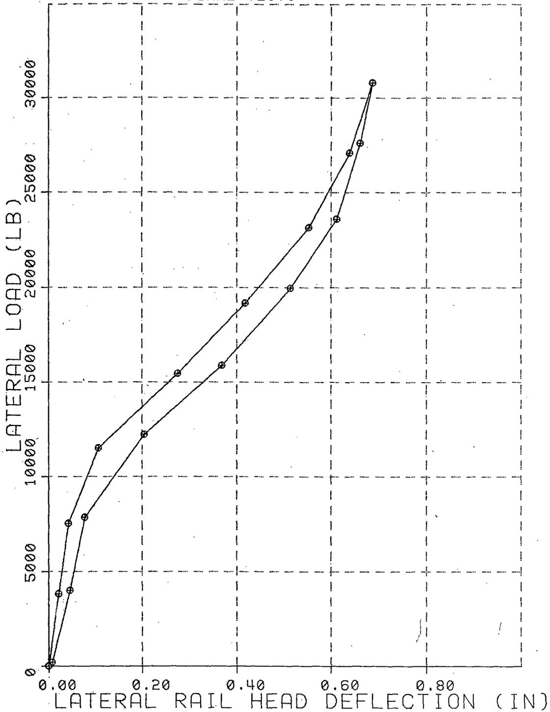
FIGURE 29. LATERAL RAIL HEAD DEFLECTION VS LATERAL LOAD, FOR CONSTANT 75 KIP LONGITUDINAL AND 20 KIP VERTICAL LOADS.
