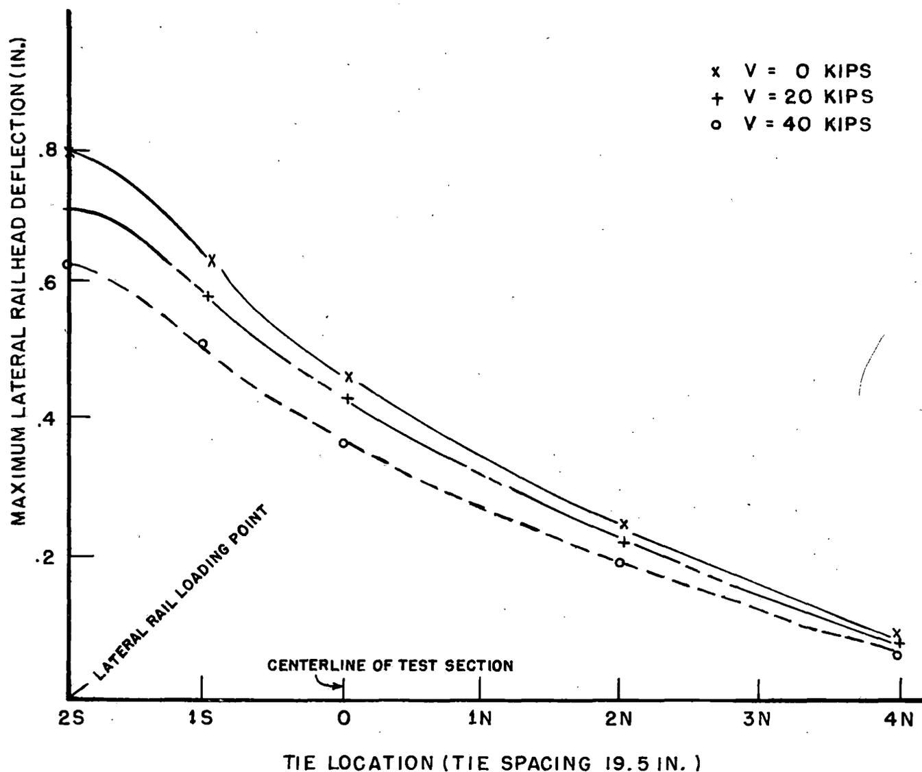
FIGURE 32. MAXIMUM LATERAL RAILHEAD DEFLECTION VS. MEASUREMENT LOCATION, FOR VARIOUS VERTICAL LOADS, AND CONSTANT 240 Kip LONGITUDINAL AND 30 Kip LATERAL LOADS.
