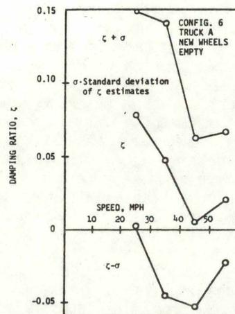
Figure 4-15. Natural Frequency and Damping Ratio Estimates from Forcer Tests
