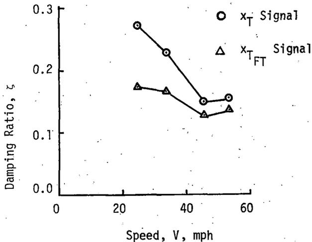
Figure 5-38. Damping Ratio versus Speed for Configuration 6 Using PSDs (Hybrid Simulation)
