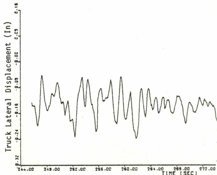
Figure 4-2. Stable Response to Track Forcing
