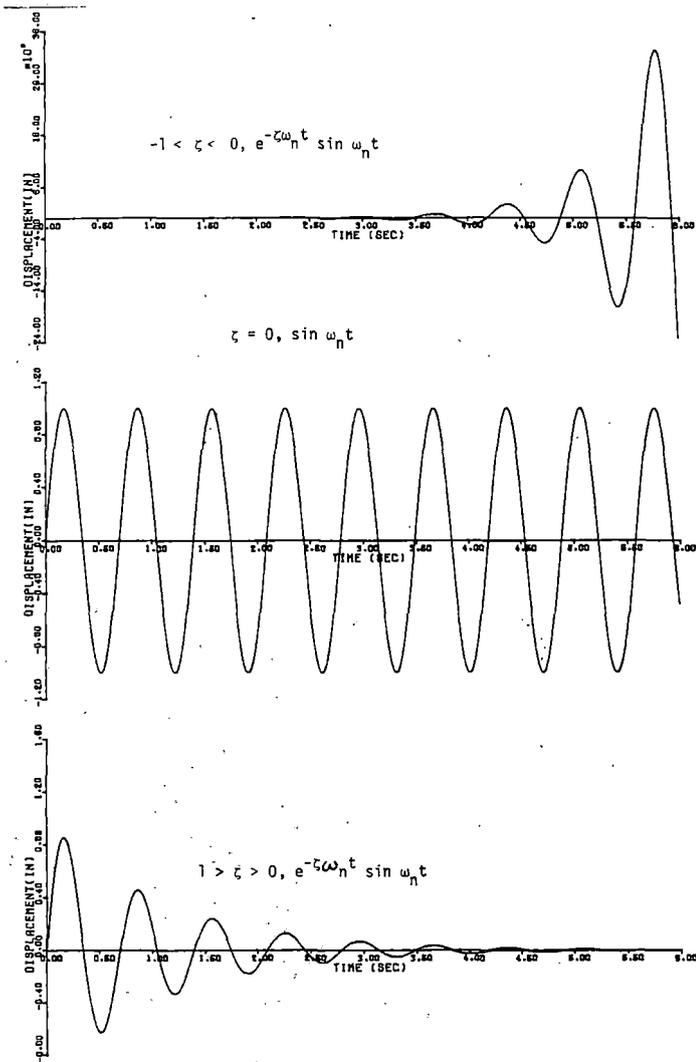
Figure 2-4. Typical System Dynamic Response
