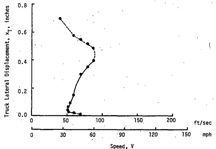
Figure 5-25. Limit Cycle Behavior of Configuration 2 Without Dither and Wheel-Rail Constraint Functions Smoothed 14 Times
