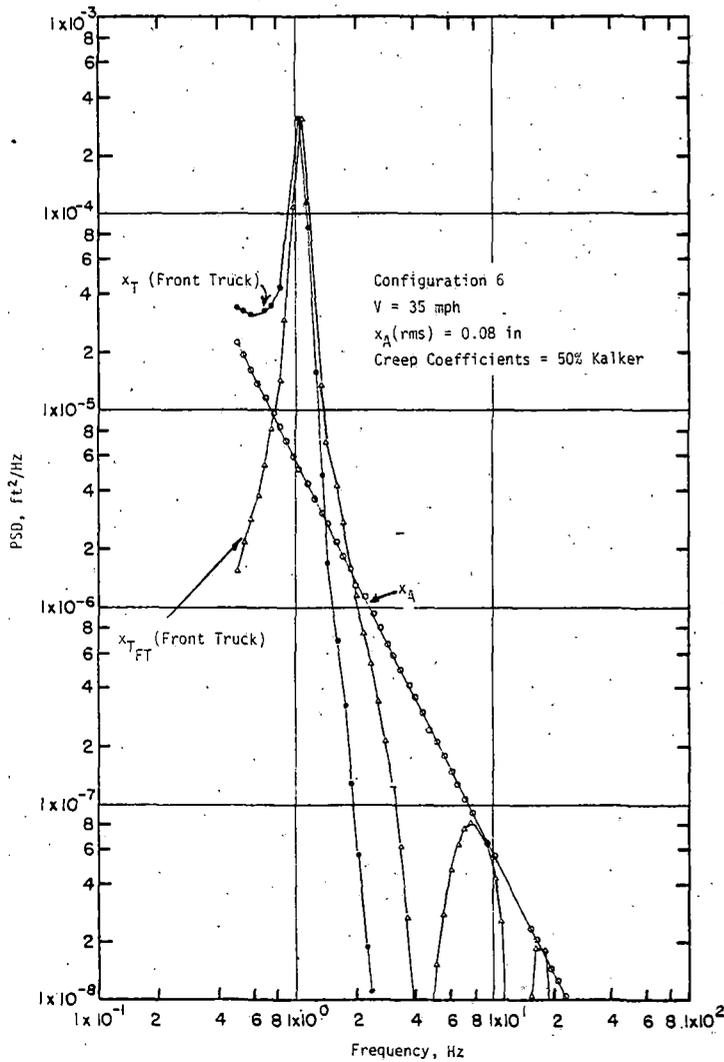
Figure 5-9. PSDs for Absolute and Relative Truck Lateral Displacement ( $x_T$  and  $x_{FT}$ , respectively)
