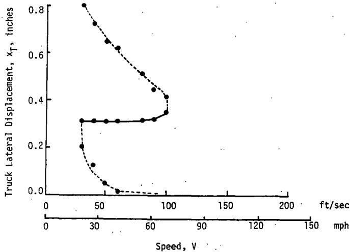
Figure 5-22. Limit Cycle Behavior of Configuration 6 With Dither and Wheel-Rail Constraint Functions Smoothed 14 Times
