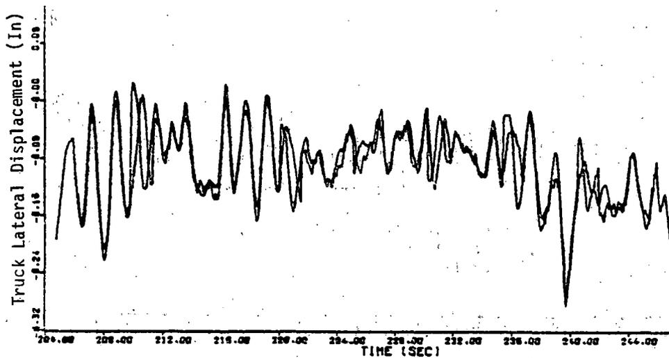
Figure 4-3. Stable Response of Trucks A and B Plotted on Same Axes
