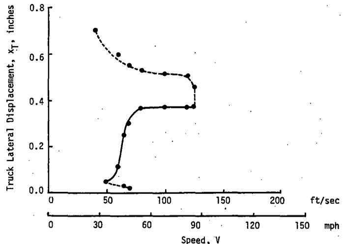
Figure 5-24. Limit Cycle Behavior of Configuration 2 With Dither and Wheel-Rail Constraint Functions Smoothed 14 Times
