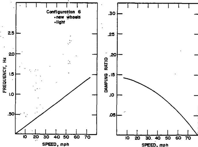
Figure 2-5. Eigenvalues for Least Damped Mode. Linear Freight Car Model.
