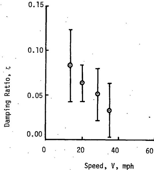
Figure 5-29. Damping Ratio versus Speed for Configuration 6 Using Log-Decrement Analysis (Hybrid Simulation).
