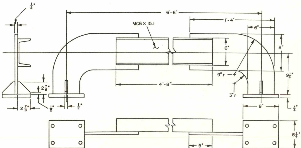
Figure 3-8. Truck Stiffener Schematic.
