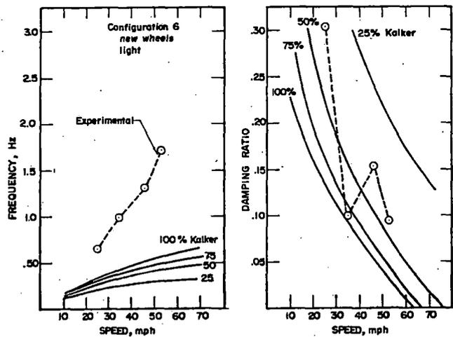
Figure 5-2. Damping Ratio and Frequency for Small Amplitude Describing Function Values
