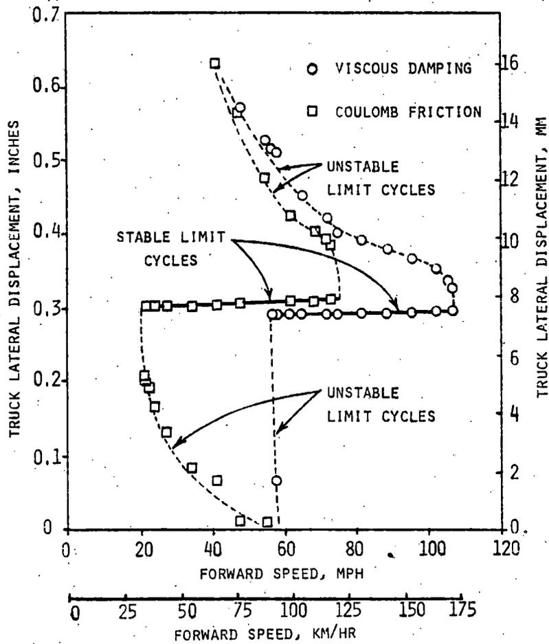
Figure 2-2. Limit Cycle Characteristics from Hybrid Simulation
