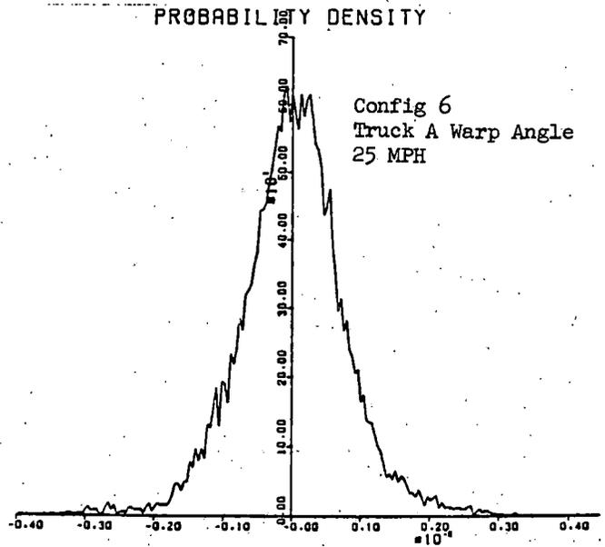
Figure 4-20. Typical Probability Density Function for Stable Behavior
