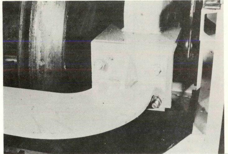
Figure 3-7. Truck Stiffener Device
