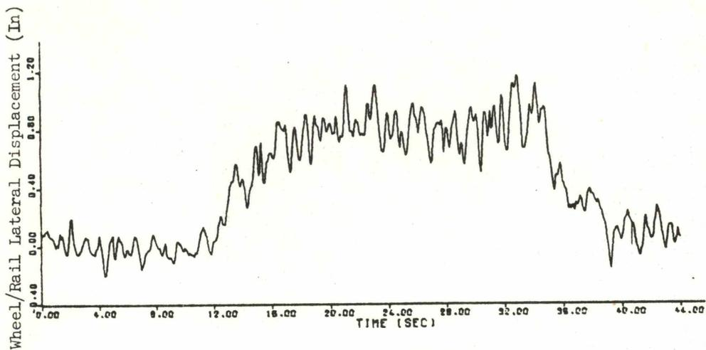
Figure 4-6. Typical Lateral Response During 6-Degree Curve Negotiation
