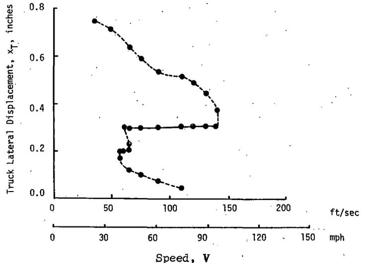
Figure 5-27. Limit Cycle Behavior of Configuration 6 with Dither and Unsmoothed Wheel-Rail Constraint Functions
