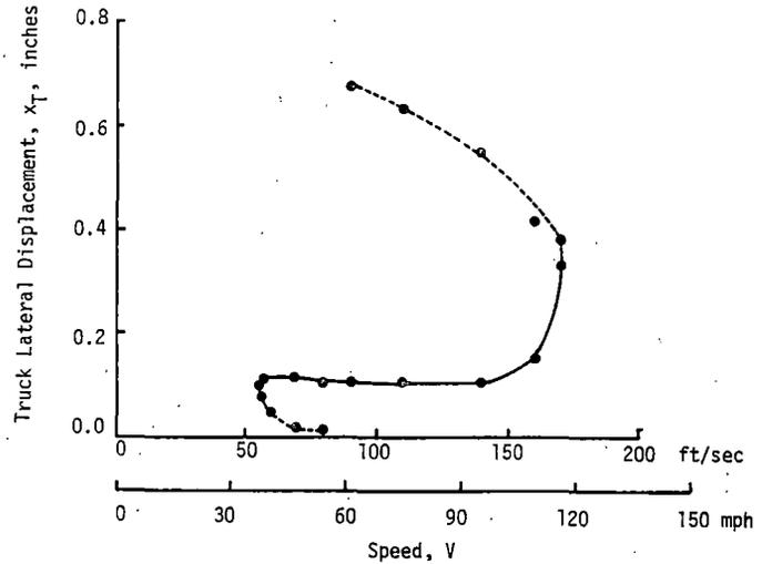
Figure 5-26. Limit Cycle Behavior of Configuration 8 With Dither and Wheel-Rail Constraint Functions Smoothed 14 Times
