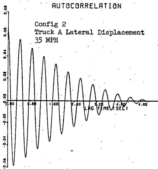
Figure 4-19. Typical Autocorrelation Function for Hunting Behavior
