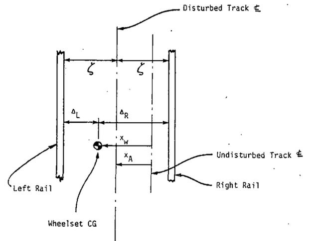
Figure 5-8. Definition of Quantities Measured by Wheel-Rail Displacement Transducers
