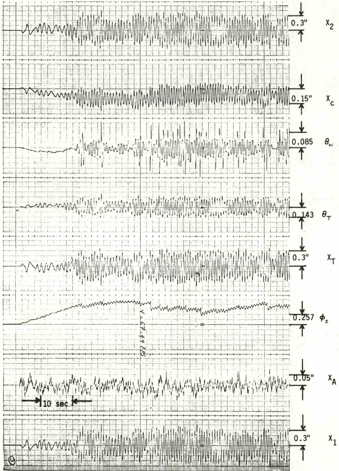
Figure 5-34. Response of Configuration 6 to Random Irregularities in Centerline Alignment at 46.0 mph (Hybrid Simulation; 0.04 inches RMS Track Centerline Alignment).
