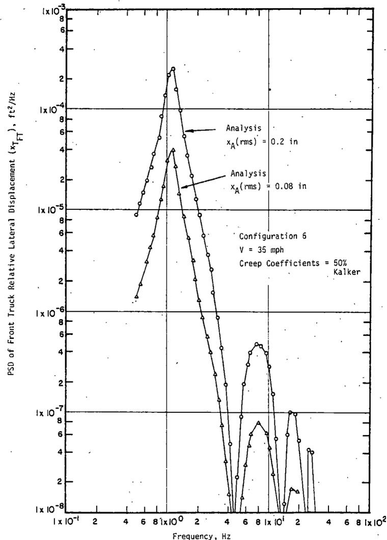
Figure 5-12. PSDs for  $x_{FT}$  at Two Levels of Alignment Input (Linear Analysis)
