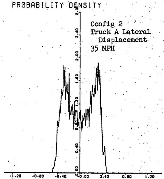
Figure 4-21. Typical Probability Density Function for Hunting Behavior
