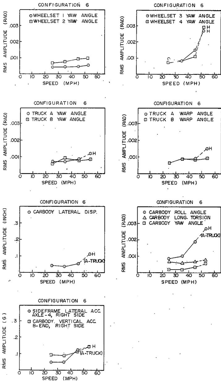
Figure 4-9. (cont) RMS Values of Model Variables
