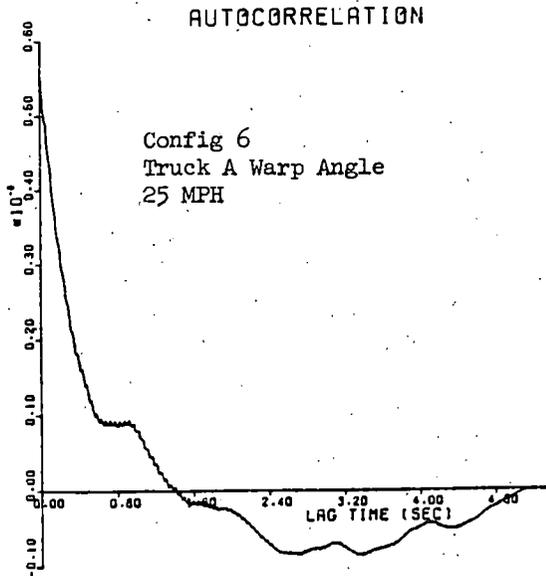
Figure 4-18. Typical Autocorrelation Function for Stable Behavior
