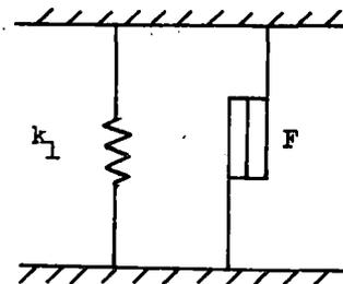
Figure 5-7. Simplified Form of Suspension Element for Nonlinear Model
