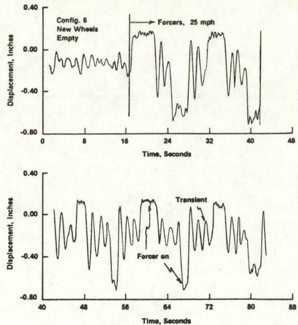
Figure 4-14. Truck Lateral Displacement Using Hydraulic Forcers
