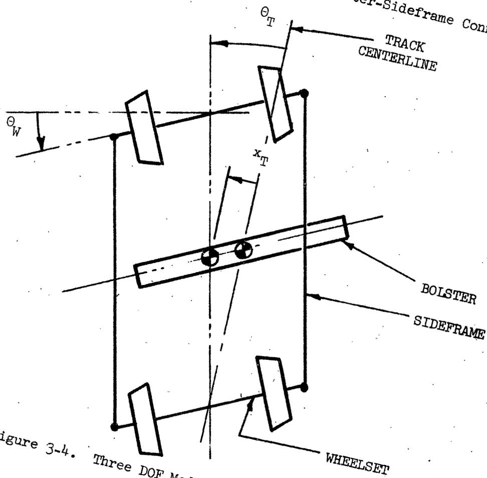
Figure 3-4. Three DOF Model for Freight Truck
