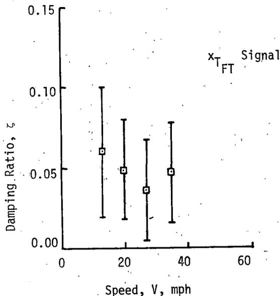
Figure 5-32. Damping Ratio Versus Speed for Configuration 6 Using Log-Decrement Analysis (Hybrid Simulation)
