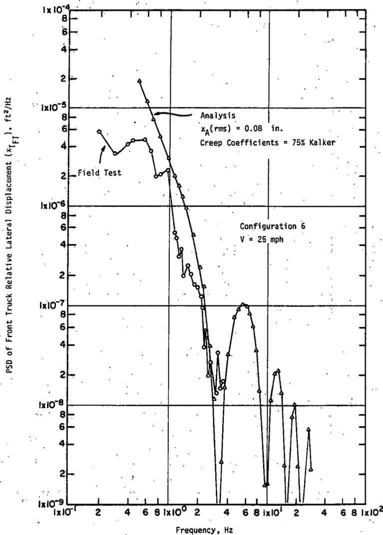
Figure 5-18. Comparison of Analysis and Test Results for Configuration 6 at 25 mph (Creep Coefficients = 75% Kalker)
