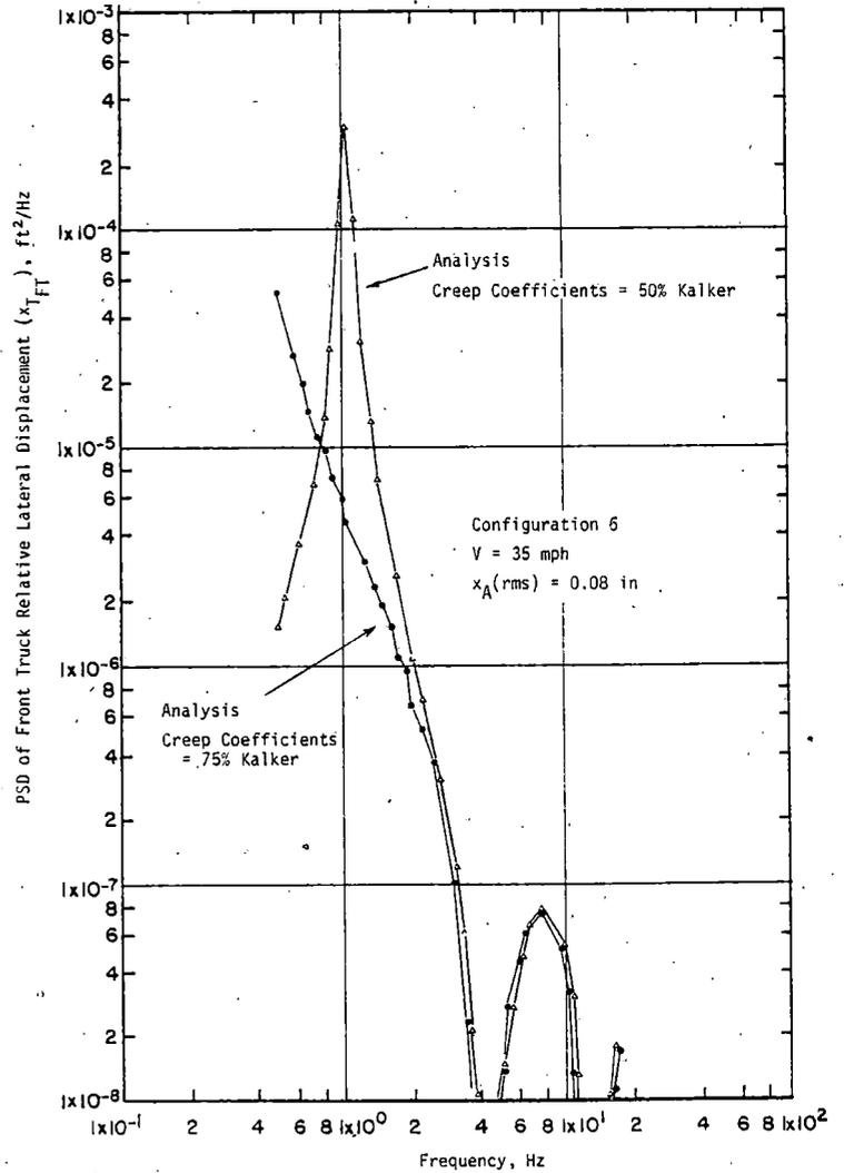
Figure 5-14. PSDs for  $x_{TFT}$  at 50 and 75% of the Nominal Kalker Creep Coefficients
