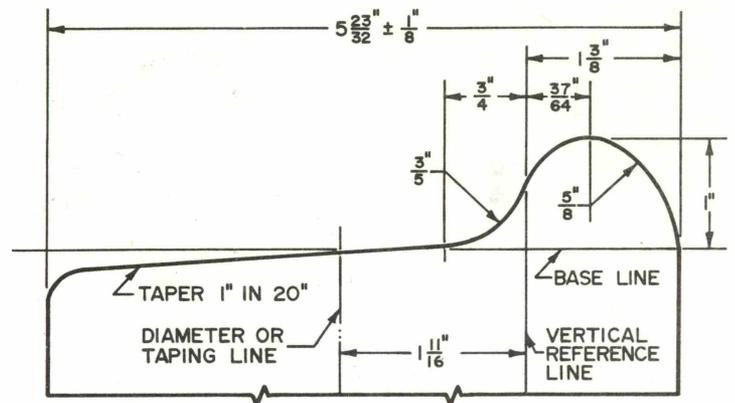
Figure 3-10. AAR Standard Tread and Flange Contour-Wide Flange Wheel.
