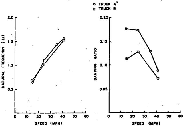
Figure 4-11. Configuration 2 Frequency and Damping Characteristics
