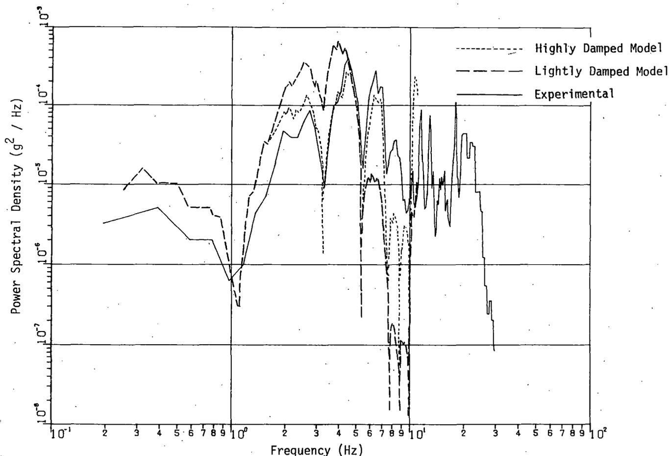
Figure 2-6. Theoretical and Experimental PSDs for Vertical Response of Refrigeration Car
