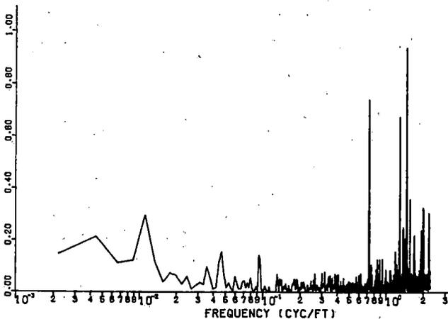
Figure 3-22. Coherence Between Alignment and Crosslevel
