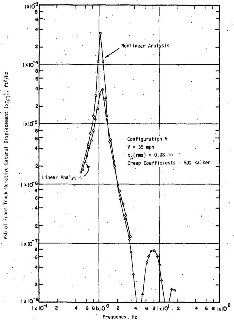
Figure 5-10. PSDs for  $x_{TFT}$  using Linear and Statistical Linearization (Nonlinear) Analyses
