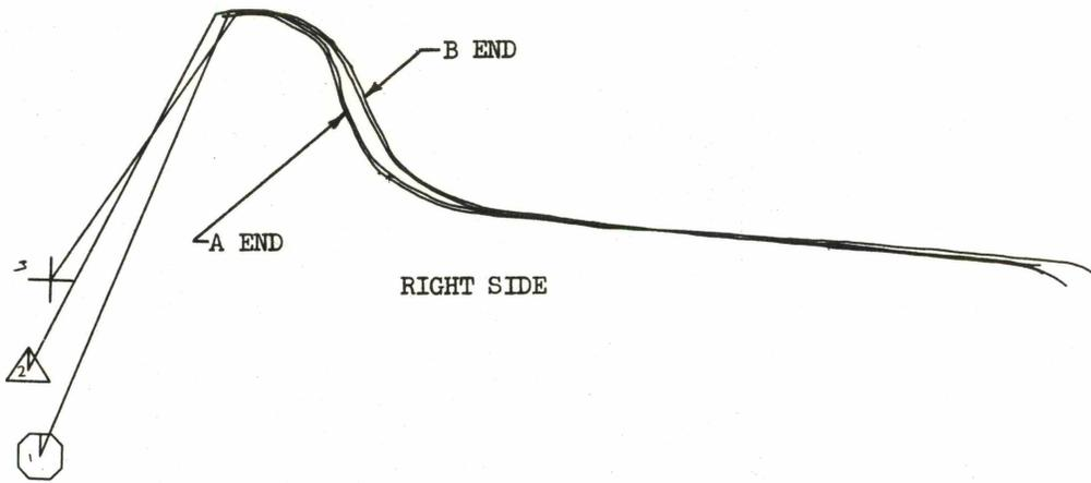
Figure 3-11. Test Vehicle Wheel Profiles, AAR Standard Profile
