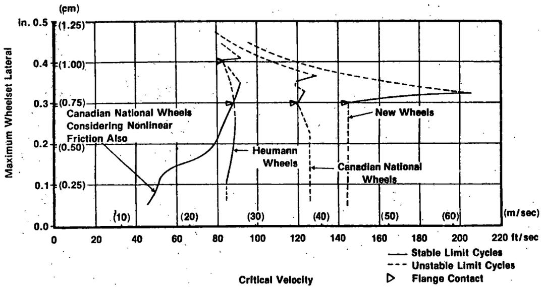
Figure 2-1. Limit Cycle Characteristics from Quasi-Linear Analysis
