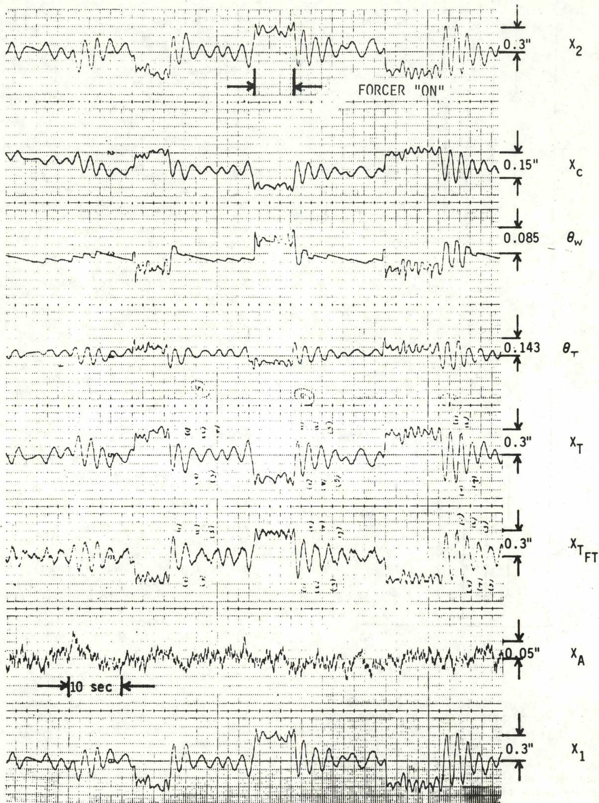
Figure 5-31. Response of Configuration 6 to Truck Forcers at 20.44 mph and Track Roughness of 0.04 inches RMS (Hybrid Simulation)
