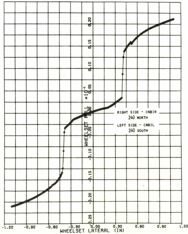
Figure 3-15. Constraint Functions for CN A Wheels
