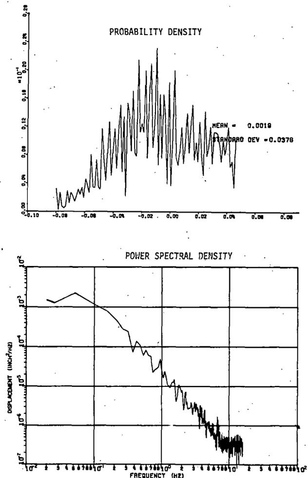
Figure 5-30. Probability Density and PSD Functions of Simulated Track Alignment Irregularities with 0.04 inches RMS Roughness for Hybrid Simulation at 27.27 mph
