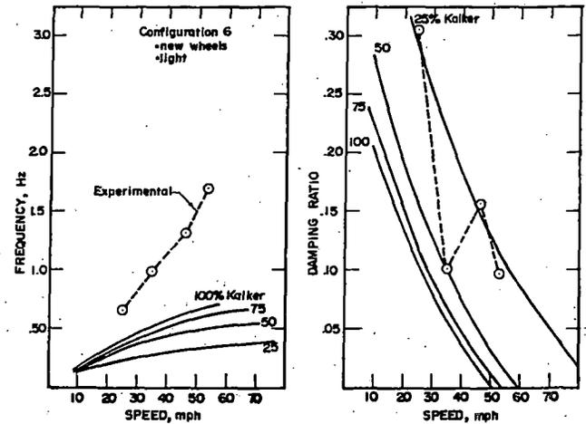
Figure 5-3. Damping Ratio and Frequency for Small Amplitude Describing Functions and Wheel Conicity of 0.075
