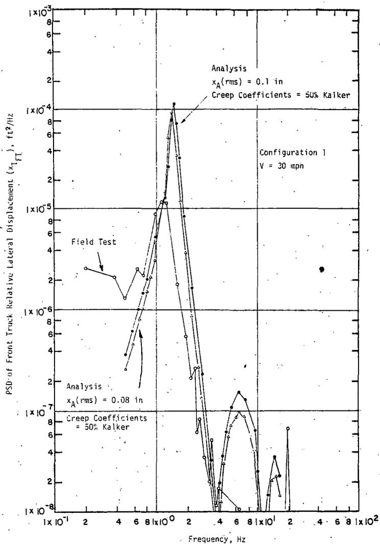
Figure 5-20. Comparison of Analysis and Test Results for Configuration 1 at 30 mph.
