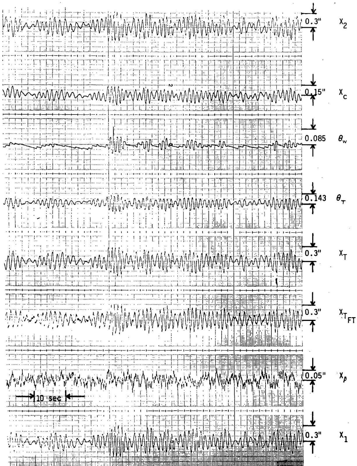
Figure 5-33. Response of Configuration 6 to Random Irregularities in Centerline Alignment at 34.3 mph (Hybrid Simulation; 0.04 inches RMS Track Centerline Alignment).
