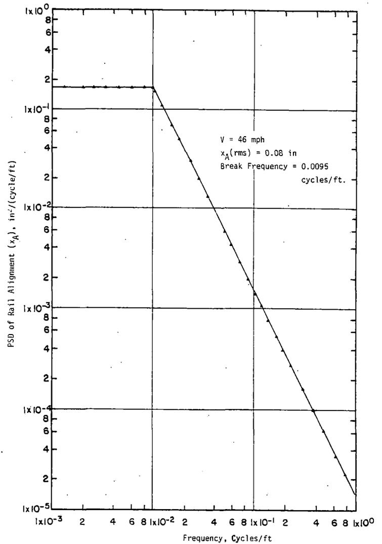
Figure 5-6. PSD of Centerline Lateral Alignment
