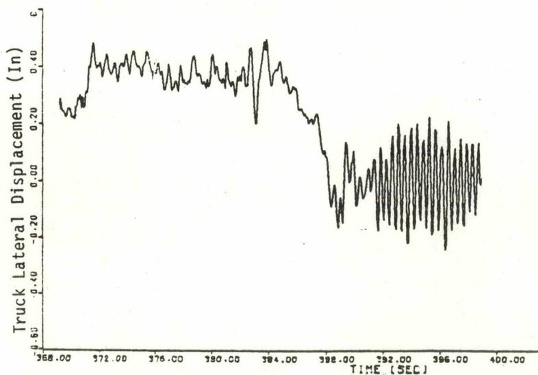
Figure 4-7. Hunting Initiated upon Exit from 6-Degree Curve at 40 MPH
