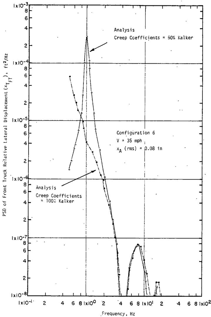
Figure 5-15. PSDs for  $x_{TFT}$  at 50 and 100% of the Nominal Kalker Creep Coefficients
