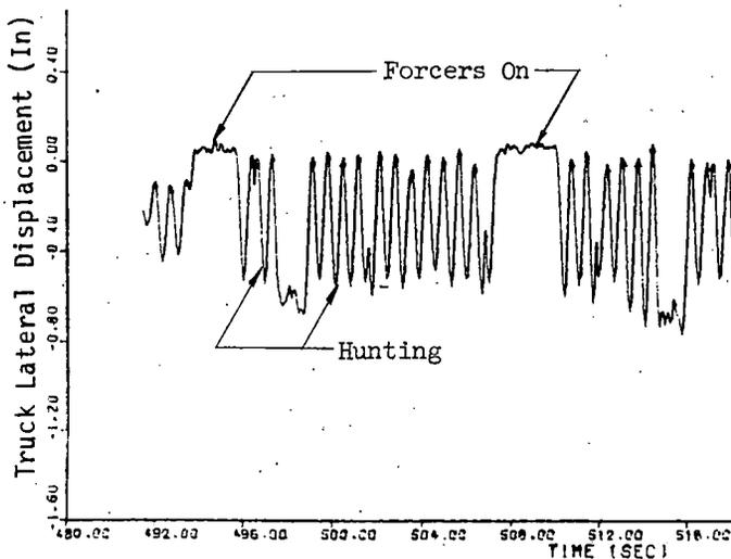
Figure 4-16. Hunting between Forcer Applications on the 45-MPH Test Run for Configuration 6
