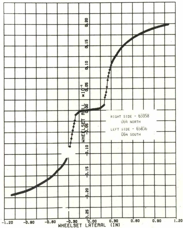
Figure 3-14. Constraint Functions for AAR Wheels
