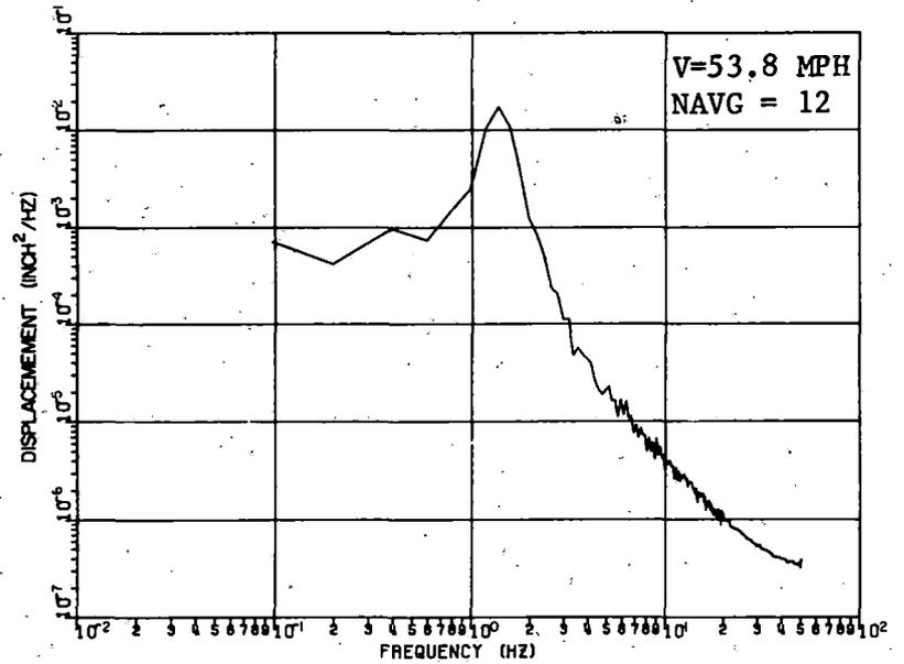
Figure 5-35. PSDs for Truck Lateral Displacement,  $x_T$ , of Configuration 6 (Hybrid Simulation; 0.04 inches RMS Track Centerline Alignment).
