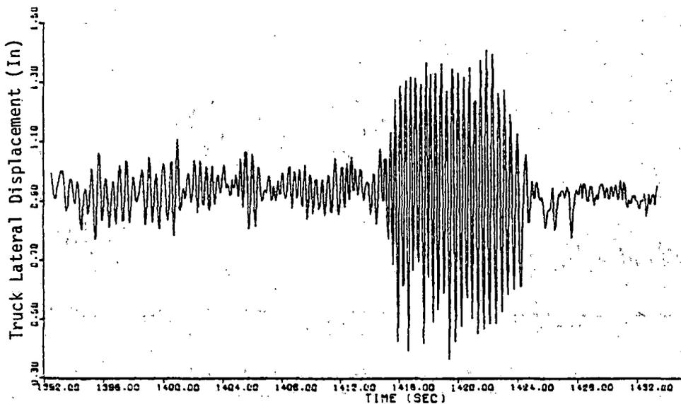
Figure 4-4. High Amplitude Intermittent Hunting
