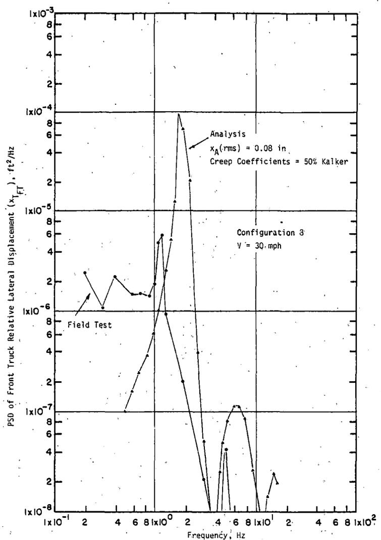
Figure 5-21. Comparison of Analysis and Test Results for Configuration 8 at 30 mph.
