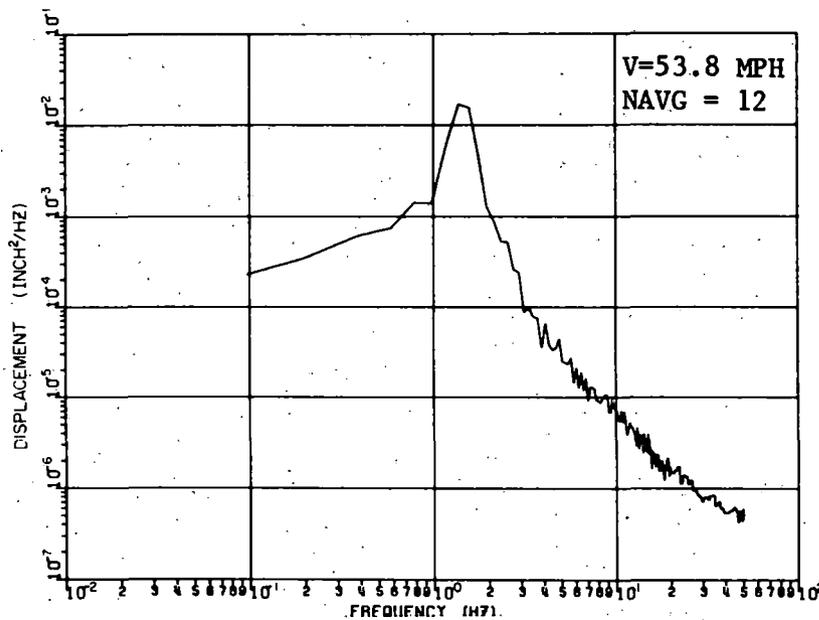
Figure 5-36. PSDs for Truck Relative Lateral Displacement,  $x_{TF}$ , of Configuration 6 (Hybrid Simulation; 0.04 inches RMS Track Centerline Alignment).
