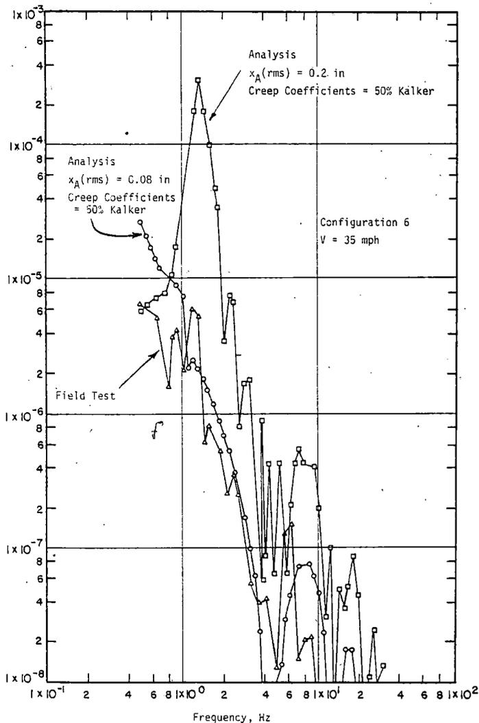
Figure 5-13. PSDs for  $x_{TFT}$  of the Rear Truck at Two Levels of Alignment Input (Nonlinear Analysis)
