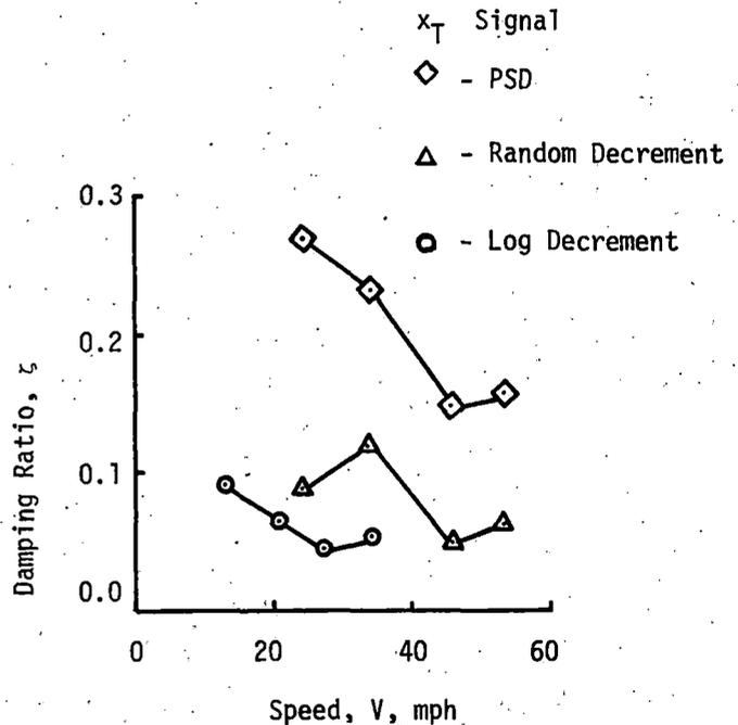
Figure 5-39. Comparison of Damping Ratio Versus Speed Characteristics of Configuration 6 as Determined by PSD, Random Decrement and Log-Decrement Analyses (Hybrid Simulation Results)
