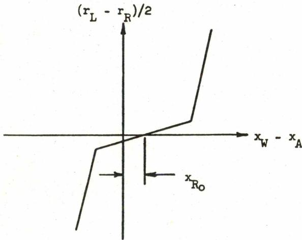
Figure 3-16. Rolling Line Offset Illustration
