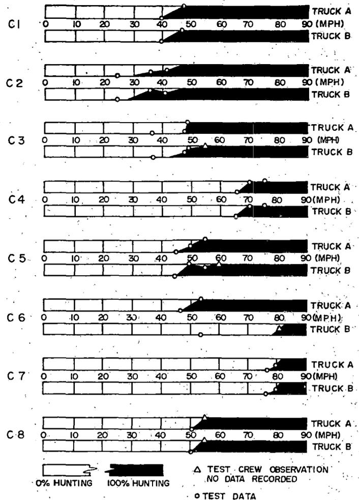
Figure 4-8. Test Vehicle Hunting Characteristics
