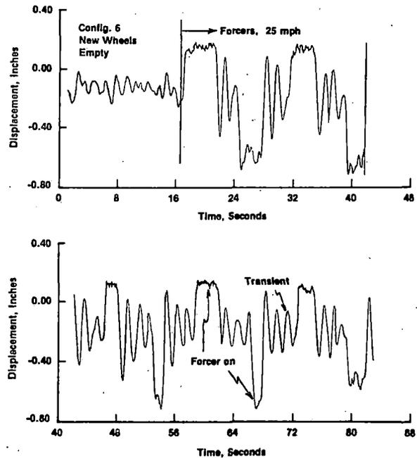
Figure 3-24. Truck Lateral Displacement Using Hydraulic Forcers
