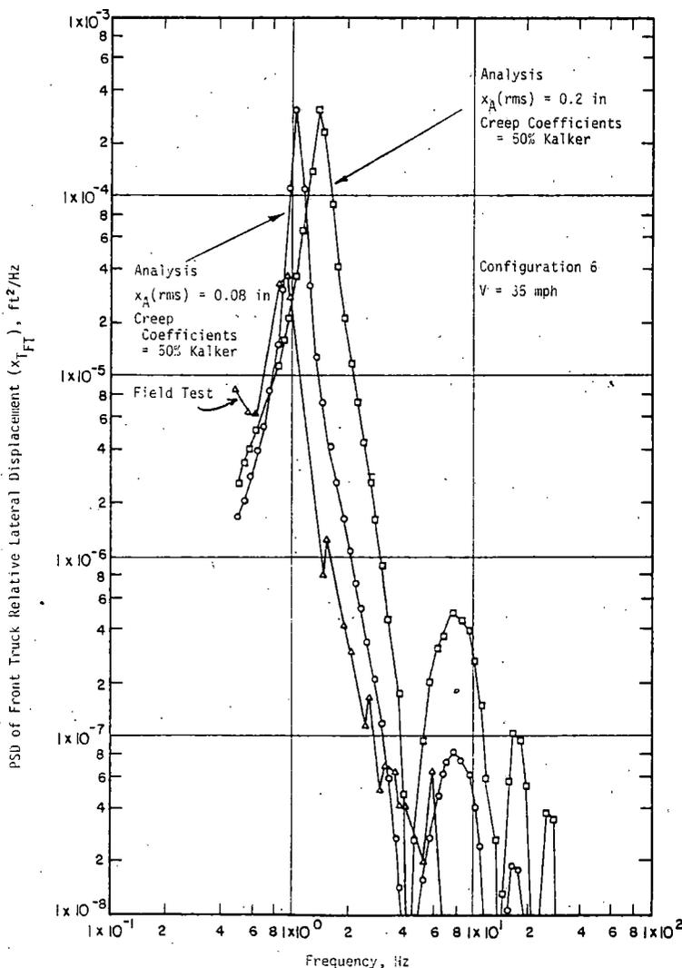
Figure 5-11. PSDs for  $x_{FT}$  of the Front Truck at Two Levels of Alignment Input (Nonlinear Analysis).
