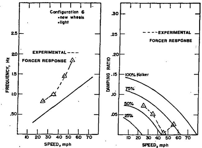
Figure 5-5. Comparison of Theoretical Results and "Forcer" Experimental Data
