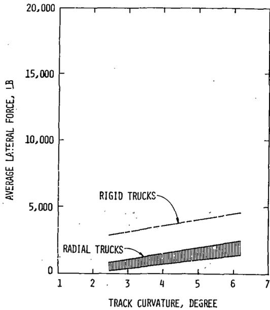
FIGURE 6.3.3-9 LATERAL FORCE ON LEADING OUTER WHEEL FOR TYPE II FREIGHT CAR TRUCK WITH EMPTY OPEN HOPPER CARS AT BALANCE SPEED (+ 2.5 MPH)
