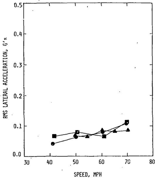
FIGURE 5.3.4-18 RMS LATERAL ACCELERATION VERSUS SPEED - 0-20 HZ FREQUENCY BAND/LOADED CARS/RIGID TRUCKS
