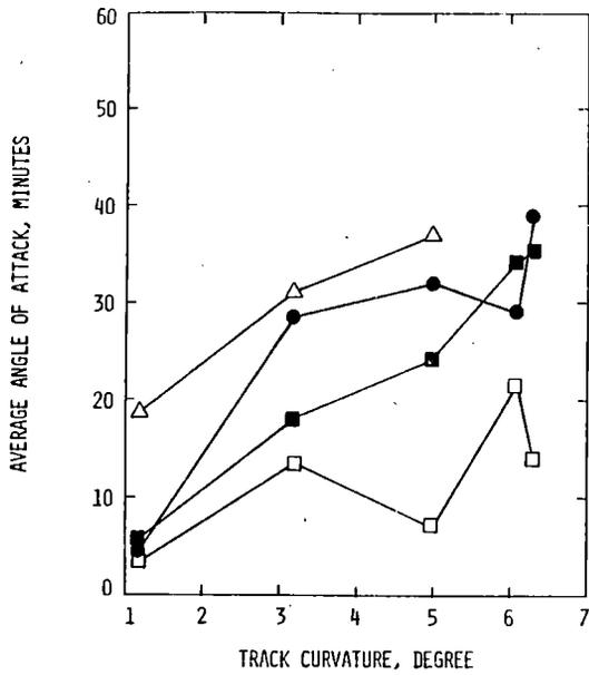
FIGURE A-25. AVERAGE ANGLE OF ATTACK VERSUS DEGREE OF CURVATURE NEAR BALANCE SPEED - RH CURVES, EMPTY CARS
