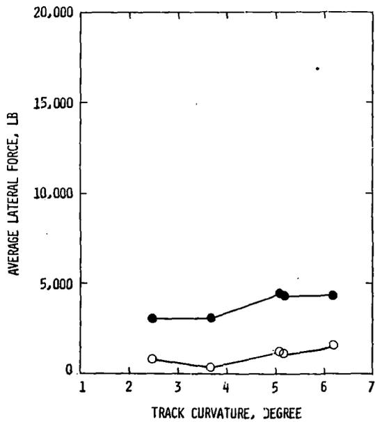
FIGURE 5.3.3-15 LATERAL FORCE ON LEADING OUTER WHEEL VERSUS DEGREE OF CURVATURE NEAR BALANCE SPEED - LEFT HAND CURVES - PRIMARY SUSPENSION TRUCKS/EMPTY HOPPER CARS
