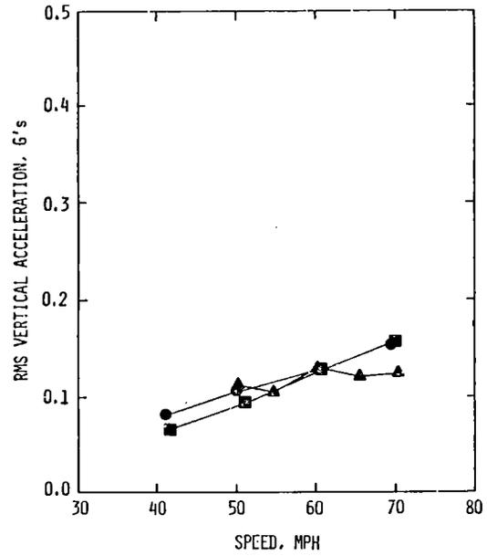
FIGURE 5.3.4-9 RMS VERTICAL ACCELERATION VERSUS SPEED - 0-20 HZ FREQUENCY BAND/LOADED CARS/RIGID TRUCKS
