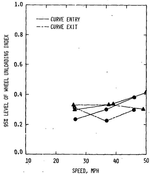
FIGURE 5.3.2-30 95% LEVEL OF WHEEL UNLOADING INDEX VERSUS SPEED - RIGID TRUCKS/EMPTY CARS/6.2° CURVE
