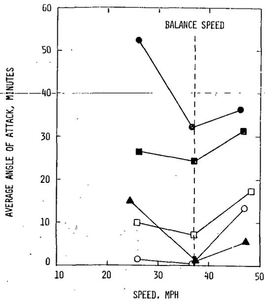
FIGURE A-13. AVERAGE ANGLE OF ATTACK VERSUS SPEED - 5.0° RH CURVE, EMPTY CARS
