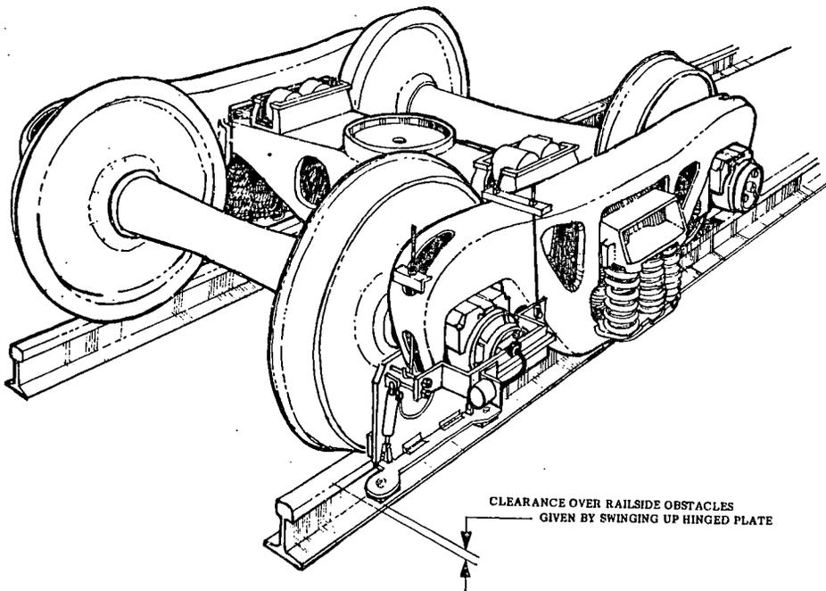
FIGURE A-2. WHEEL TO RAIL DISPLACEMENT MEASUREMENT
