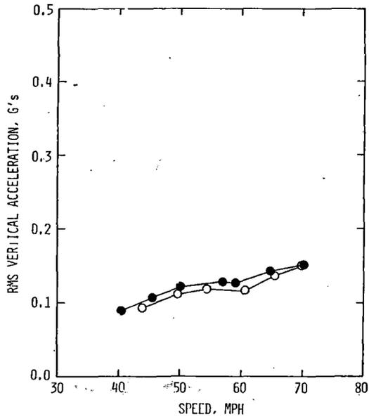
FIGURE 5.3.4-1 RMS VERTICAL ACCELERATION VERSUS SPEED - 0-20 HZ FREQUENCY BAND/EMPTY CARS/PRIMARY SUSPENSION TRUCKS
