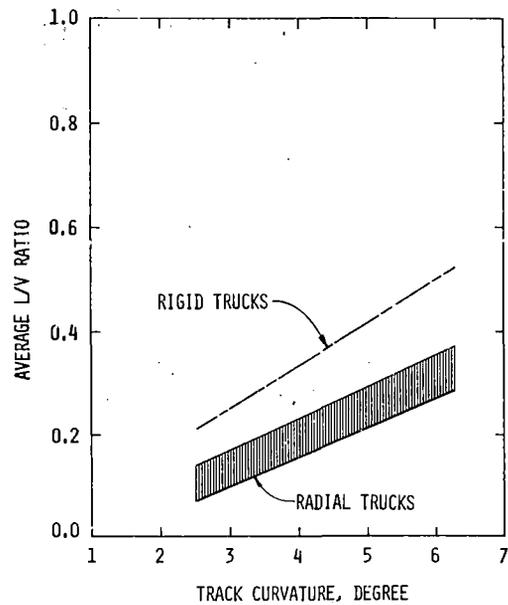
FIGURE 6.3.3-20 L/V RATIO ON LEADING OUTER WHEEL FOR TYPE II FREIGHT CAR TRUCKS WITH LOADED OPEN HOPPER CARS AT BALANCE SPEED (+ 2.5 MPH)
