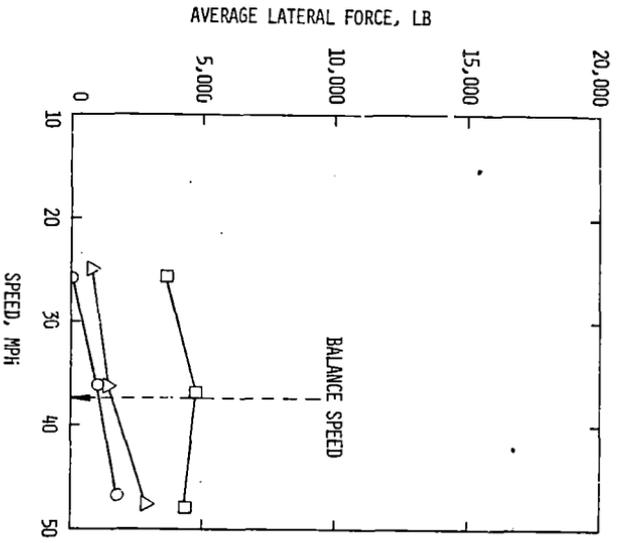
FIGURE 5.3.3-35 LATERAL FORCE ON LEADING OUTER WHEEL
