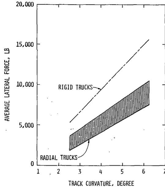
FIGURE 6.3.3-10 LATERAL FORCE ON LEADING OUTER WHEEL FOR TYPE II FREIGHT CAR TRUCK WITH LOADED OPEN HOPPER CARS AT BALANCE SPEED (+ 2.5 MPH)
