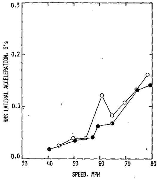
FIGURE 5.3.1-37 RMS LATERAL ACCELERATION AT LEADING AXLE/LEADING TRUCK VERSUS SPEED - PRIMARY SUSPENSION TRUCKS/EMPTY CARS
