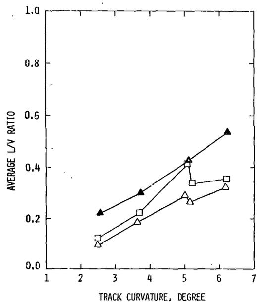
FIGURE 5.3.3-76 L/V RATIO ON LEADING OUTER WHEEL VERSUS DEGREE OF CURVATURE NEAR BALANCE SPEED - LEFT HAND CURVES - SECONDARY SUSPENSION TRUCKS/LOADED HOPPER CARS
