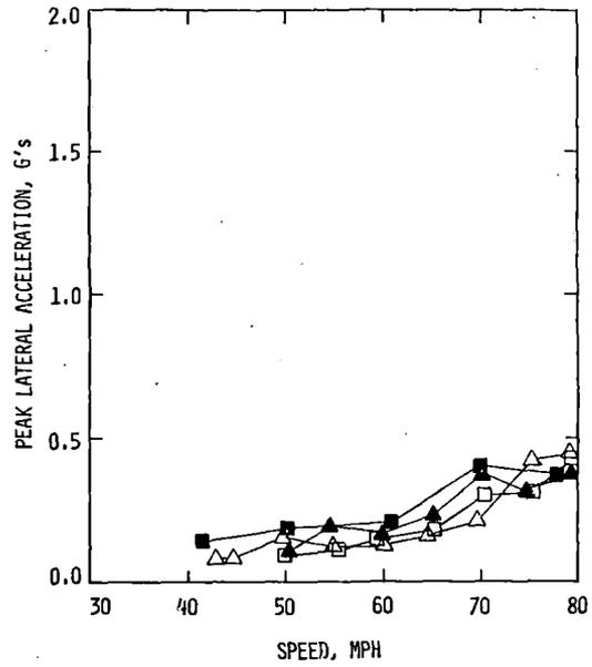
FIGURE 5.3.1-27 PEAK LATERAL ACCELERATION AT CARBODY CENTER/SILL LEVEL VERSUS SPEED - SECONDARY SUSPENSION TRUCKS/LOADED CARS
