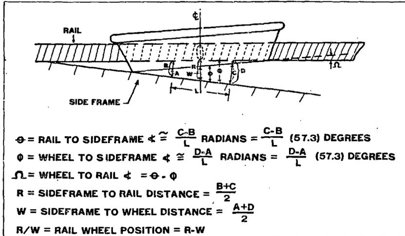
FIGURE A-3. WHEEL/RAIL POSITION MEASUREMENT
