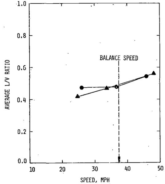
FIGURE 5.3.3-48 L/V RATIO ON LEADING OUTER WHEEL VERSUS SPEED - 5.2 CURVE/RIGID TRUCKS/EMPTY HOPPER CARS
