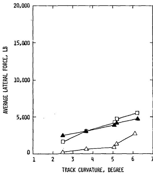
FIGURE 5.3.3-16 LATERAL FORCE ON LEADING OUTER WHEEL VERSUS DEGREE OF CURVATURE NEAR BALANCE SPEED - LEFT HAND CURVES - SECONDARY SUSPENSION TRUCKS/EMPTY HOPPER CARS
