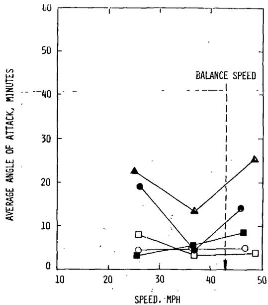
FIGURE A-5. AVERAGE ANGLE OF ATTACK VERSUS SPEED - 1.1° RH CURVE, EMPTY CARS
