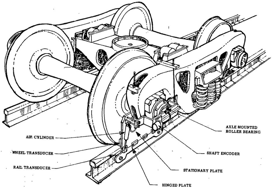
FIGURE A-1. WHEEL TO RAIL DISPLACEMENT MEASUREMENT
