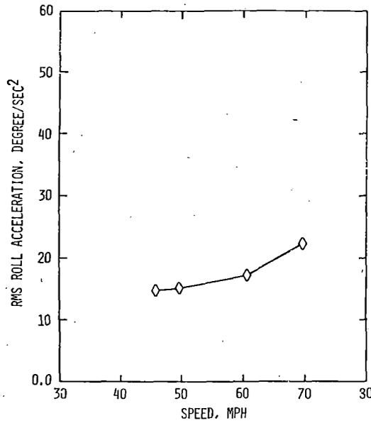
FIGURE 5.3.4-23 RMS ROLL ACCELERATION VERSUS SPEED - 0-20 HZ FREQUENCY BAND/LOADED CARS/ PRIMARY + SECONDARY SUSPENSION TRUCKS
