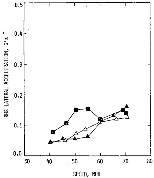
FIGURE 5.3.4-11 RMS LATERAL ACCELERATION VERSUS SPEED - 0-20 HZ FREQUENCY BAND/EMPTY CARS/SECONDARY SUSPENSION TRUCKS
