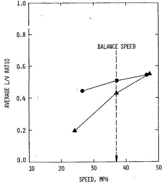
FIGURE 5.3.3-46 L/V RATIO ON LEADING OUTER WHEEL VERSUS SPEED - 5.1 CURVE/RIGID TRUCKS/EMPTY HOPPER CARS
