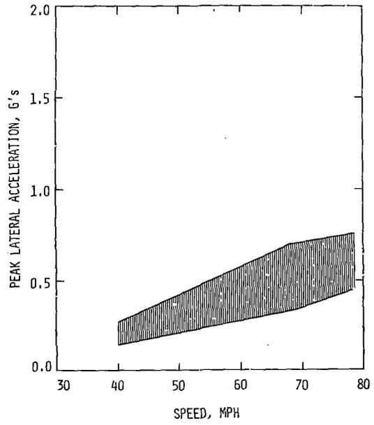
FIGURE 6.3.1-4 PEAK LATERAL ACCELERATION LEVELS FOR TYPE II FREIGHT CAR TRUCKS WITH LOADED OPEN HOPPER CARS
