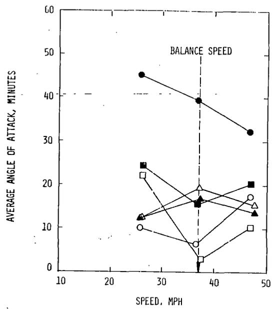
FIGURE A-14. AVERAGE ANGLE OF ATTACK VERSUS SPEED - 5.0° RH CURVE, LOADED CARS
