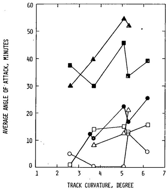
FIGURE A-27. AVERAGE ANGLE OF ATTACK VERSUS DEGREE OF CURVATURE NEAR BALANCE SPEED - LH CURVES, EMPTY CARS
