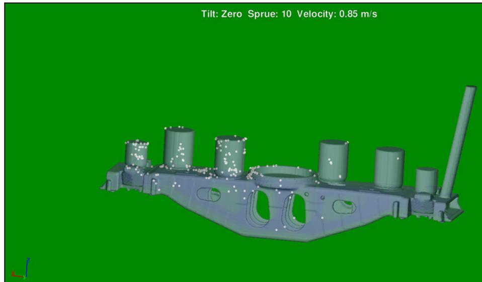
**Figure 14. Mold Angle: 0° Sprue Angle: 10° Initial Velocity: 0.85 m/s**
