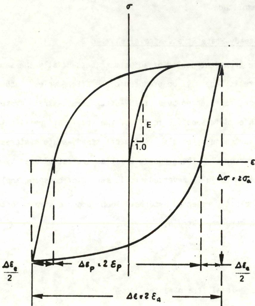
Figure C.3 SCHEMATIC OF A STEADY-STATE STRESS-STRAIN HYSTERESIS LOOP
