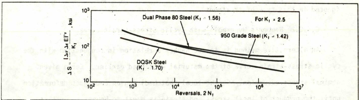
Figure C.12 NEUBER PLOTS OF NOTCHED FATIGUE-TEST DATA
