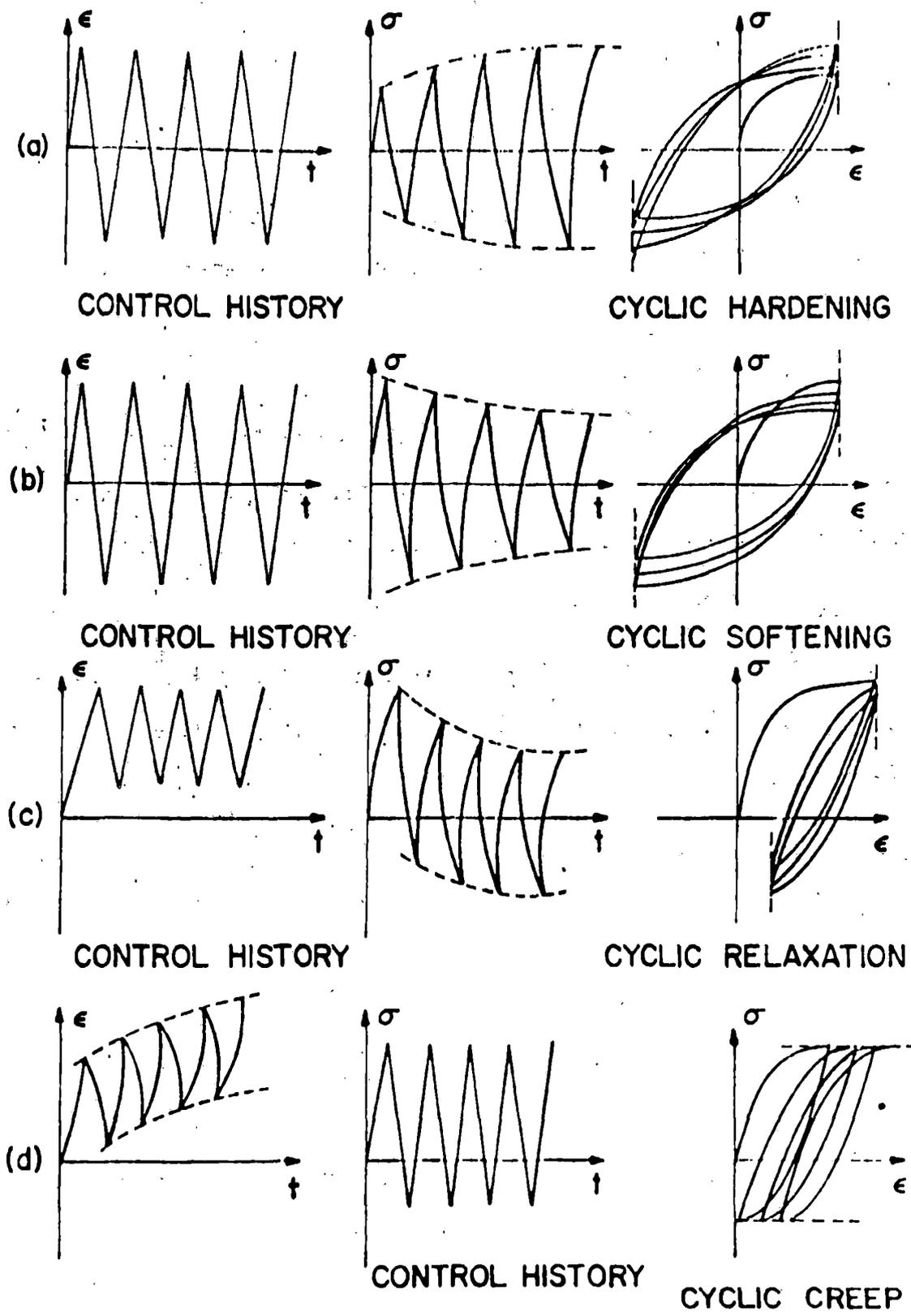
Figure C.2 SCHEMATIC ILLUSTRATIONS OF CYCLIC TRANSIENT PHENOMENA
