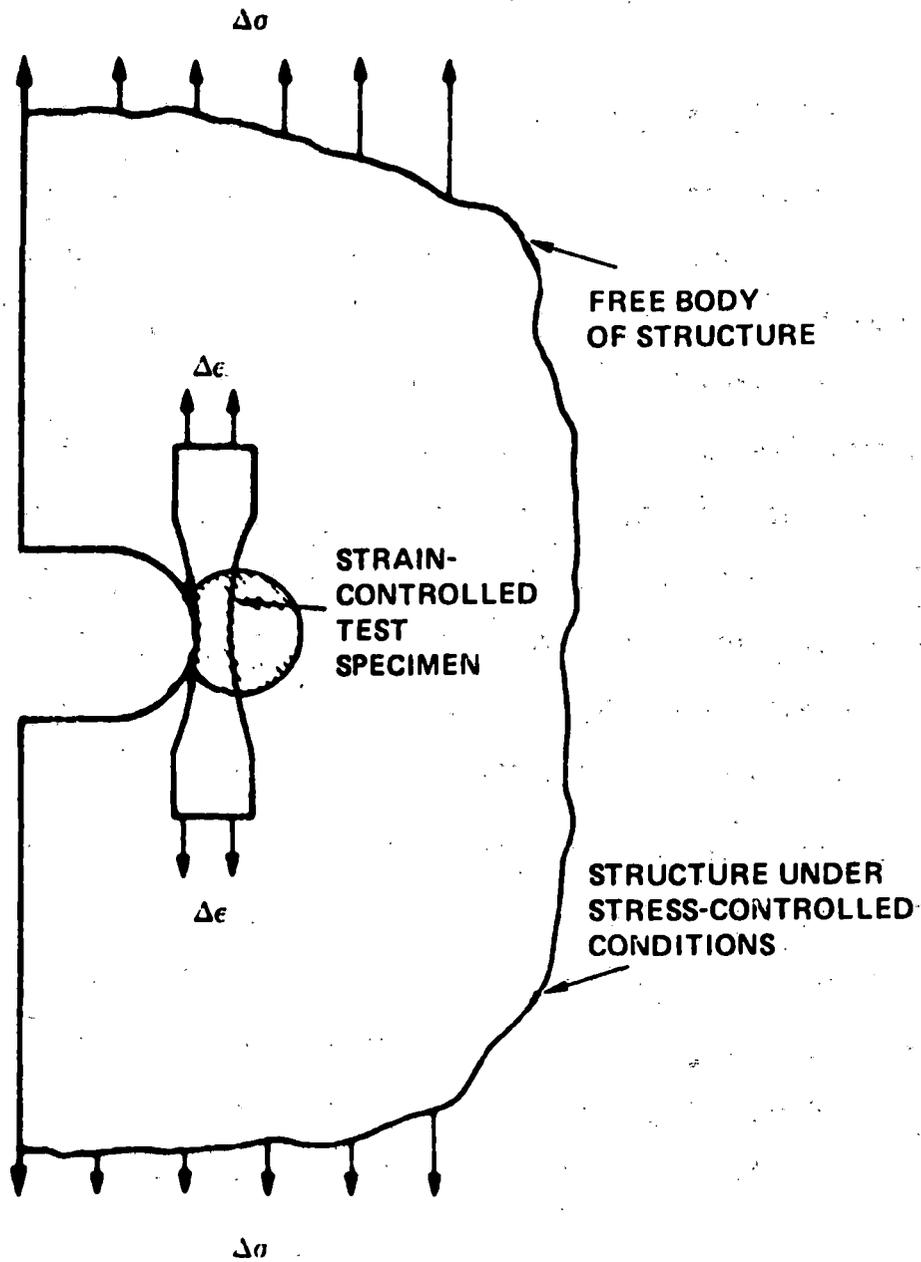
Figure C.1 STRAIN-CONTROLLED TEST SPECIMEN SIMULATION FOR STRESS CONCENTRATIONS IN STRUCTURES.
