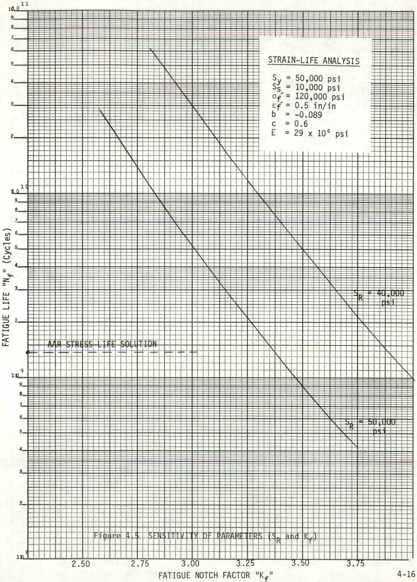
Figure 4.5 SENSITIVITY OF PARAMETERS ( $S_R$  and  $K_f$ )
