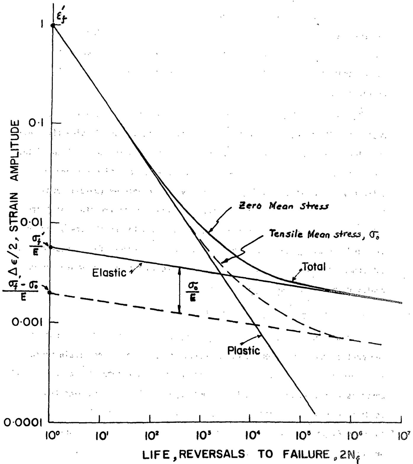
Figure C.11 STRAIN-LIFE CURVE WITH MEAN STRESS MODIFICATION
