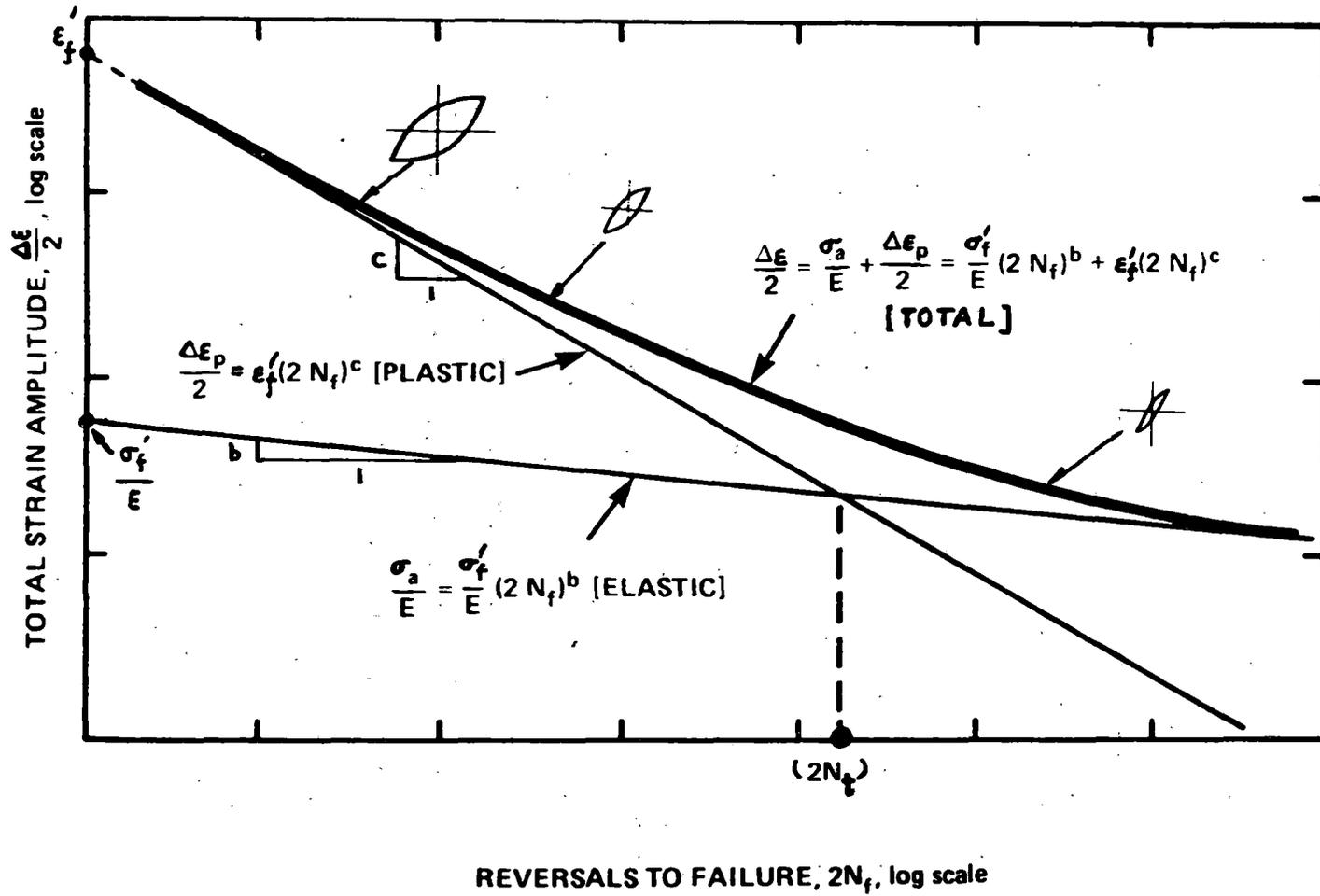
Figure C.9 STRAIN-(FATIGUE) LIFE RELATIONSHIP
