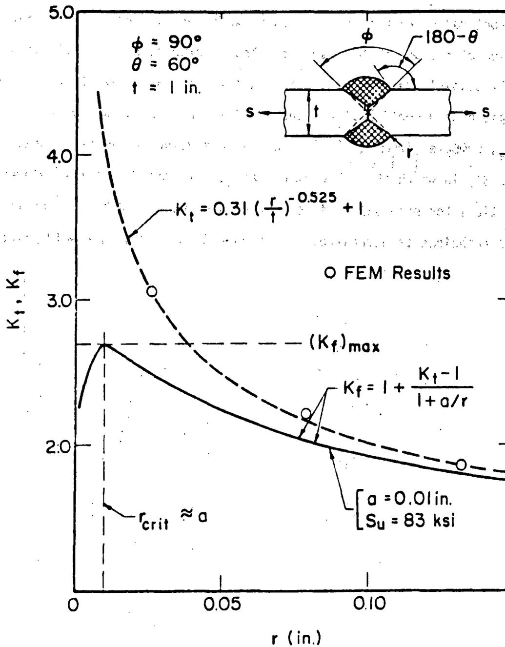
Figure C.18 ELASTIC STRESS CONCENTRATION FACTOR ( $K_t$ ) AND FATIGUE NOTCH FACTOR ( $K_f$ ) AS A FUNCTION OF TOE ROOT RADIUS
