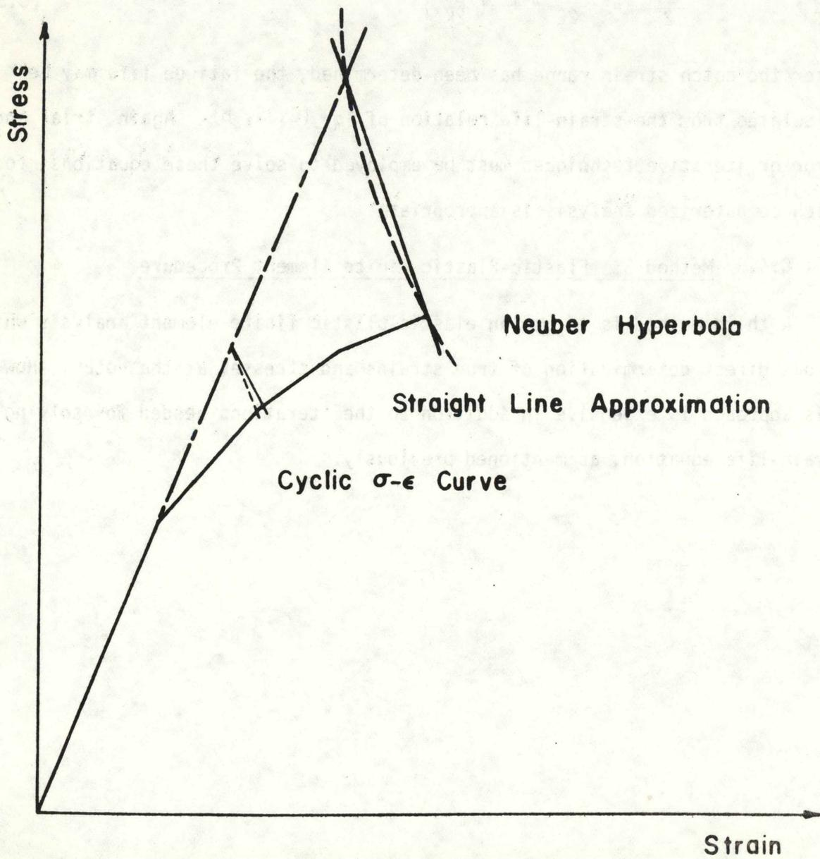
Figure C.14 CONSTRUCTION FOR DETERMINING NOTCH ROOT STRESS AND STRAIN
