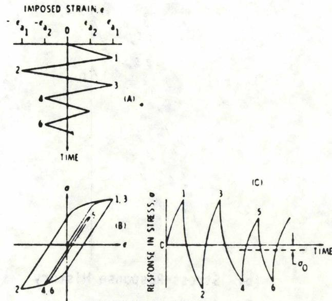
Figure 3.11 DEVELOPMENT OF COMPRESSIVE MEAN STRESS BECAUSE OF SEQUENCE EFFECT
