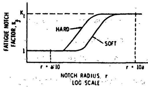
Figure C.16 FATIGUE-NOTCH FACTOR VERSUS NOTCH RADIUS AS A FUNCTION OF RELATIVE HARDNESS
