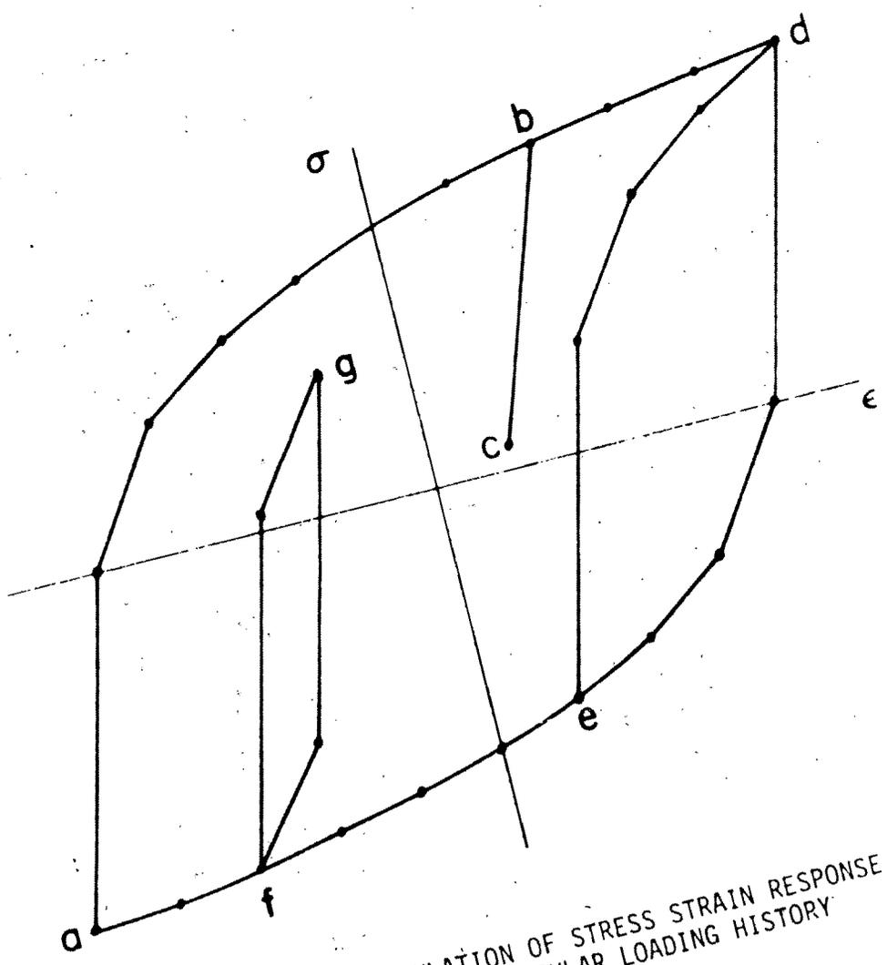
Figure 3.7 SIMULATION OF STRESS STRAIN RESPONSE FOR AN IRREGULAR LOADING HISTORY
