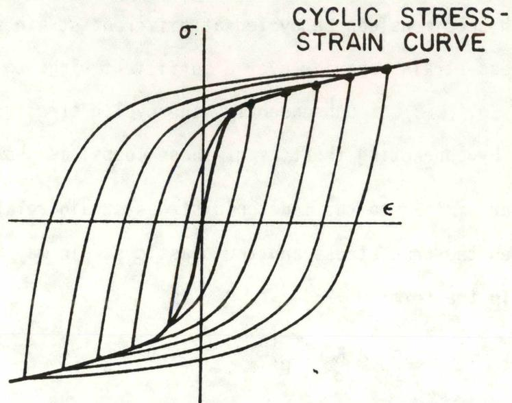
Figure C.4 STEADY-STATE STRESS-STRAIN LOOPS AND CONSTRUCTION OF CYCLIC STRESS-STRAIN CURVE
