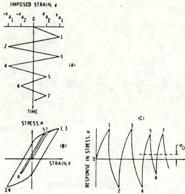
Figure 3.10 DEVELOPMENT OF TENSILE MEAN STRESS BECAUSE OF SEQUENCE EFFECT
