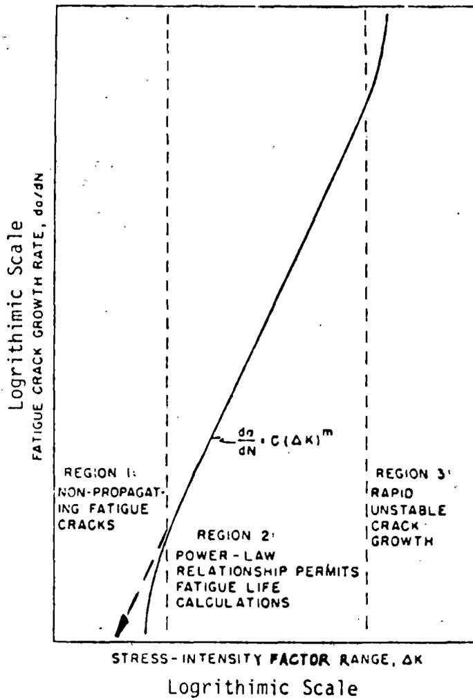
Figure 2.5 SCHEMATIC OF TYPICAL CRACK GROWTH DATA
