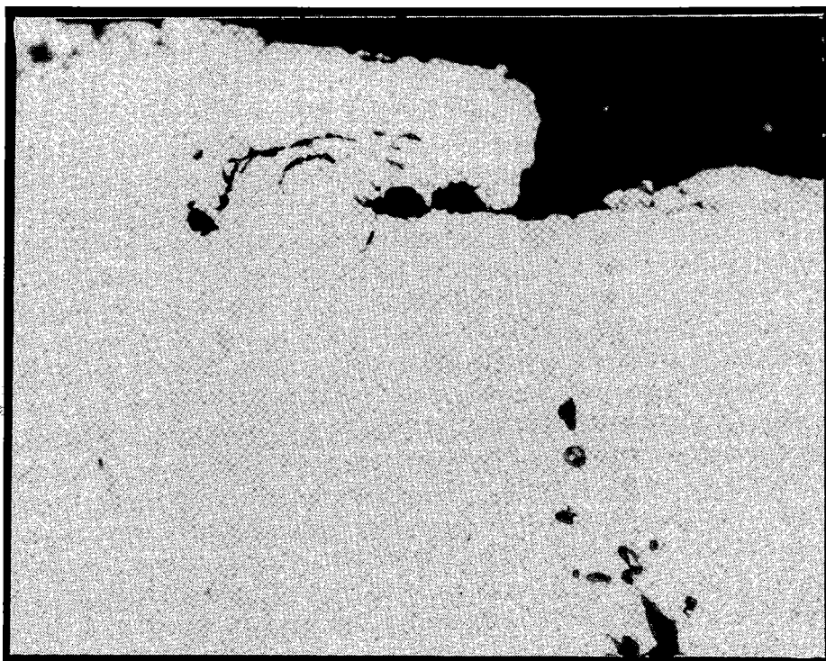
Figure 22. Optical Micrograph of Transverse Section through Shell in Figure 20
