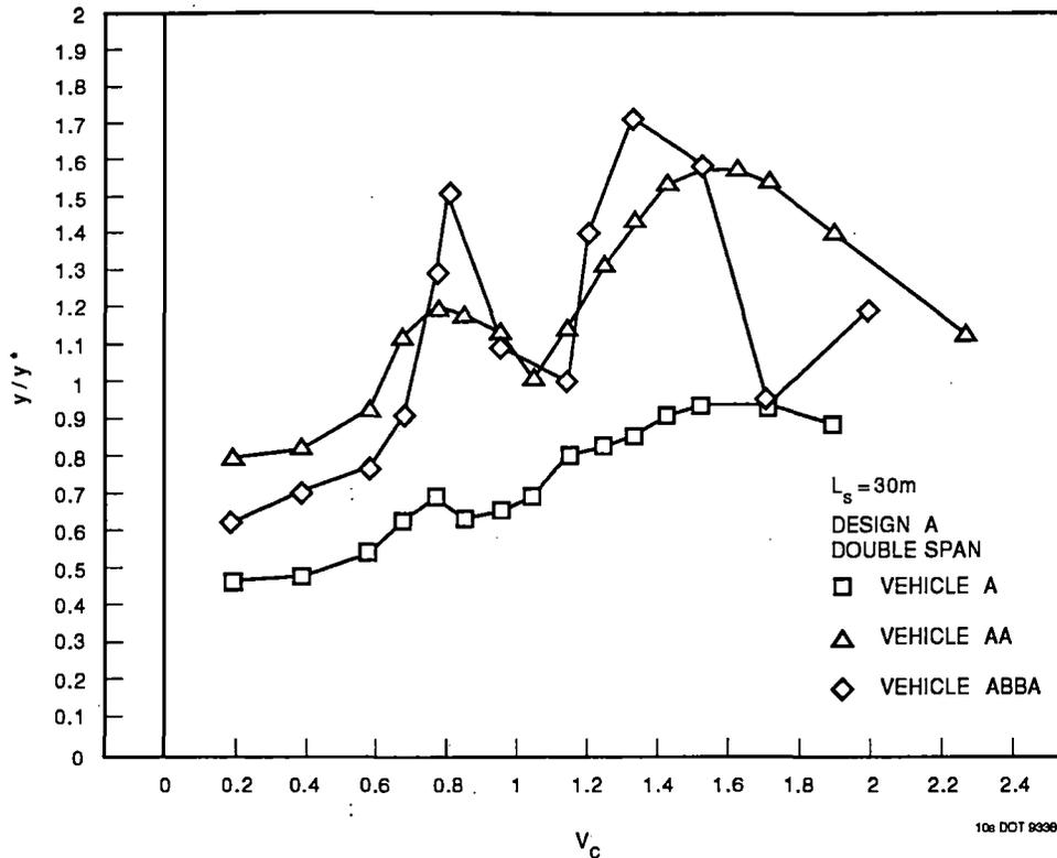
**Figure 4-12. Effect of Vehicle Consist - Double Span**
