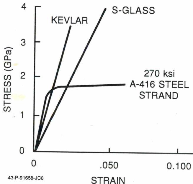
Figure 3-11. Stress-Strain Curves for Nonmetallic Fibers for Pre-Stressing
