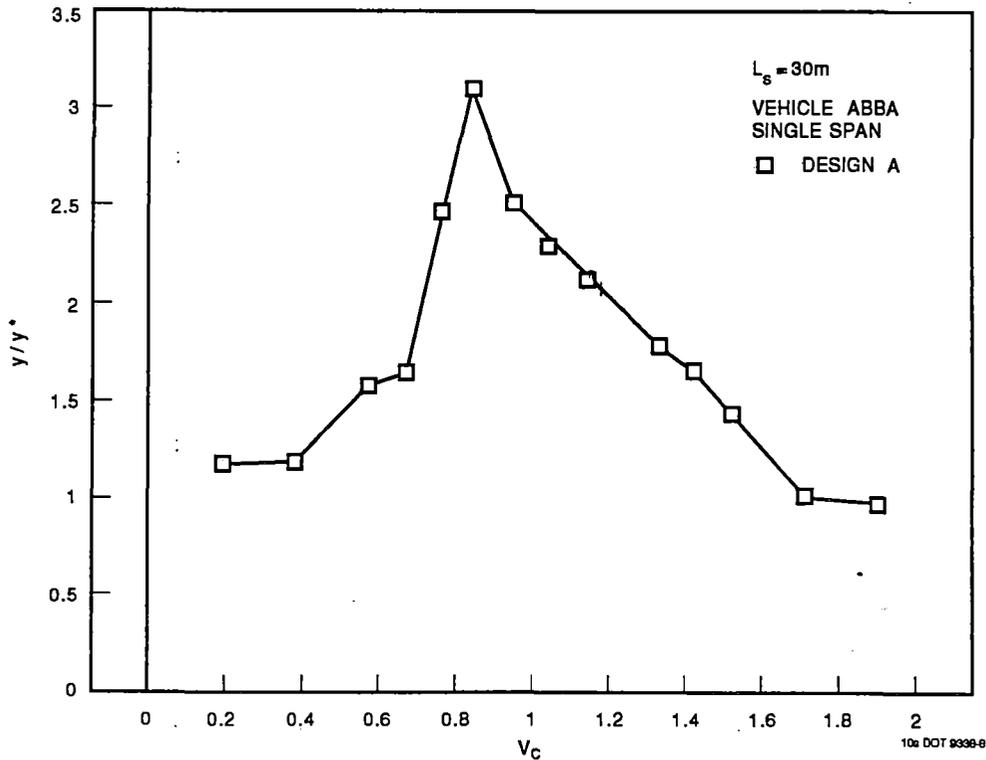
Figure 4-7. Dynamic Response - Single Span Guideway
