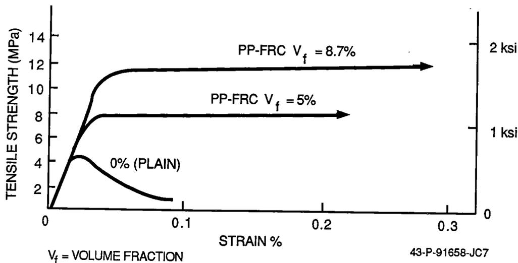
**Figure 3-10. Typical Uniaxial Tensile Strengths for Polypropylene Fiber Reinforced Concrete (PP-FRC)**
