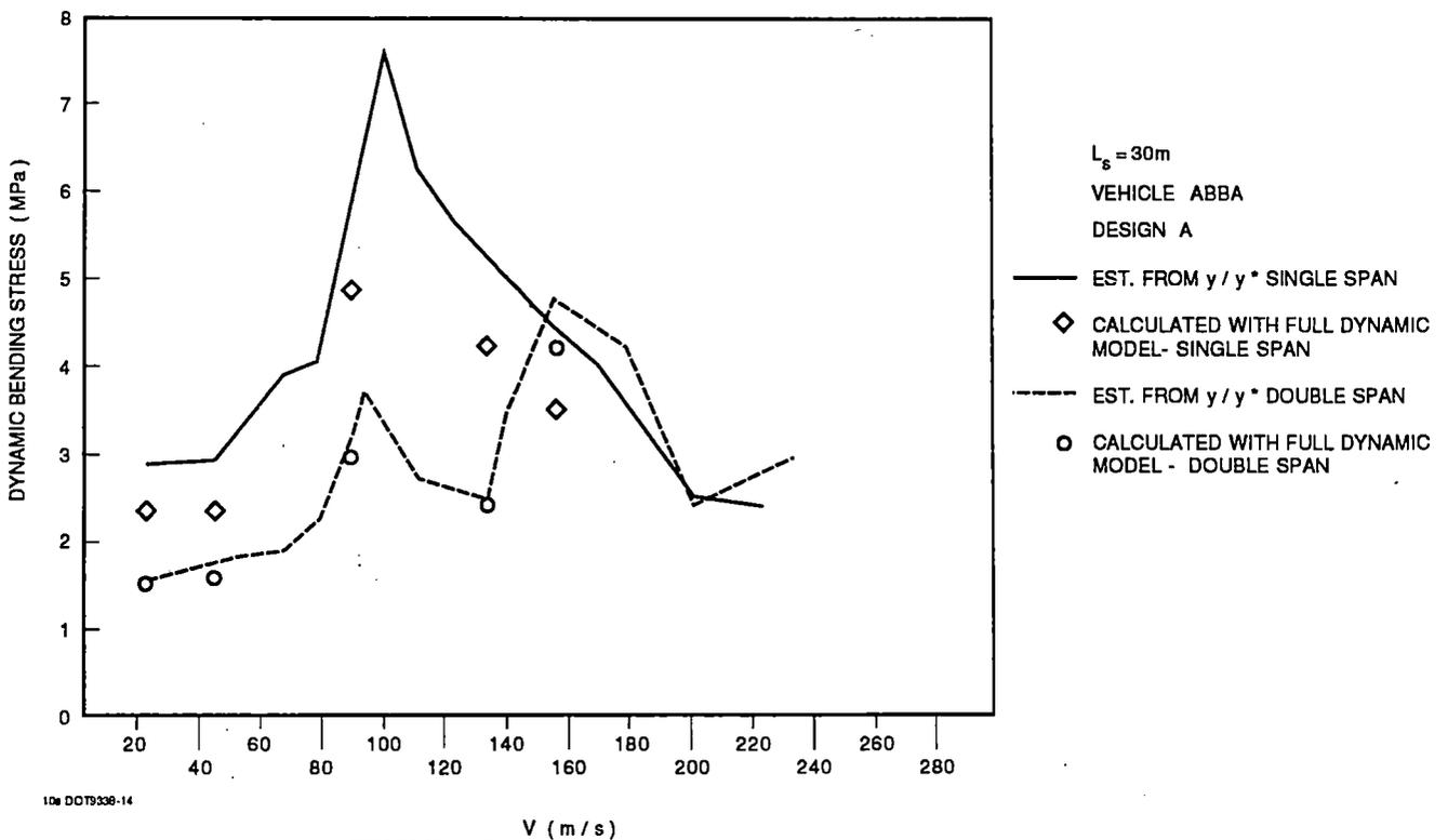
Figure 4-18. Numerical Example of Guideway Dynamic Bending Stress
