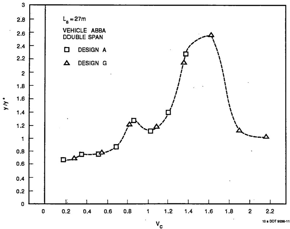
Figure 4-16. Dynamic Response - 27m Double Span
