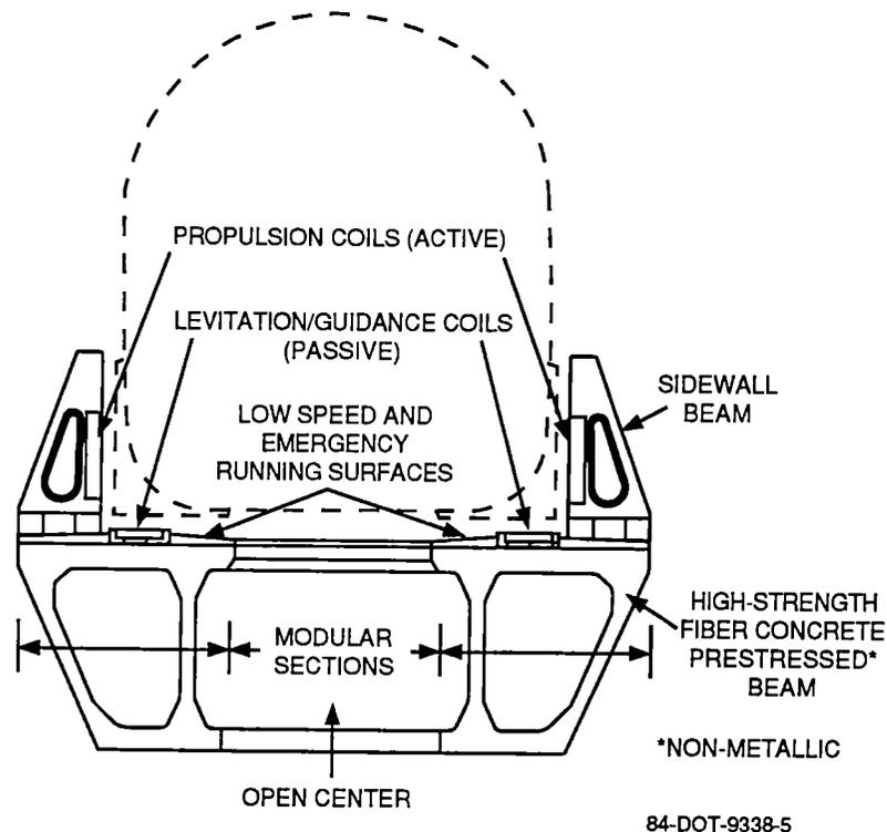
**Figure 3-1. General Layout of Configuration I Guideway with Ground-Coil SC/ED Layout**
