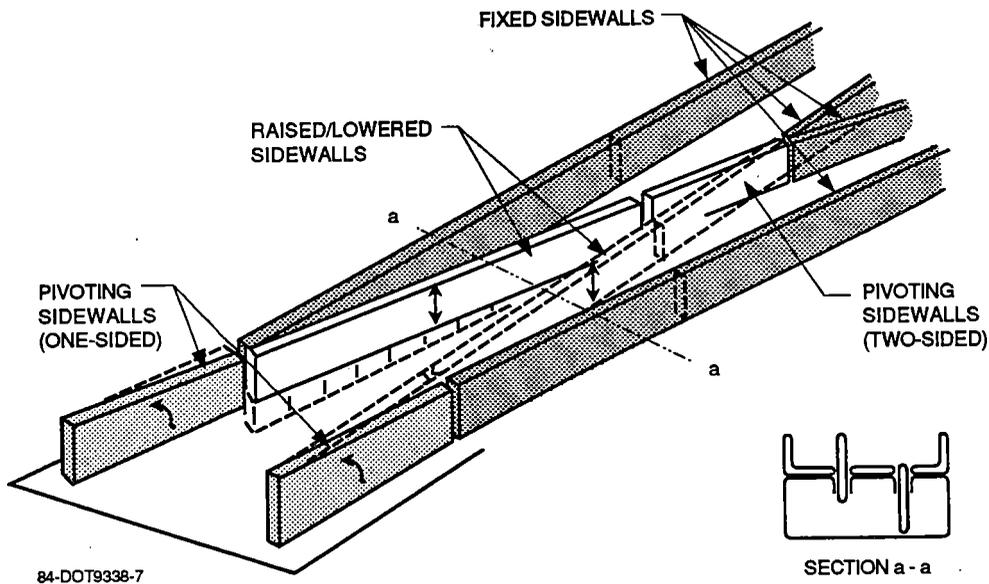
**Figure 3-14. Type II Switch Concept for Terminal Areas**
