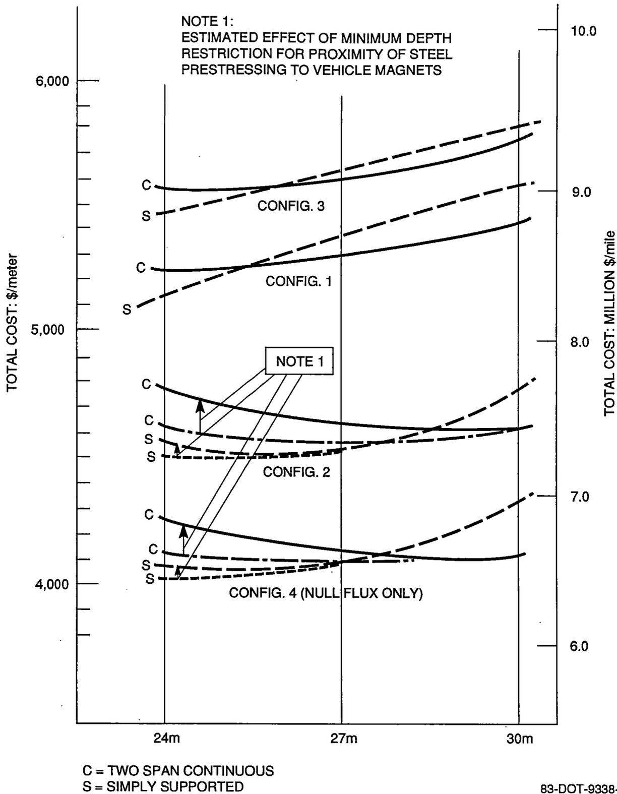
Figure 5-3. Guideway Construction Cost per Unit Length of Two-Way Guideway Structure
