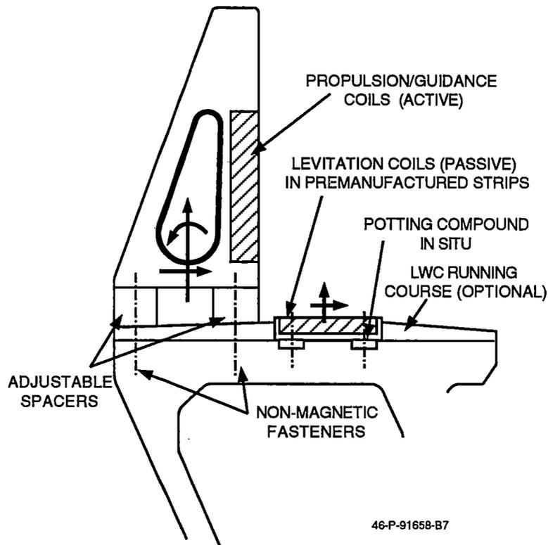
**Figure 3-4. Alignment of Guideway Components (Ground Coil Scheme)**
