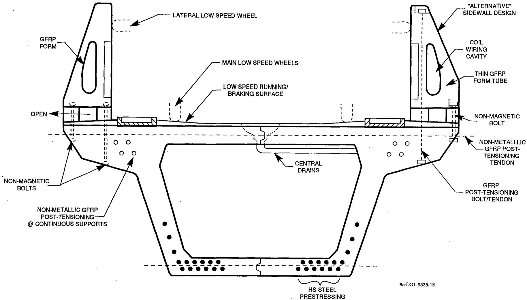
**Figure 3-7. Configuration III - Single Cell Two-Piece Guideway**
