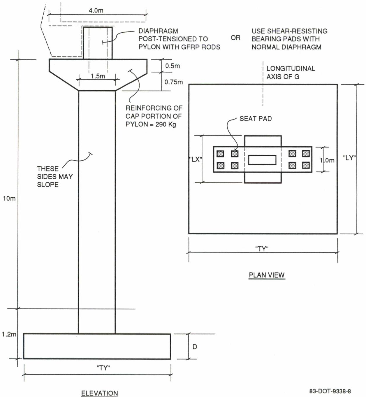
**Figure 4-23. Typical Pylon/Footing Configuration**
