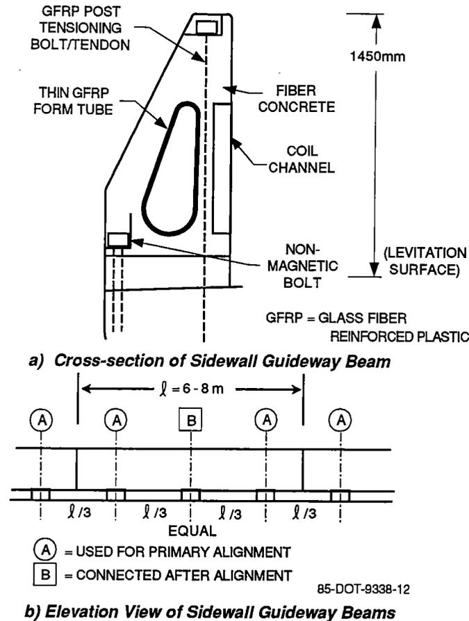
**Figure 3-3. Elevation View of Sidewall Guideway Beams Configuration I**
