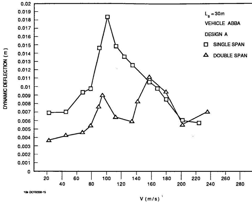
Figure 4-17. Numerical Example of Guideway Dynamic Deflection
