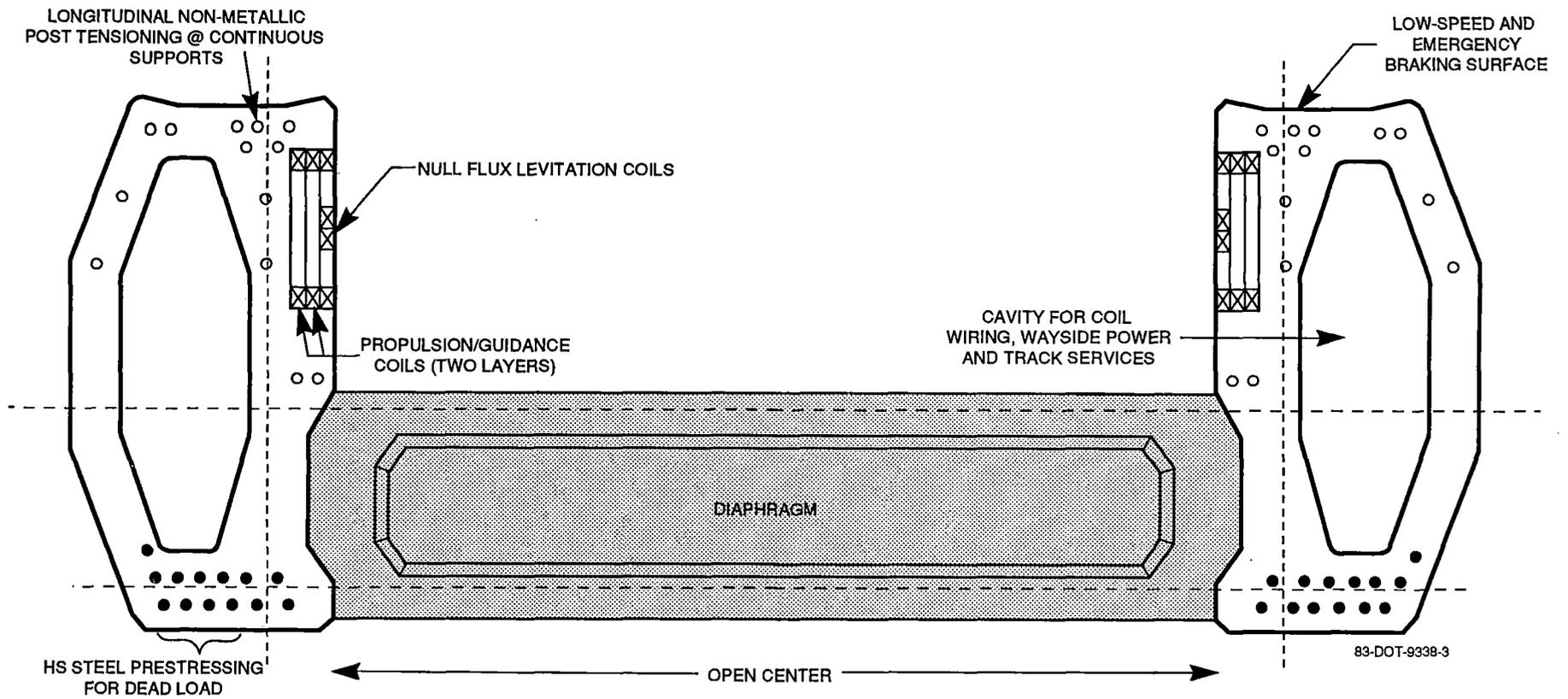
**Figure 3-8. Open-Bottom, Null Flux Guideway Configuration IV**
