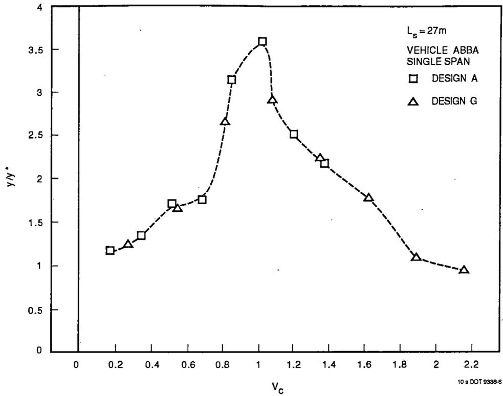
Figure 4-15. Dynamic Response - 27m Single Span
