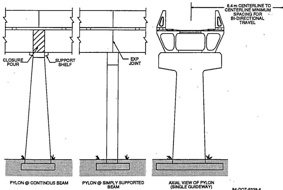
**Figure 3-9. Typical Pylon Configurations**
