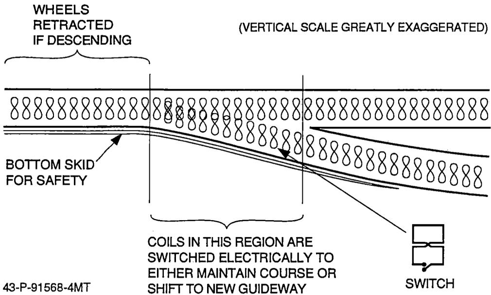
**Figure 3-13. Type I-B Open Bottom Guideway Vertical Switch System**
