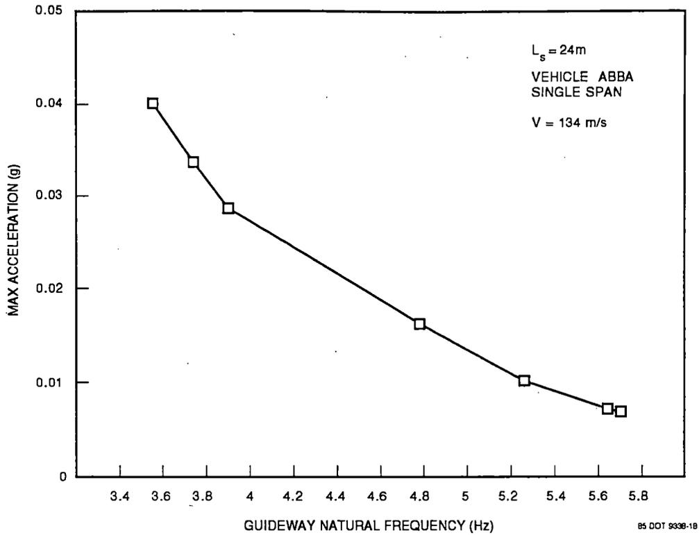
**Figure 4-20. Vehicle Heave Acceleration - 24m Single Span**
