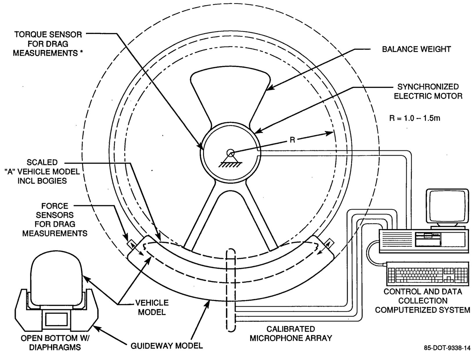
**Figure 8-4. Aerodynamic Drag and Acoustic Emission Test Setup (Same Test Machine as for Magnetic Effects Study)**
