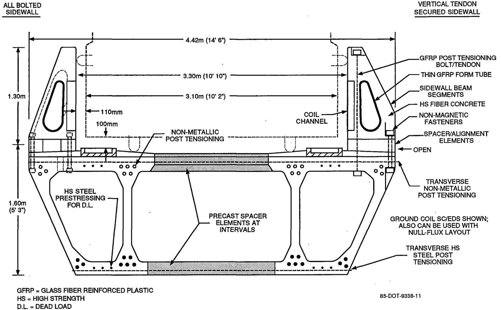
**Figure 3-2. Open-Bottom, Modular Sidewall Guideway Configuration I**
