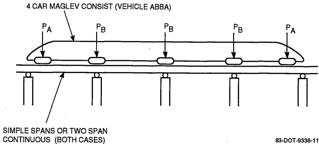
**Figure 4-4. Dynamic Model of Guideway Loads**
