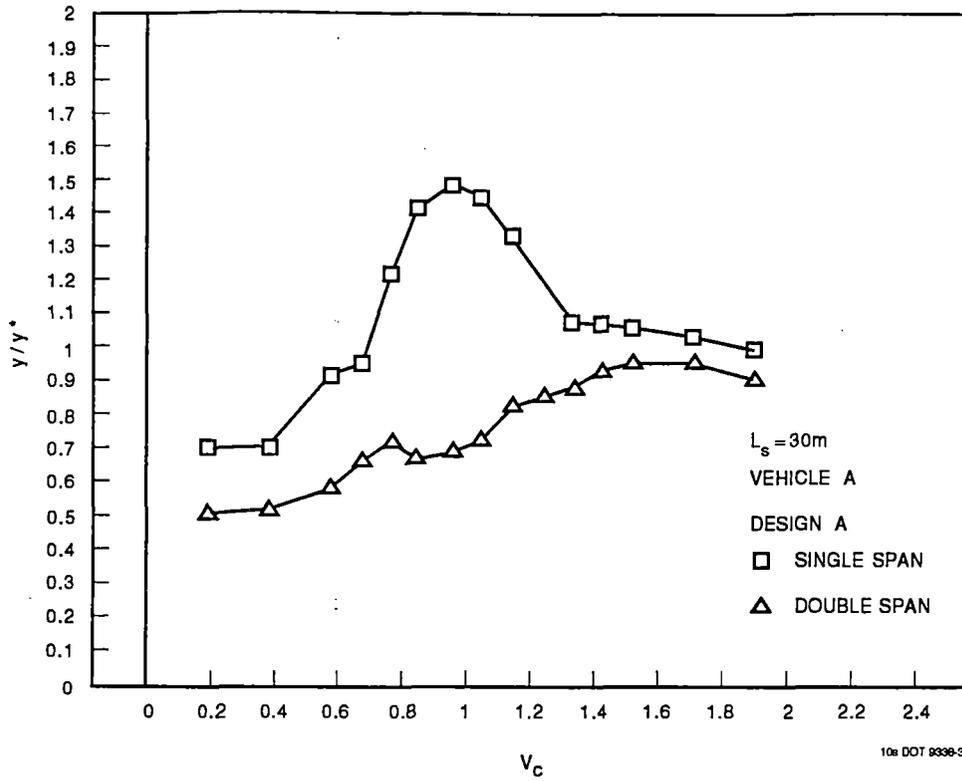
**Figure 4-8. Dynamic Response for Vehicle A**
