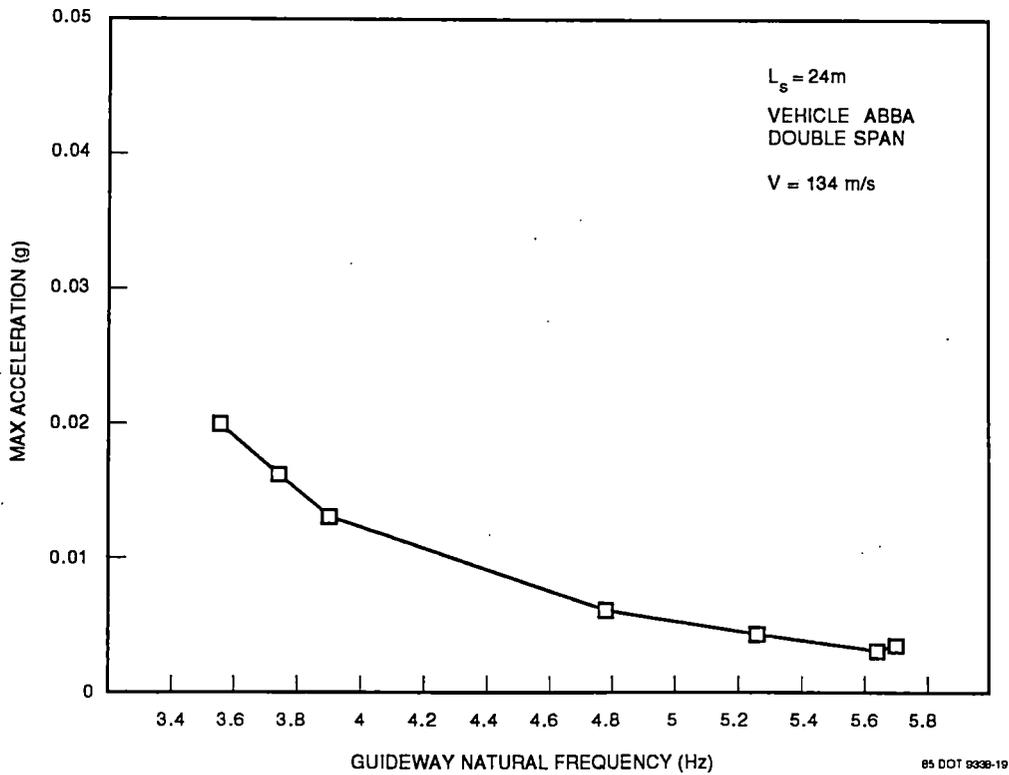
**Figure 4-21. Vehicle Heave Acceleration - 24m Double Span**
