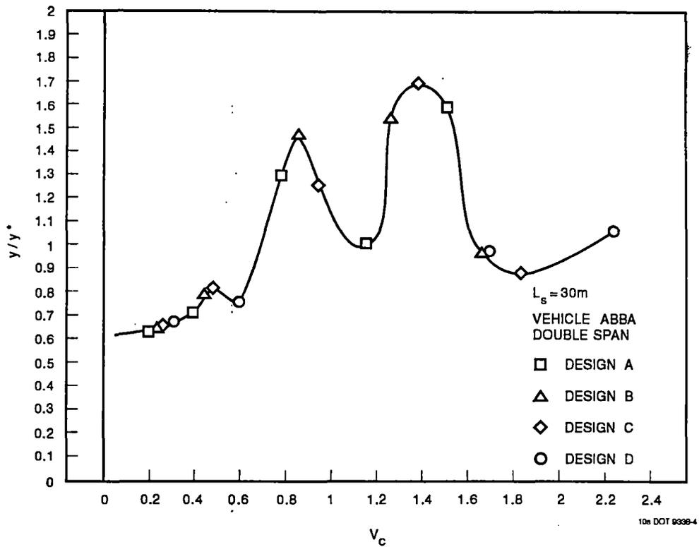
Figure 4-6. Dynamic Response - Second Span of a Double Span Guideway
