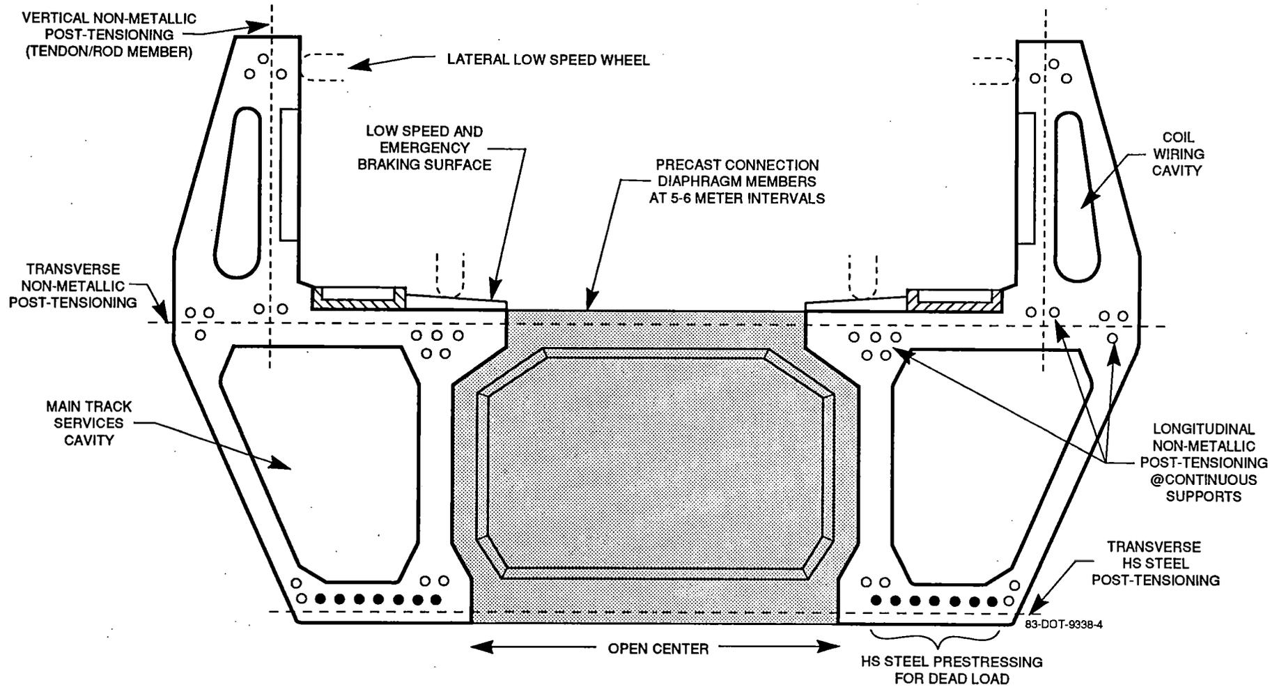
**Figure 3-6. Open-Bottom, Integral Sidewall Guideway Configuration II**
