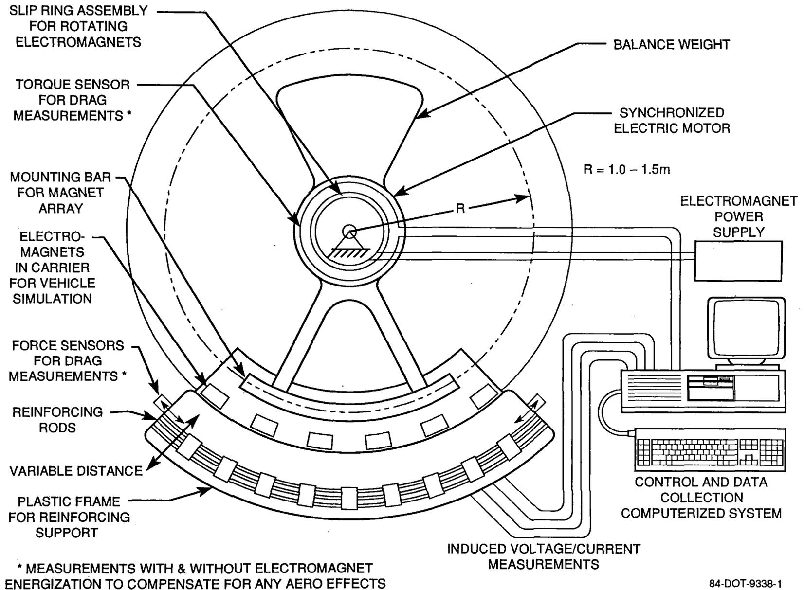
*Figure 8-3. Interaction Test Setup (Same Test Machine as for Acoustic Study)*
