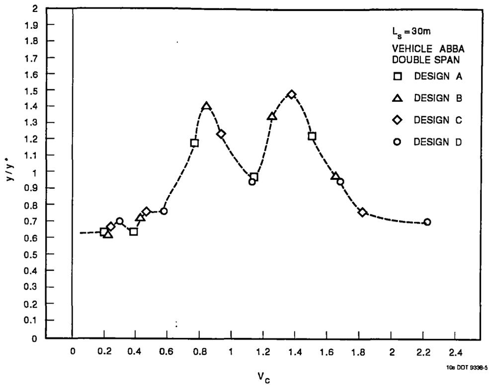
Figure 4-5. Dynamic Response - First Span of a Double Span Guideway
