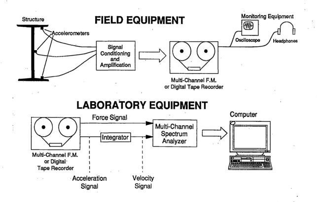
Figure 7. Schematic of Vibration Measurement System
