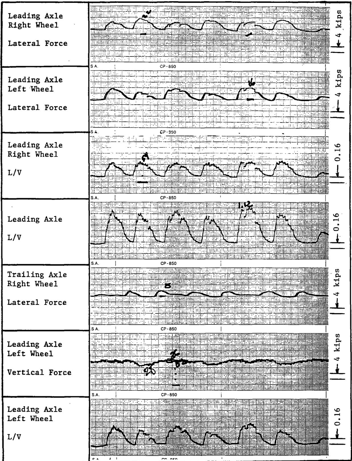
FIGURE 2-10. LOCOMOTIVE - STRIP CHART DATA - SECTION 2.2, 39' WAVELENGTH, 2.25" PEAK TO PEAK, RUN 77, 5 MPH
