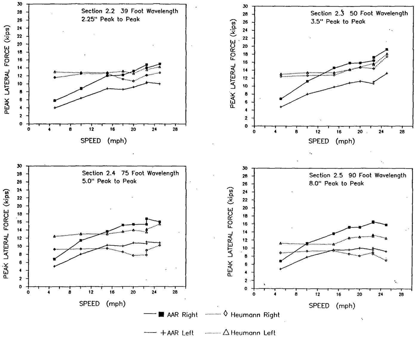
**FIGURE 3.4-1 LOADED FLAT CAR - PEAK LATERAL WHEEL FORCES AT LOW SPEED TEST SECTION**
