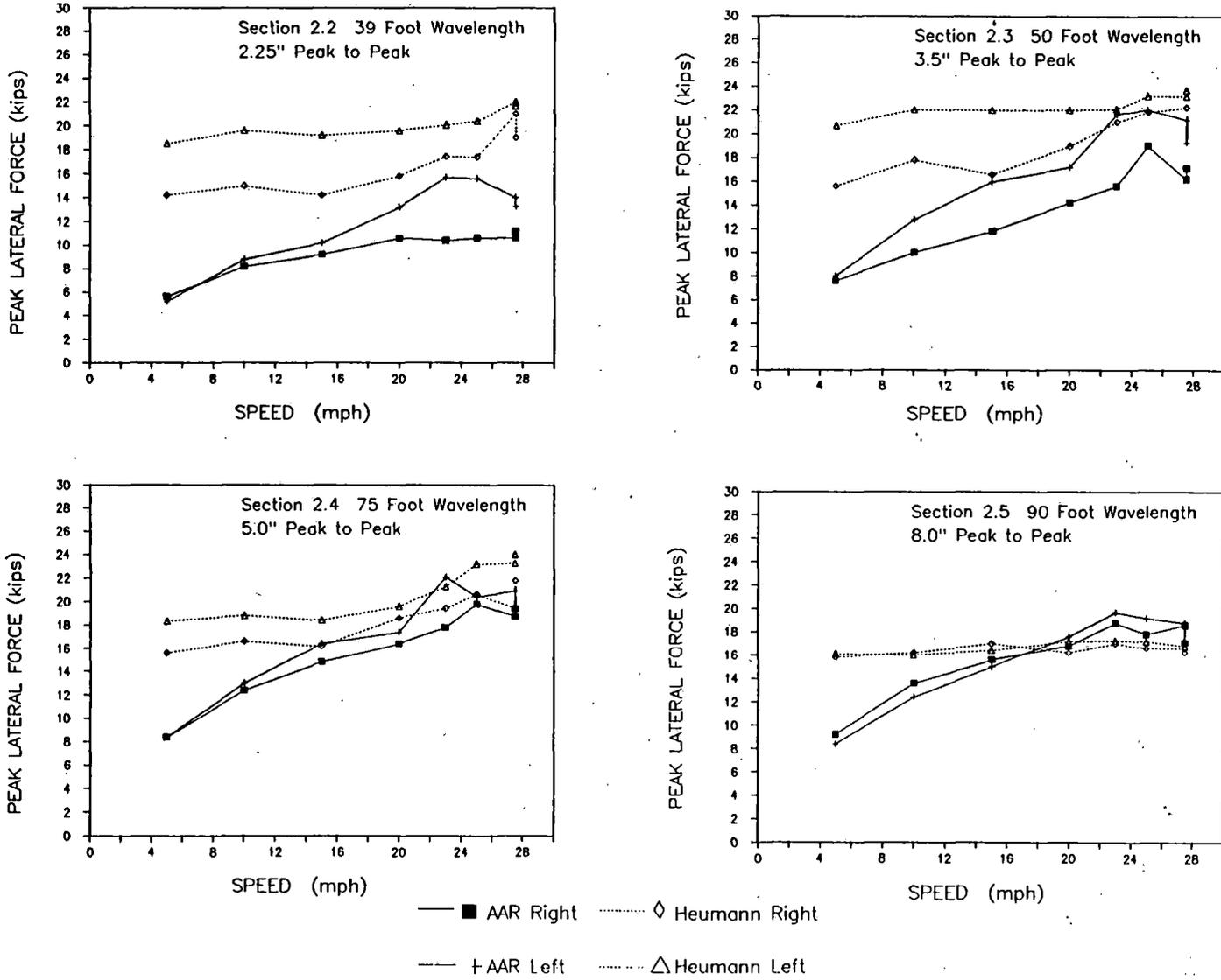
FIGURE 3.2-1 LOADED HOPPER CAR - PEAK LATERAL WHEEL FORCES AT LOW SPEED TEST SECTION
