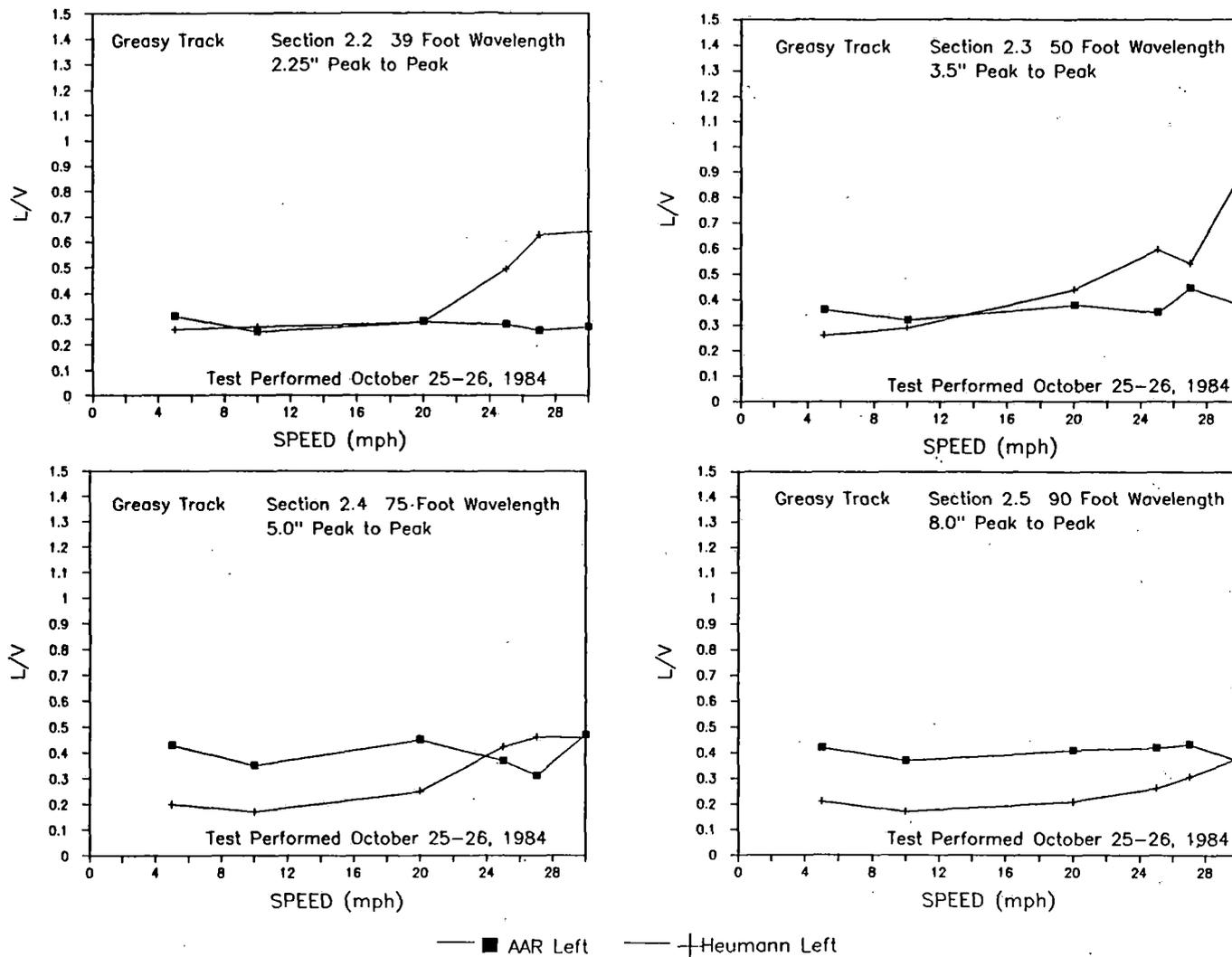
**FIGURE 3.5-2 EMPTY HOPPER CAR - PEAK LATERAL TO VERTICAL WHEEL FORCE RATIOS AT LOW SPEED TEST SECTION**
