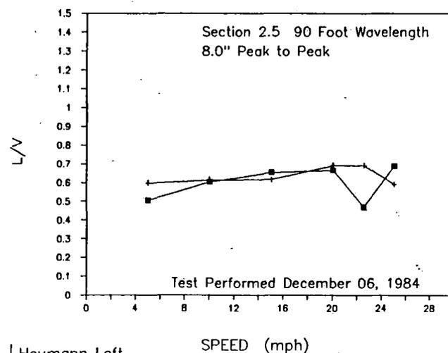
**FIGURE 3.4-4 LOADED FLAT CAR - PEAK LATERAL TO VERTICAL WHEEL FORCE RATIOS AT LOW SPEED TEST SECTION**
