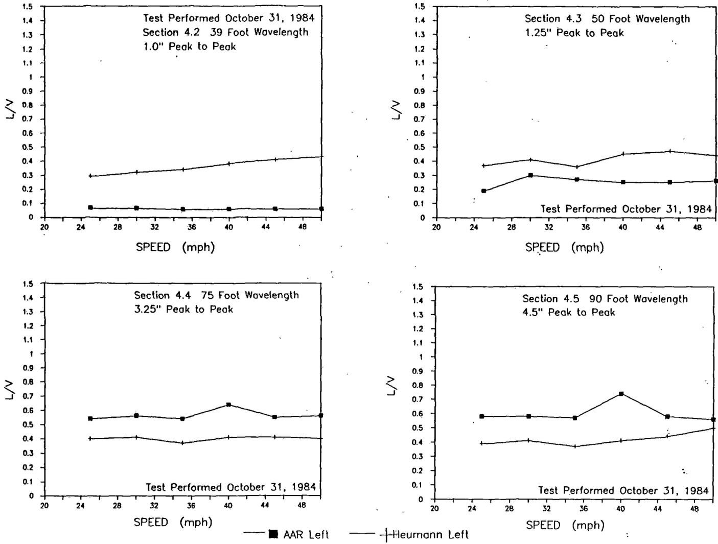
**FIGURE 3.2-6 LOADED HOPPER CAR - PEAK LATERAL TO VERTICAL WHEEL FORCE RATIOS AT HIGH SPEED TEST SECTION**
