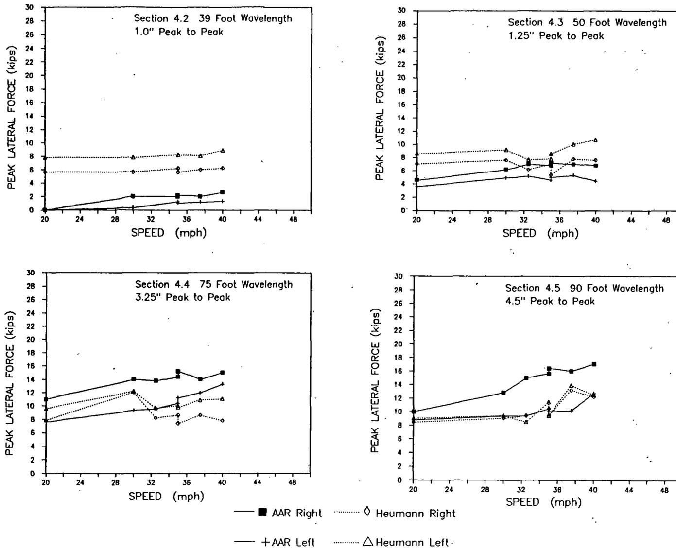
FIGURE 3.4-3 LOADED FLAT CAR - PEAK LATERAL WHEEL FORCES AT HIGH SPEED TEST SECTION
