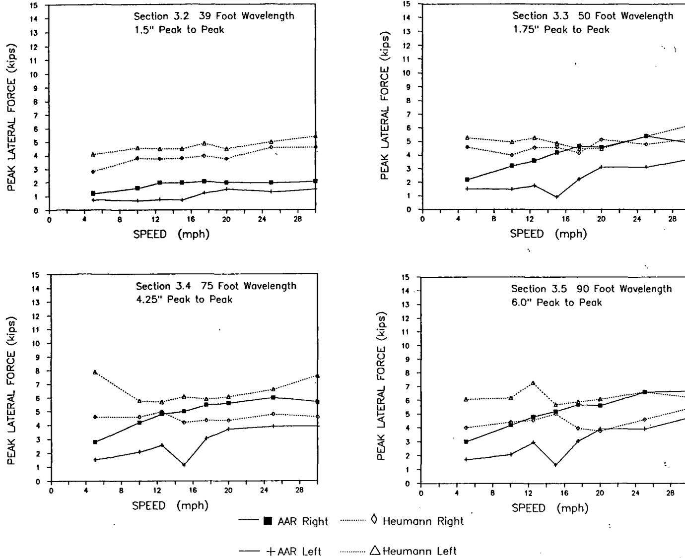
FIGURE 3.7-2 EMPTY FLAT CAR - PEAK LATERAL WHEEL FORCES AT INTERMEDIATE SPEED TEST SECTION
