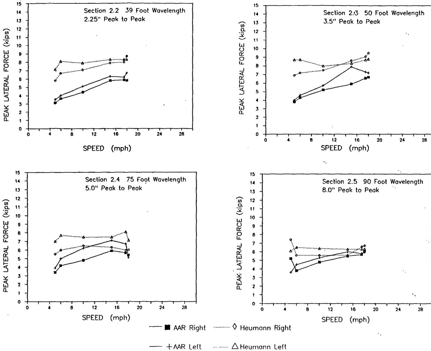
FIGURE 3.6-1 EMPTY TANK CAR - PEAK LATERAL WHEEL FORCES AT LOW SPEED TEST SECTION
