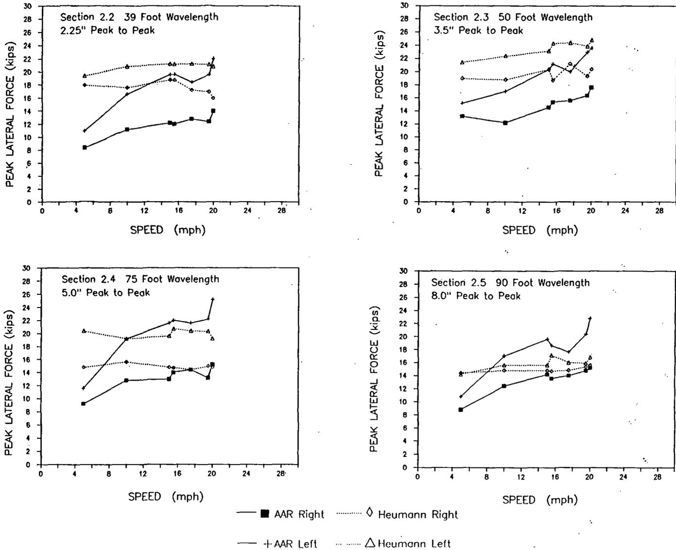
FIGURE 3.3-1 LOADED TANK CAR - PEAK LATERAL WHEEL FORCES AT LOW SPEED TEST SECTION
