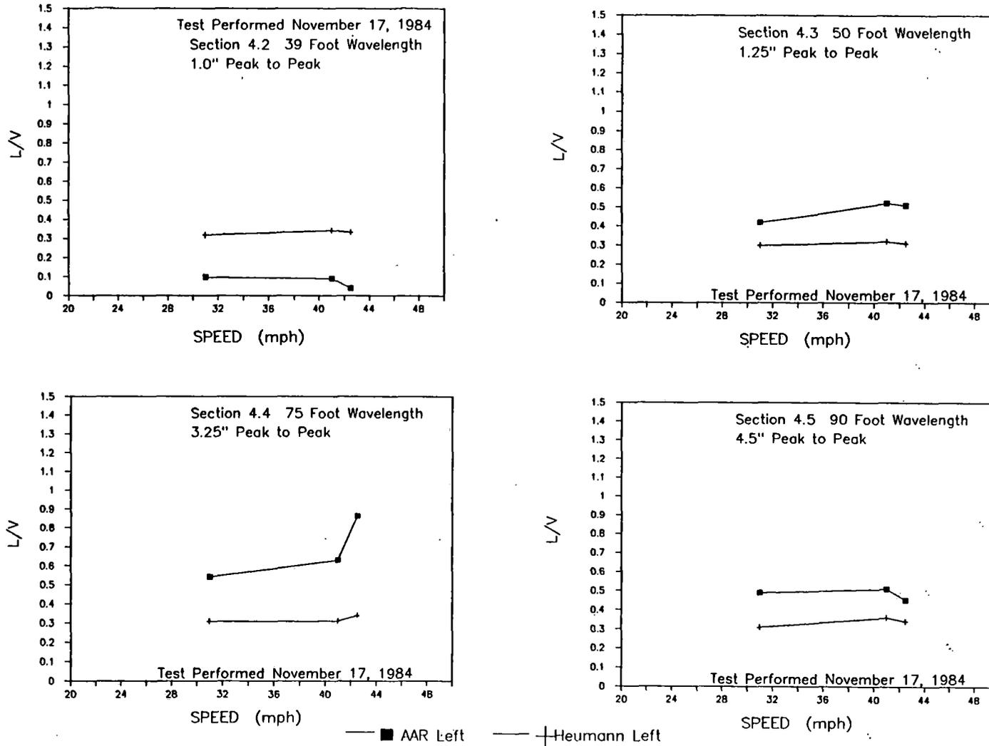
**FIGURE 3.3-6 LOADED TANK CAR - PEAK LATERAL TO VERTICAL WHEEL FORCE RATIOS AT HIGH SPEED TEST SECTION**
