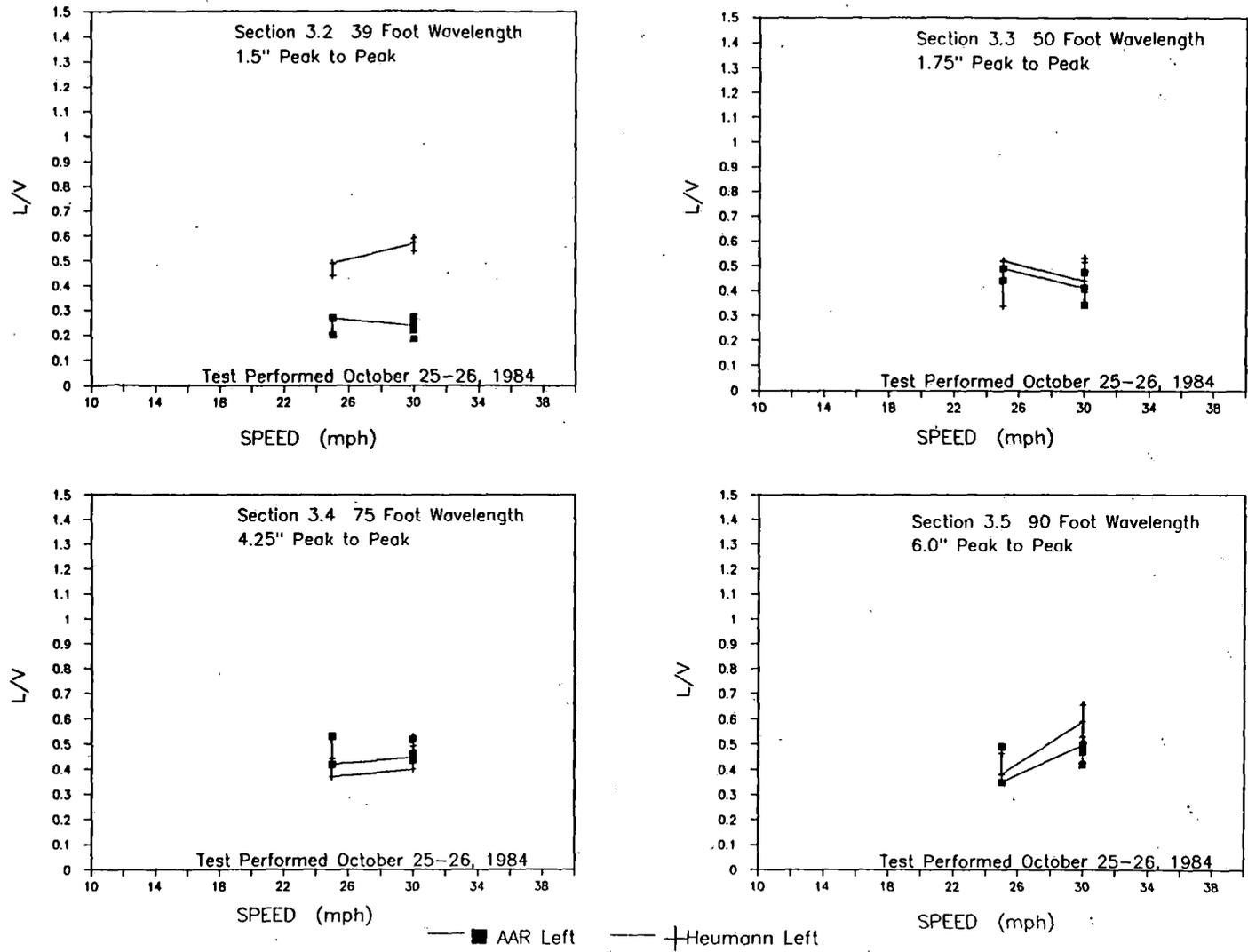
**FIGURE 3.5-4 EMPTY HOPPER CAR - PEAK LATERAL TO VERTICAL WHEEL FORCE RATIOS AT INTERMEDIATE SPEED TEST SECTION**
