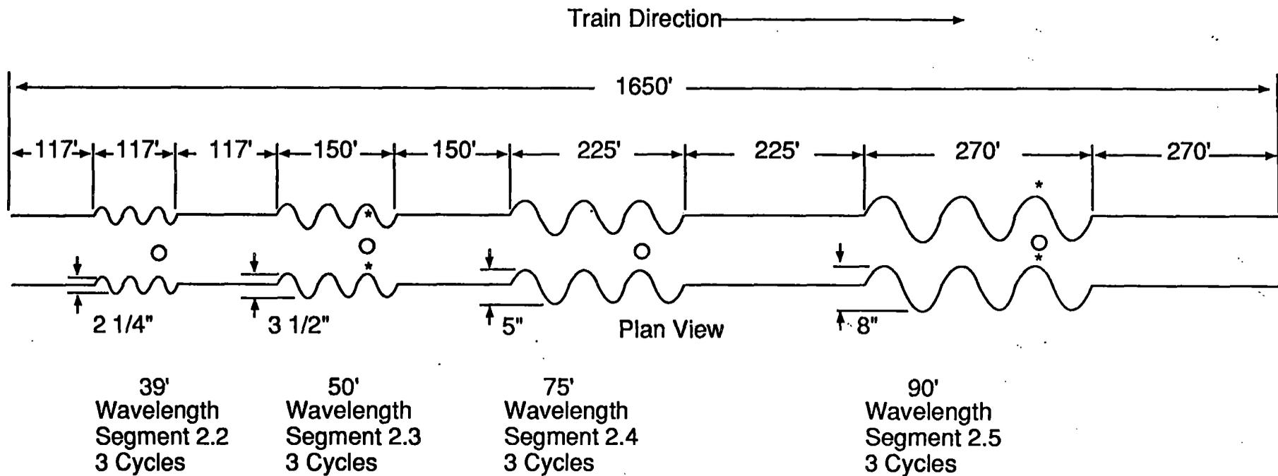
Slow Speed Test Section 0-30 MPH
