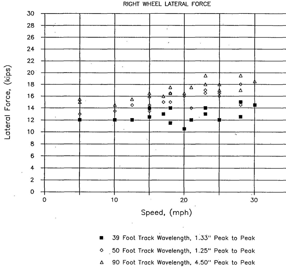
**FIGURE 4-1 TEST AT BENNINGTON, NH - LOCOMOTIVE**
