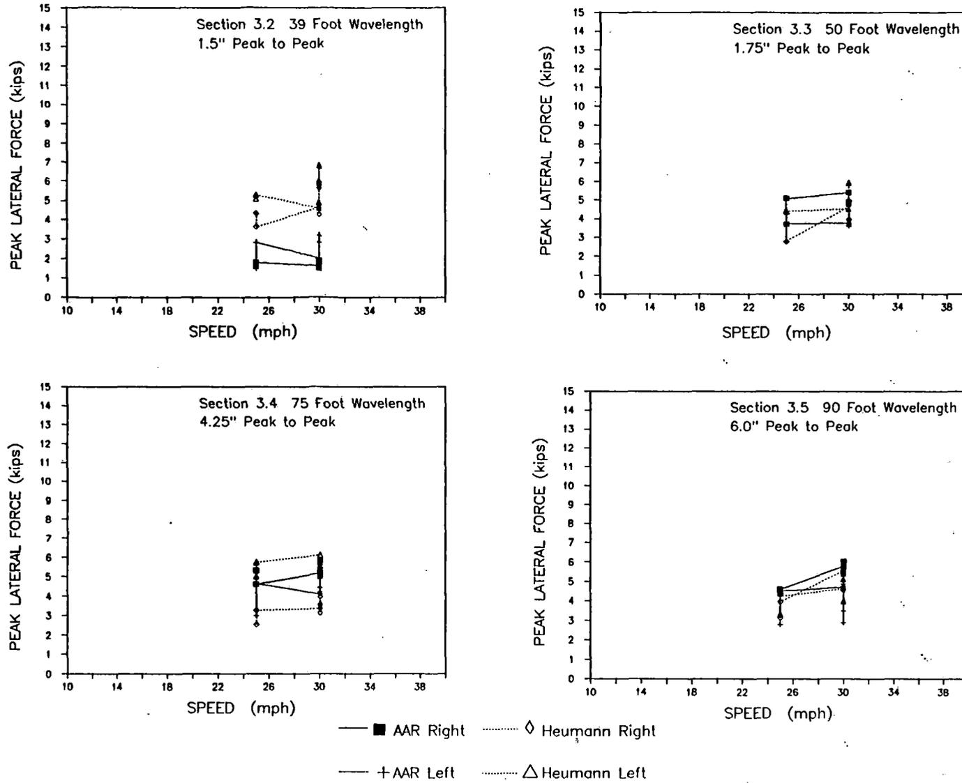
FIGURE 3.5-3 EMPTY HOPPER CAR - PEAK LATERAL WHEEL FORCES AT INTERMEDIATE SPEED TEST SECTION
