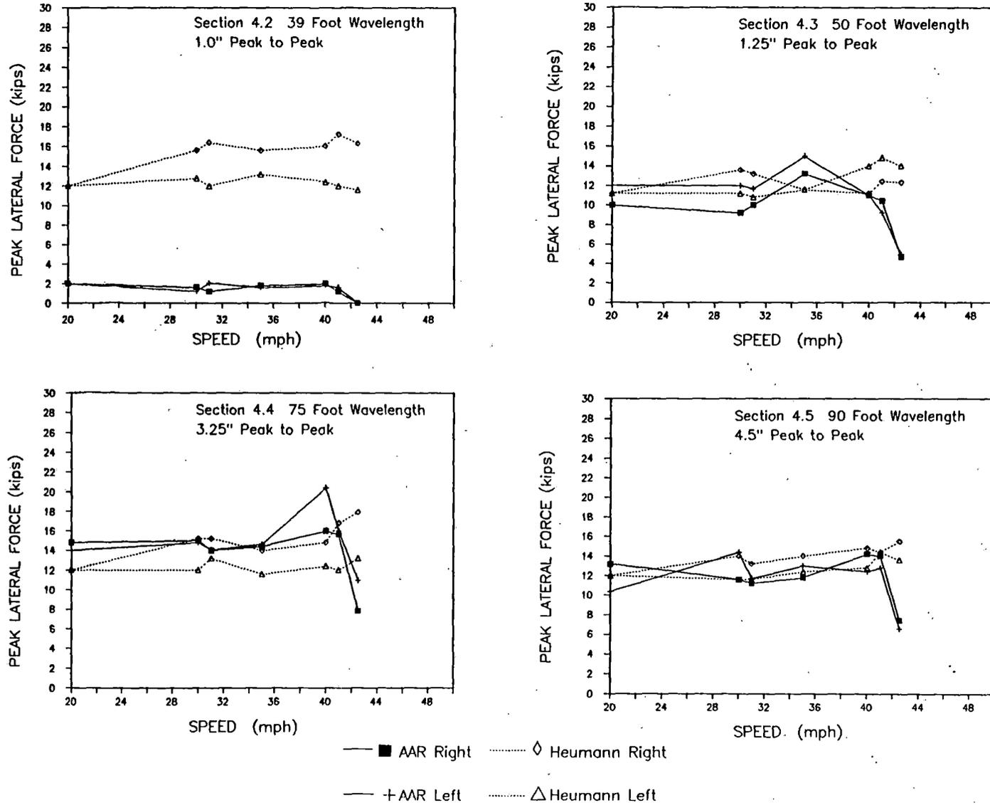
**FIGURE 3.3-3 LOADED TANK CAR - PEAK LATERAL WHEEL FORCES AT HIGH SPEED TEST SECTION**
