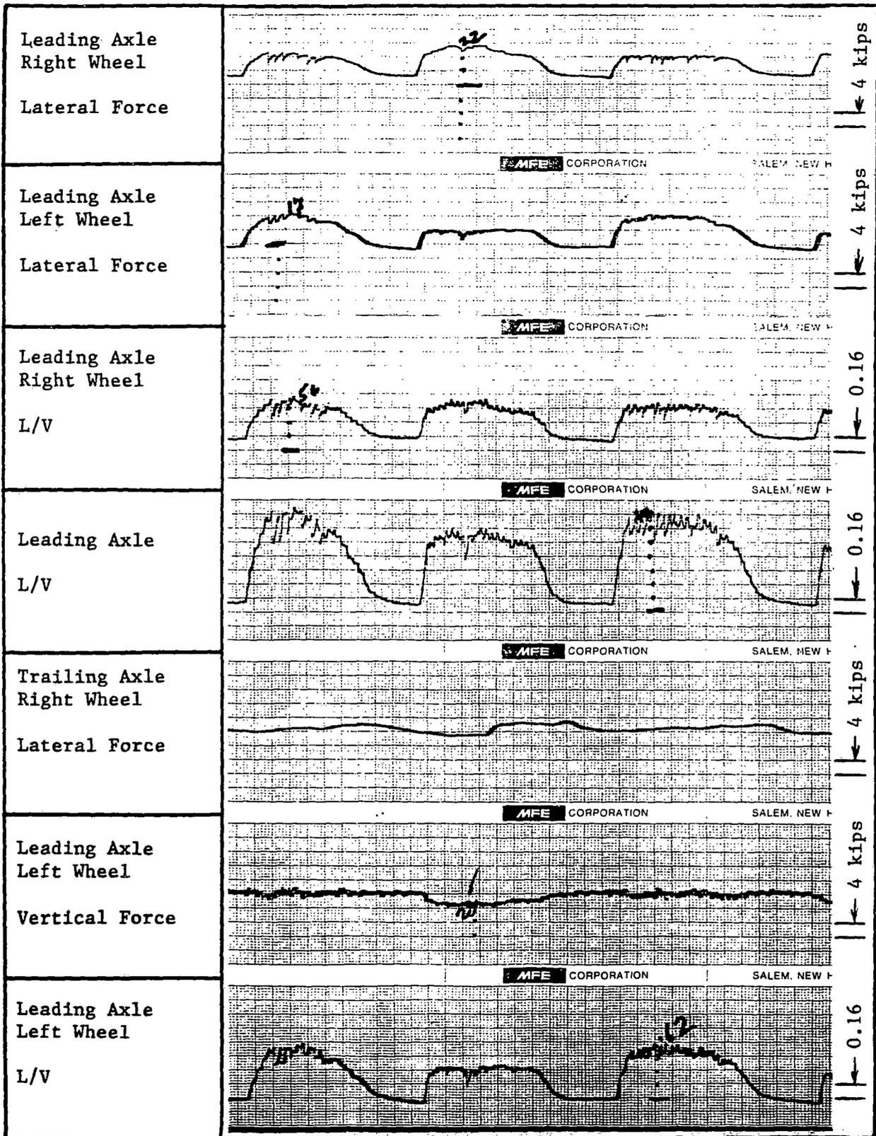
FIGURE 2-13. LOCOMOTIVE - STRIP CHART DATA - SECTION 2.5,
