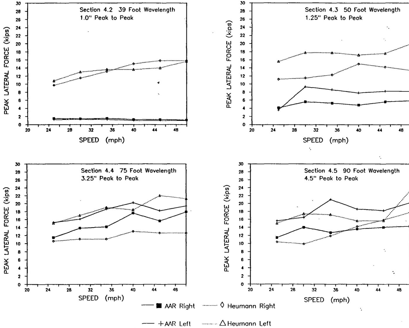
**FIGURE 3.2-5 LOADED HOPPER CAR - PEAK LATERAL WHEEL FORCES AT HIGH SPEED TEST SECTION**
