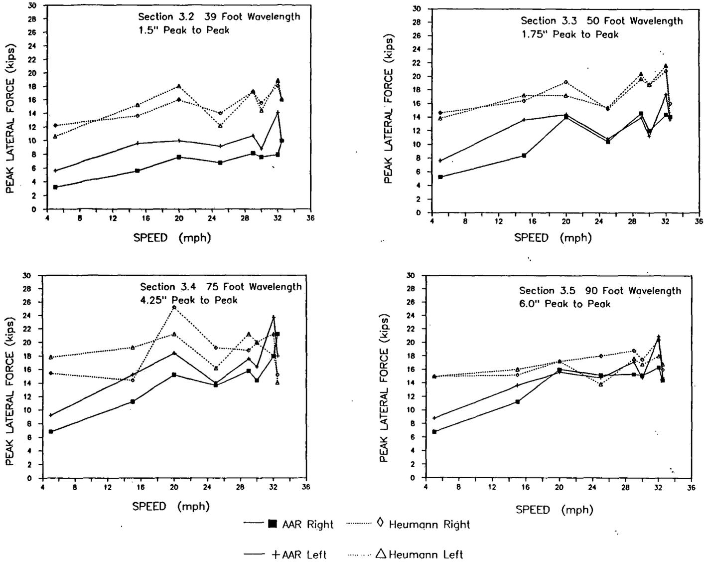
**FIGURE 3.3-2 LOADED TANK CAR - PEAK LATERAL WHEEL FORCES AT INTERMEDIATE SPEED TEST SECTION**
