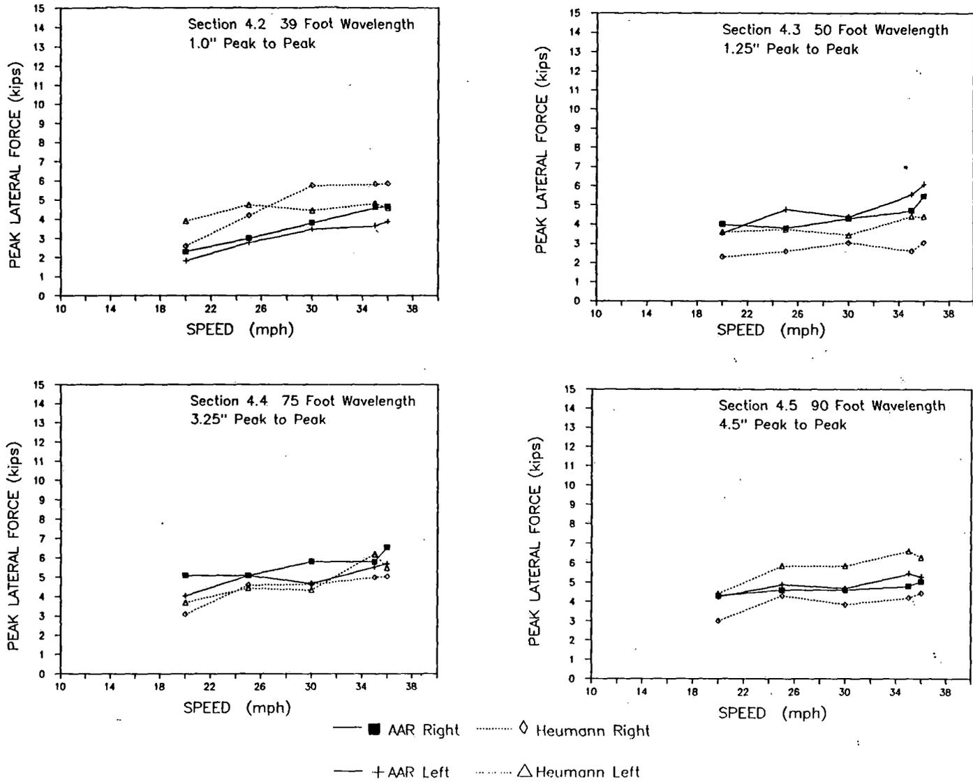
**FIGURE 3.6-3 EMPTY TANK CAR - PEAK LATERAL WHEEL FORCES AT HIGH SPEED TEST SECTION**
