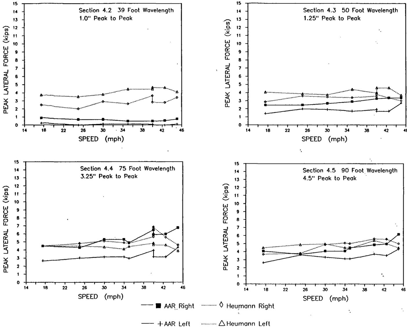
FIGURE 3.7-3 EMPTY FLAT CAR - PEAK LATERAL WHEEL FORCES AT HIGH SPEED TEST SECTION
