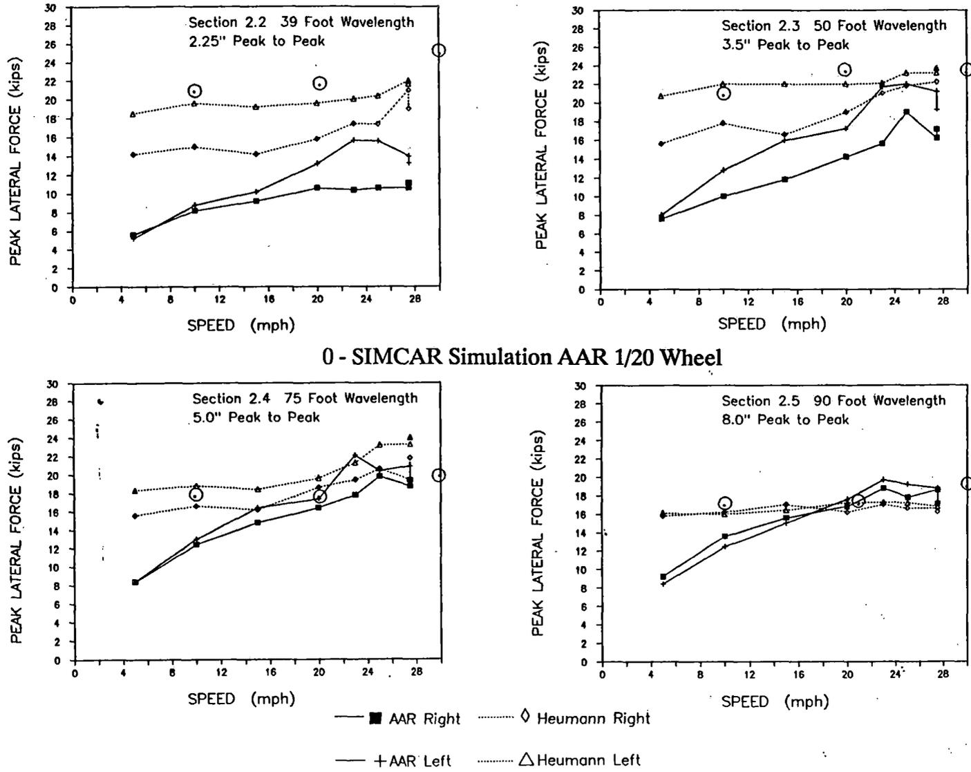
**FIGURE 4-3 LOADED HOPPER CAR - COMPARISON OF TEST MEASUREMENTS WITH SIMCAR SIMULATION RESULTS - PEAK LATERAL WHEEL FORCES AT LOW SPEED TEST SECTION**
