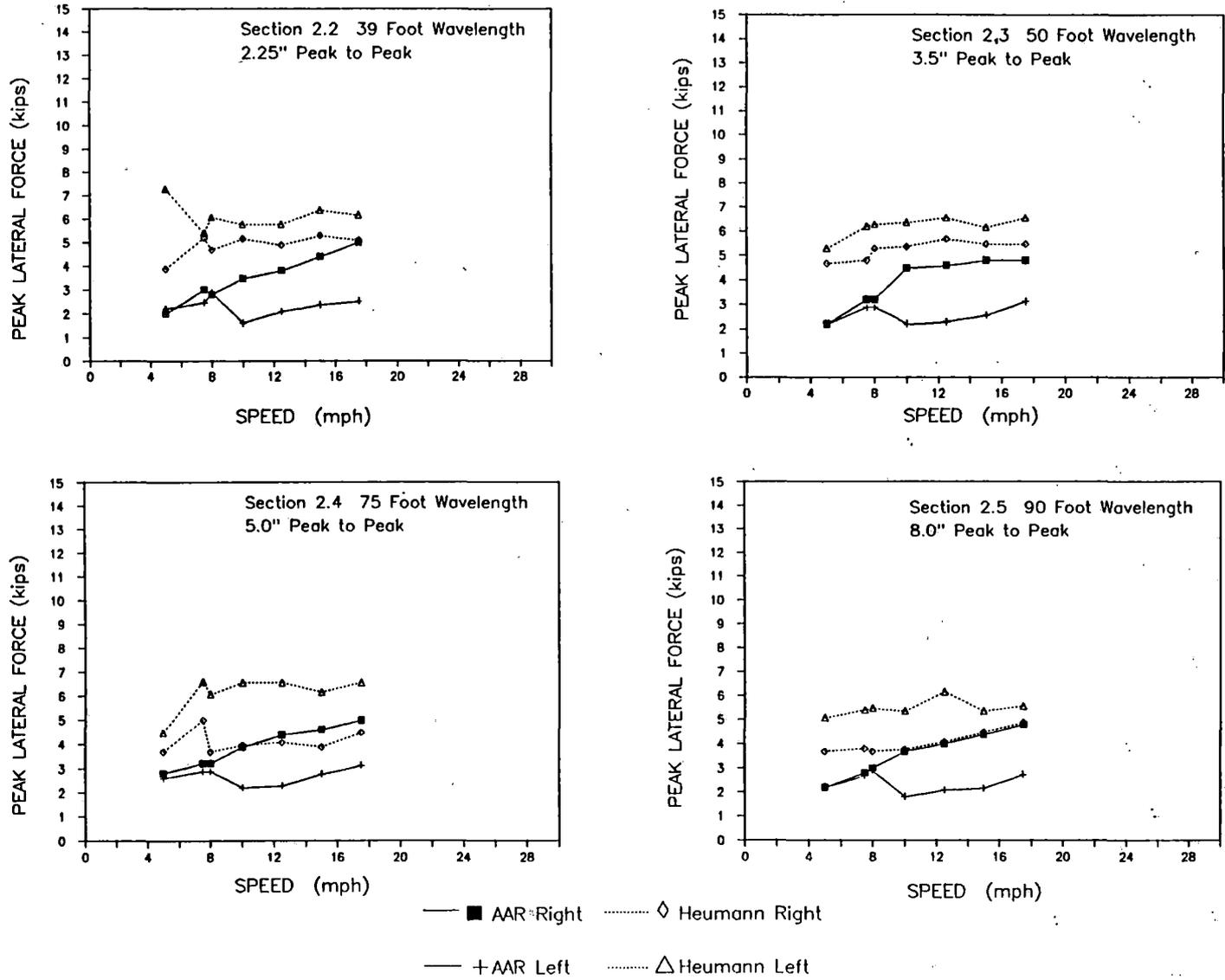
**FIGURE 3.7-1 EMPTY FLAT CAR - PEAK LATERAL WHEEL FORCES AT LOW SPEED TEST SECTION**
