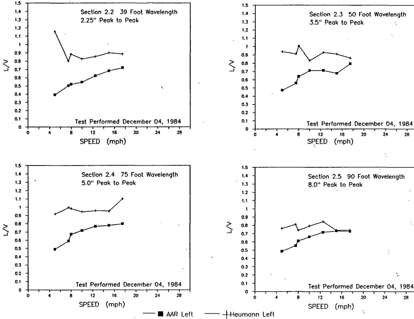
**FIGURE 3.7-4 EMPTY FLAT CAR - PEAK LATERAL TO VERTICAL WHEEL FORCE RATIOS AT LOW SPEED TEST SECTION**
