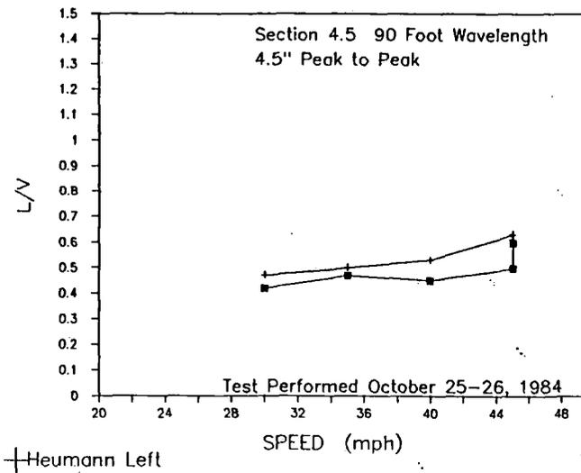
**FIGURE 3.5-6 EMPTY HOPPER CAR - PEAK LATERAL TO VERTICAL WHEEL FORCE RATIOS AT HIGH SPEED TEST SECTION**
