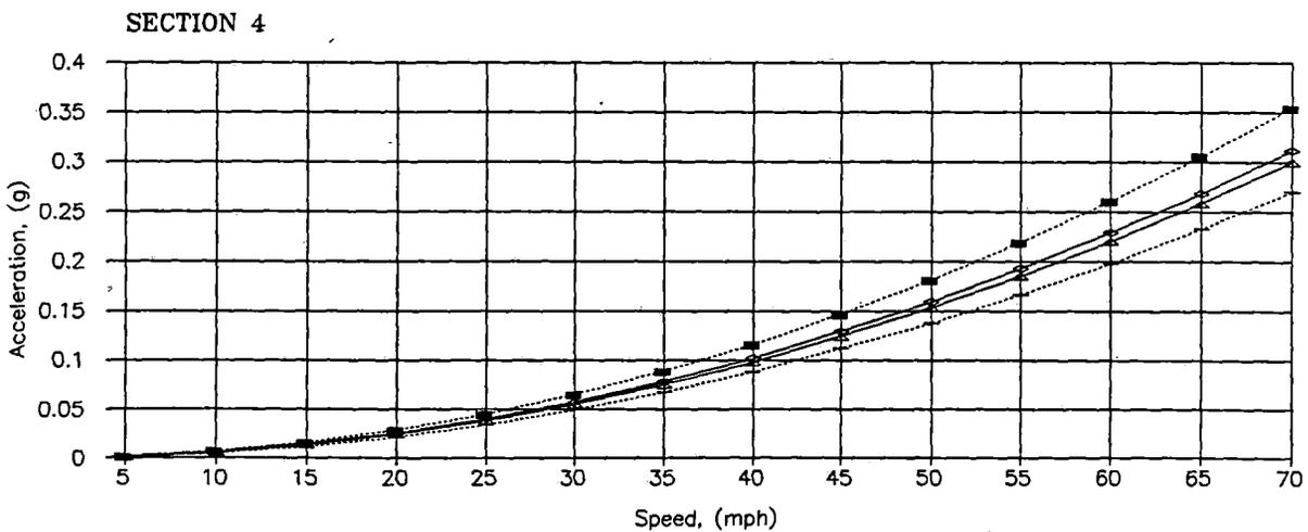
**FIGURE 2-8. ACCELERATION OF POINT PERFECTLY FOLLOWING SPECIFIED ALIGNMENT VARIATION**
