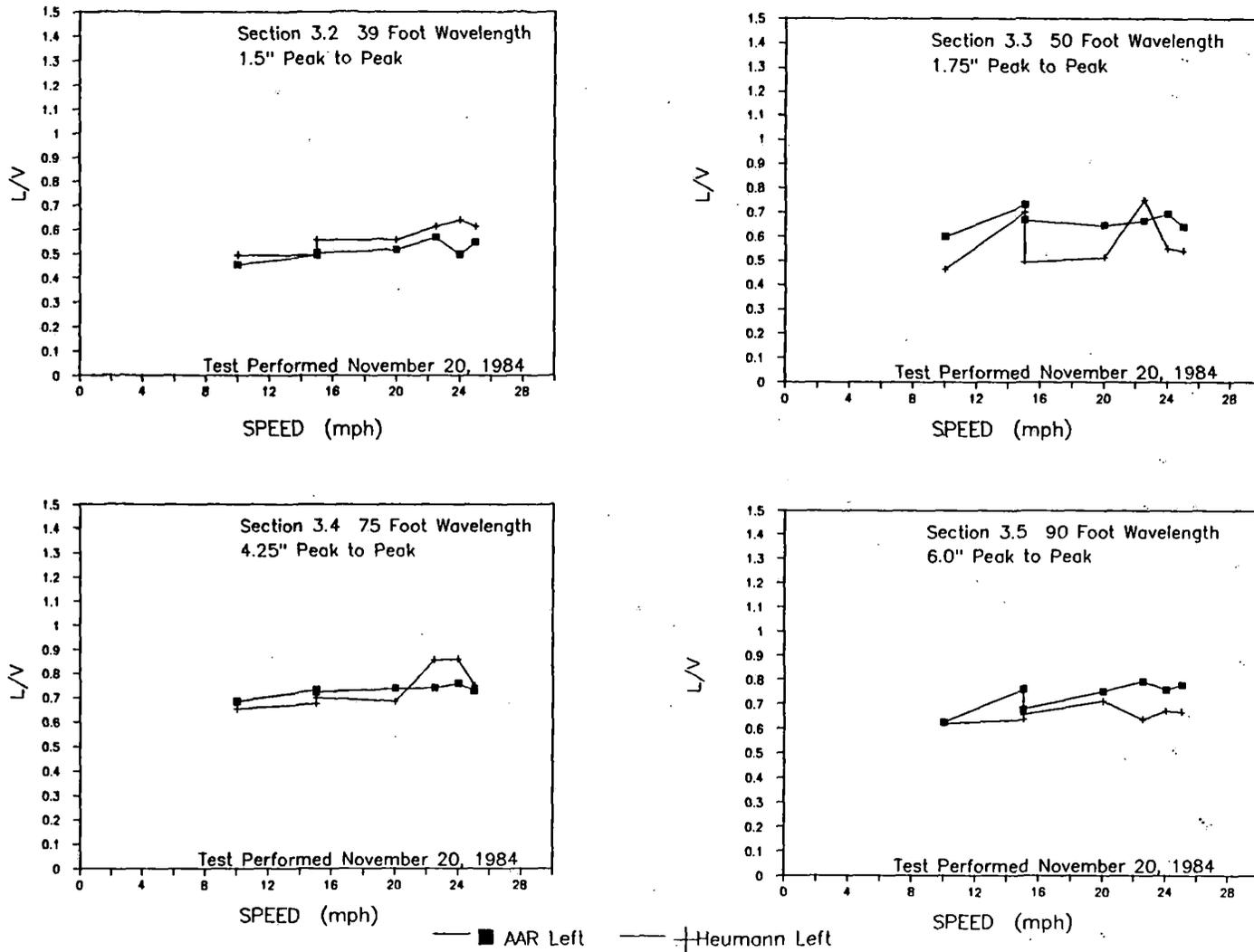
**FIGURE 3.6-5 EMPTY TANK CAR - PEAK LATERAL TO VERTICAL WHEEL FORCE RATIOS AT INTERMEDIATE SPEED TEST SECTION**
