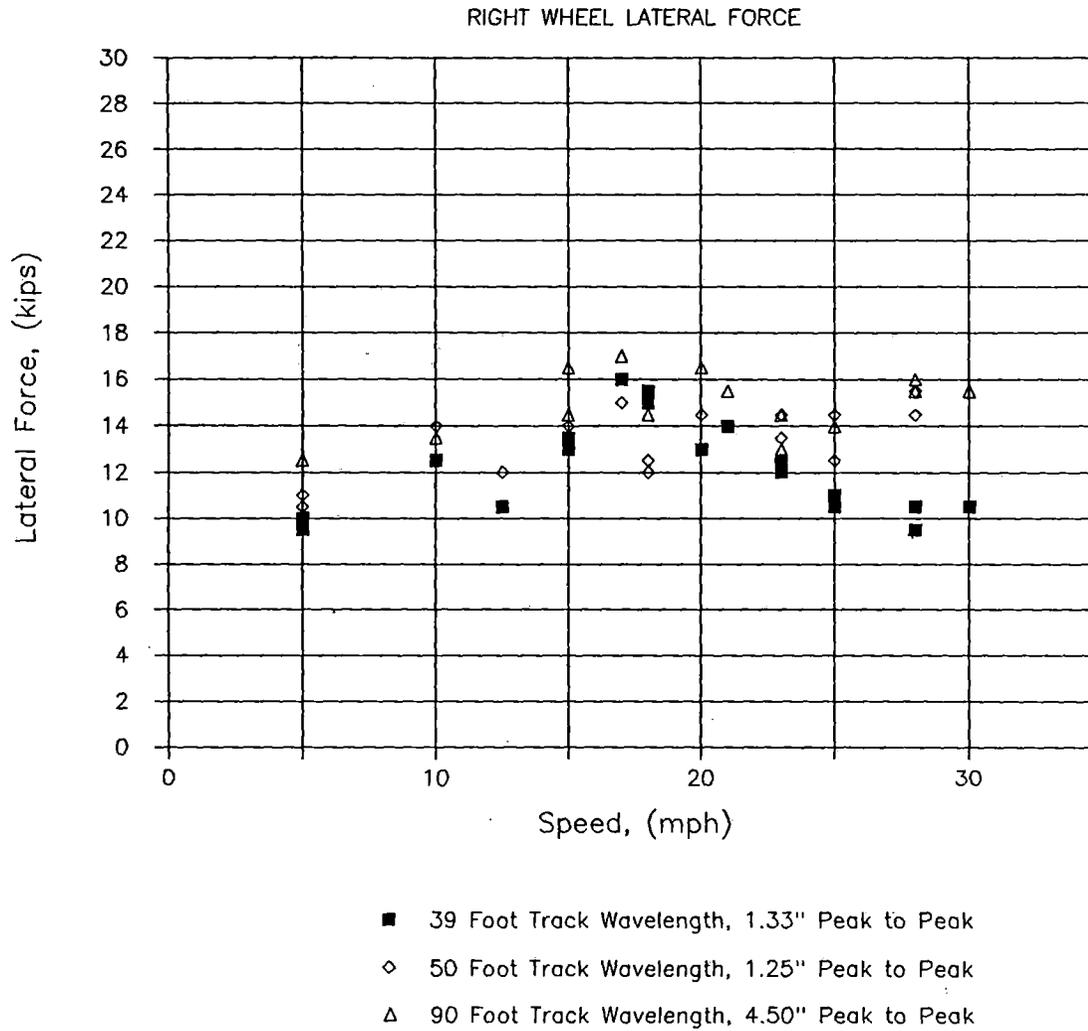
**FIGURE 4-2 TEST AT BENNINGTON, NH - HOPPER CAR**
