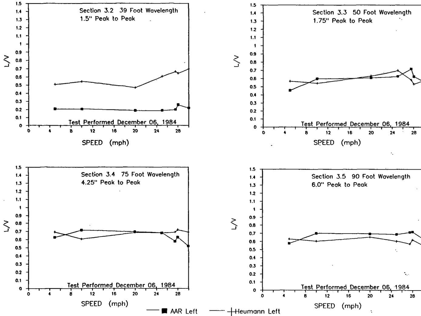
**FIGURE 3.4-5 LOADED FLAT CAR - PEAK LATERAL TO VERTICAL WHEEL FORCE RATIOS AT INTERMEDIATE SPEED TEST SECTION**
