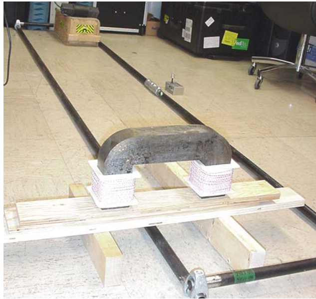
Figure 5. 1:3 scaled down model with actual transmit and receive coils
