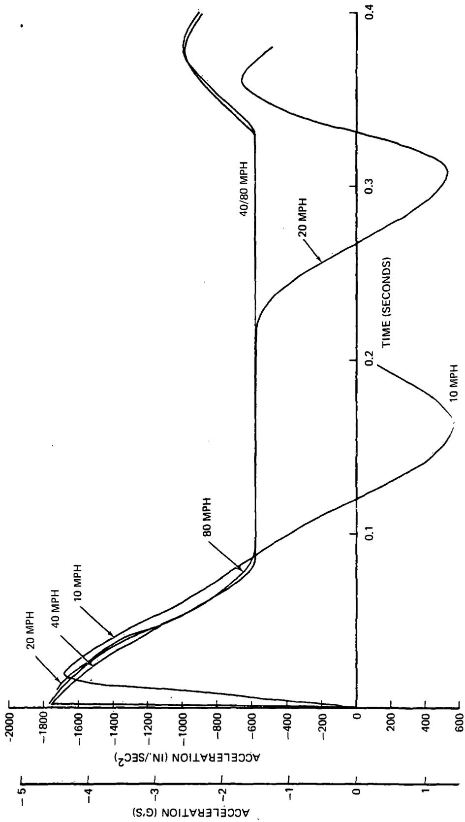
Figure 3-1. Freight Train Locomotives in Head-On Collision: Acceleration vs Time
