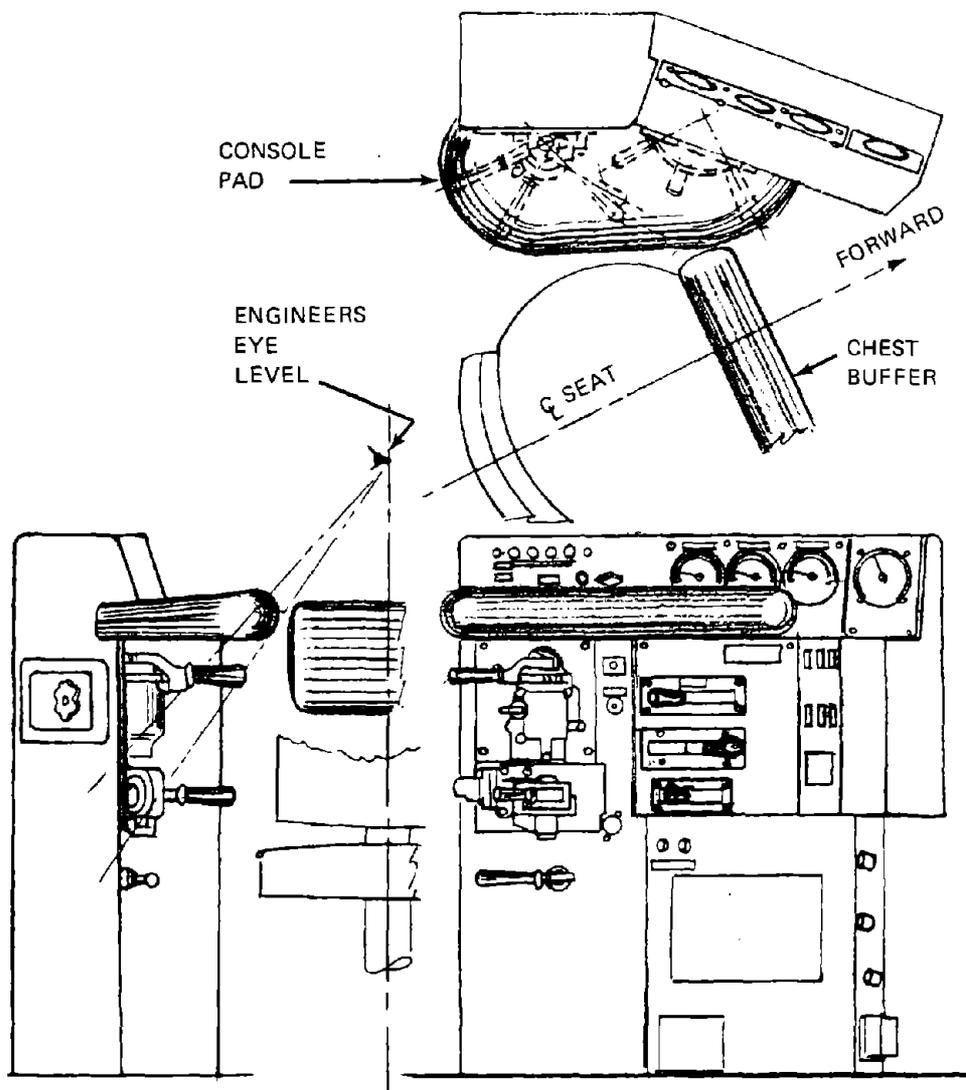
Figure 3-9. Existing Engineman's Station with Buffer and Padding
