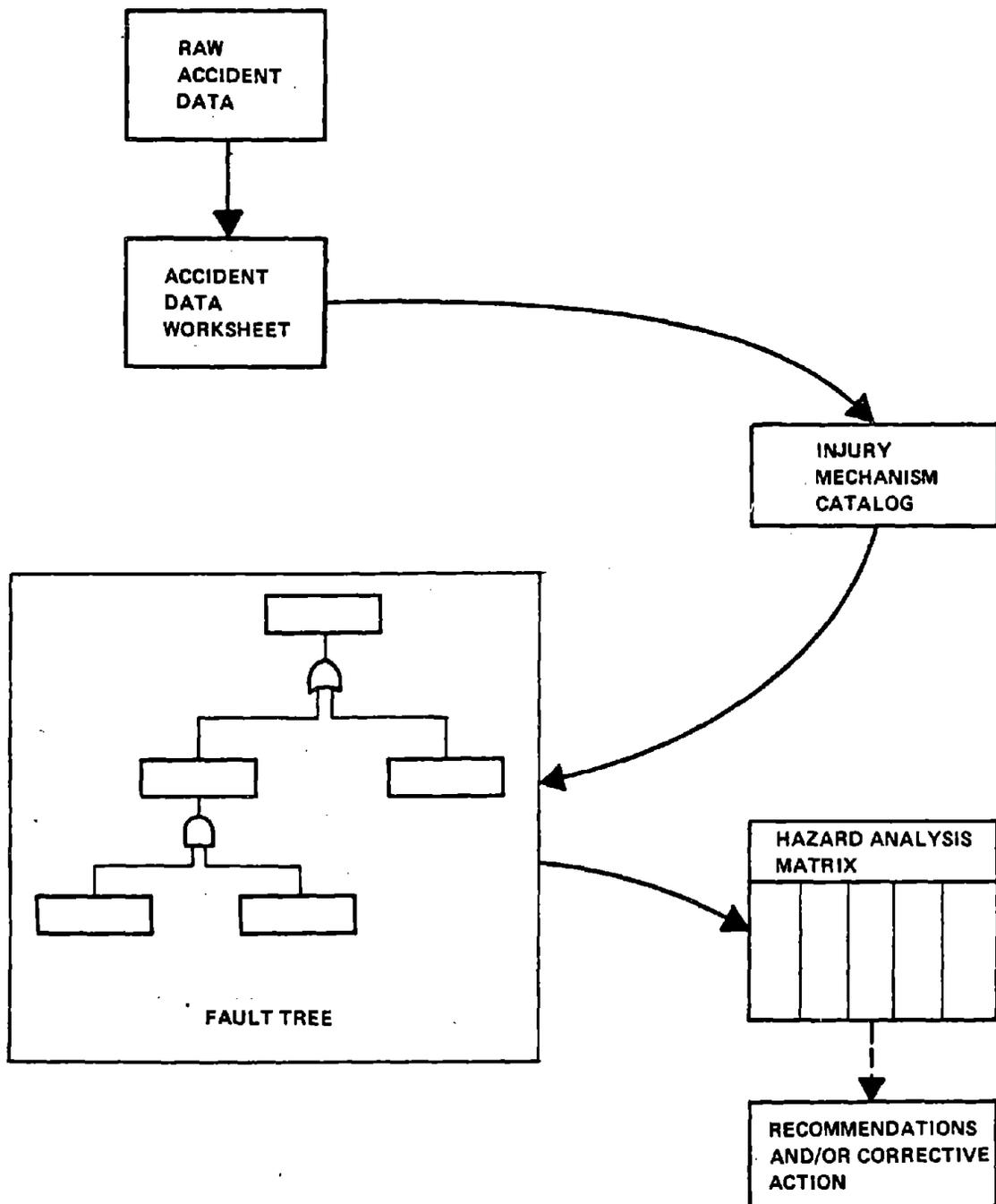
Figure 2-2. Safety Analysis Procedure Used for the Rail Injury Minimization Program
