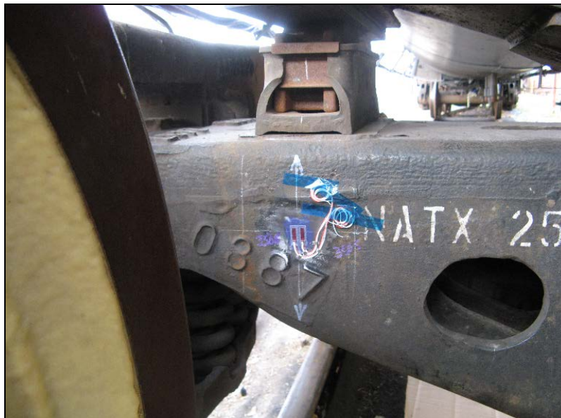
Figure 7. Strain Gauges Measuring Bolster Side Bearing Loads
