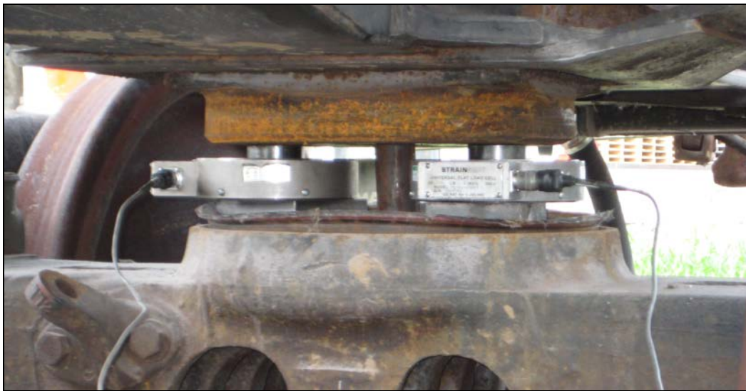
Figure 20. Center Bolster Force Calibration
