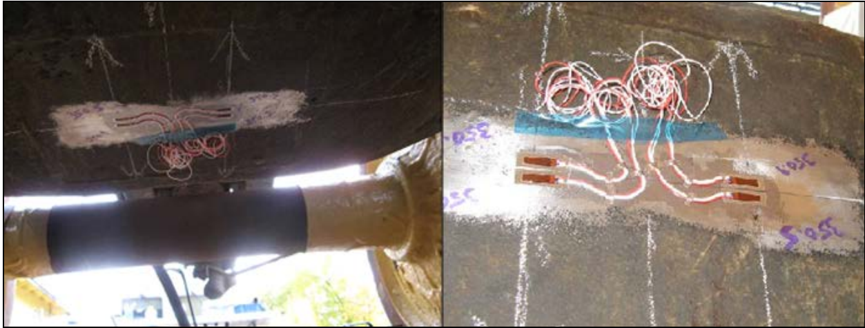
Figure 8. Strain Gauges Measuring Bolster Center Bowl Load
