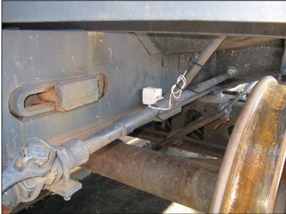
Figure 10. Vertical Accelerometer Mounted on the Stub Sill and Each End of the Car
