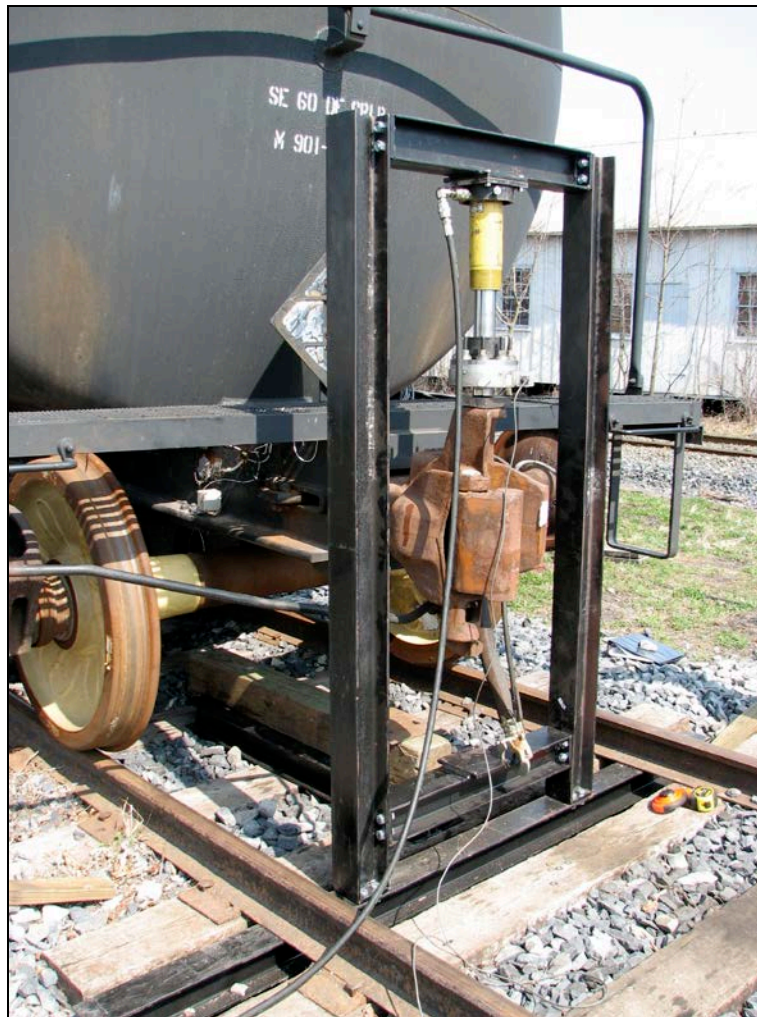
Figure 17. Vertical Coupler Force Calibration
