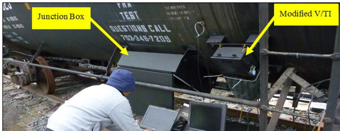
Figure 15. Modified VTI and Junction Box
