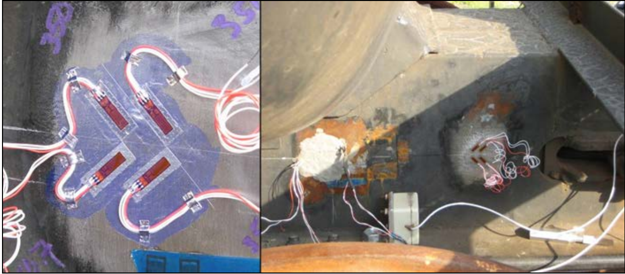
Figure 6. Shear Gauges Measuring Vertical Coupler Force
