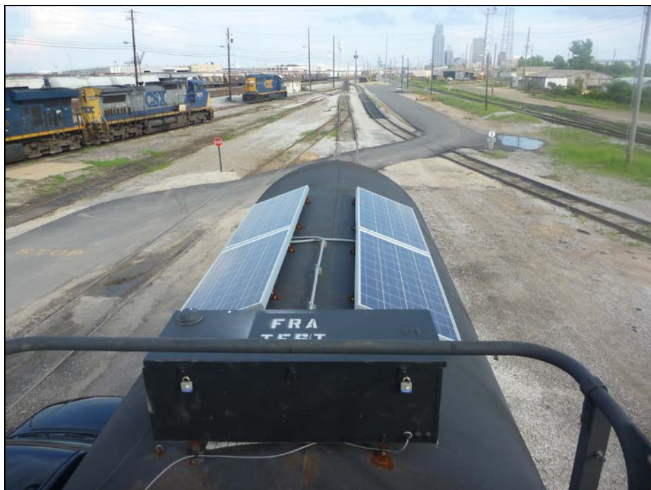
Figure 16. View of Solar Panels and Battery Box
