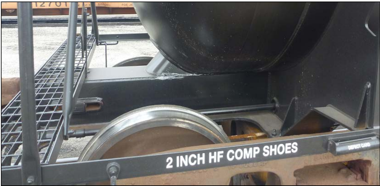
Figure 2. Detail View of the Stub Sill and Head Brace Attached to the Tank
