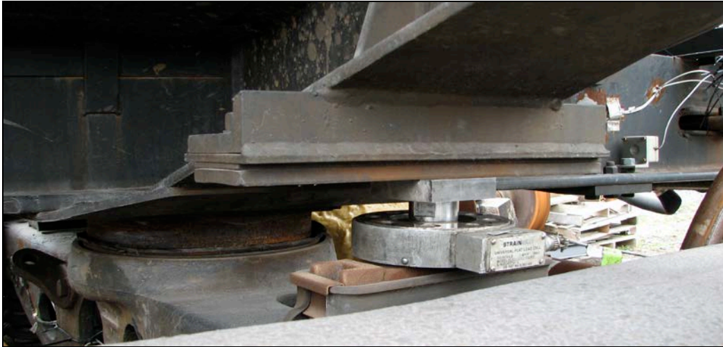
Figure 19. Side Bolster Force Calibration
