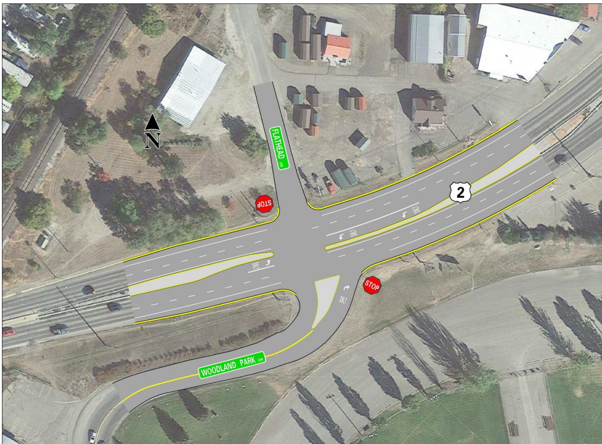
Figure 5, Existing Flathead Drive/US Highway 2 Intersection Configuration
