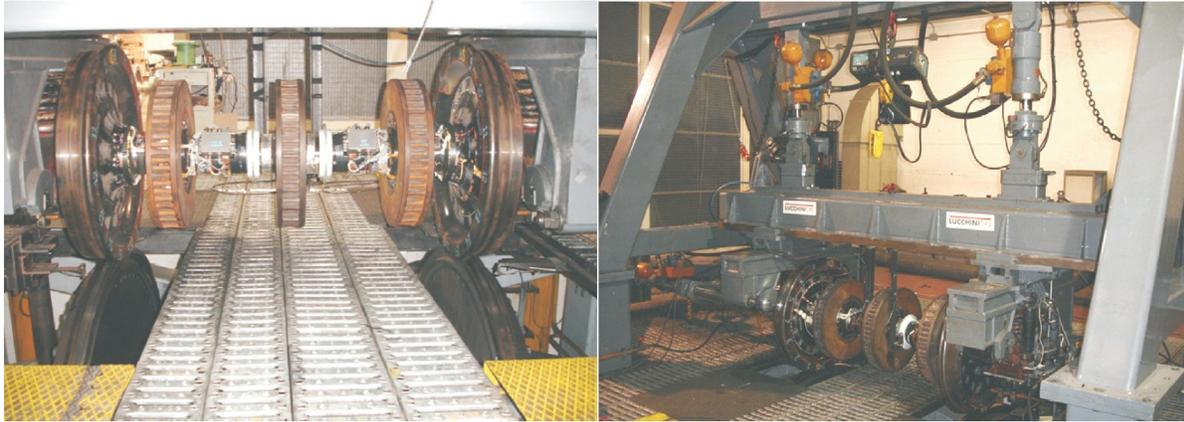
**Figure 57: A full-scale wheelset on rail rollers test rig at Lucchini [85].**
