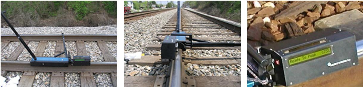
Figure 59: The Salient push-tribometer<sup>5</sup> is widely used internationally.
