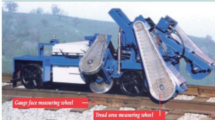
**Figure 63: The Surveyor™ simultaneously measures friction at the top and gage face of both rails using four separate measuring wheels [88].**
