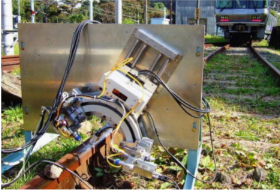
**Figure 9: Portable X-ray diffraction analyzer with X-ray fluorescence capability.**
