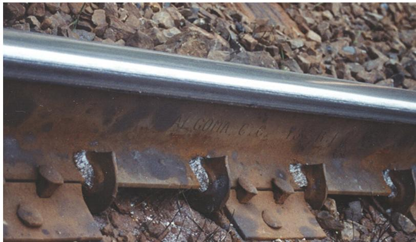
**Figure 2: In the unlubricated case, wear of the rail gage-face (and wheel flange) can be severe, with wear particles piling up around the rail fasteners**
