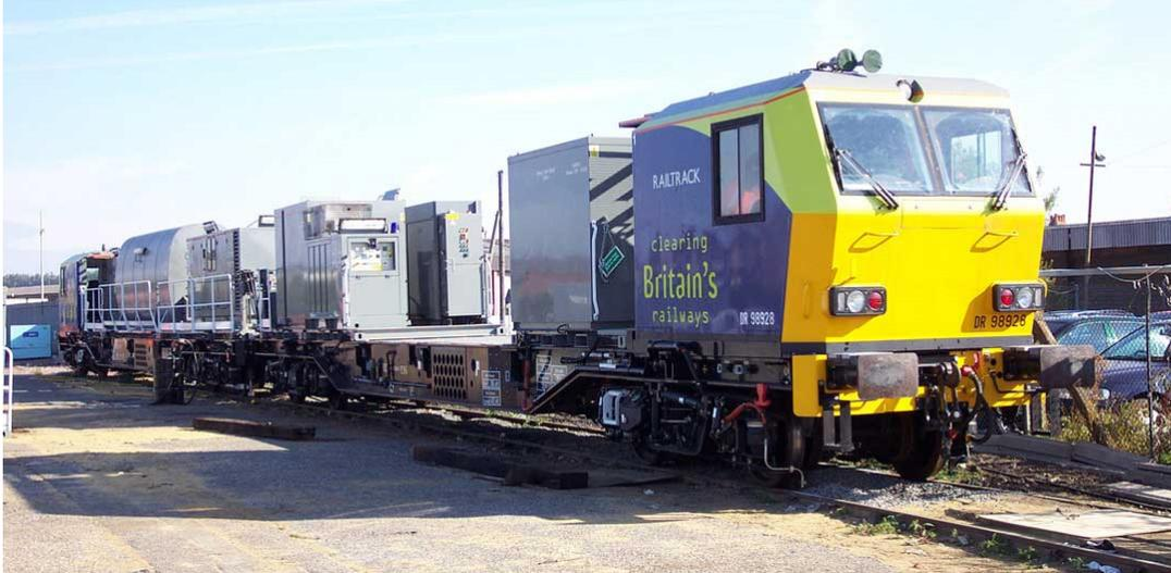
**Figure 48: The Railtrack multipurpose track cleaning vehicle.**
