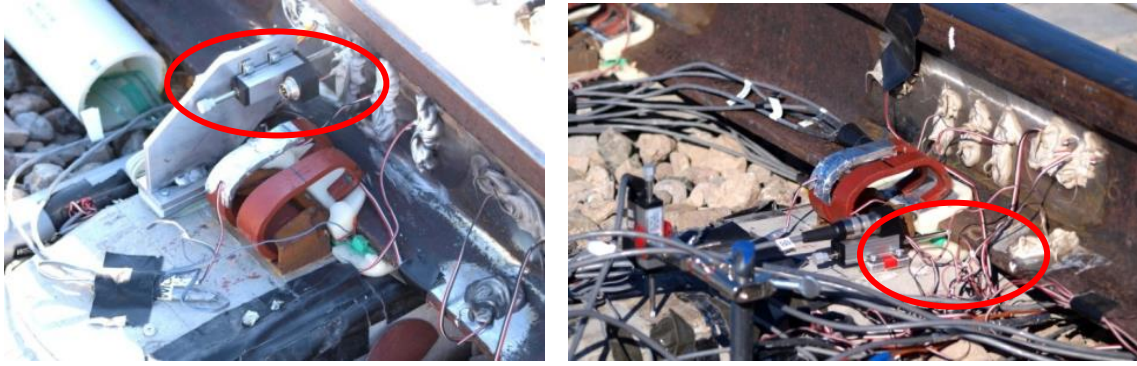
Figure 124. Position of Lateral Displacement at Rail Web [left]; Lateral Displacement at Rail Base [right]
