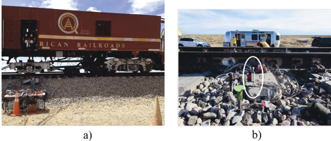
Figure 240. a) TLV Applying Controlled Wheel Load and b) Linear Potentiometers Installed to Measure Vertical Crosstie Displacement
