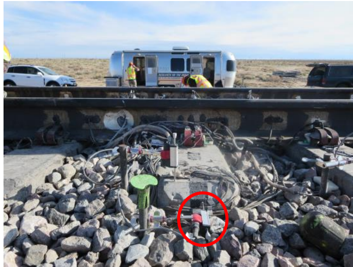
Figure 140. Lateral Crosstie Displacement Measuring Potentiometers
