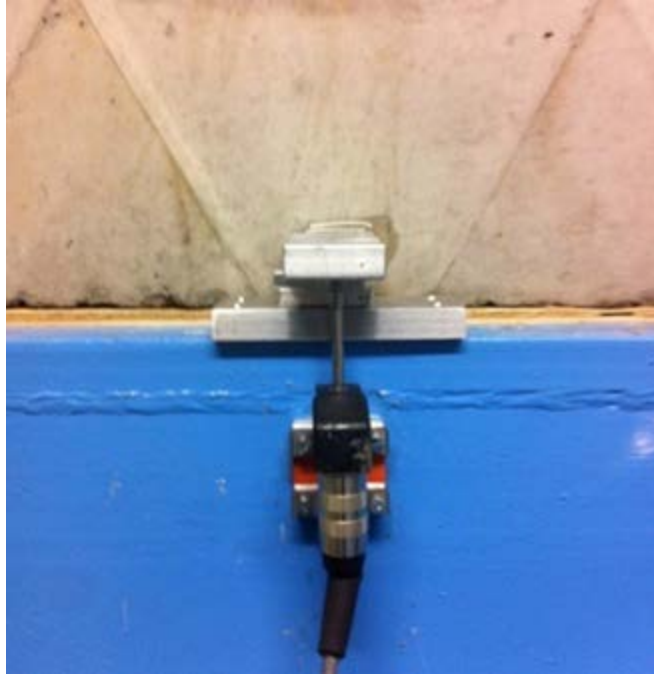
Figure 21. Linear Potentiometer Used to Measure Vertical Crosstie Displacement
