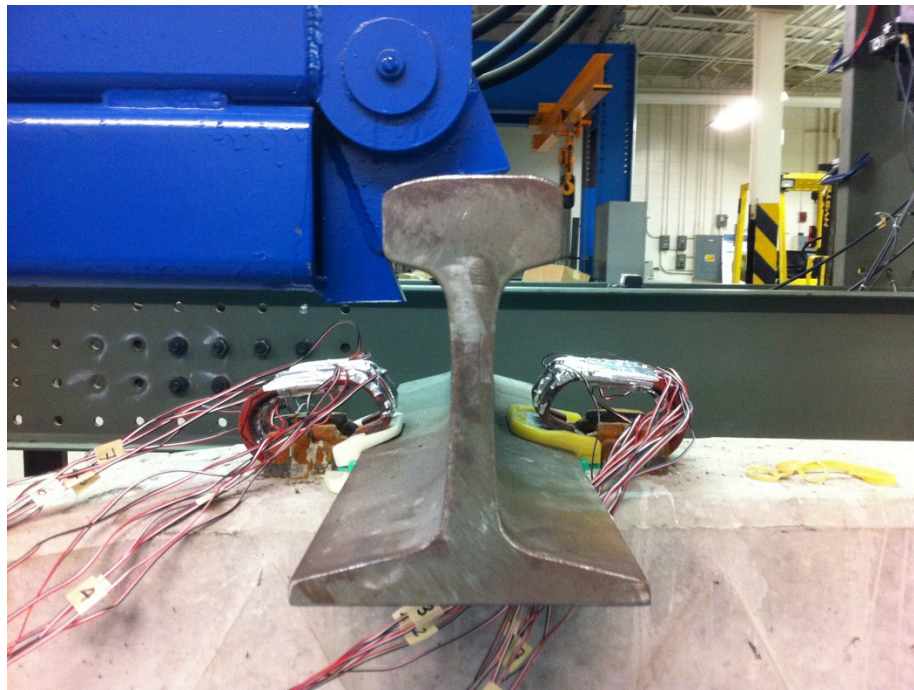
Figure 86. Instrumented Clips Used in SLTM Experimentation
