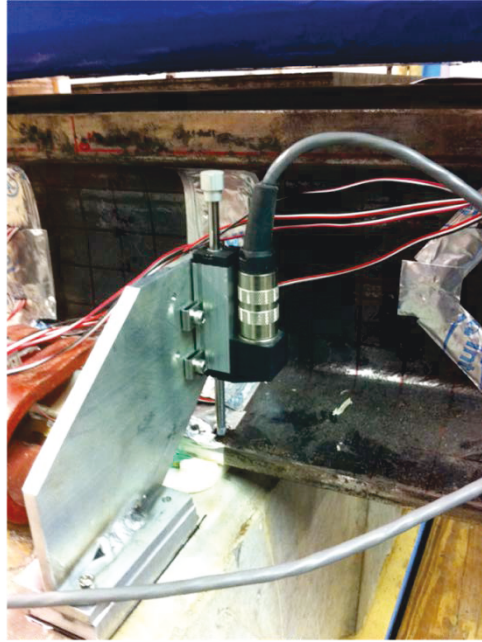
Figure 78. Potentiometers and Aluminum Fixture Used to Measure Rail Seat Vertical Displacement
