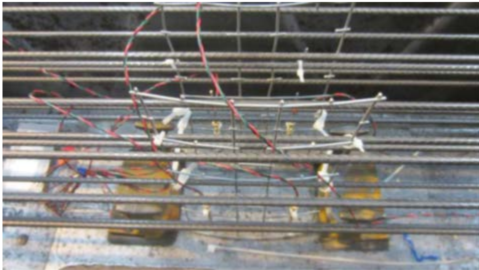
Figure 23. Mesh to Hold Embedded Crosstie Strain Gauges Prior to Concrete Being Poured
