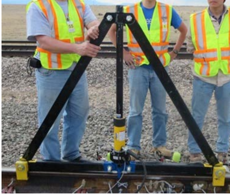
Figure 14. Delta Frame – Vertical Load Orientation
