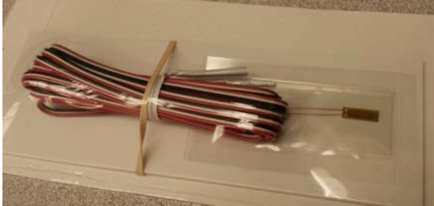
Figure 15. Standard 120-ohm Foil Type Shear Strain Gauge
