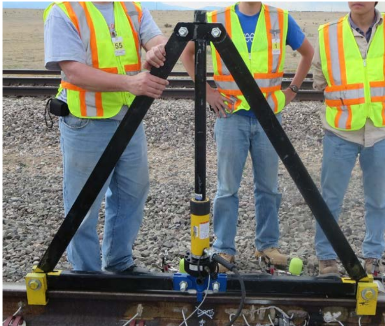
Figure 113. Delta Frame – Vertical Load Orientation
