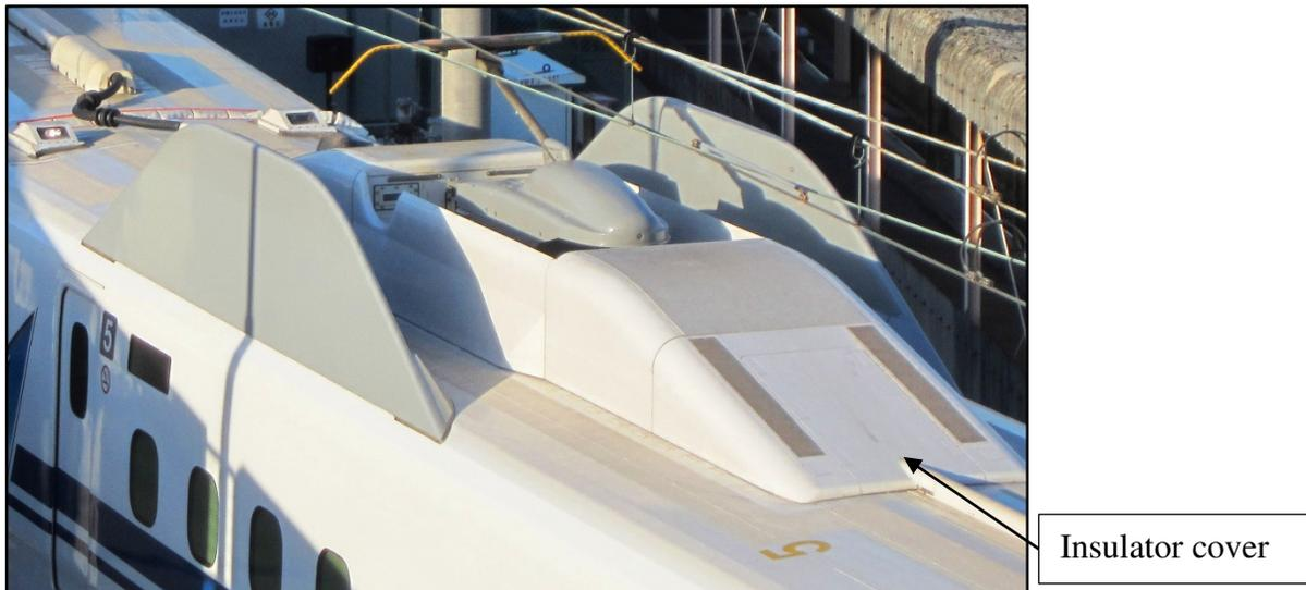
Figure 21: Shinkansen HSR Aerodynamic Pantograph
