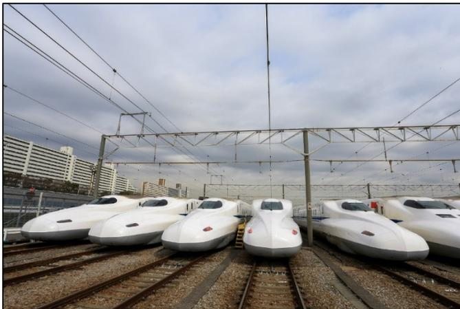
Figure 35: Typical Storage of Trainsets within a Tokaido Shinkansen Yard
