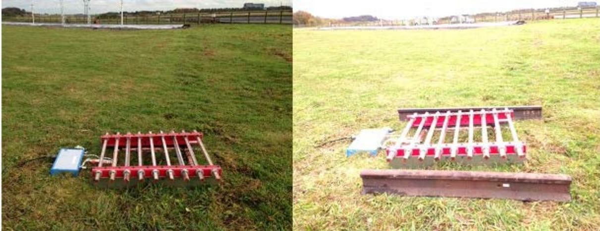
**Figure 3: TMMS sensor testing over native soil, with and without rails on each side.**
