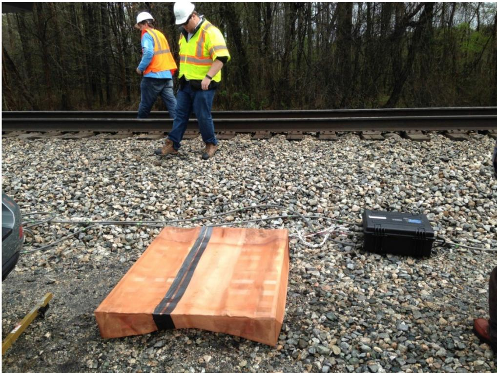
Figure 16: TMMS sensor in approximate location of test conducted on gravel access road on side of rail line.
