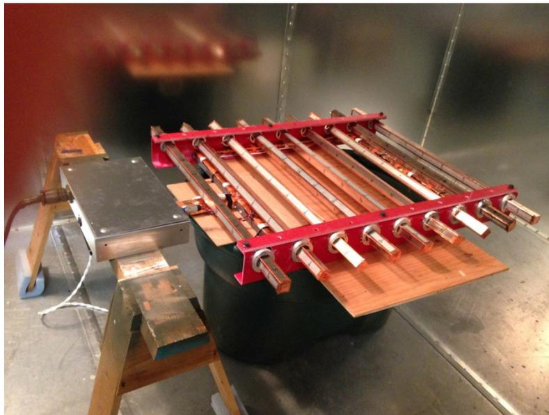
**Figure 2: Assembled magnet/coil array with first generation detection electronics in shield room, performing initial detection tests over a plastic tank full of water.**
