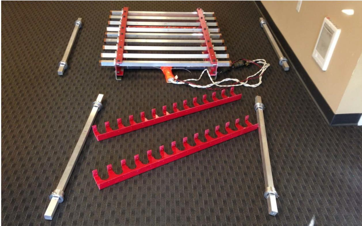
**Figure 22: Newly manufactured magnet bars and fiberglass frame components to enable the future assembly and testing of a 13-magnet version of the TMMS sensor.**
