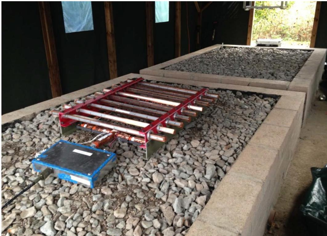
**Figure 7: Foreground: TMMS sensor taking a measurement on the “fouled” ballast box. The “clean” ballast box is visible directly behind the fouled ballast box.**
