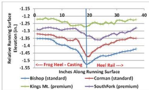
Figure 3. Longitudinal Profiles and the Frog Heel/Frog Heel-Rail Interface
