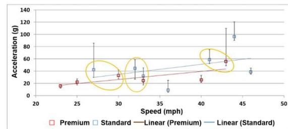
Figure 4. Acceleration Wheel Transfer Zone Over the Frog Point of the Standard and Premium Frogs on the Mainline Route
