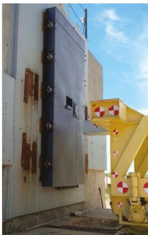
Figure 1. Test Setup: Fuel Tank Mounted on Crash Wall and Impact Vehicle
