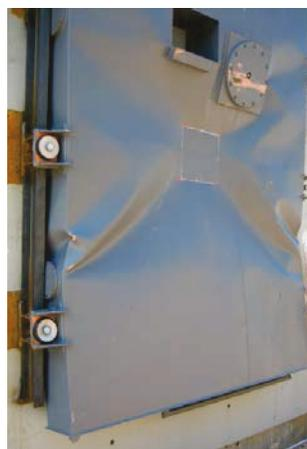
Figure 2. Post-Test Fuel Tank
