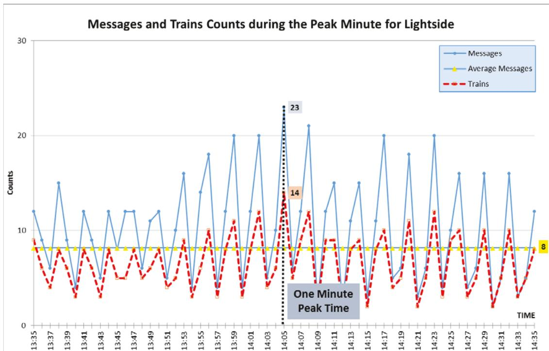
**Figure 34. Counts of Train Messages/Minute During the 1-Hour Window Around the Peak Period for Base Station Lightside**
