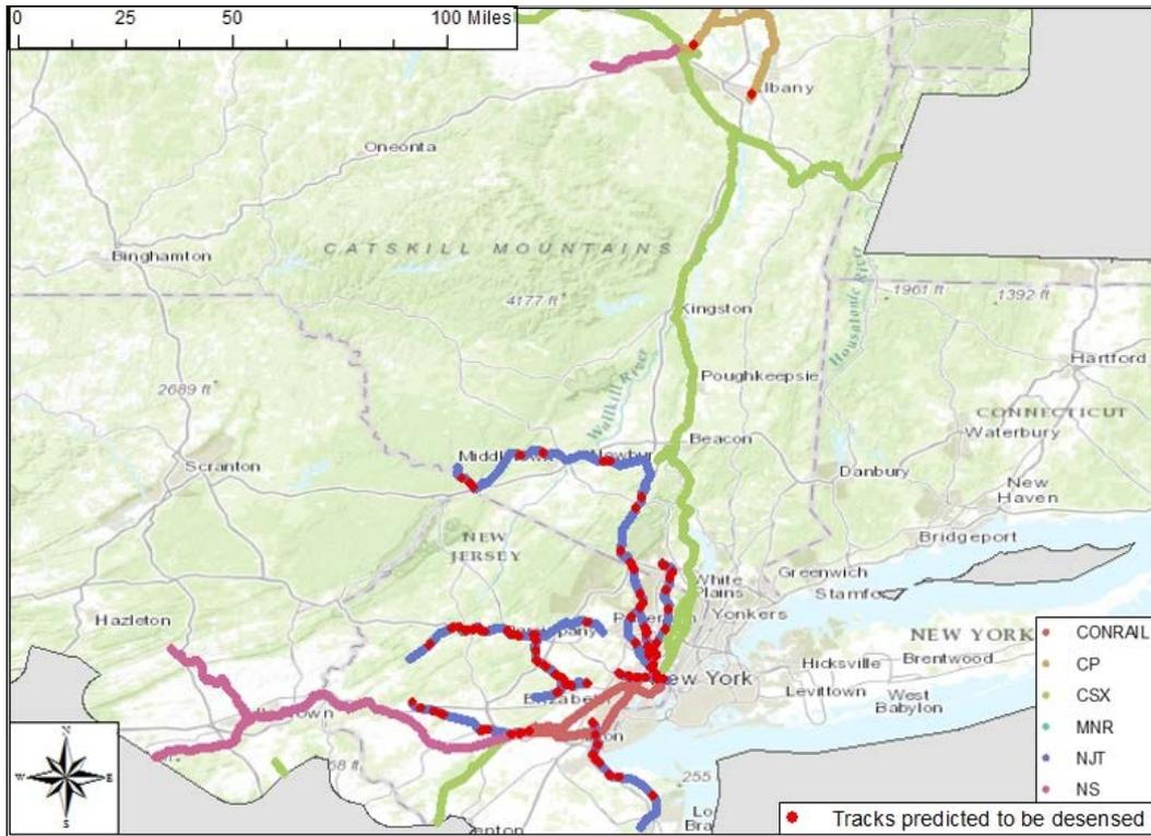
**Figure 24. Location of ITC-Controlled Tracks Predicted to be Desensed by ACSES Base Stations in the New York DUA**
