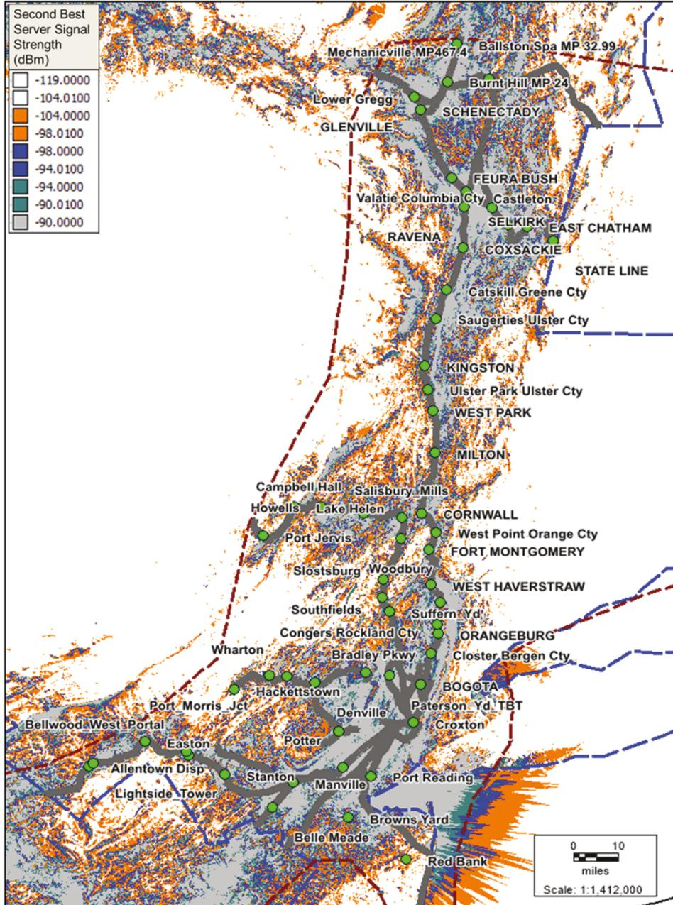
**Figure 31. Predicted Second Best ITC Base Station Server Signal Strength for the New York DUA**
