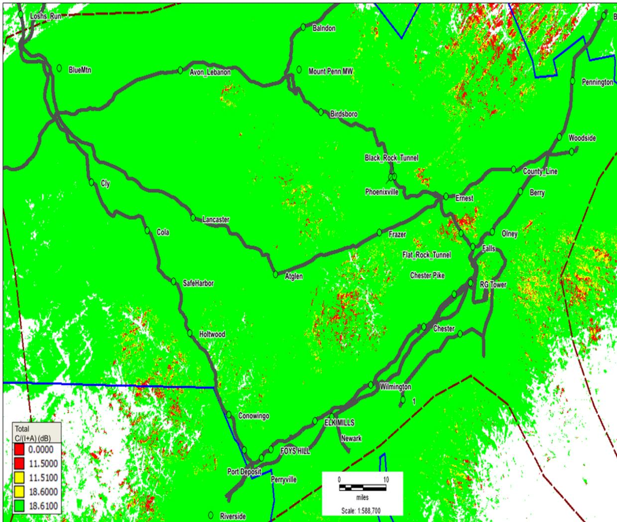
**Figure 51. Predicted C/(I+A) Levels of the Base Station Frequency Plan Prepared for the Philadelphia DUA**
