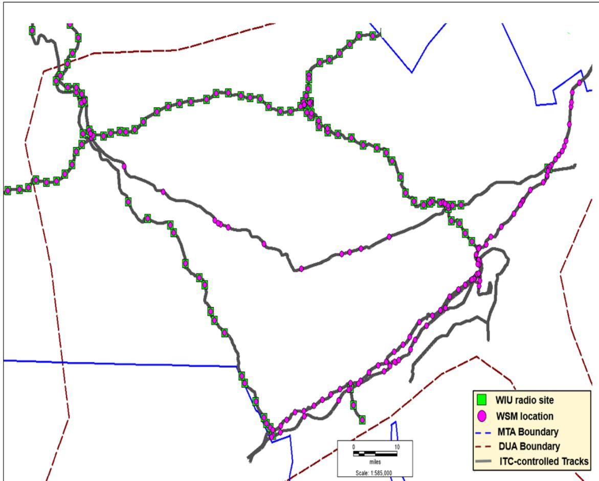
**Figure 53. WSM and WIU Radio Locations Inside the Philadelphia DUA**
