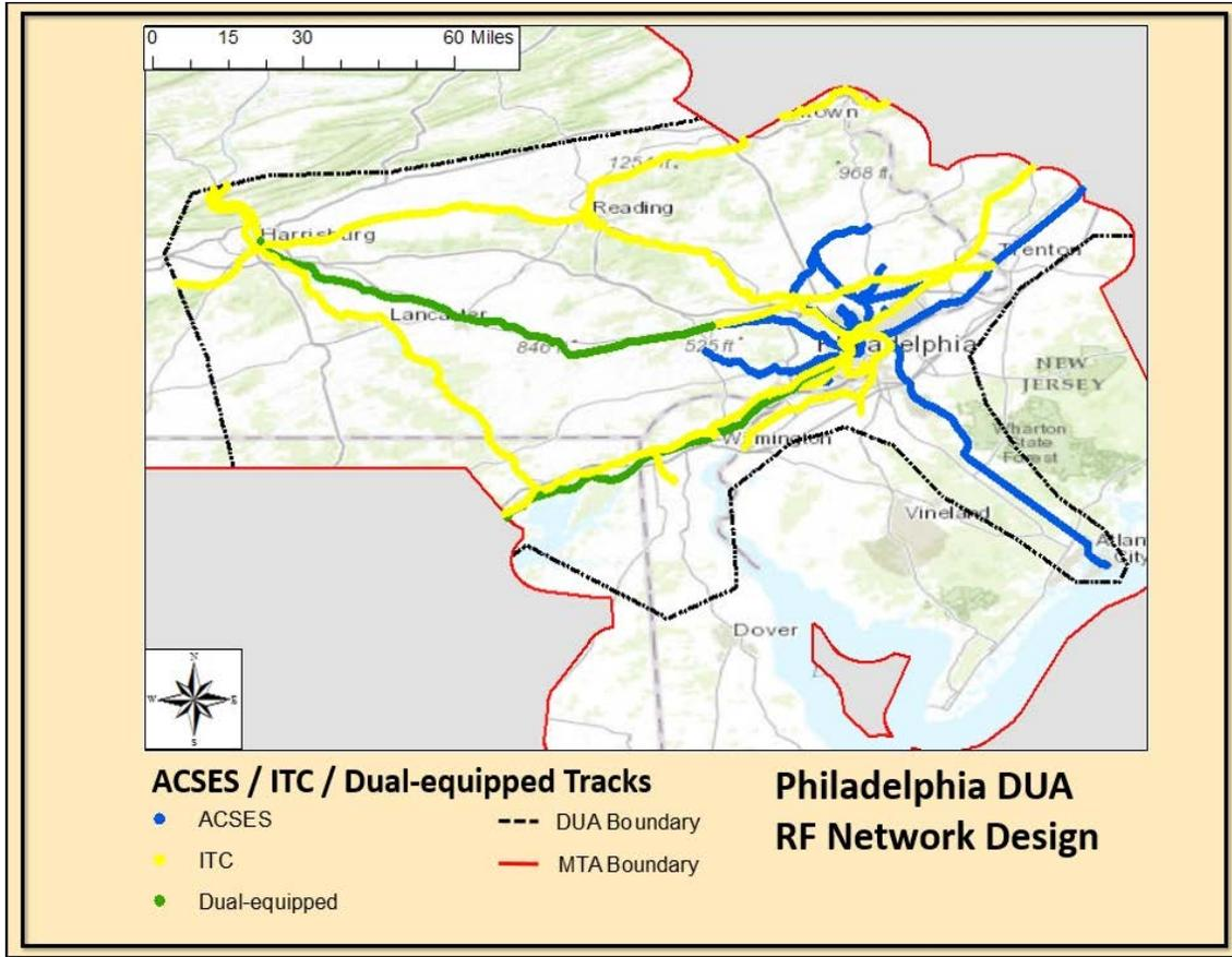
**Figure 39. ACSES, ITC and Dual-Equipped Tracks in Philadelphia DUA**
