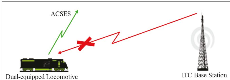
**Figure 5. Illustration of a Dual-Equipped Locomotive Self-Desense**
