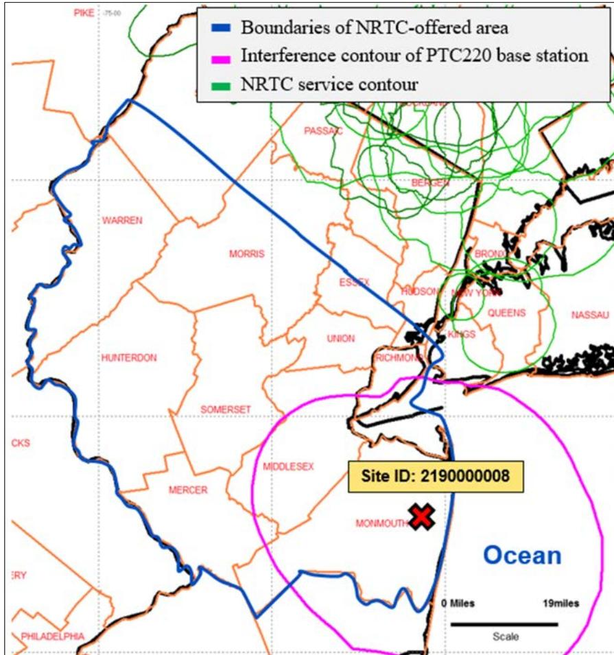
**Figure 14. Evaluation of the Usability of NRTC Spectrum for ITC Site 2190000008 with Modified Configuration (Antenna Azimuth at 180 Degrees)**
