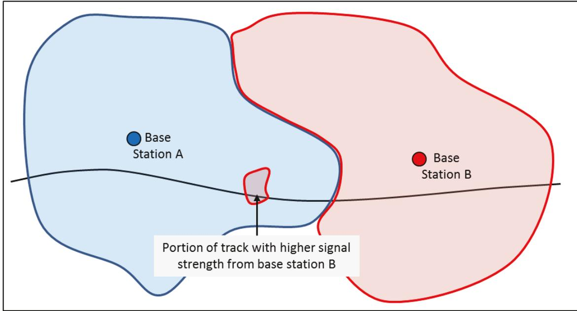
**Figure 11. Typical Base Station Coverage Case Handled by TTCI's Smoothing Algorithm**
