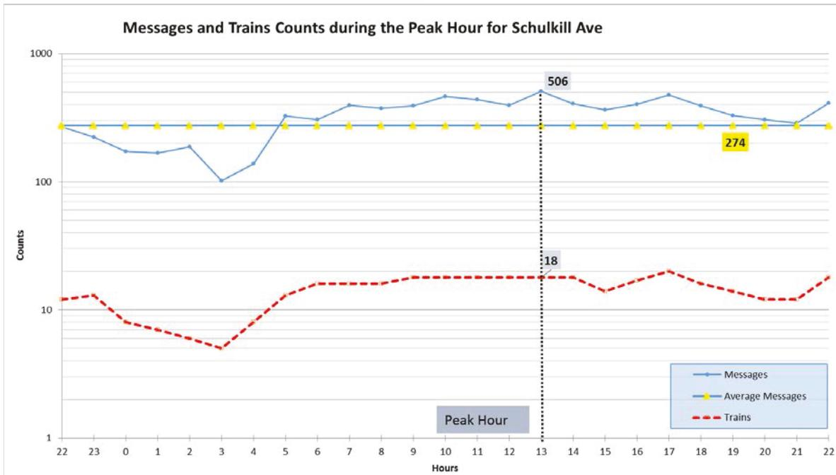
**Figure 57. Counts of Train Messages/Minute During the 24-Hour Around the Peak Period for Base Station Schukill Ave**
