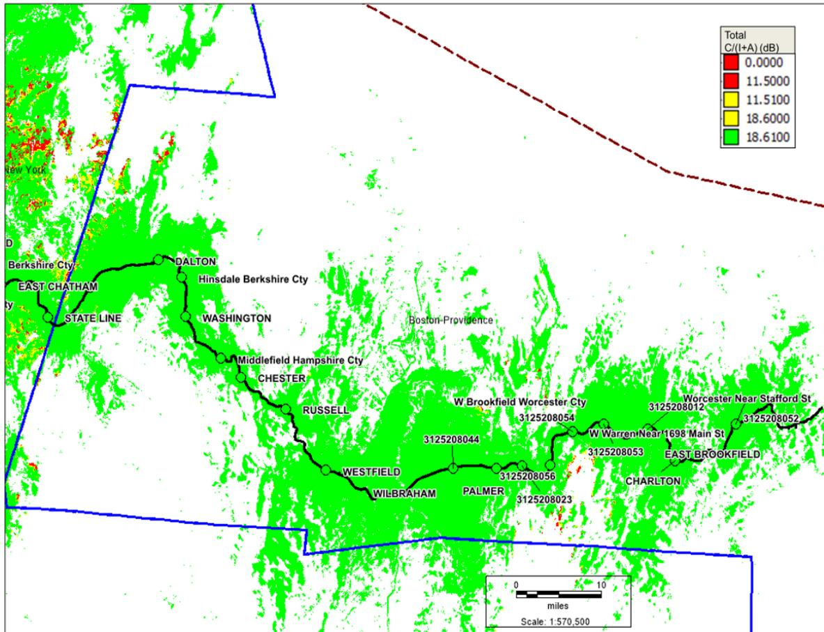
**Figure 85. Predicted C/(I+A) Levels of the ITC Base Station Frequency Plan Prepared for the Boston DUA**
