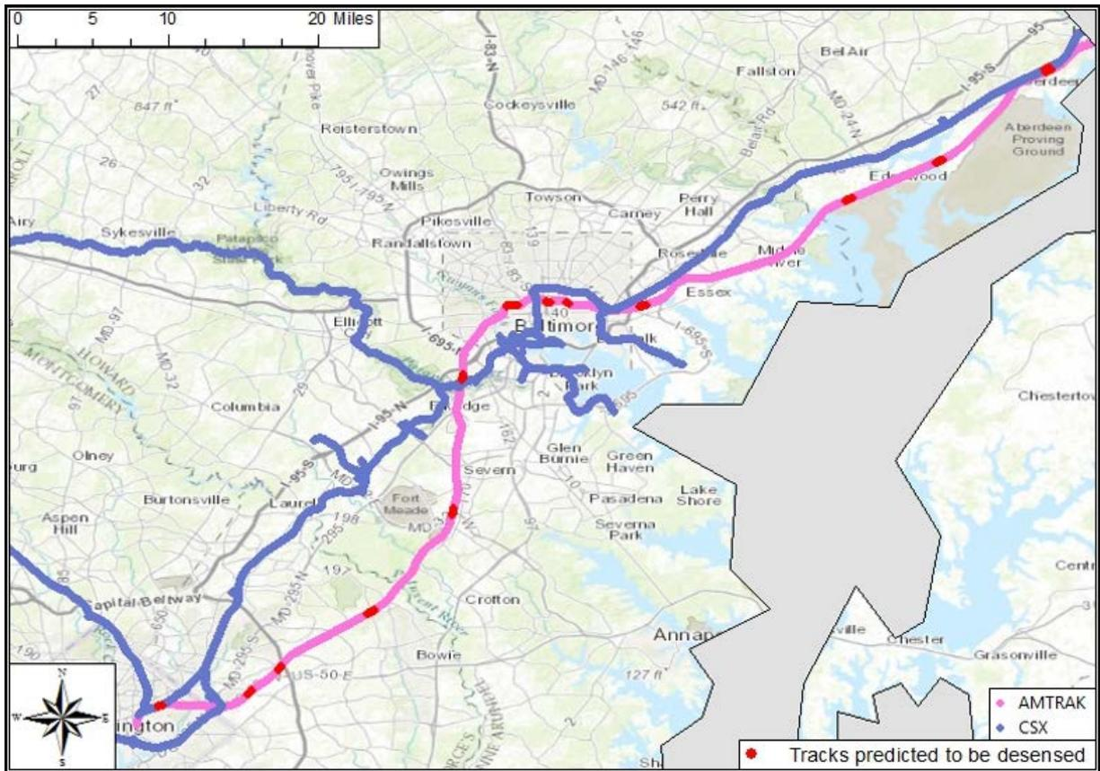
**Figure 66. Location of ITC-Controlled Tracks Predicted to be Desensed by ACSES Base Stations in the Washington, D.C. DUA**
