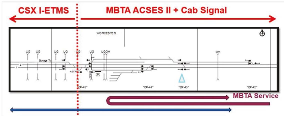
**Figure 79. Illustration of the Transition Area Between CSX and MBTA at CP45**
