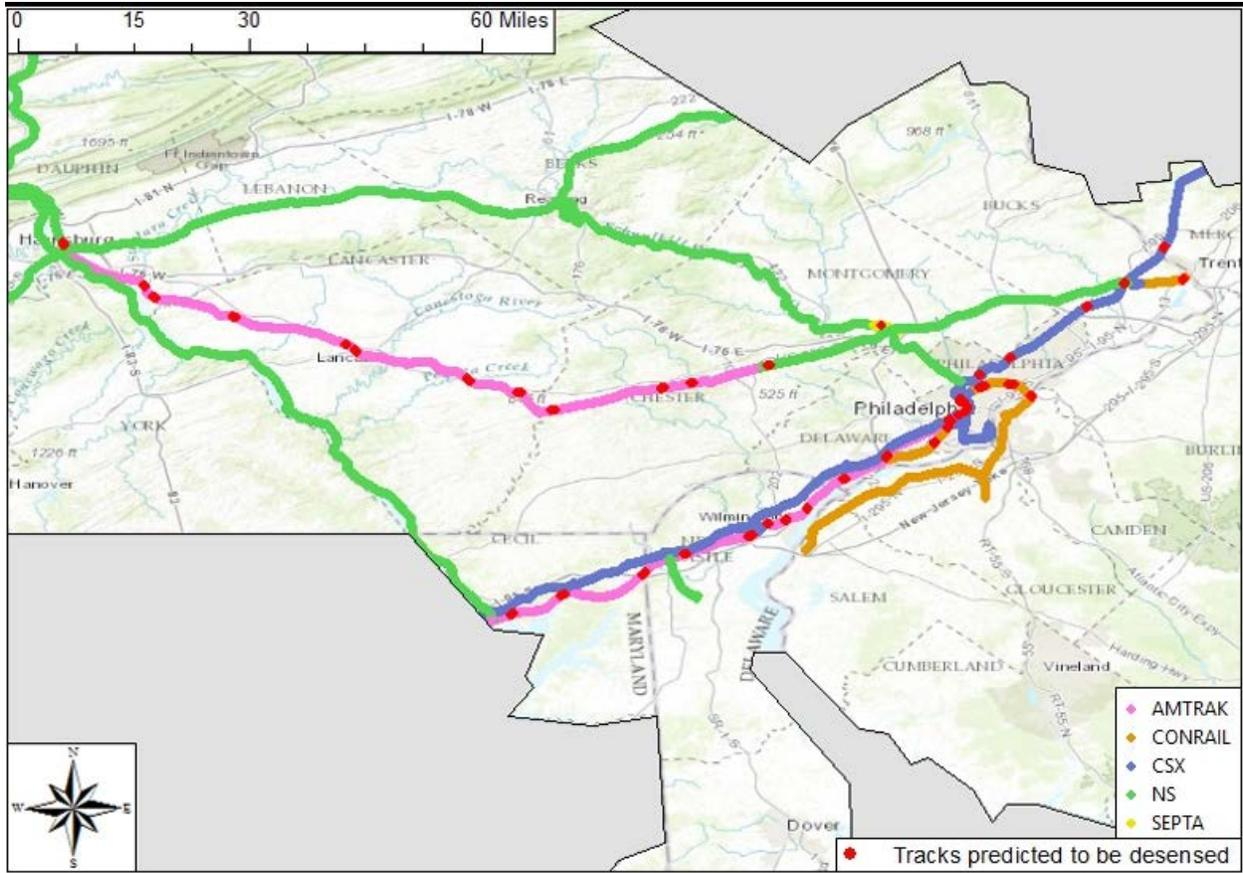
**Figure 45. Location of ITC-Controlled Tracks Predicted to be Desensed by ACSES Base Stations in the Philadelphia DUA**
