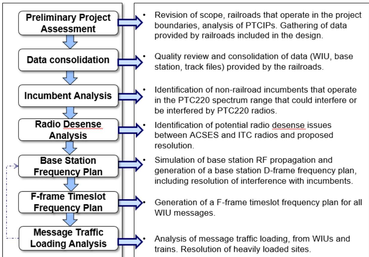
Figure 9. Macro Steps of TTCI's RF Network Design Methodology
