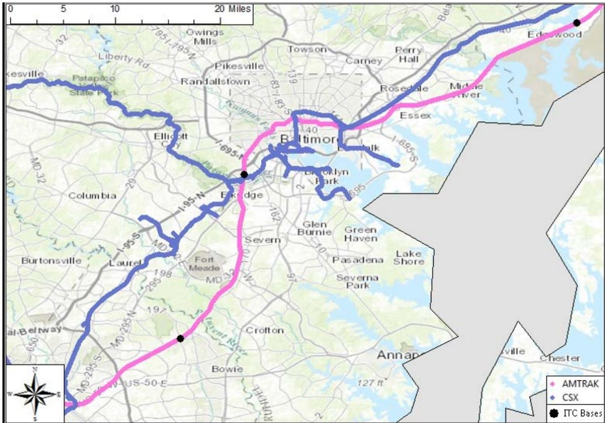
**Figure 64. Location of ITC Base Stations Predicted to be Desensed by ACSES Base Stations in the Washington, D.C. DUA**
