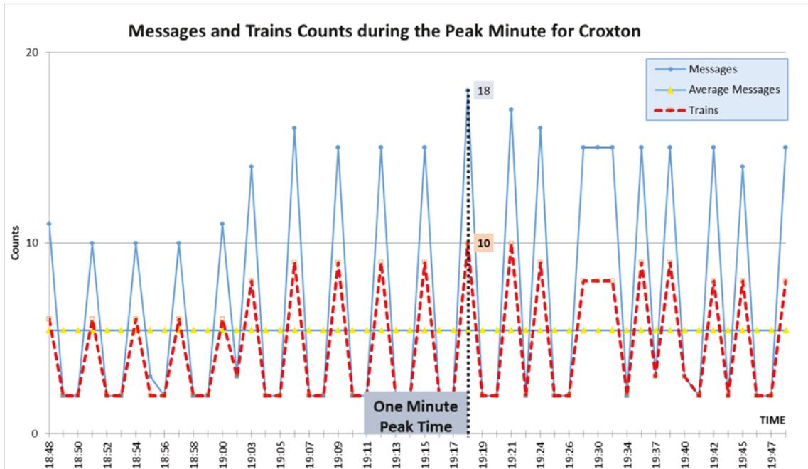
**Figure 35. Counts of Train Messages/Minute During the 1-Hour Window Around the Peak Period for Base Station Croxton**
