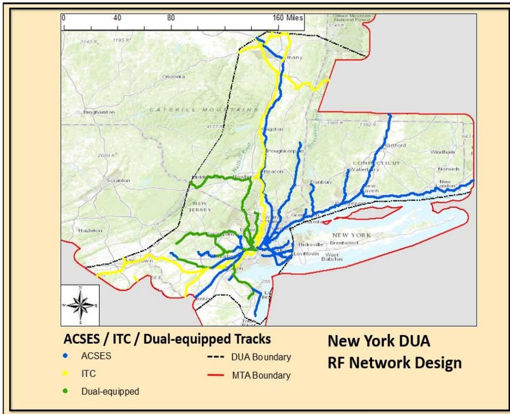
**Figure 18. ACSES, ITC and Dual-Equipped Tracks in New York DUA**
