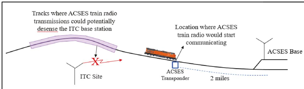
**Figure 7. Illustration of the Activation of an ACSES Locomotive Radio Distant from Tracks that Could Potentially be Desensed**
