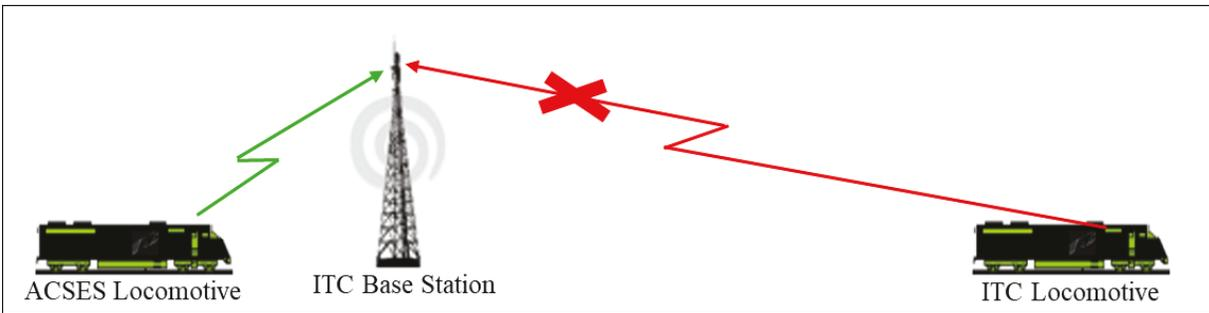
**Figure 4. Illustration of an ACSES Locomotive Desensing a Fixed ITC Site**
