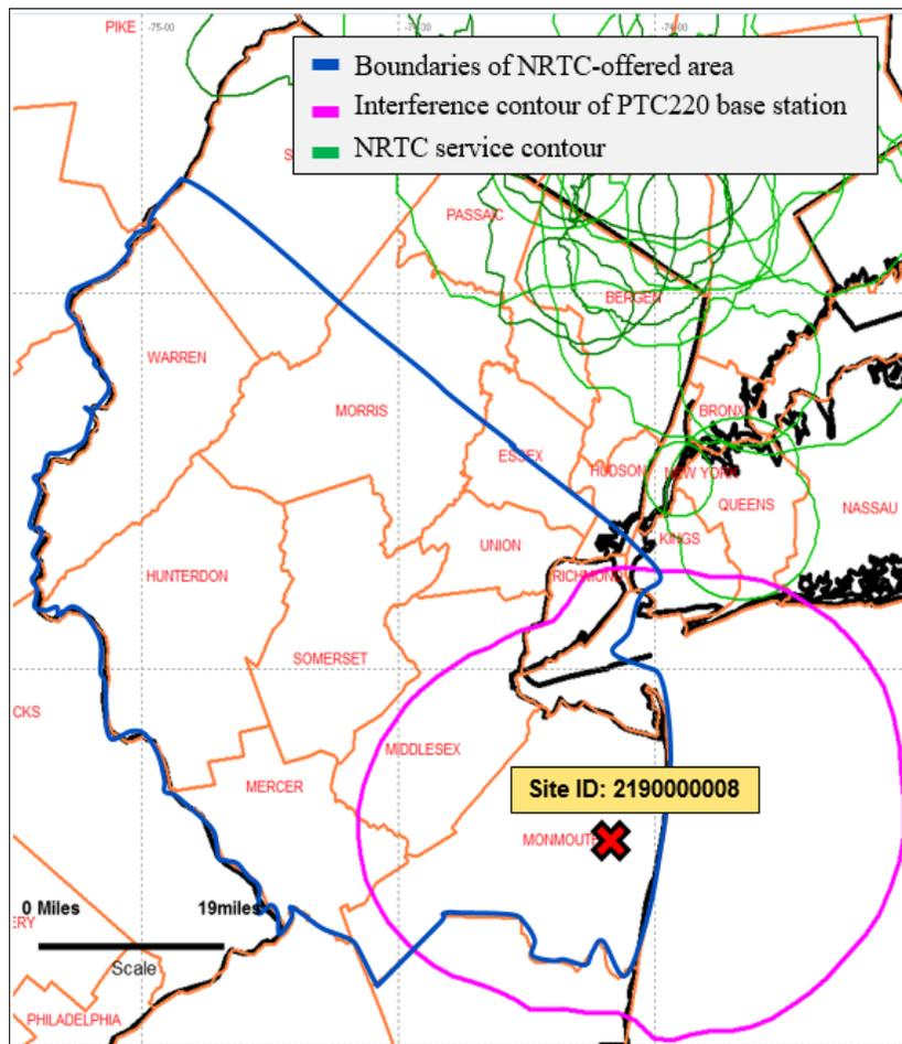
**Figure 13. Evaluation of the Usability of NRTC Spectrum for ITC Site 2190000008 with its Original Configuration (Antenna Azimuth at 0 degree)**
