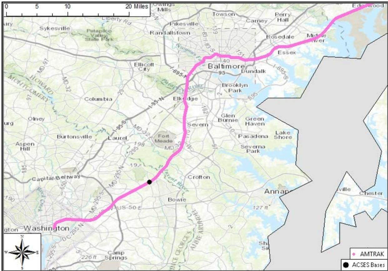
**Figure 65. Location of ACSES Base Stations Being Desensed by ITC Base Stations in the Washington, D.C. DUA**
