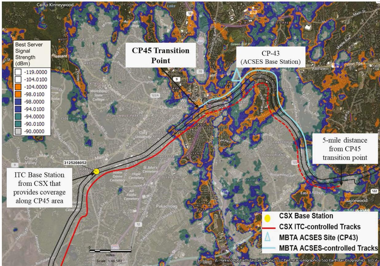
**Figure 80. Details of CP45 Transition Area Including Coverage Predictions for CSX Base Station**
