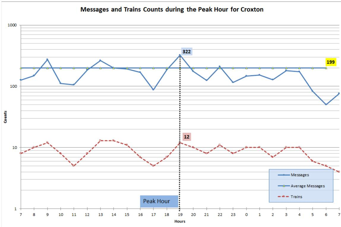
**Figure 37. Counts of Train Messages/Minute During the 24-hour Window Around the Peak Period for Base Station Croxton**
