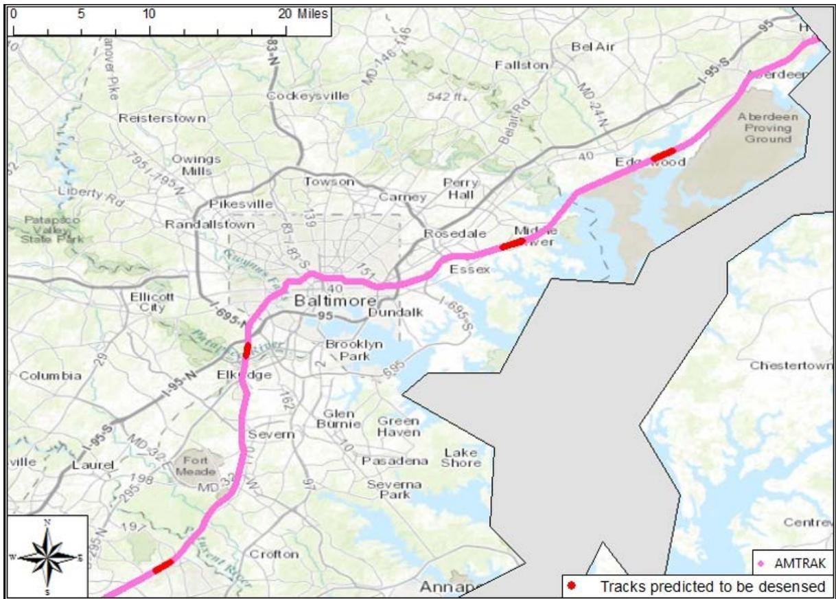
**Figure 67. Location of ACSES-Controlled Tracks Predicted to be Desensed by ITC Base Stations in the Washington, D.C. DUA**
