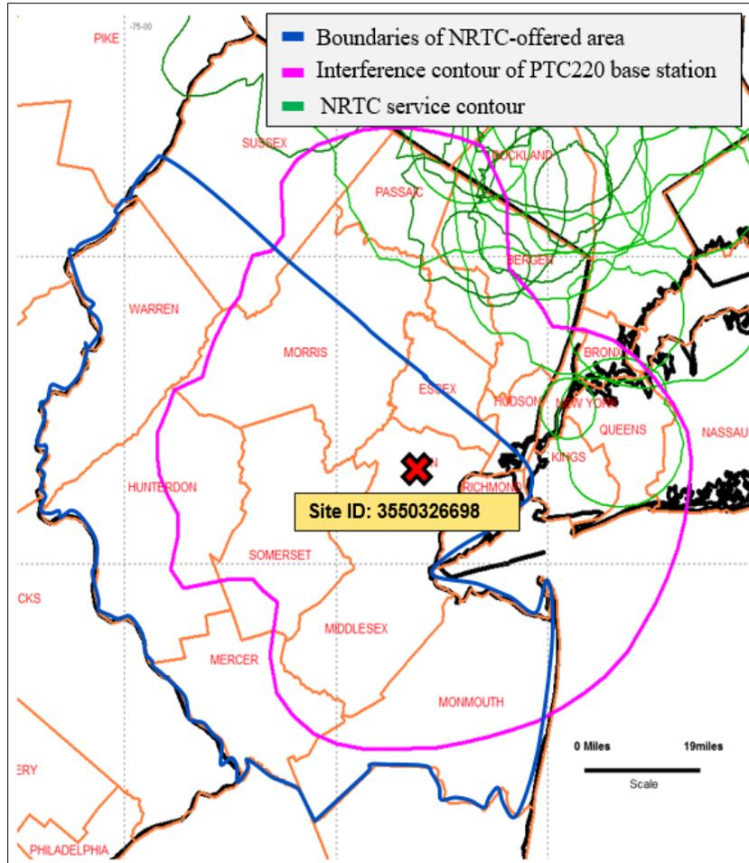
**Figure 16. Evaluation of the Usability of NRTC Spectrum for ITC Site ID 3550086698**
