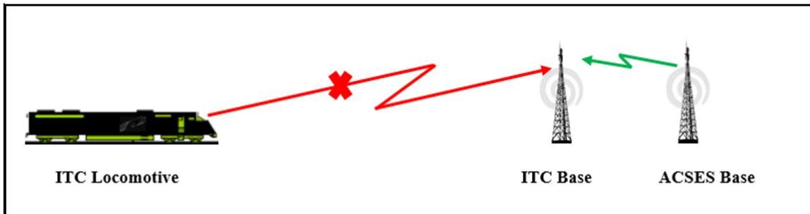
**Figure 2. Illustration of a Fixed ACSES Site Desensing a Fixed ITC Site**
