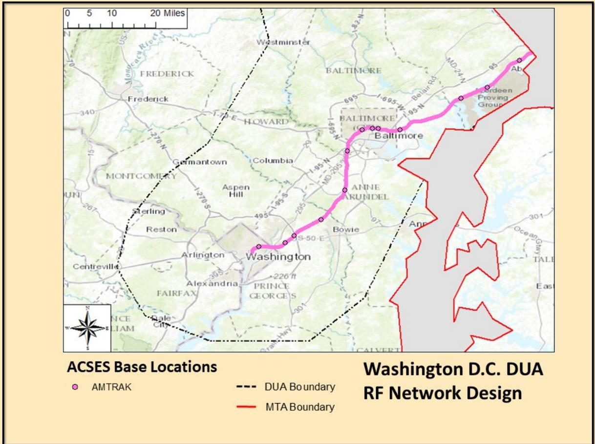
**Figure 63. Location of ACSES Base Stations and ACSES-Controlled Tracks in the Washington, D.C. DUA**
