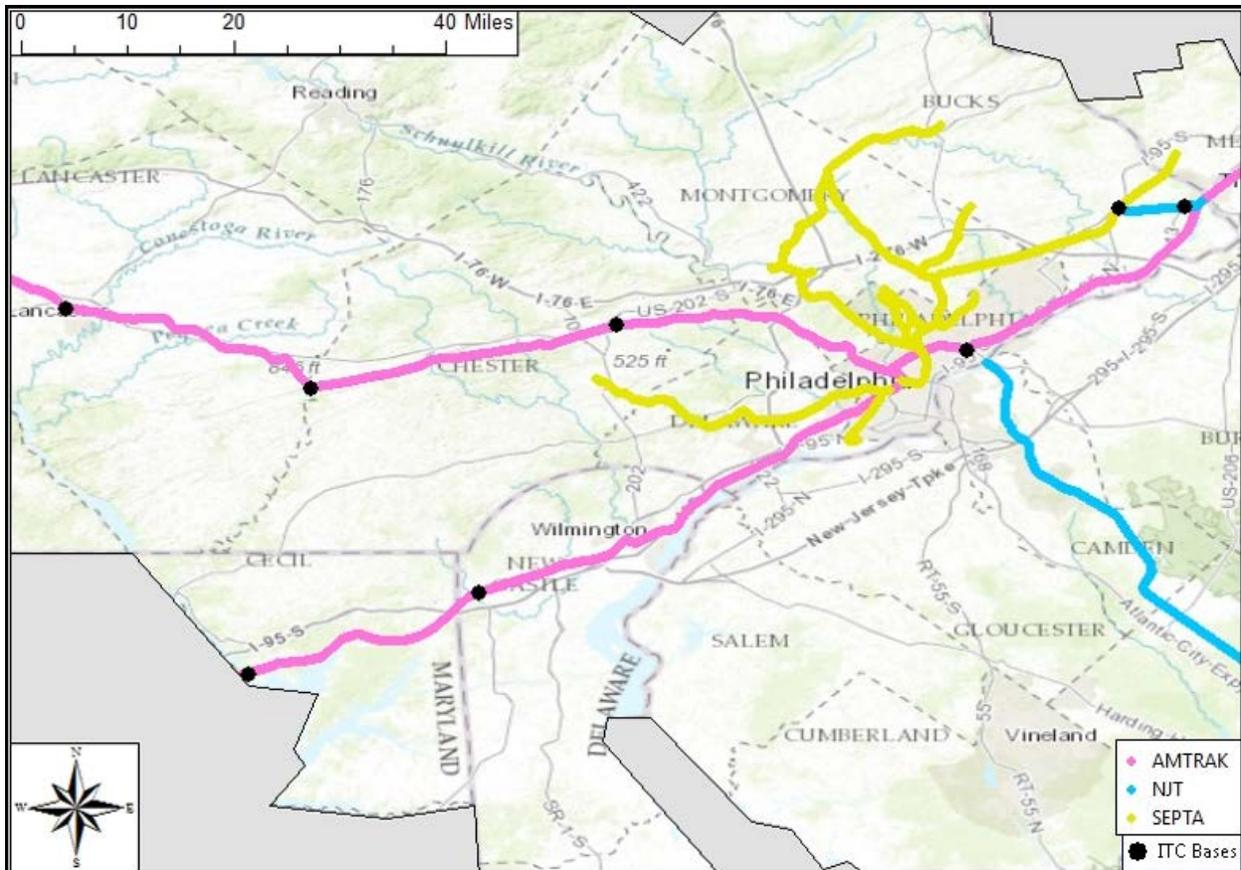
**Figure 48. Location of ITC Base Stations Predicted to be Desensed by ACSES Locomotive Radios in the Philadelphia DUA**
