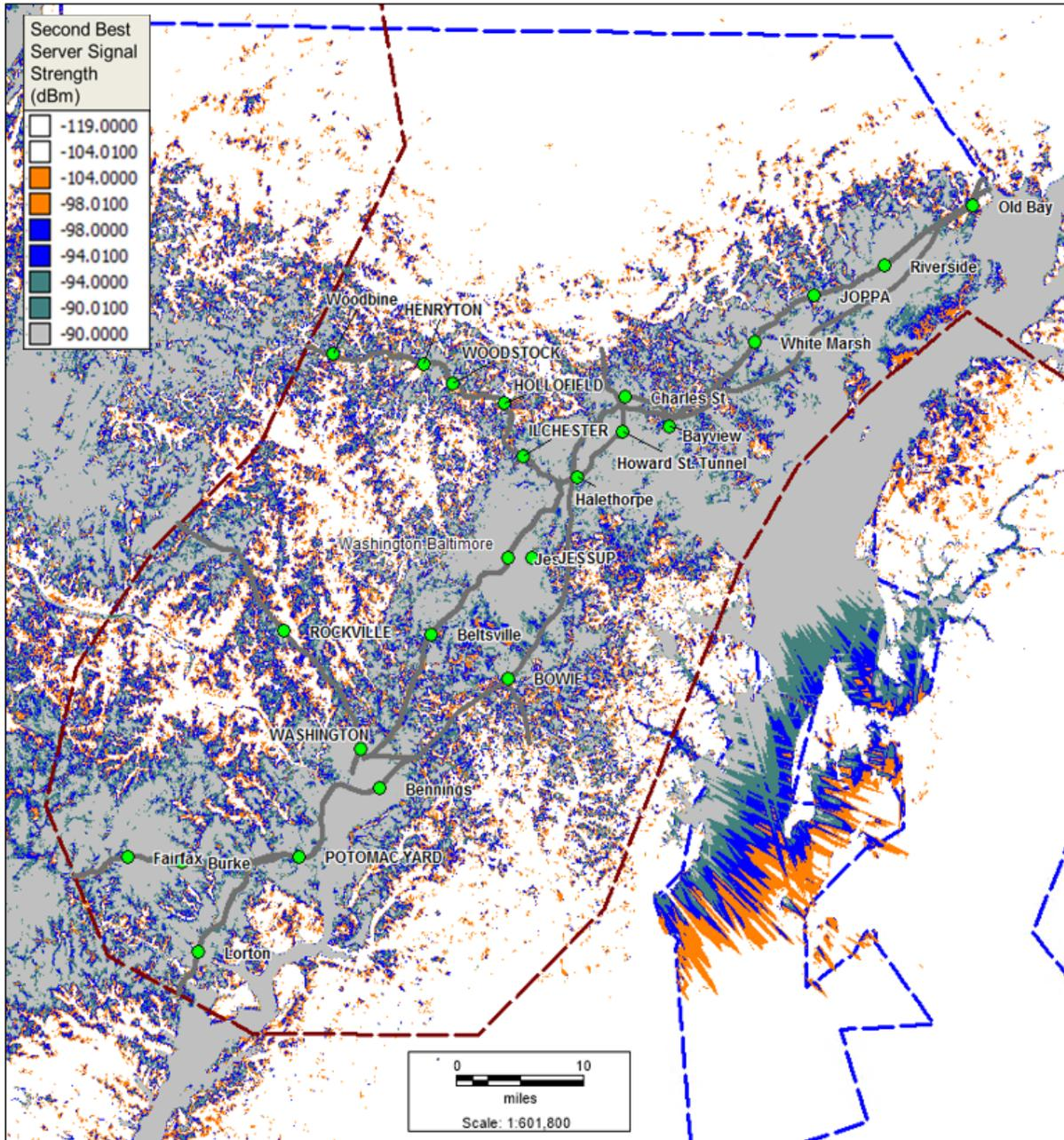
**Figure 73. Predicted Second Best ITC Base Station Server Signal Strength for the Washington, D.C. DUA**
