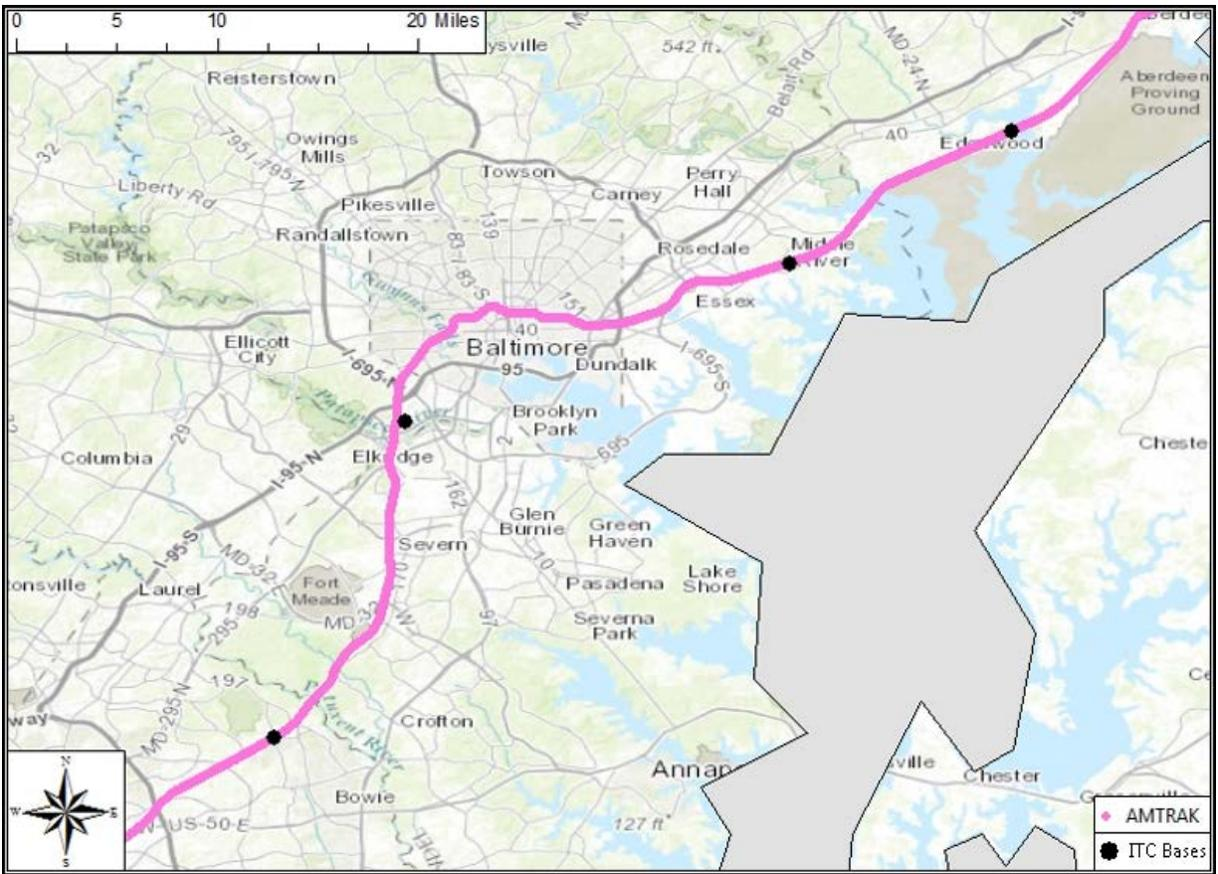
**Figure 69. Location of ITC Base Stations Predicted to be Desensed by ACSES Locomotive Radios in the Washington, D.C. DUA**
