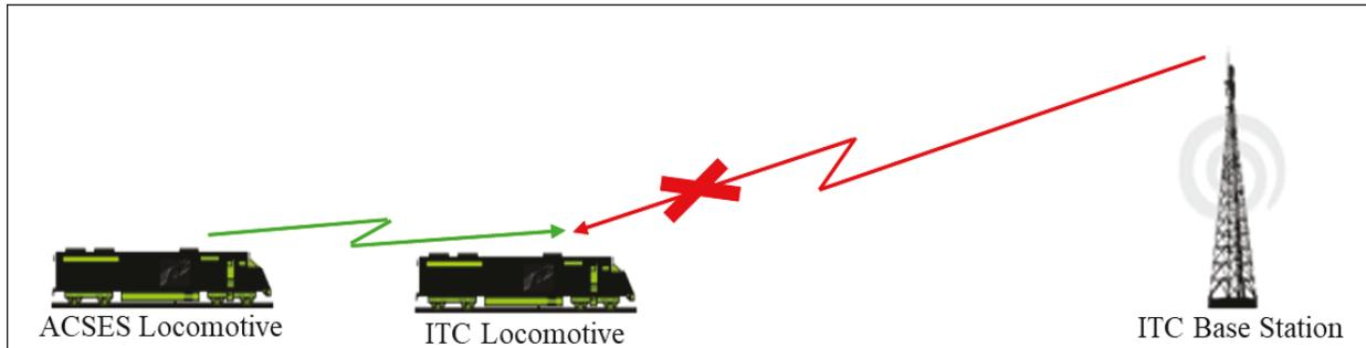
**Figure 6. Illustration of an ACSES Locomotive Desensing an ITC Locomotive**
