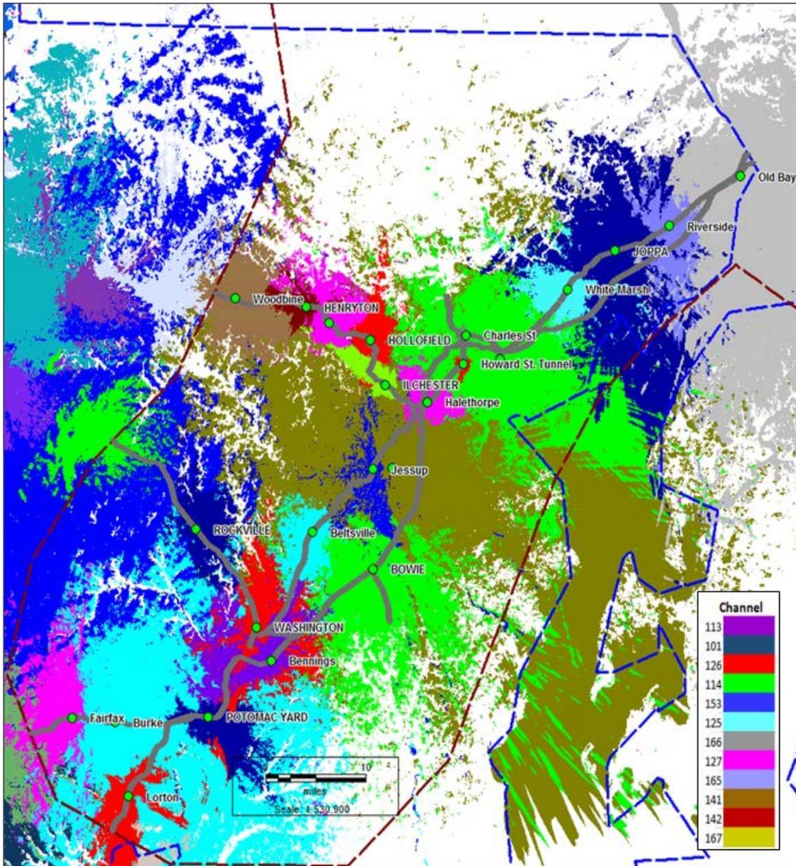
**Figure 71. ITC Base Station Best Serving Sectors for the Washington, D.C. DUA**
