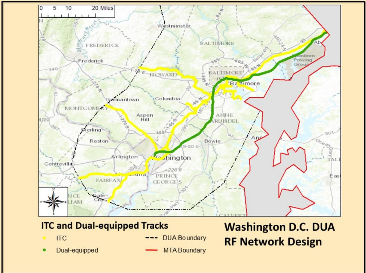
Figure 60. Visualization of ITC and Dual-Equipped Tracks in the Washington, D.C. DUA
