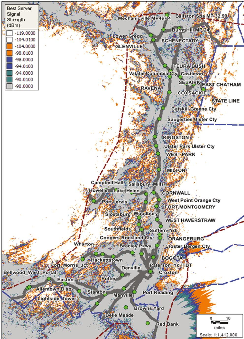
**Figure 28. Best Serving ITC Base Station Signal Strength Inside the New York DUA**
