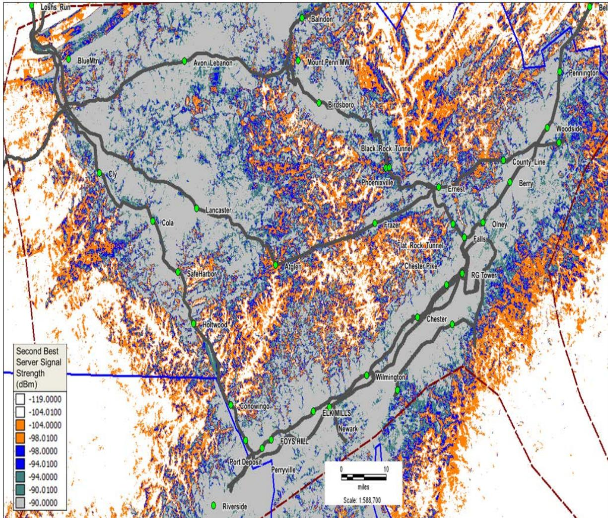
**Figure 52. Predicted Second Best Base Station Server Signal Strength Inside the Philadelphia DUA**
