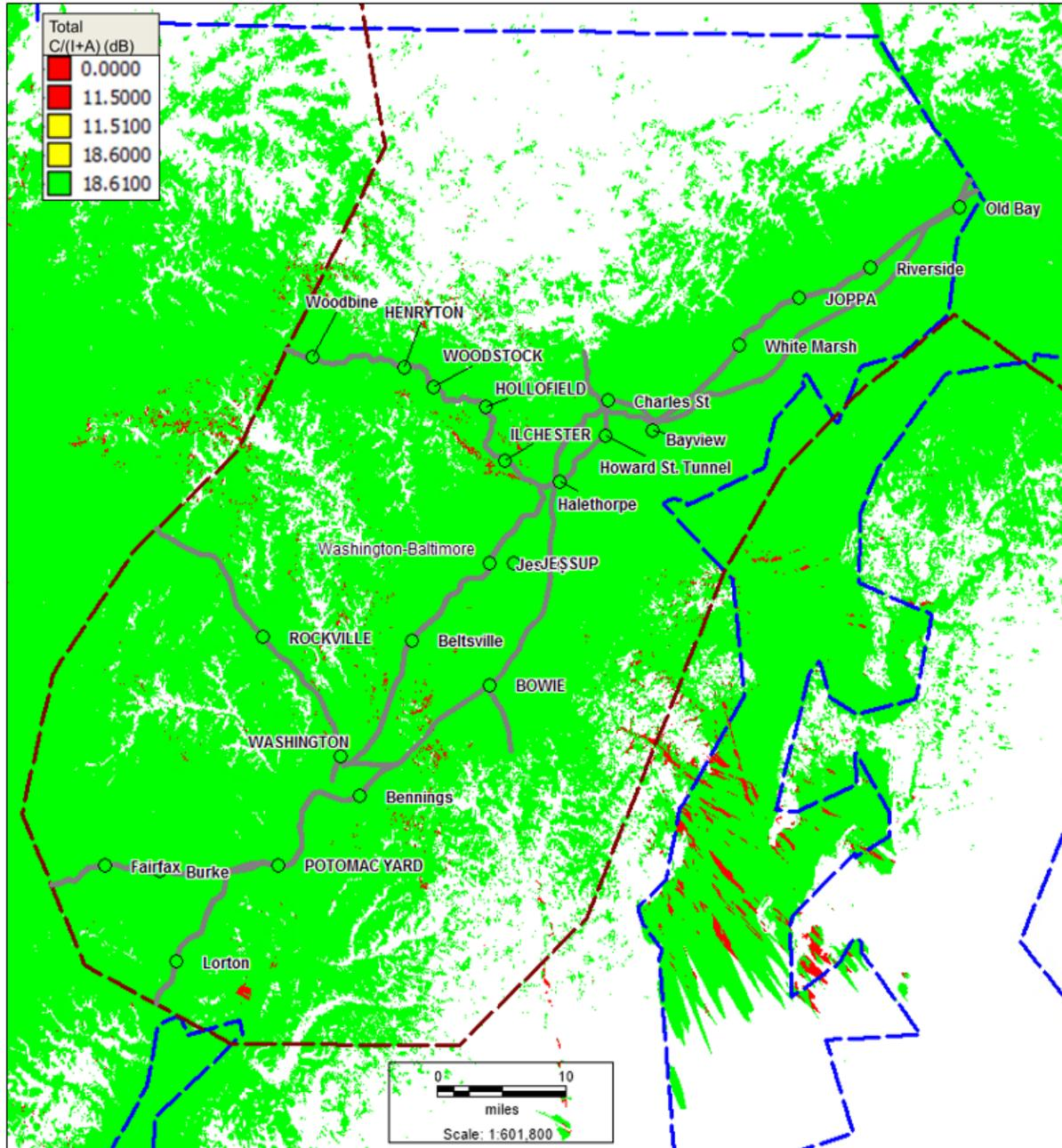
**Figure 72. Predicted C/(I+A) Levels of the ITC Base Station Frequency Plan Prepared for the Washington, D.C. DUA**
