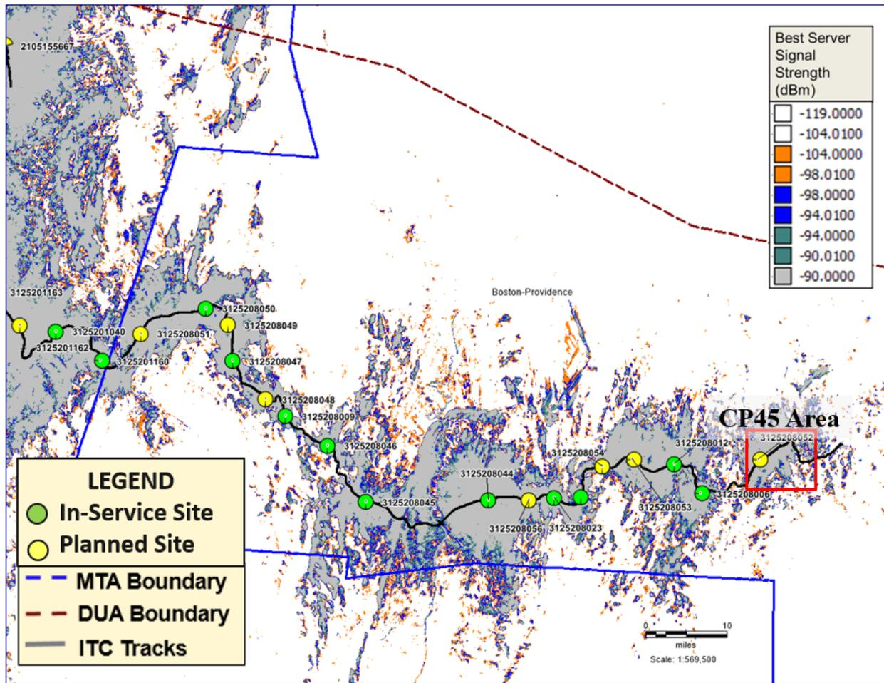
**Figure 83. Best Serving ITC Base Station Signal Strength Inside the Boston DUA**
