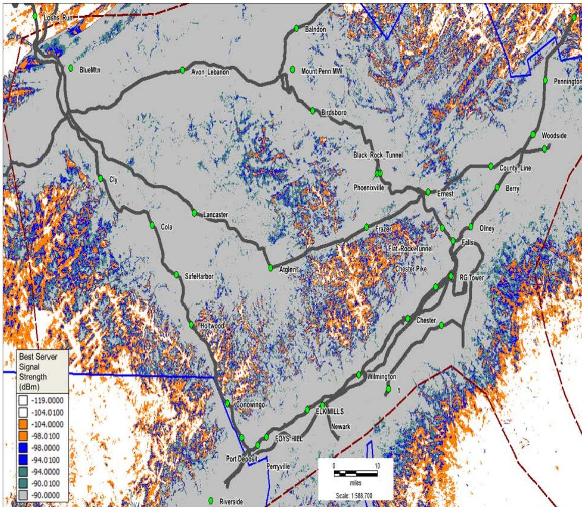
**Figure 49. Predicted Best Serving Base Station Signal Strength Inside the Philadelphia DUA**
