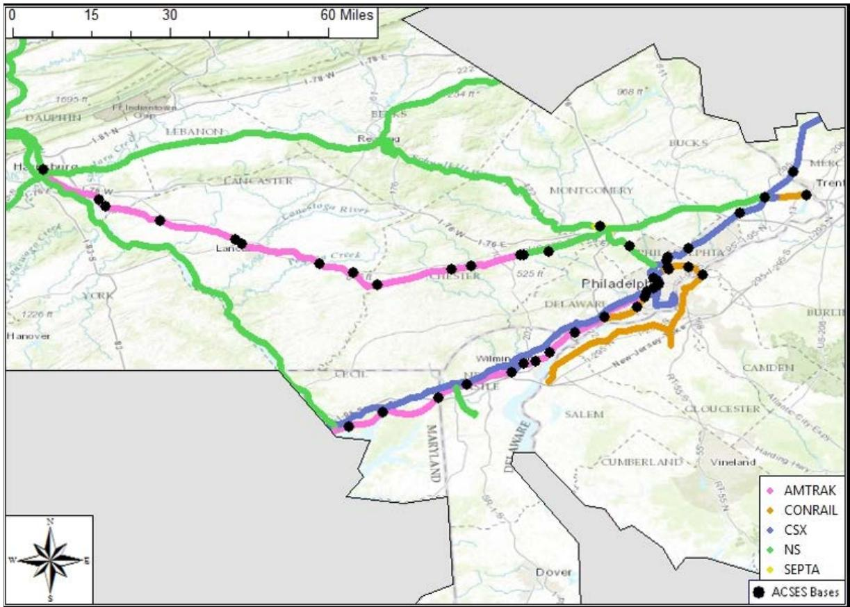
**Figure 47. Location of ACSES Base Stations Predicted to be Desensed by ITC Locomotives in the Philadelphia DMA**
