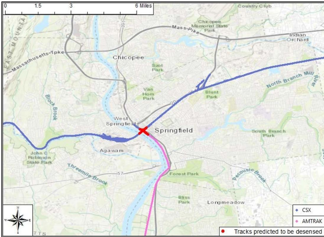
**Figure 81. ITC-Controlled Tracks from CXS Predicted to be Desensed by Amtrak ACSES Base Station Near Springfield**
