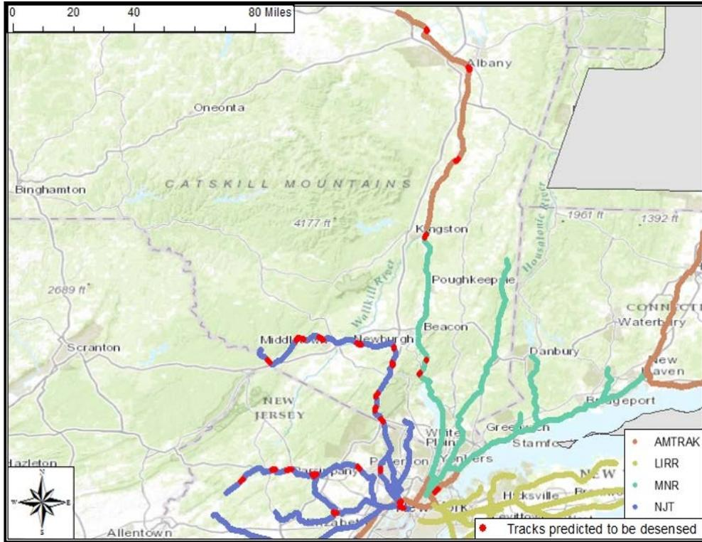
**Figure 25. Location of ACSES-Controlled Tracks Predicted to be Desensed by ITC Sites in the New York DUA**
