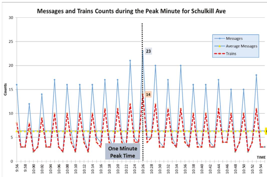
**Figure 55. Counts of Train Messages/Minute During the One-Hour Around the Peak Period for Base Station Schukill Ave**
