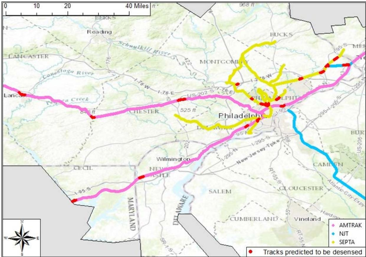
**Figure 46. Location of ACSES-Controlled Tracks Predicted to be Desensed by ITC Base Stations in the Philadelphia DUA**
