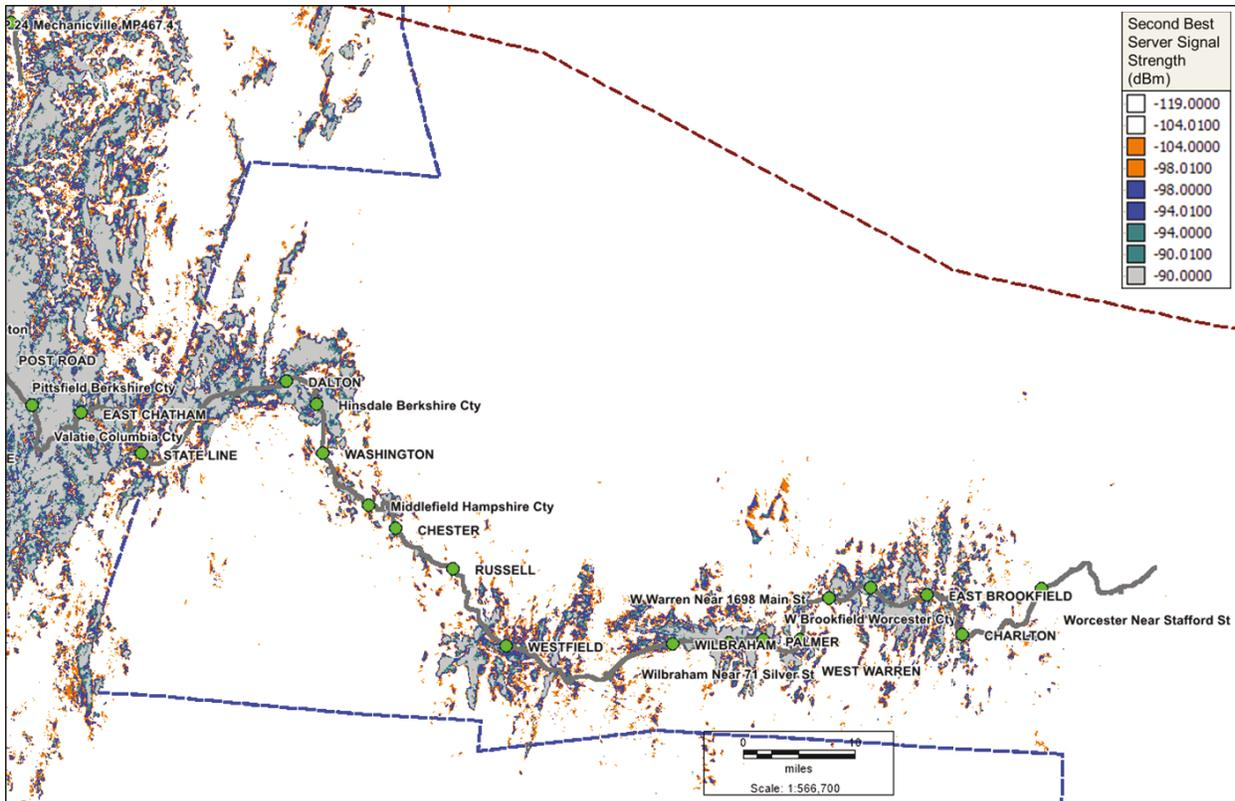
**Figure 86. Predicted Second Best ITC Base Station Server Signal Strength for the Boston DUA**
