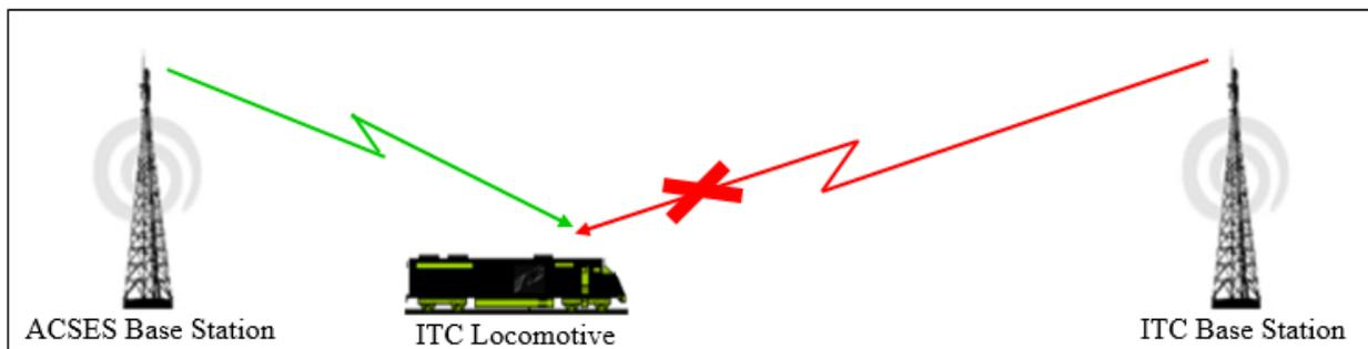
**Figure 3. Illustration of a Fixed ACSES Site Desensing an ITC Locomotive**
