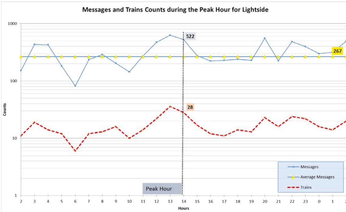
**Figure 36. Counts of Train Messages/Minute During the 24-Hour Window Around the Peak Period for Base Station Lightside**
