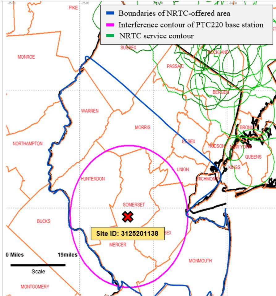
**Figure 15. Evaluation of the Usability of NRTC Spectrum for ITC Site ID 3125201138**
