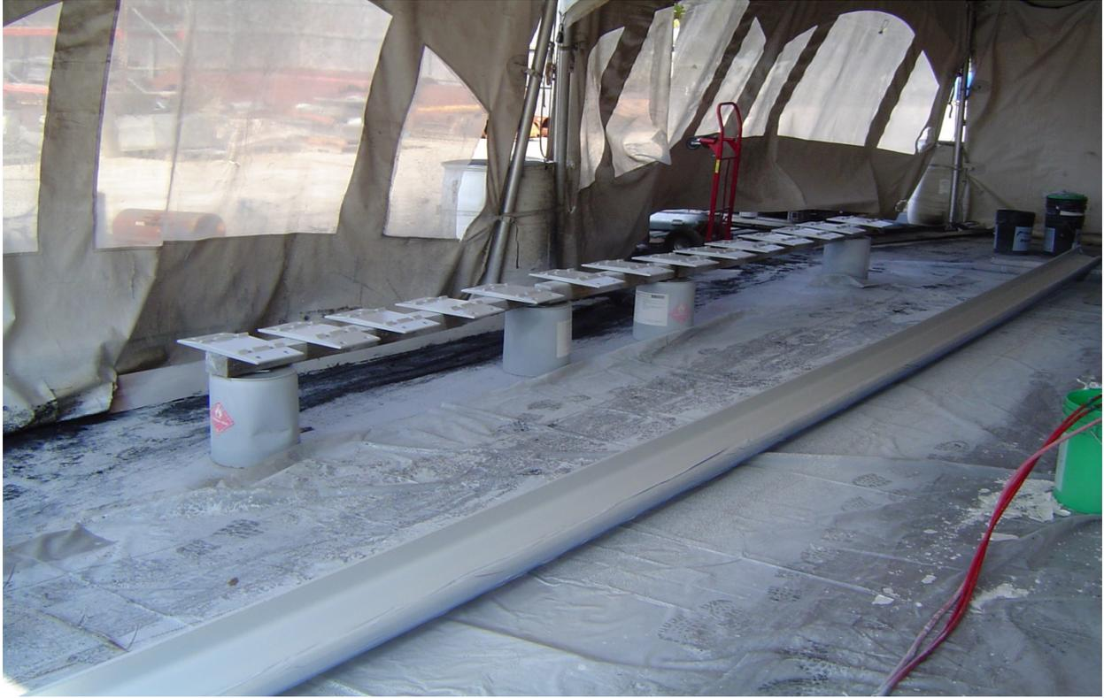
**Figure 2. Rail Segments and Tie Plates Treated with EonCoat® at the EWI Facility**
