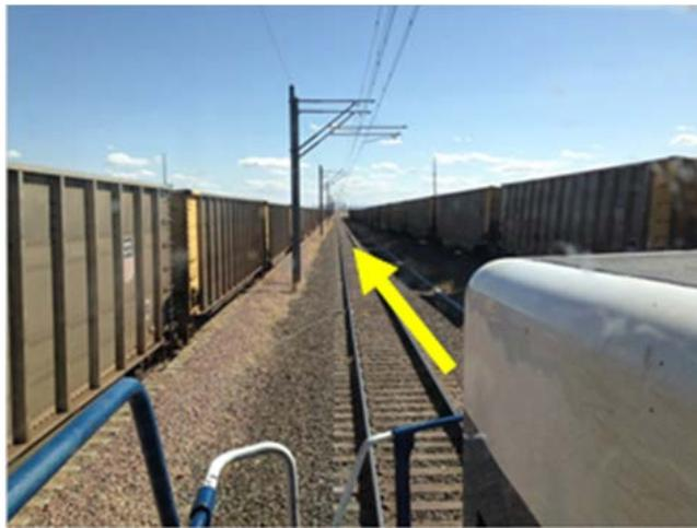
**Figure 15. Multipath testing with operation between adjacent cars**
