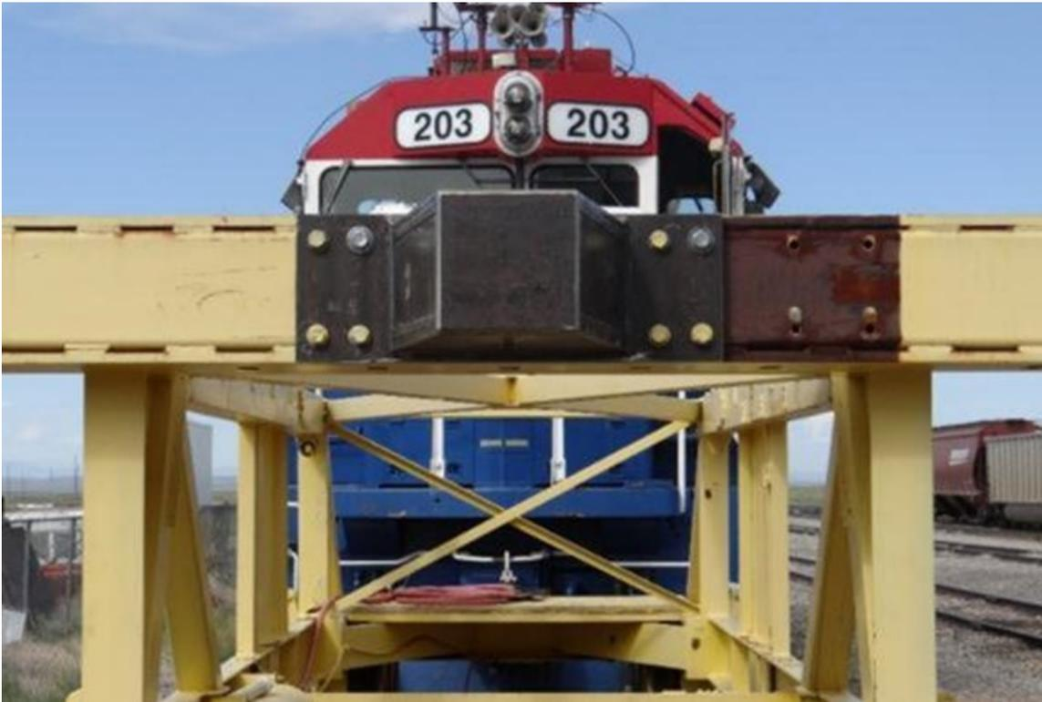
**Figure 5. Impact Cart with Impactor Attached**
