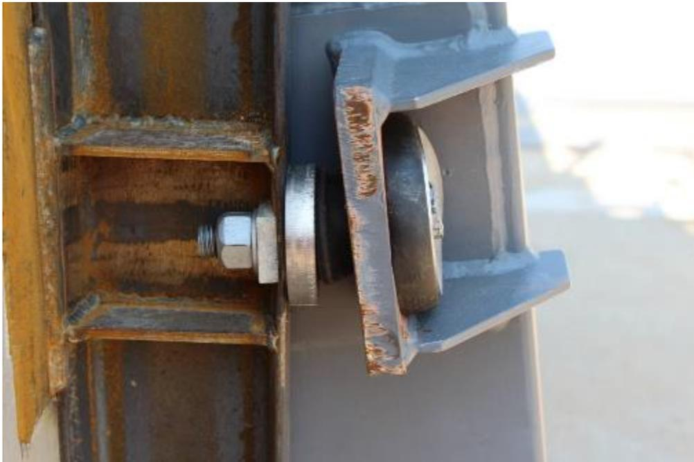
**Figure 22. Deformed Tank Mount**
