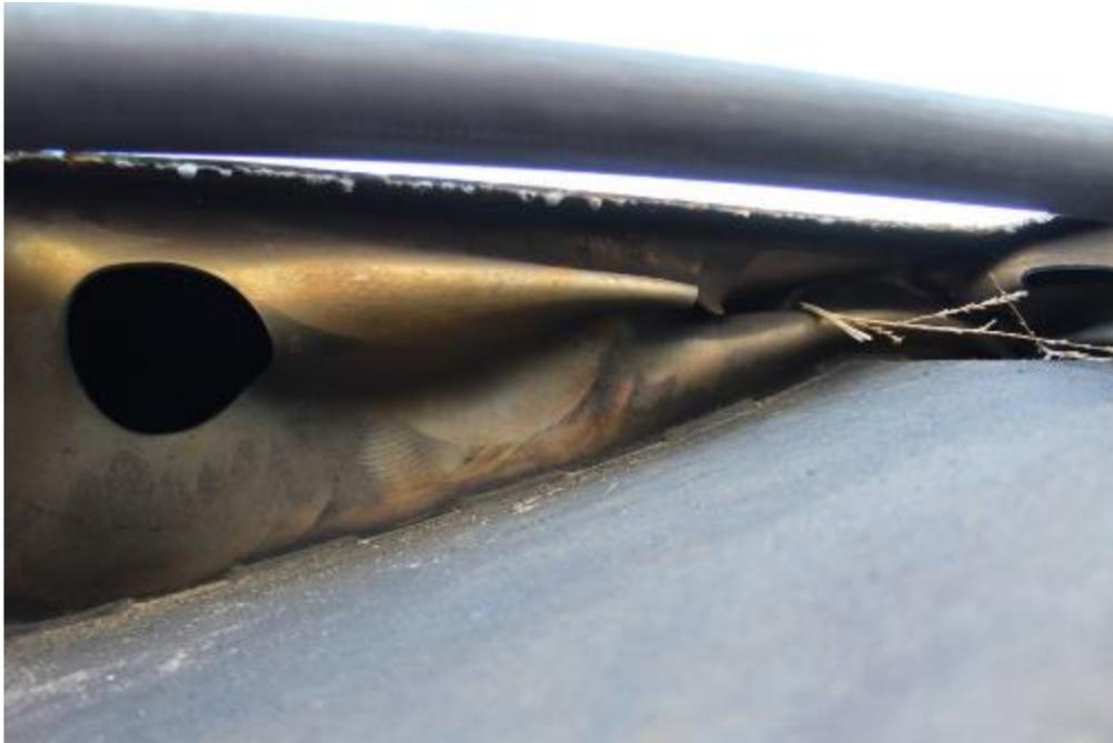
**Figure 21. Interior Baffle Deformation**
