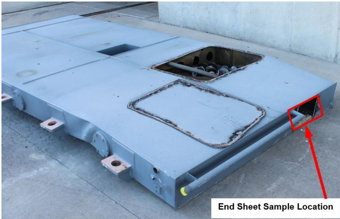
**Figure 14. Fuel Tank End Sheet Sample**
