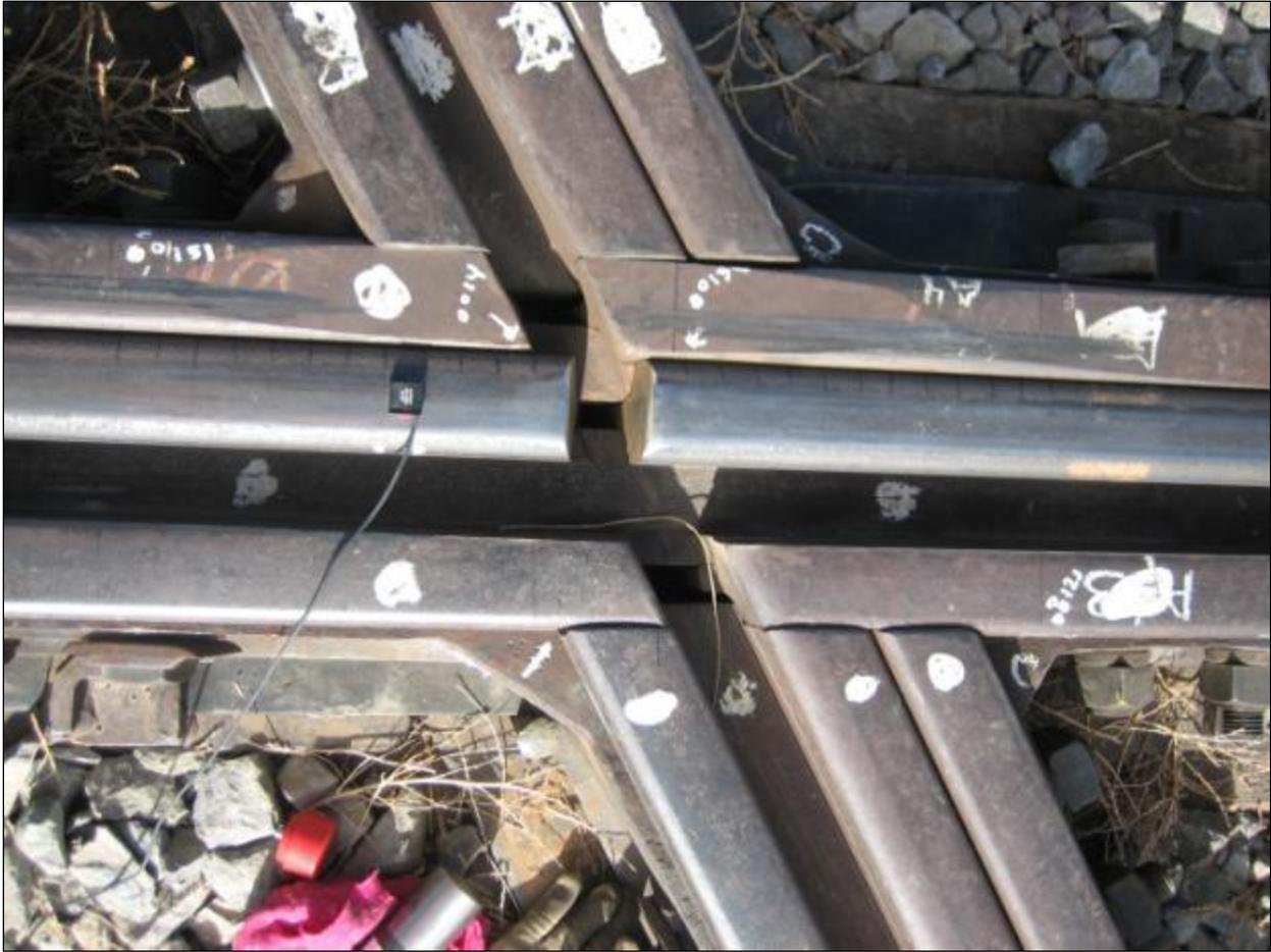
**Figure 18. Hammer Test on the Flexible Gap Corner of Three-Rail Crossing**
