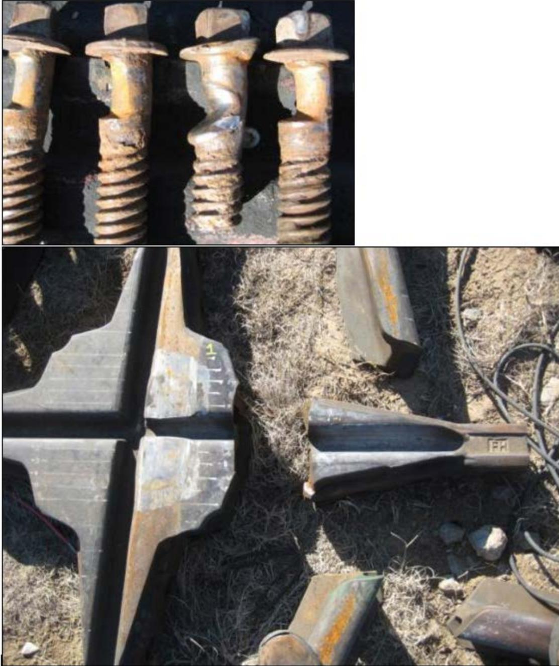
**Figure 4. Components Failures in Cast Crossing**
