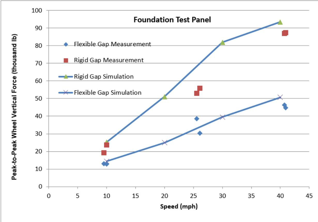
Figure 28. Comparison of Predicted and Measured W/R Impact Forces
