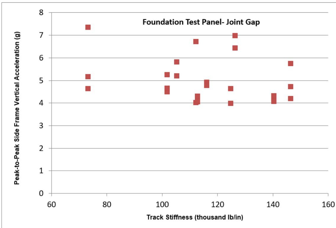
Figure 23. Effect of Track Stiffness (Flexible Joint Gap Side) on Side Frame Acceleration
