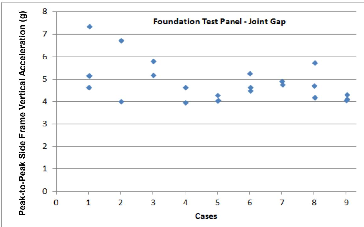
Figure 22. Side Frame Vertical Accelerations Over Flexible Joint Gap
