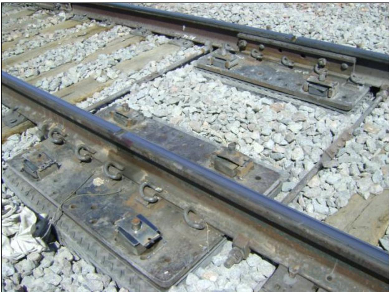
**Figure 5. Scaled Test Panel with Two Different Types of Gaps (Lower Rail – Rigid Gap, Upper Rail – Flexible Gap)**
