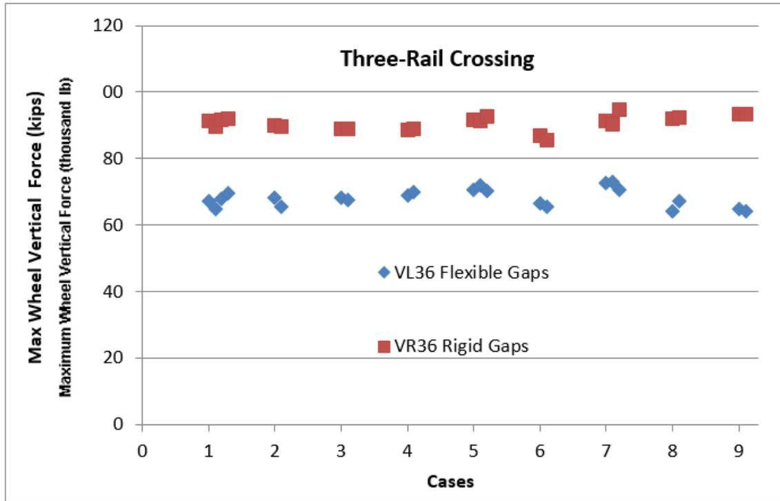
Figure 12. Maximum W/R Impact Forces on Full-Scale Three-Rail Crossing
