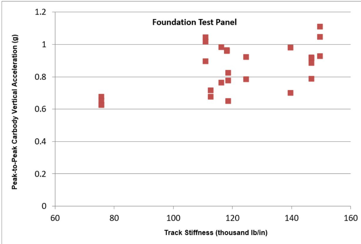
**Figure 21. Effect of Track Stiffness on Carbody Acceleration**
