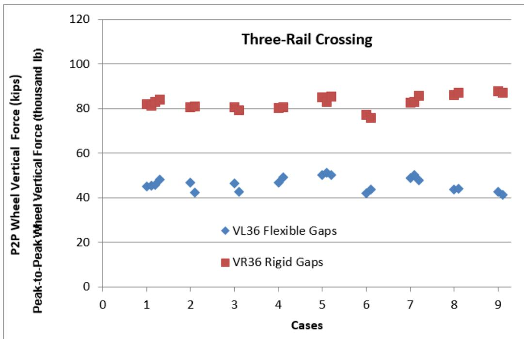
Figure 13. Peak-to-Peak W/R Impact Forces on Full-Scale Three-Rail Crossing
