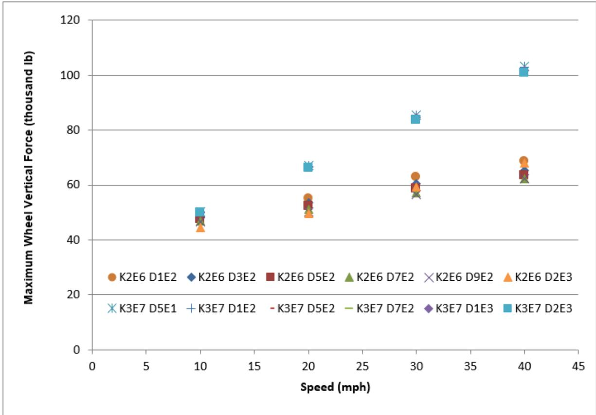
**Figure 31. Effect of Gap Damping on W/R Impact (Connection Stiffness Between Rail and Ground  $K = 50,000$  lb/in)**
