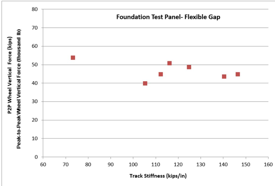
**Figure 16. Effect of Track Stiffness on Flexible Joint Gap Impact**
