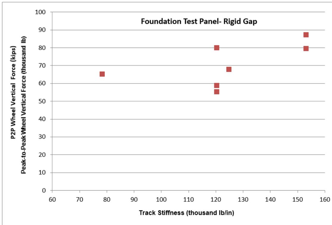
**Figure 15. Effect of Track Stiffness on Rigid Gap Impact**
