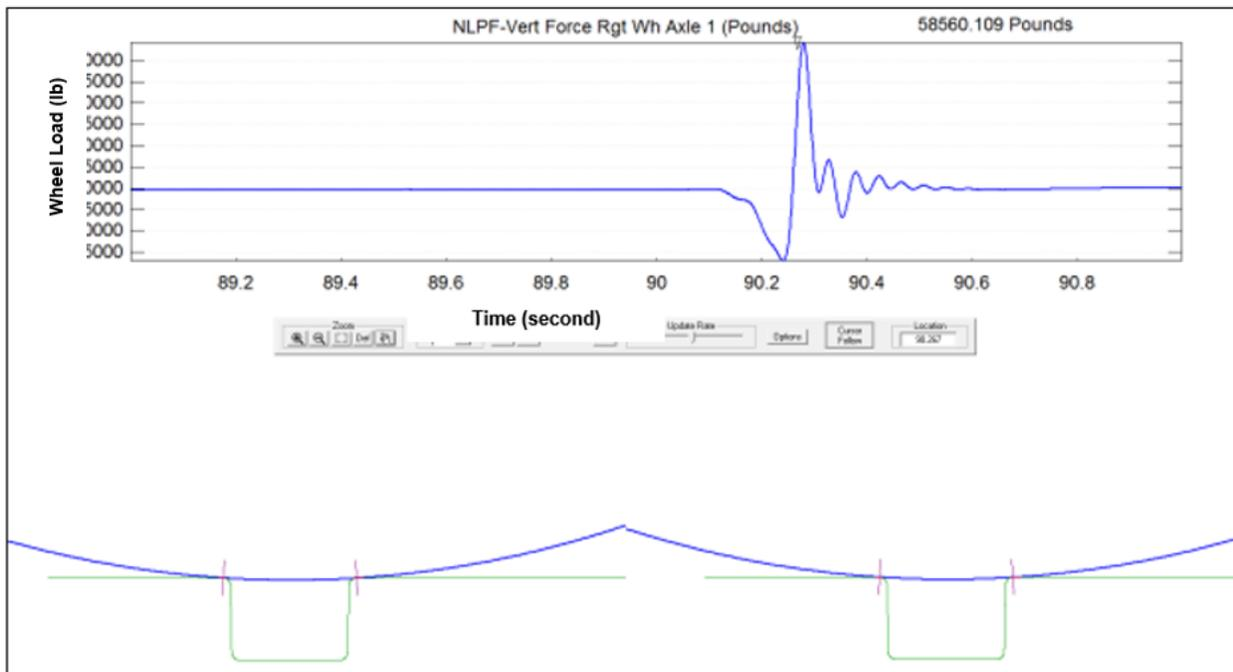
**Figure 26. Vertical W/R Impact on a Rigid Gap (Connection Stiffness Between Rail and Ground  $K = 50,000$  lb/in, 40 mph)**
