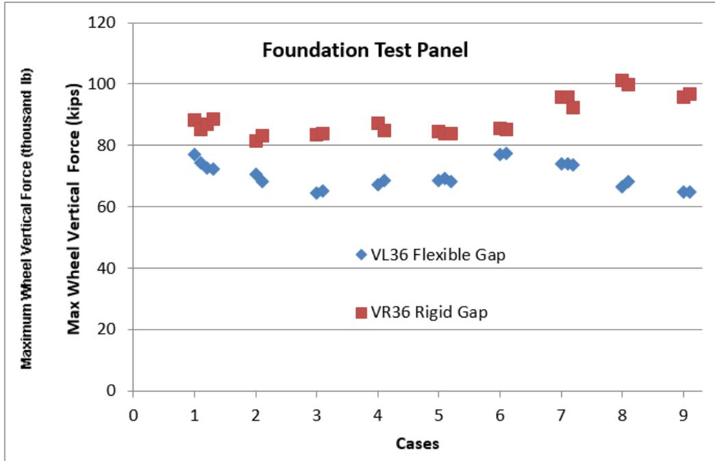
Figure 9. Maximum W/R Impact Forces on Scaled Panel (315, 000 lb. Car, 40 mph)
