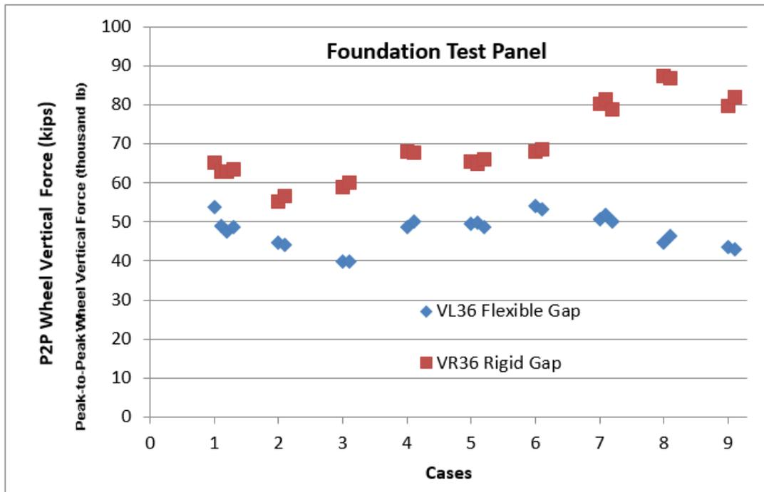
Figure 10. Peak-to-Peak W/R Impact Forces on Scaled Panel (315,000 lb. Car, 40 mph)
