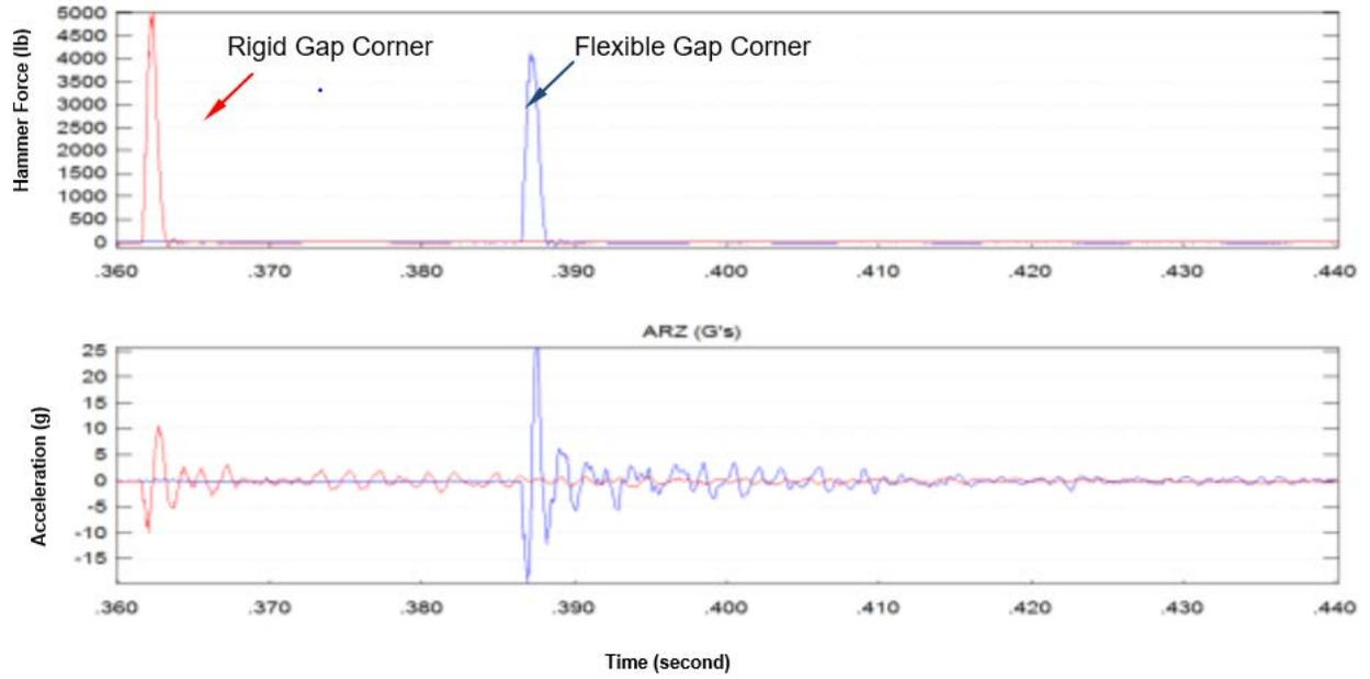
**Figure 19. Hammer Impact and Rail Response on Three-Rail Crossing**
