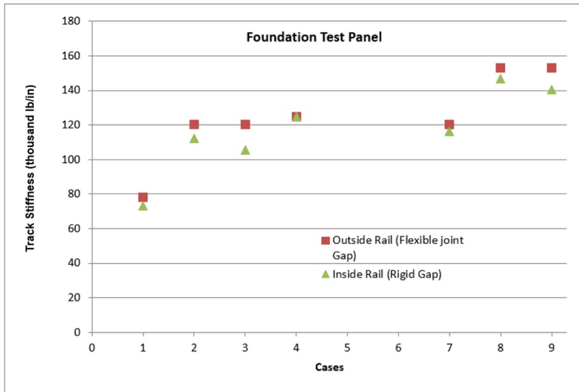
Figure 14. Measured Track Stiffness for Test Cases
