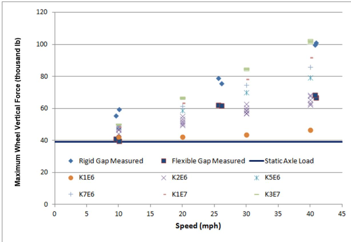
**Figure 30. Effect of Flexible Gap Stiffness and Damping on W/R Impact**
