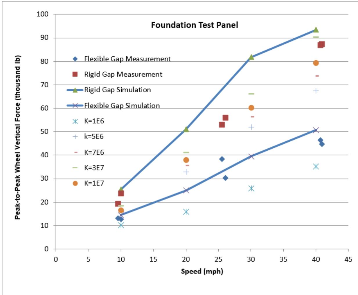
**Figure 29. Effect of Gap Stiffness on W/R Impact Over Flangeway Gap (Connection Stiffness Between Rail and Ground  $K = 50,000$  lb/in, Gap Flexibility  $D_2 = 700$  lb/in/s)**
