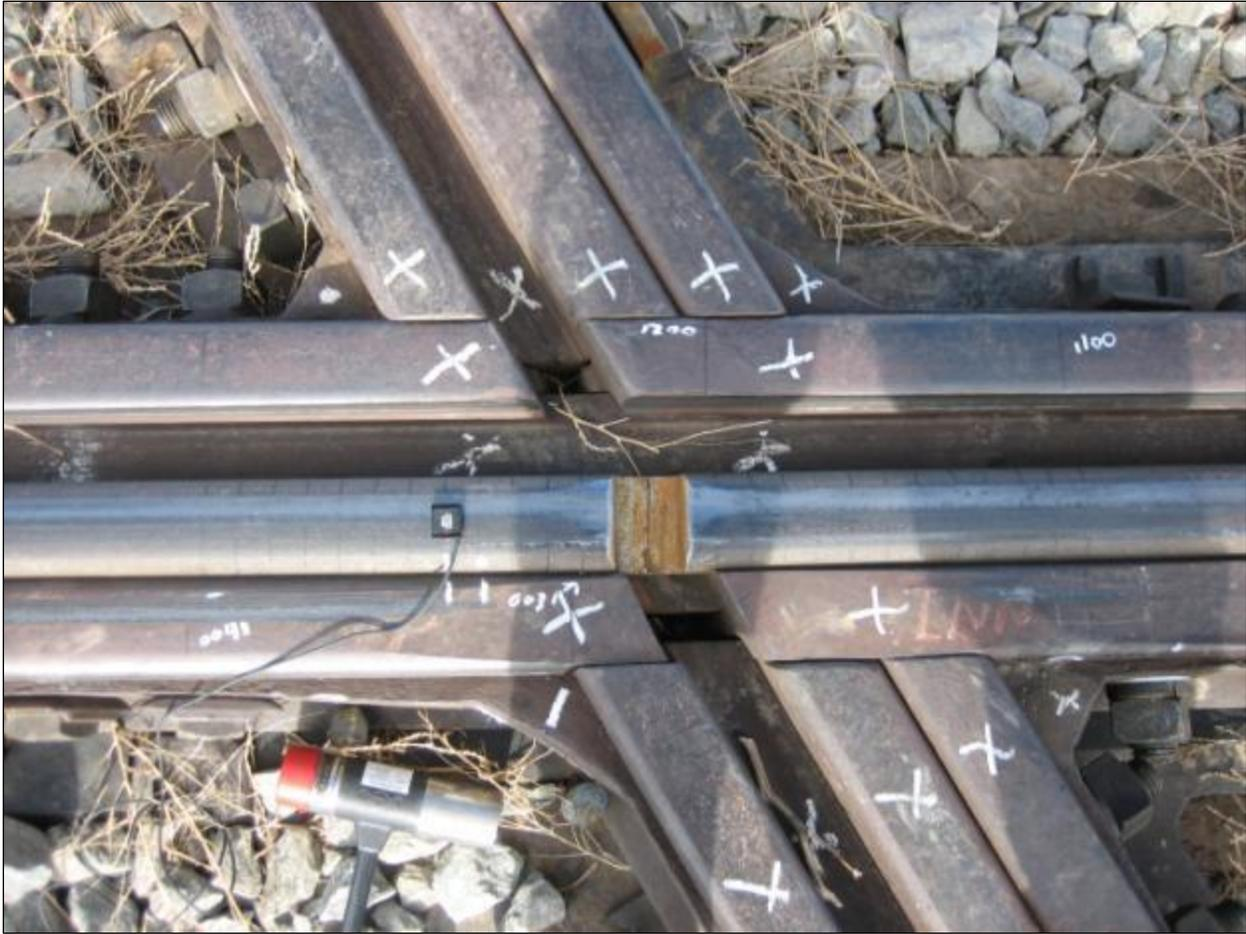
**Figure 17. Hammer Test on the Rigid Gap Corner of Three-Rail Crossing**
