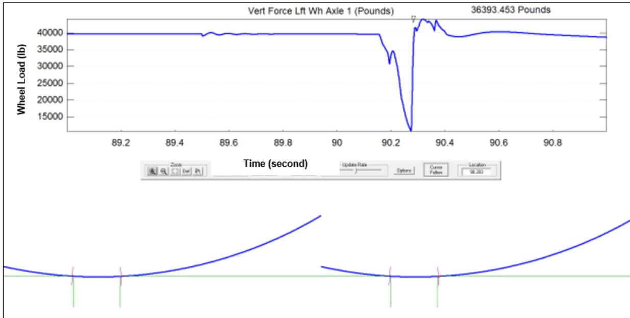
**Figure 27. Vertical W/R Impact on a Flexible Gap (Connection Stiffness Between Rail and Ground  $K = 50,000$  lb/in, Gap Flexibility  $K_2 = 1,000,000$  lb/in,  $D_2 = 700$  lb/in/s, 40 mph)**
