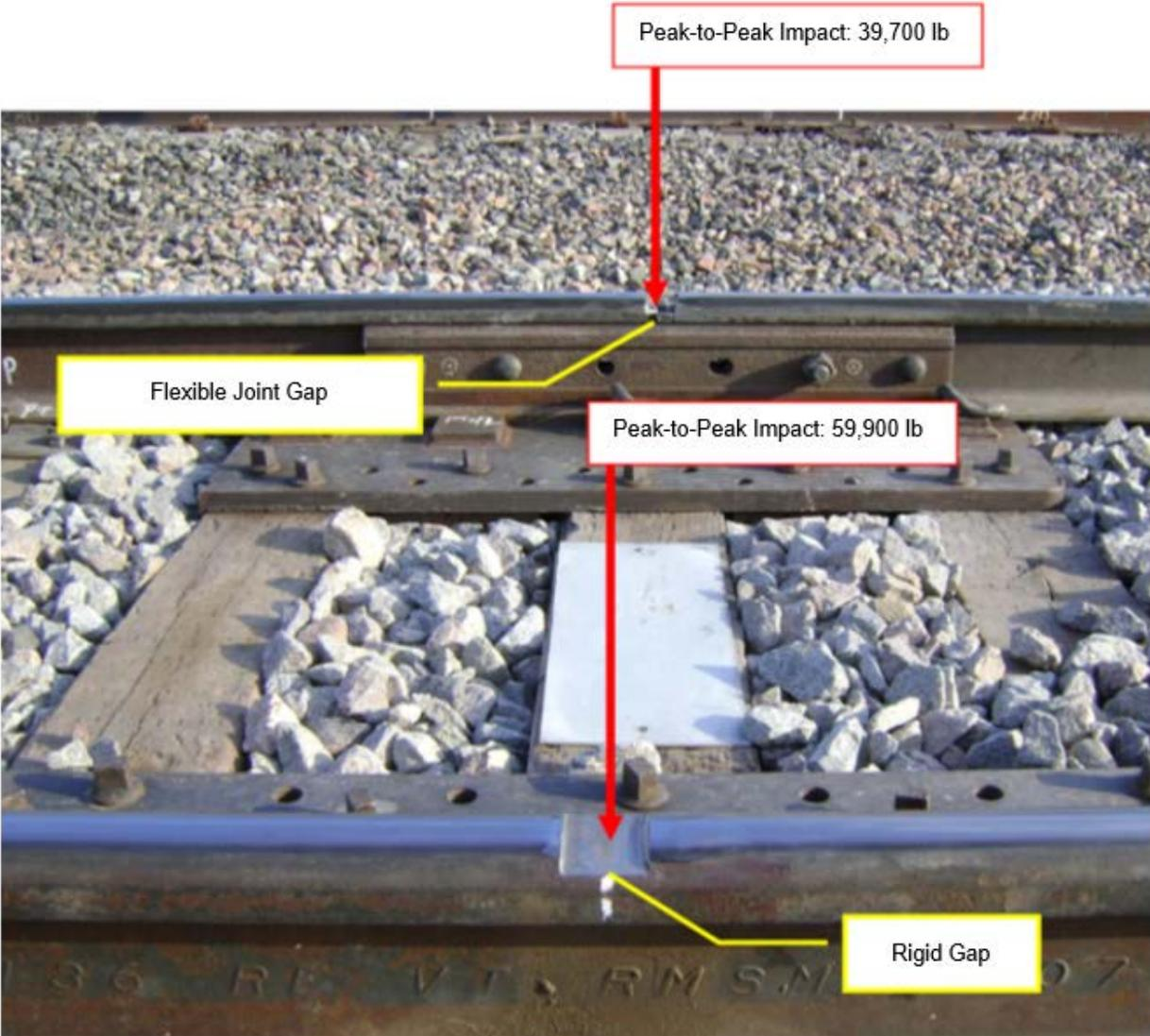
**Figure 8. Peak-to-Peak Impact Comparison (Panel Test Case 3)**
